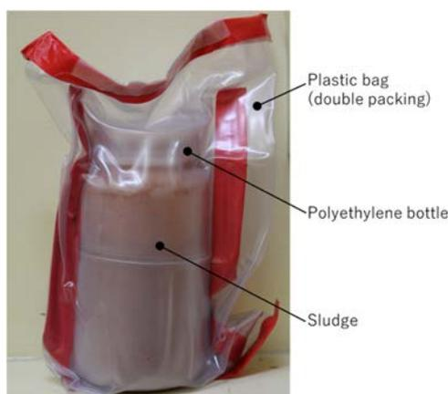
Figure 7.1 Plastic bottle used for sludge items before stabilization
