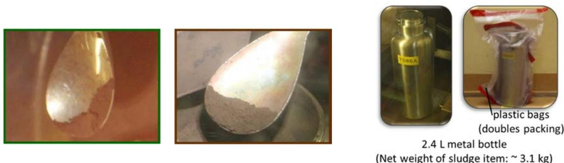
Figure 4.3 The sludge after stabilization and storage conditions
