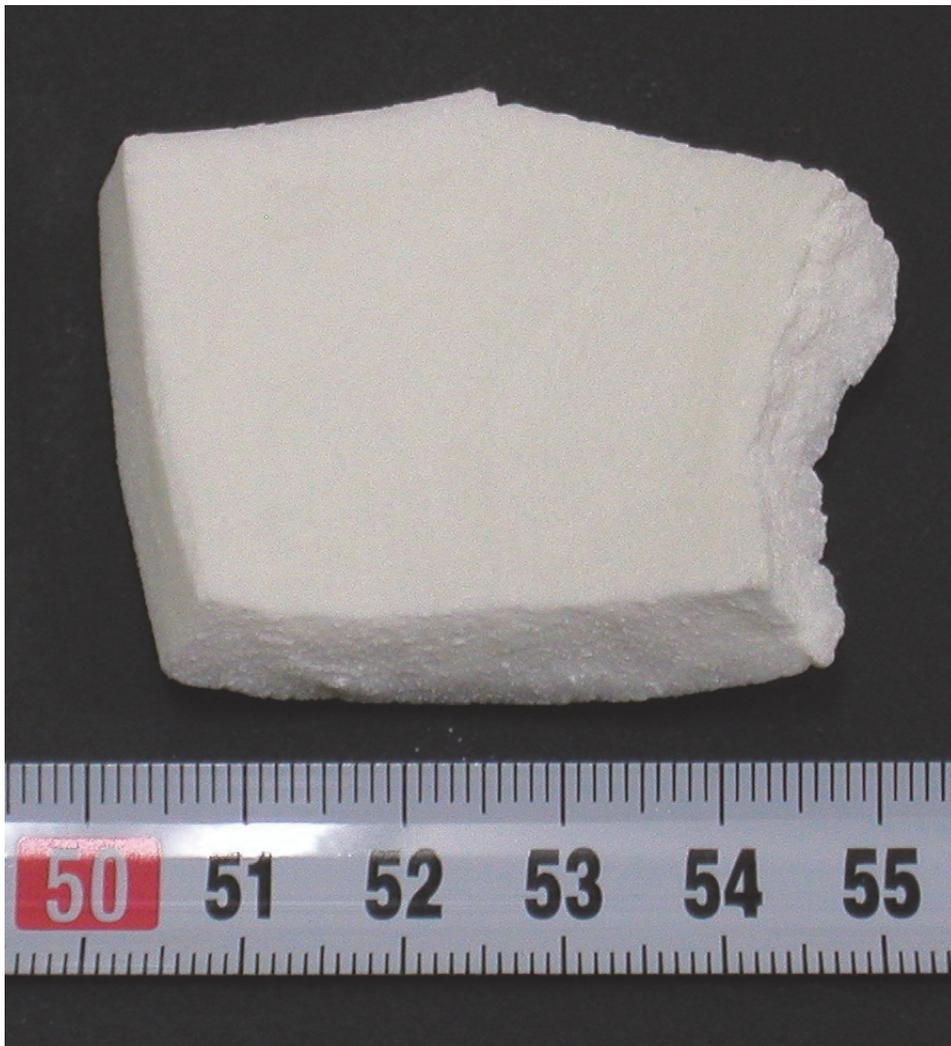
Fig.7 A lump of the dried hydrous titanic acid.
