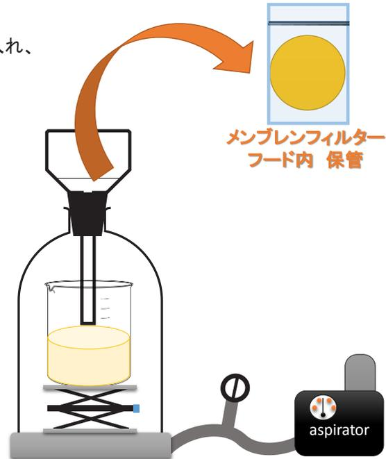
Fig.3.4(13)  $^{90}\text{Sr}$  の分析作業手順
