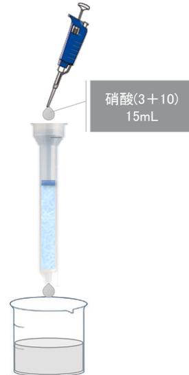
Fig.3.2(51)  $^{63}\text{Ni}$  の分析作業手順
