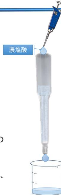
Fig.3.2(25)  $^{63}\text{Ni}$  の分析作業手順
