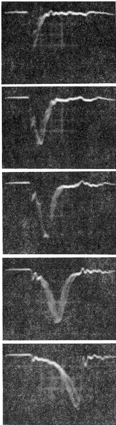
Photo 14.3 Waveform of energy monitor current as a function of beam energy. The beam pulse width is 0.0625\mu\text{sec} (abscissa 0.02\mu\text{sec/division} ).
