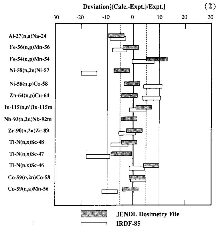
Fig. 4.1.3(a) Deviations of calculated reaction rates from measured ones for the spectrum #1.
