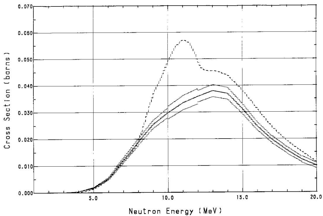
**Fig. A.38**  $^{63}\text{Cu}(n, \alpha)^{60}\text{Co}$  cross section
