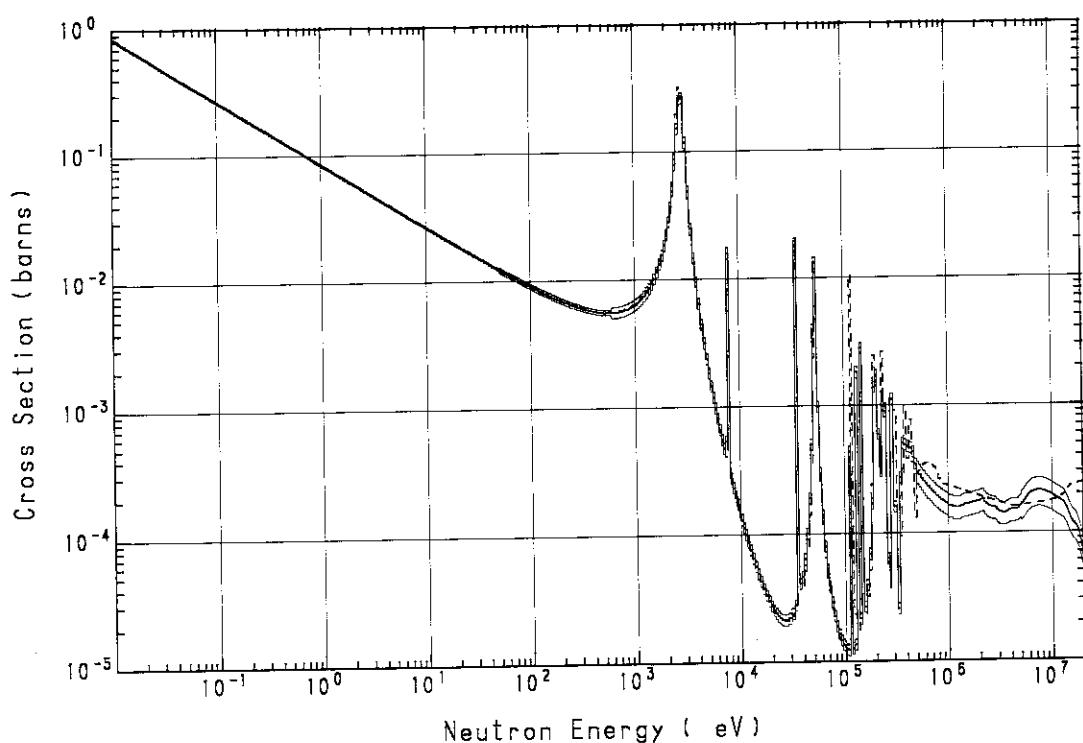
Fig. A.8  $^{23}\text{Na}(n, \gamma)^{24}\text{Na}$  cross section
