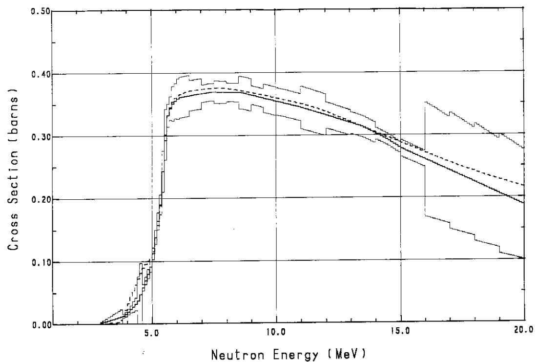
**Fig. A.3**  ${}^7\text{Li}$  t production cross section
