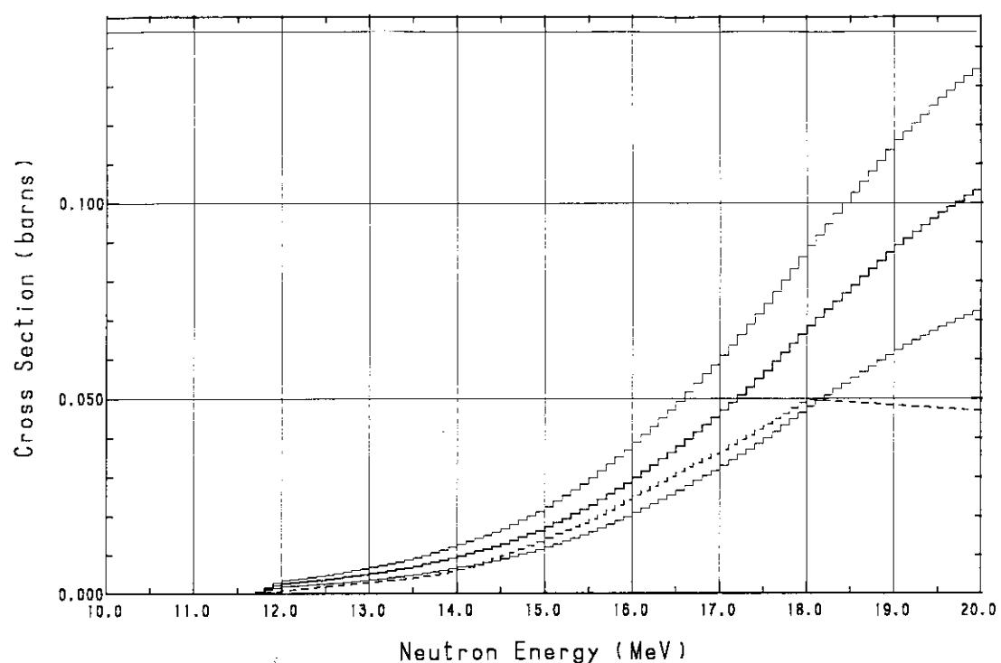
Fig. A.21  $^{48}\text{Ti}(\text{n},\text{np})^{47}\text{Sc}$  cross section
