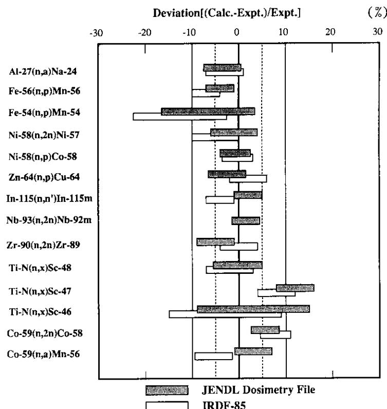
Fig. 4.1.3(b) Deviations of calculated reaction rates from measured ones for the spectrum #2.
