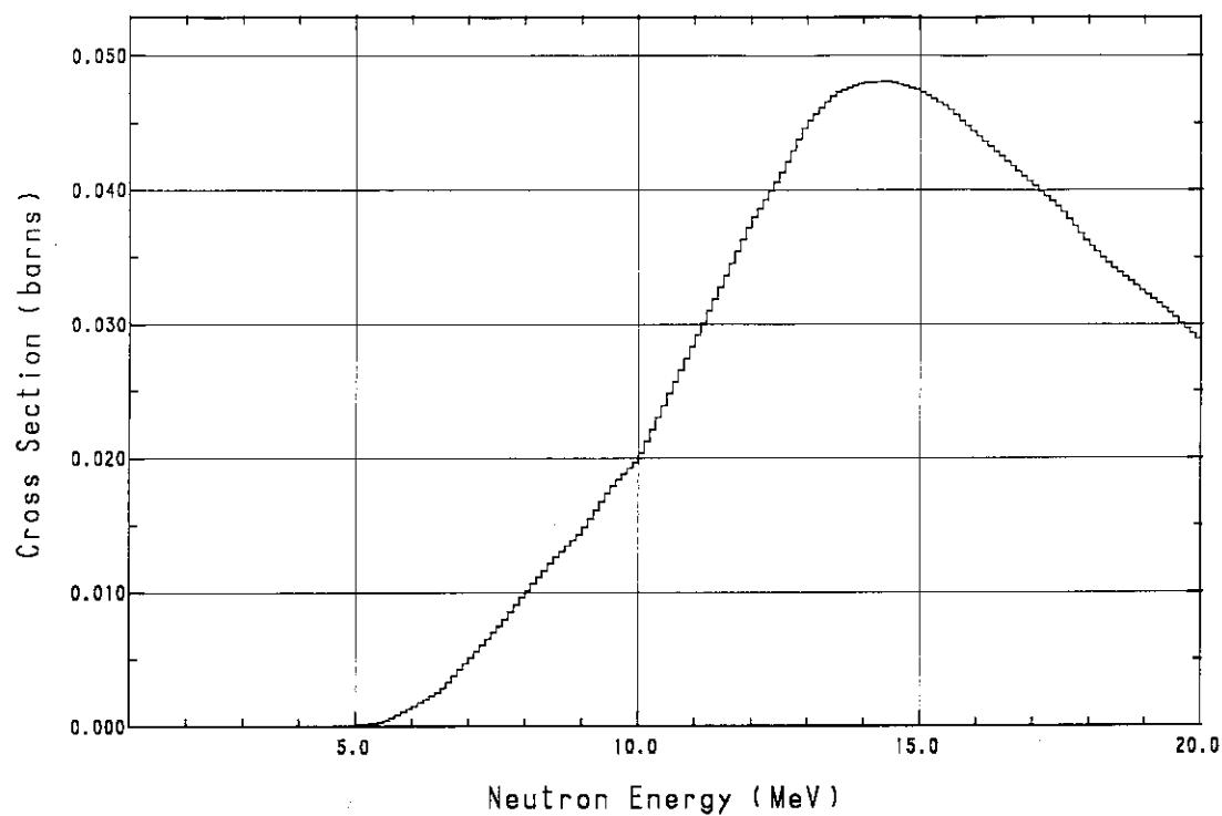
Fig. A.17  $\text{Ti}(n, x)^{48}\text{Sc}$  cross section
