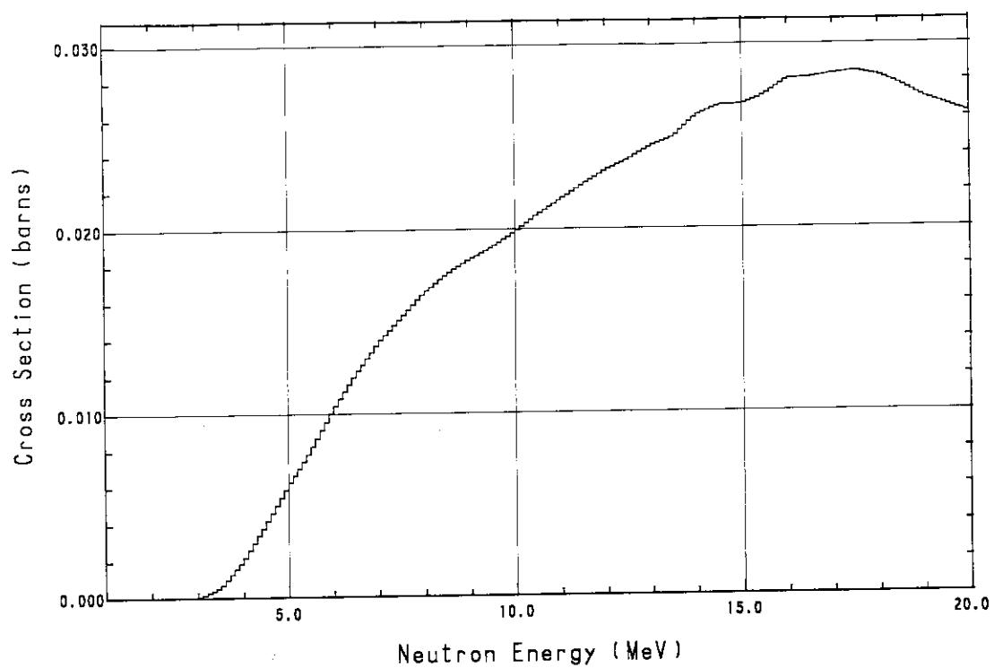
Fig. A.15  $\text{Ti}(n, x)^{46}\text{Sc}$  cross section
