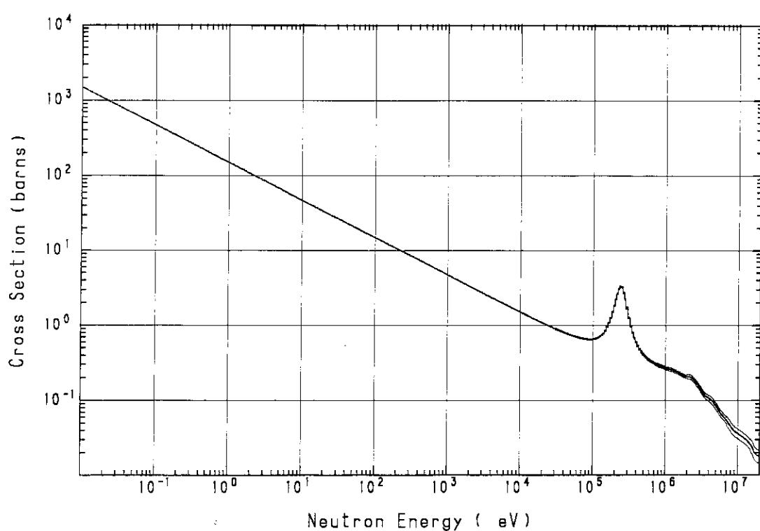
Fig. A.1  ${}^6\text{Li}(n, t)\alpha$  cross section
