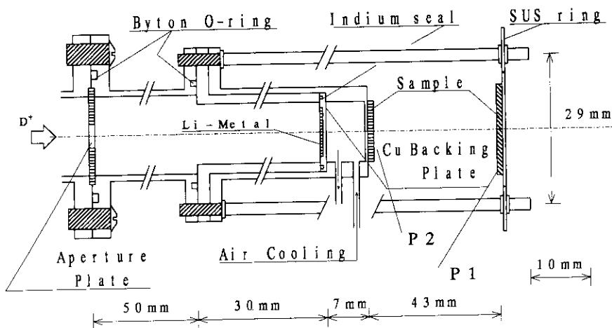
**Fig. 4.2.1** The lithium metal target assembly.
