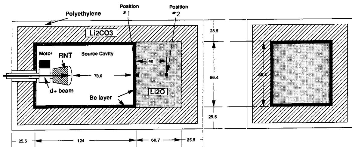
**Fig. 4.1.1** Cross sectional view of the Phase-II B system. (unit of length is cm)
