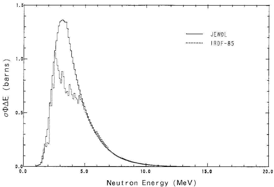
**Fig. 3.1.3** Contributions to the  $^{252}\text{Cf}$  spontaneous fission spectrum average values of  $^{31}\text{P}(\text{n}, \text{p})^{31}\text{Si}$  reaction cross section.
