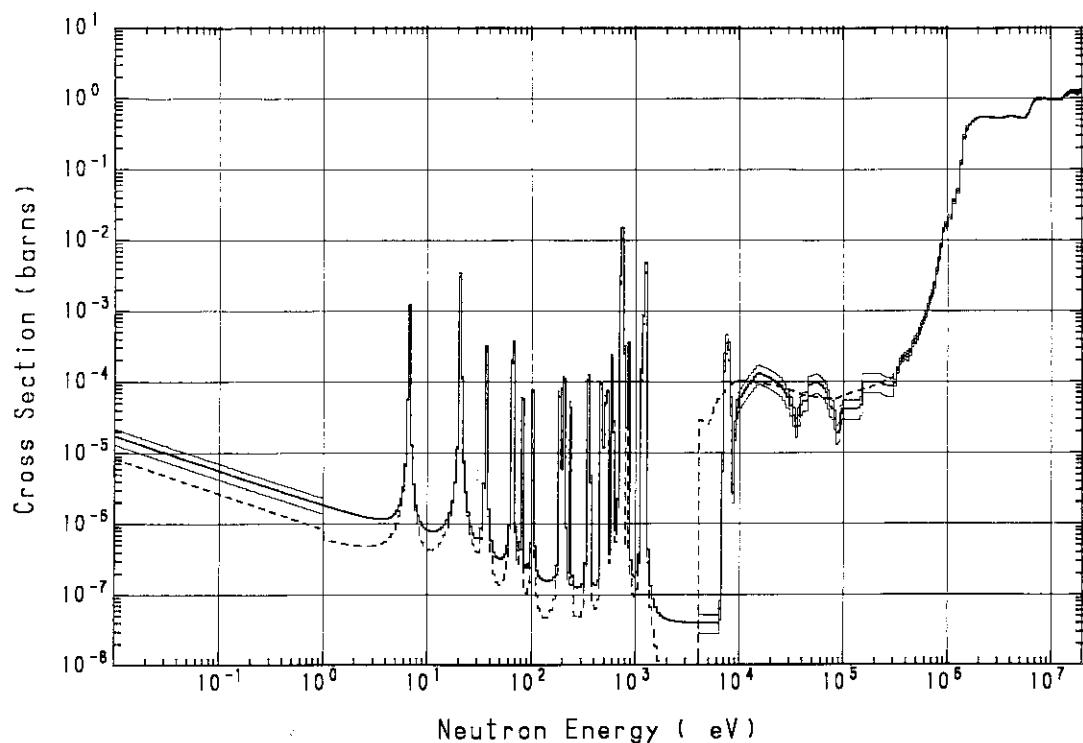
Fig. A.57  $^{238}\text{U}$  fission cross section
