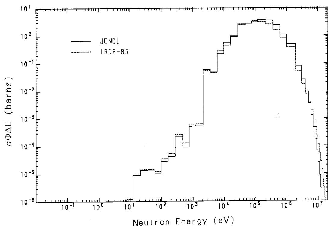
**Fig. 3.1.10** Contributions to the BIG-TEN spectrum average values of  $^{45}\text{Sc}$  ( $n, \gamma$ )  $^{46}\text{Sc}$  reaction cross section.
