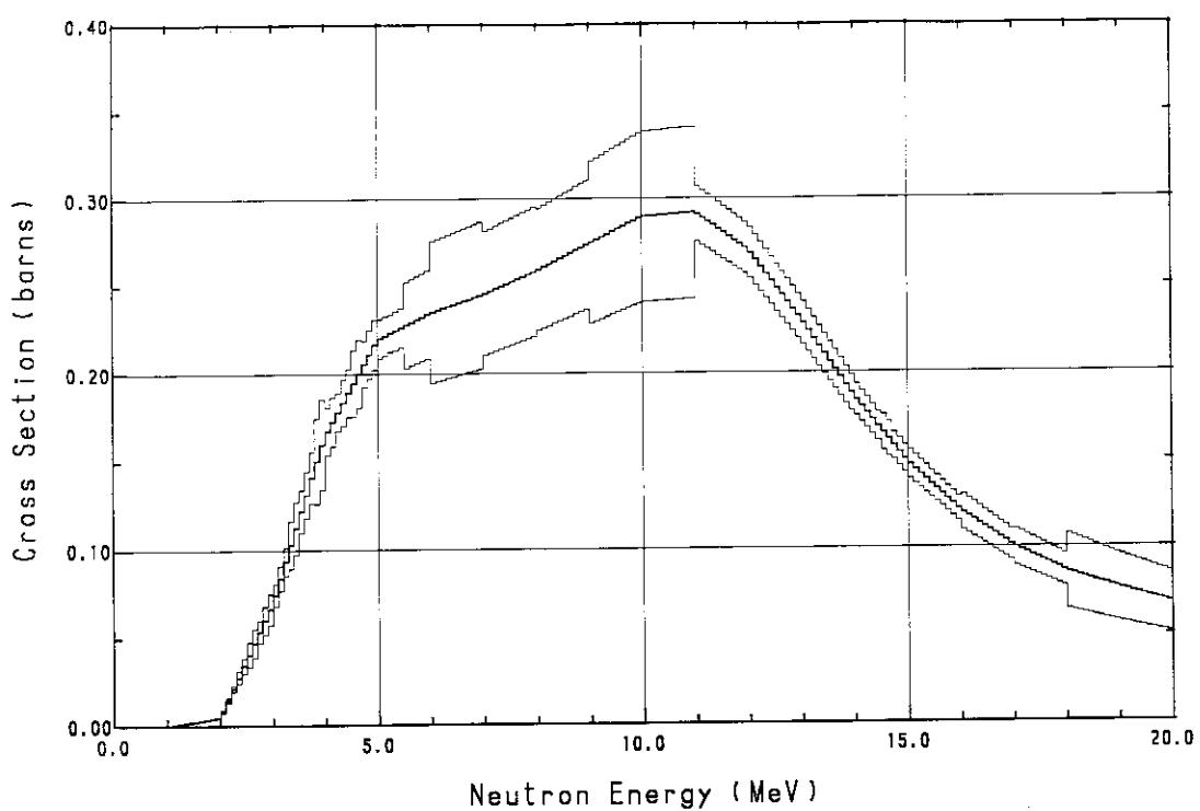
Fig. A.40  $^{64}\text{Zn}(\text{n}, \text{p})^{64}\text{Cu}$  cross section
