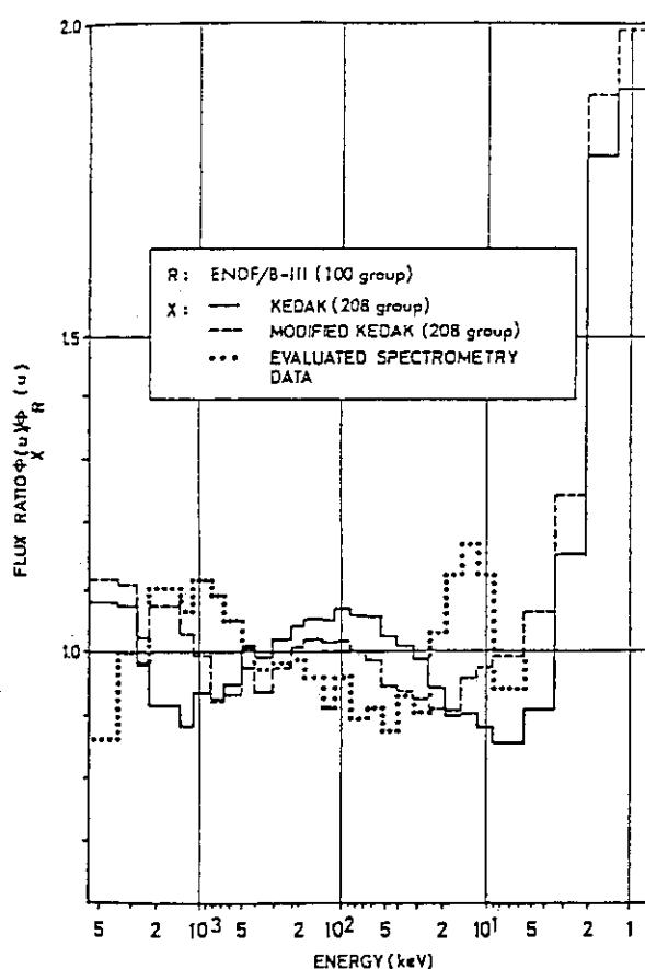
**Fig. 3.3.6** Comparison of discrete-ordinate transport calculations and evaluated spectrometry measurements of the  $\Sigma\Sigma$  central neutron spectrum. (all data are collapsed in a similar multigroup structure and ratios are calculated relatively to the ENDF /B-III, S<sub>16</sub>-P<sub>3</sub>, 100-group calculation)
