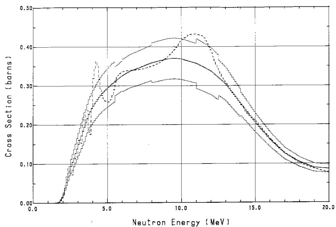
Fig. A.13  $^{32}\text{S}(\text{n}, \text{p})^{32}\text{P}$  cross section
