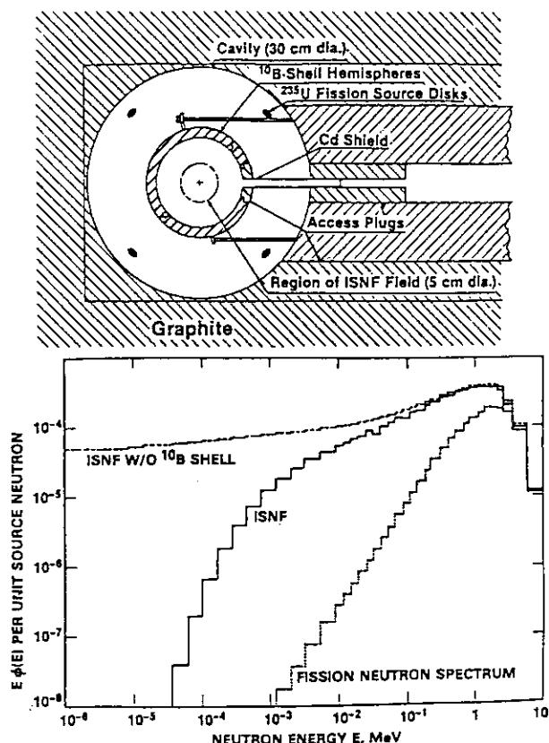
**Fig. 3.3.1** Upper view: The ISNF located within a 30 cm diameter cavity in the thermal column of the NIST reactor.
