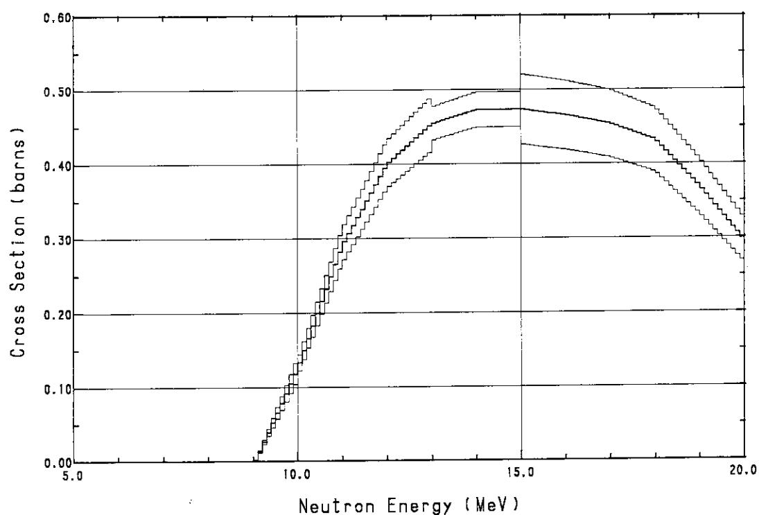
Fig. A.43  $^{93}\text{Nb}(\text{n}, 2\text{n})^{92\text{m}}\text{Nb}$  cross section
