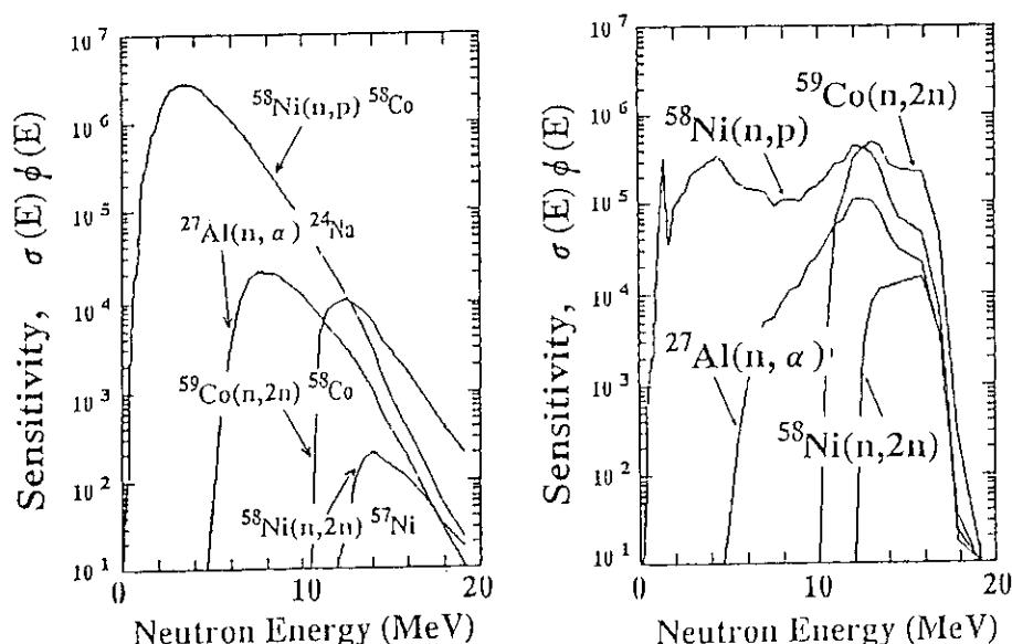
**Fig. 4.2.5** Comparison of the responses of the  $^{58}\text{Ni}(n, p)$ ,  $^{27}\text{Al}(n, \alpha)$ ,  $^{59}\text{Co}(n, 2n)$  and  $^{58}\text{Ni}(n, 2n)$  reactions to the spectra of the  $^{252}\text{Cf}$  spontaneous fission neutrons (left) and thick Li(d, n) source (right), respectively.
