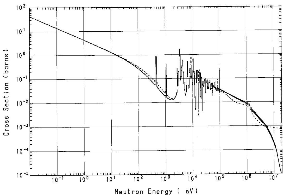
Fig. A.14  $^{45}\text{Sc}(\text{n}, \gamma)^{46}\text{Sc}$  cross section
