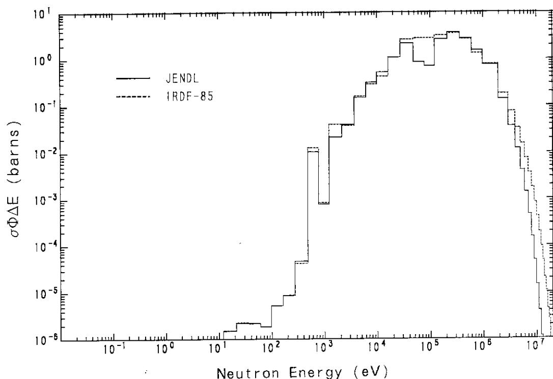
**Fig. 3.1.12** Contributions to the BIG-TEN spectrum average values of  $^{63}\text{Cu}(\text{n}, \gamma)^{64}\text{Cu}$  reaction cross section.
