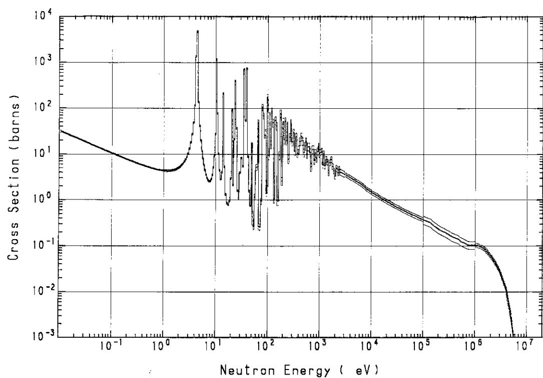
Fig. A.49  $^{181}\text{Ta}(\text{n}, \gamma)^{182}\text{Ta}$  cross section
