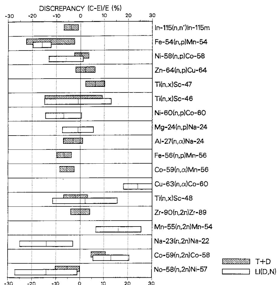
**Fig. 5.2.2** (C-E)/E values of the average cross sections of tested 14 reactions for IRDF-85 in the T+d fusion simulated field and the thick Li (d, n) neutron field.
