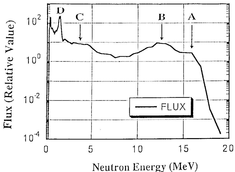
**Fig. 4.2.3** Measured neutron spectra of the thick Li(d, n) neutron source at  $0^\circ$ . Arrows in the figure indicate peaks correspond to the ground state (A) and broad first (B) and fourth (C) excited states of residual nucleus of  ${}^8\text{Be}$ , and a parasitic neutron group from  ${}^{12}\text{C}(\text{d}, \text{n})$  reactions (D).
