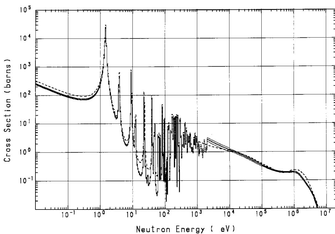
Fig. A.46  $^{115}\text{In}(n, \gamma)$   $^{116\text{m}}\text{In}$  cross section
