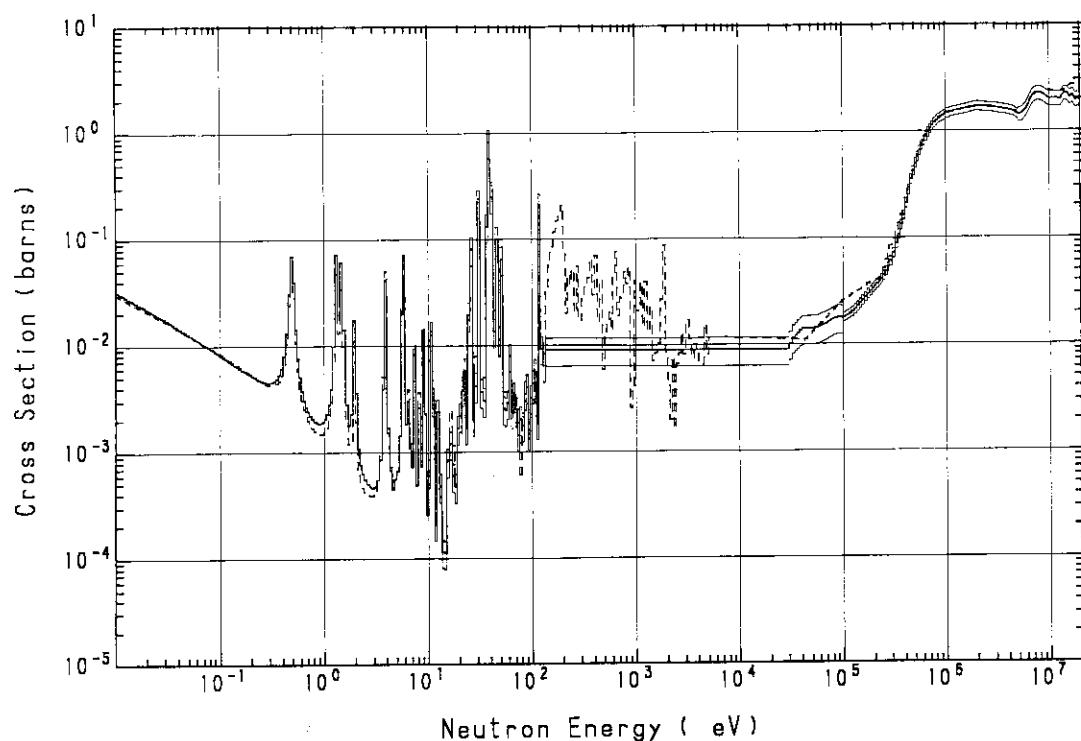
Fig. A.59  $^{237}\text{Np}$  fission cross section
