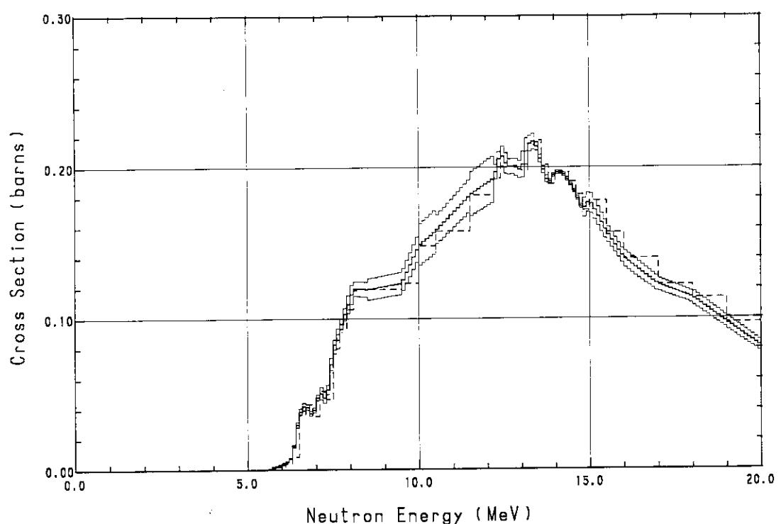
Fig. A.9  $^{24}\text{Mg}(\text{n}, \text{p})^{24}\text{Na}$  cross section
