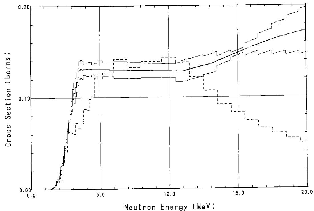
Fig. A.12  $^{31}\text{P}(\text{n}, \text{p})^{31}\text{Si}$  cross section
