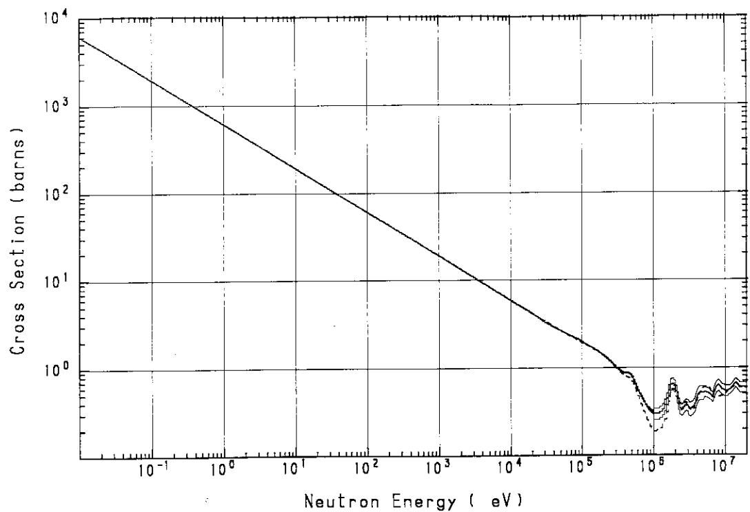
Fig. A.5  $^{10}\text{B}$   $\alpha$  production cross section
