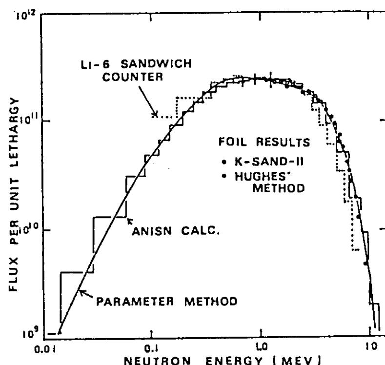
Fig. 3.3.8 Neutron spectrum in the core-center field of YAYOI.
