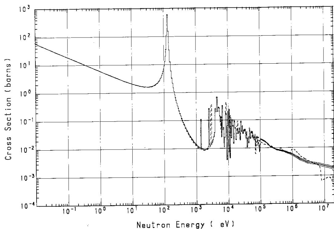
Fig. A.31  $^{59}\text{Co}(n, \gamma)^{60}\text{Co}$  cross section
