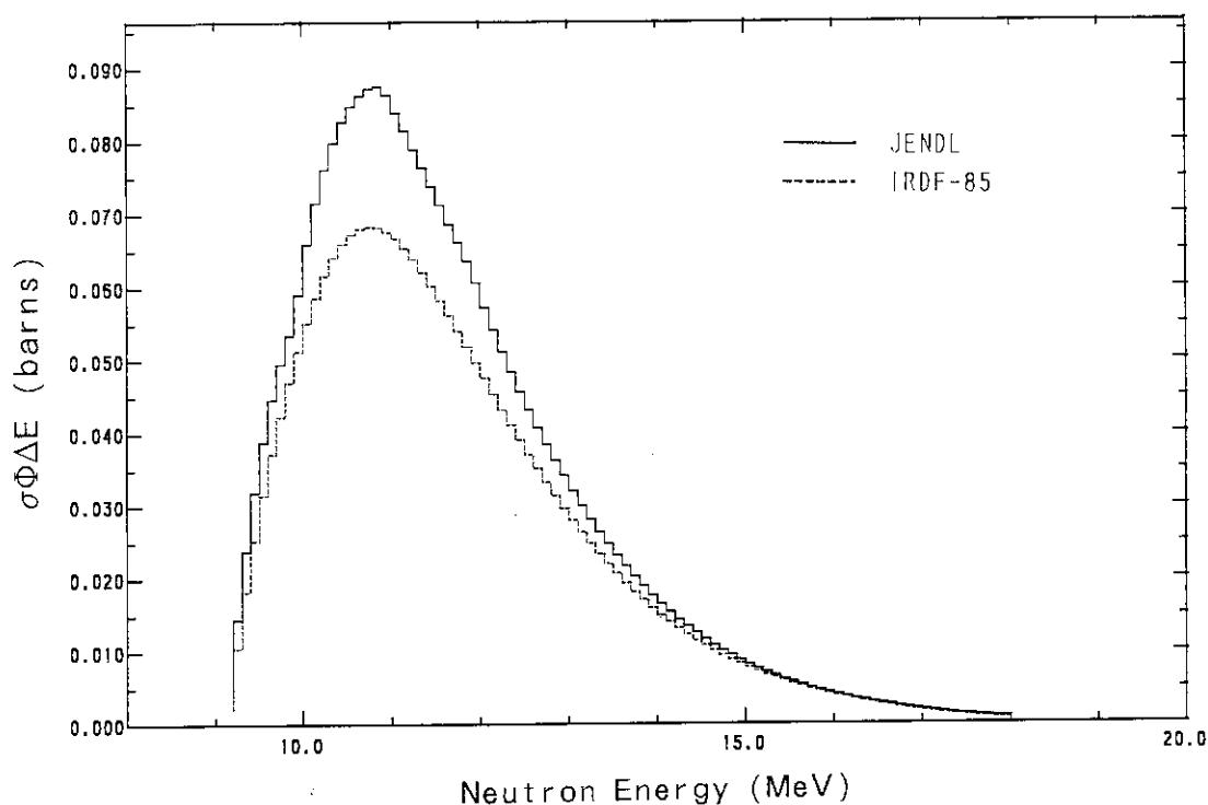
**Fig. 3.1.8** Contributions to the  $^{252}\text{Cf}$  spontaneous fission spectrum average values of  $^{127}\text{I}(\text{n}, 2\text{n})^{126}\text{I}$  reaction cross section.
