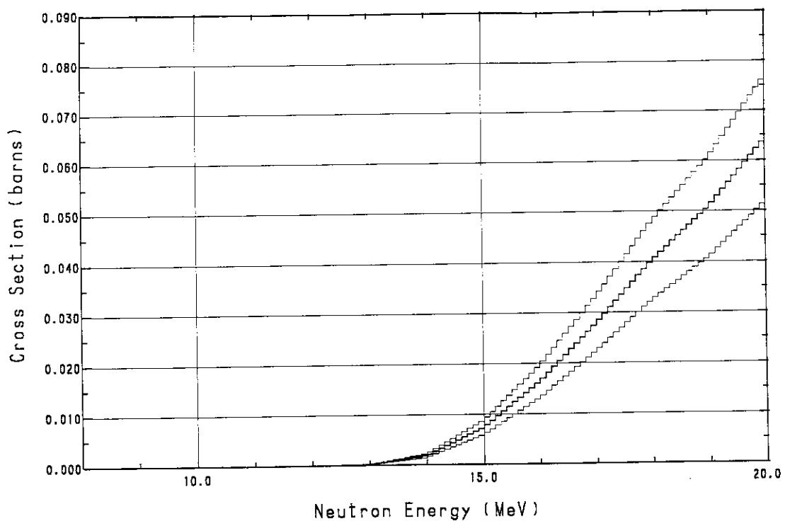
Fig. A.28  $^{57}\text{Fe}(\text{n}, \text{np})^{56}\text{Mn}$  cross section
