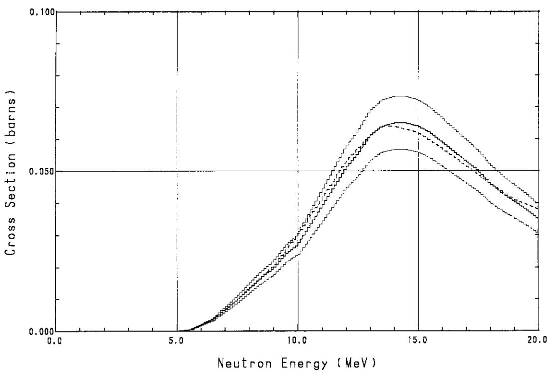
Fig. A.22  $^{48}\text{Ti}(\text{n},\text{p})^{48}\text{Sc}$  cross section
