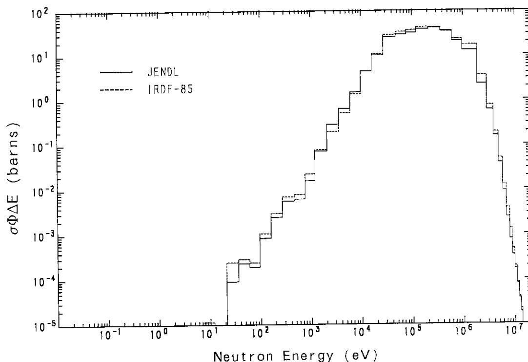
**Fig. 3.1.13** Contributions to the BIG-TEN spectrum average values of  $^{115}\text{In}(\text{n}, \gamma)^{116m}\text{In}$  reaction cross section.
