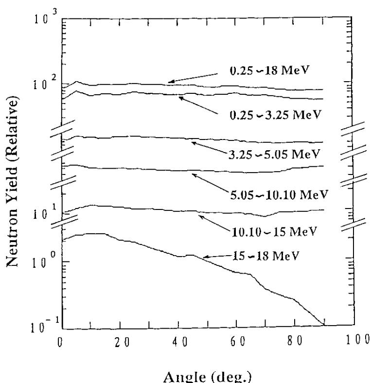
**Fig. 4.2.4** Angular distributions of the thick Li(d, n) neutrons in some energy intervals.
