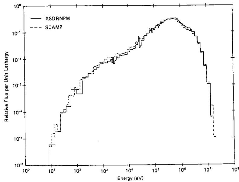
**Fig. 3.3.3** Typical calculated CFRMF central flux spectra. Differences between two spectra show the uncertainty of CFRMF spectrum.
