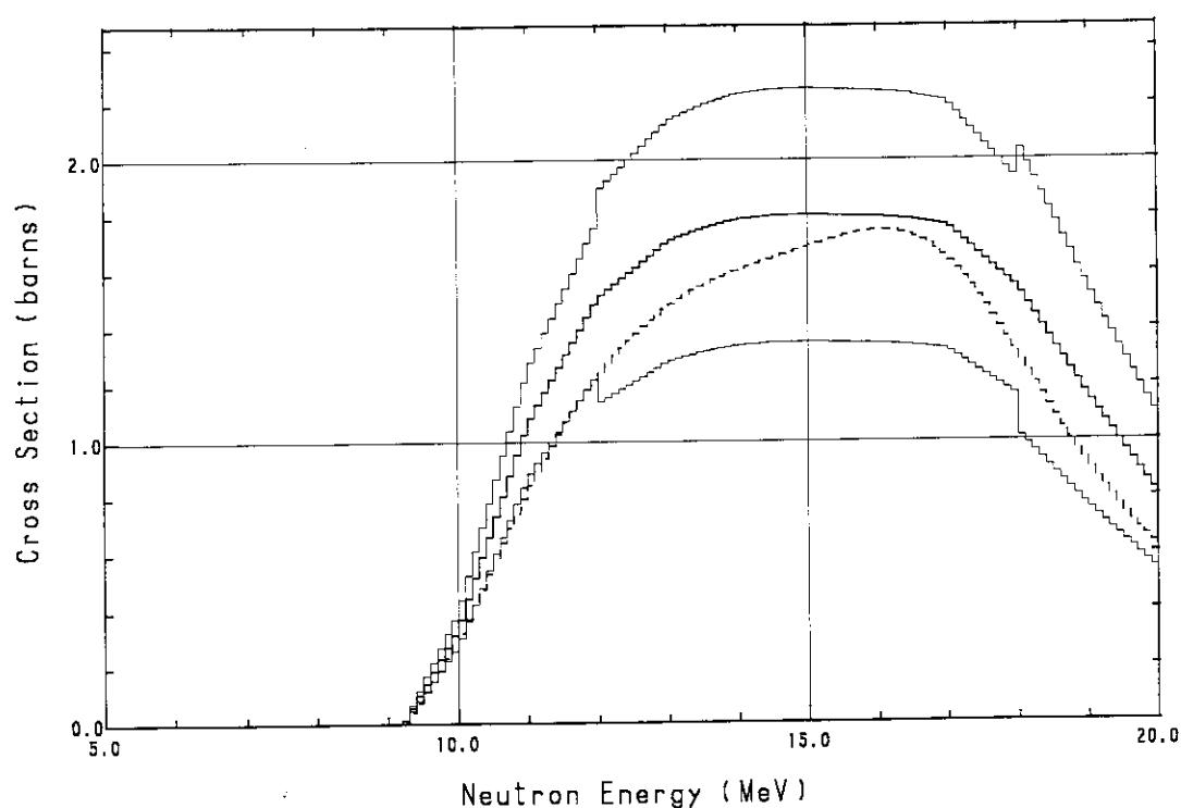
Fig. A.47  $^{127}\text{I}(\text{n}, 2\text{n})^{126}\text{I}$  cross section
