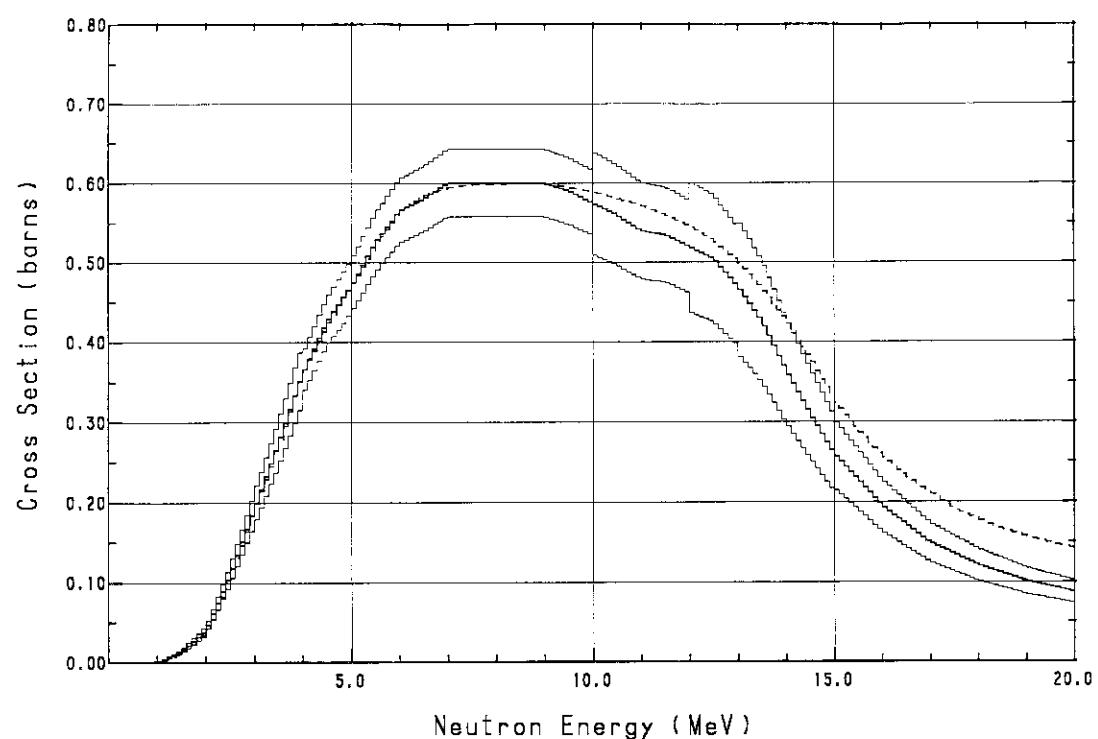
Fig. A.34  $^{58}\text{Ni}(n, p)^{58}\text{Co}$  cross section
