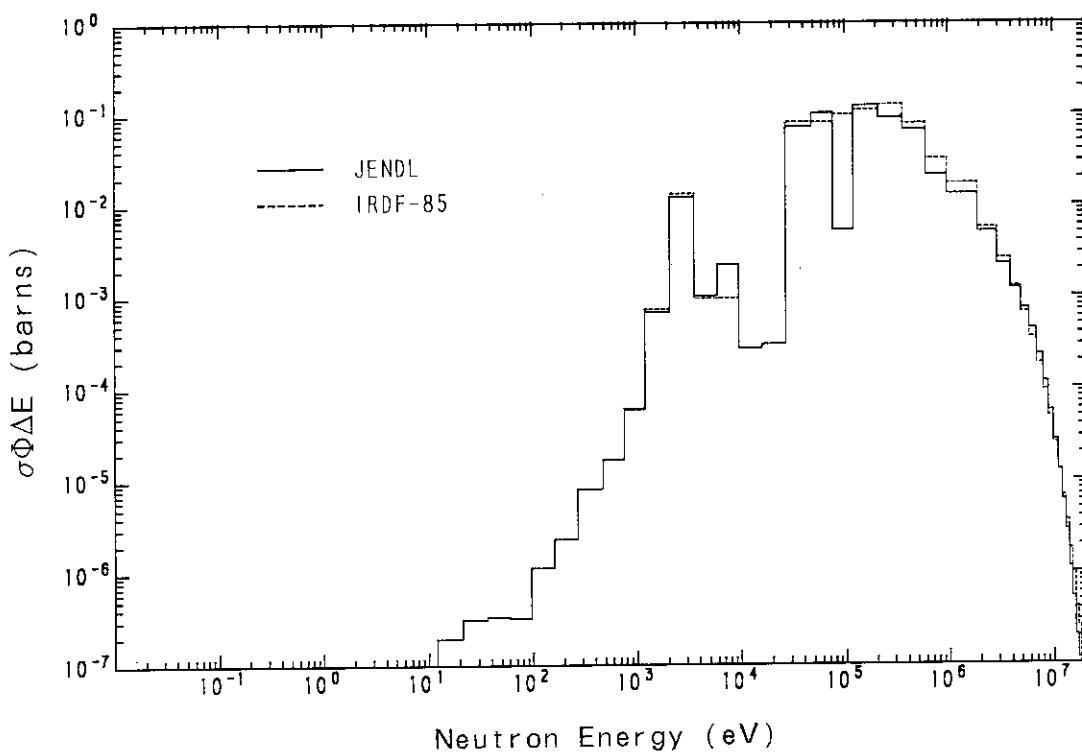
**Fig. 3.1.9** Contributions to the BIG-TEN spectrum average values of  $^{23}\text{Na}(\text{n}, \gamma)^{24}\text{Na}$  reaction cross section.
