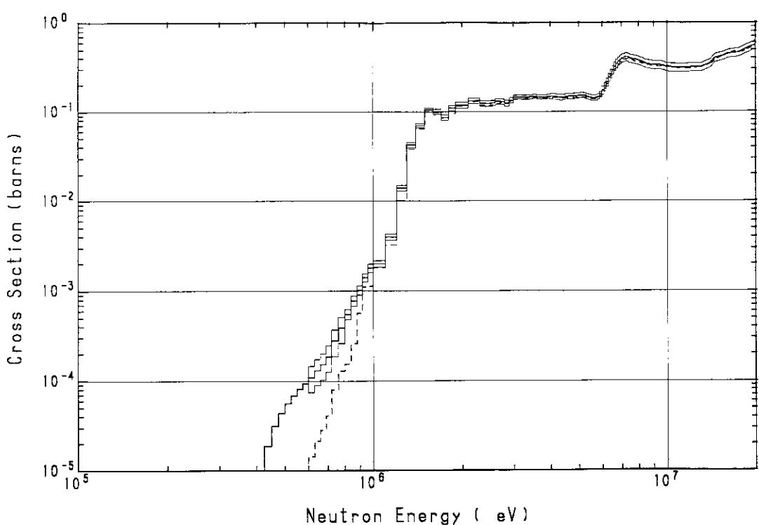
Fig. A.54  $^{232}\text{Th}$  fission cross section
