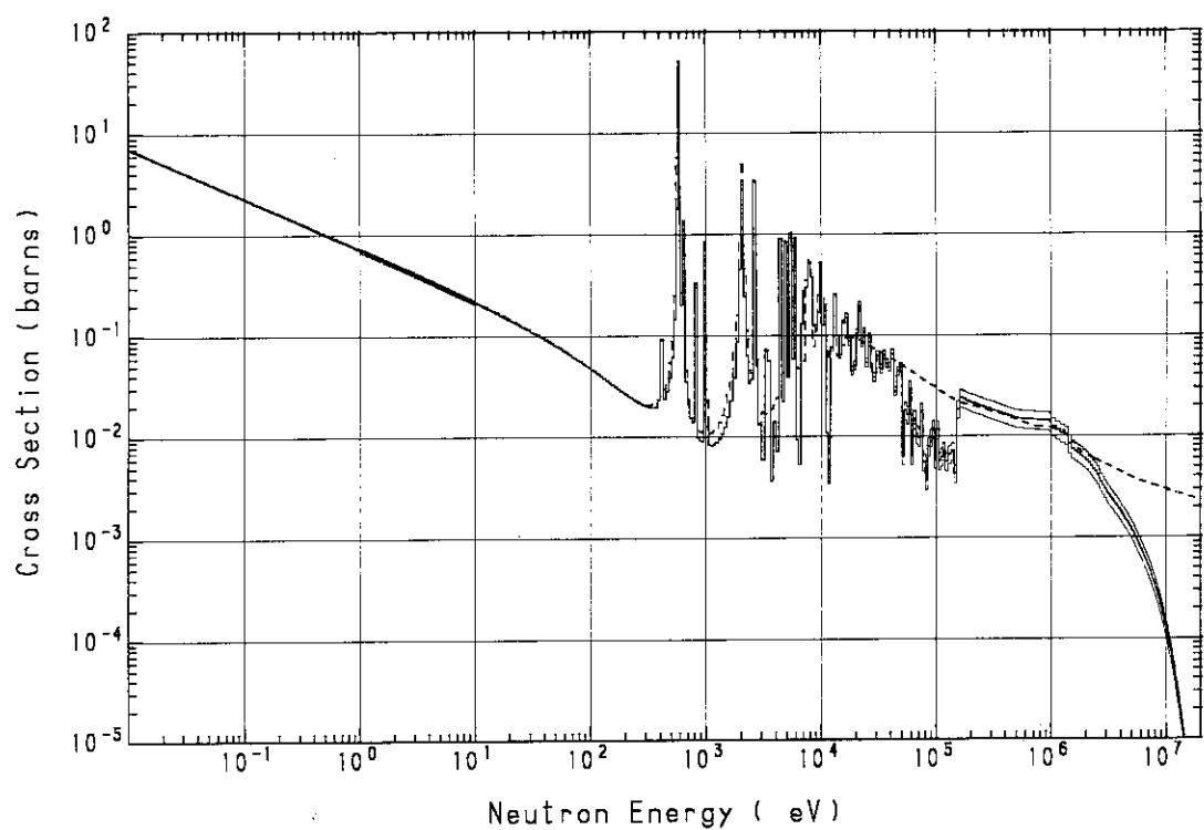
**Fig. A.37**  $^{63}\text{Cu}(n, \gamma)^{64}\text{Cu}$  cross section
