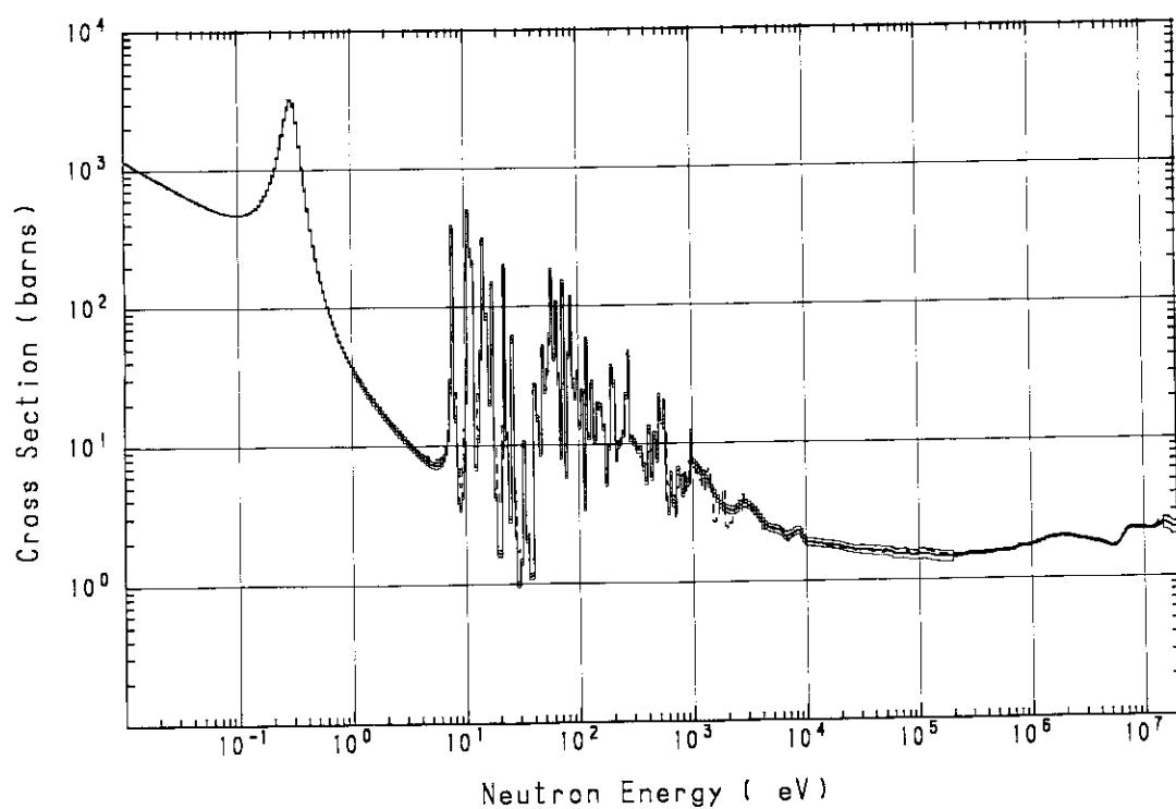
Fig. A.60  $^{239}\text{Pu}$  fission cross section
