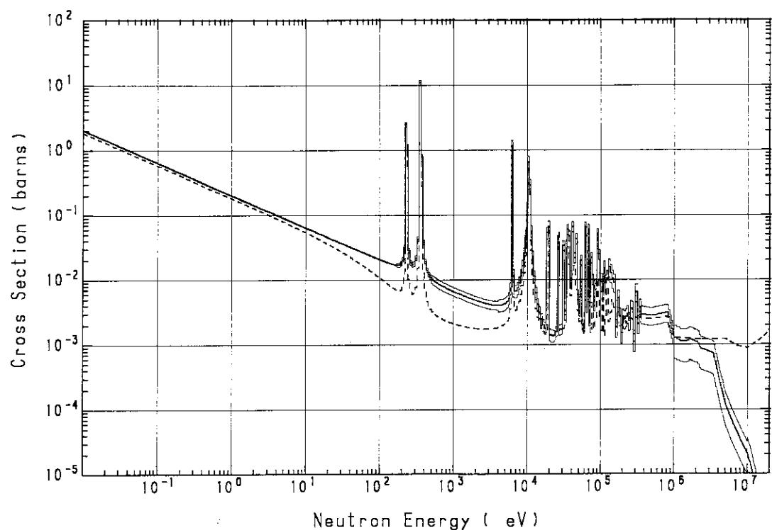
**Fig. A.29**  $^{58}\text{Fe}(n, \gamma)^{59}\text{Fe}$  cross section
