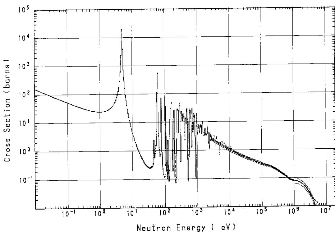
Fig. A.52  $^{197}\text{Au}(\text{n}, \gamma)^{198}\text{Au}$  cross section
