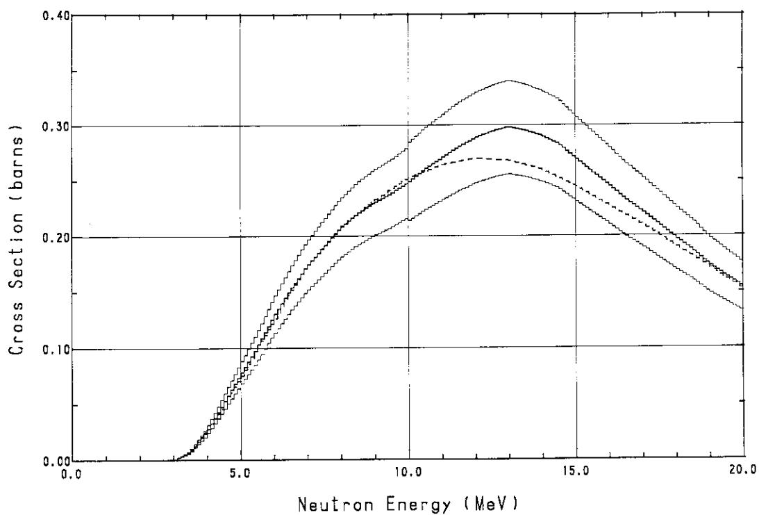
Fig. A.18  $^{46}\text{Ti}(n, p)^{46}\text{Sc}$  cross section
