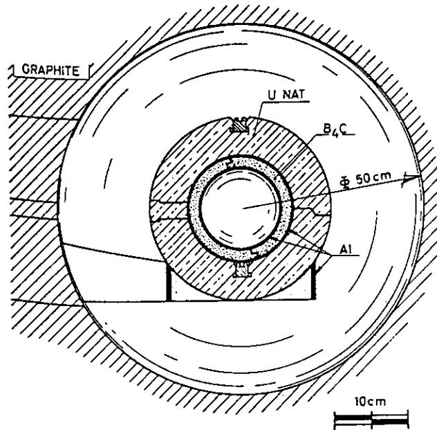
**Fig. 3.3.4** Cross sectional in-pile view of the  $\Sigma\Sigma$  facility.
