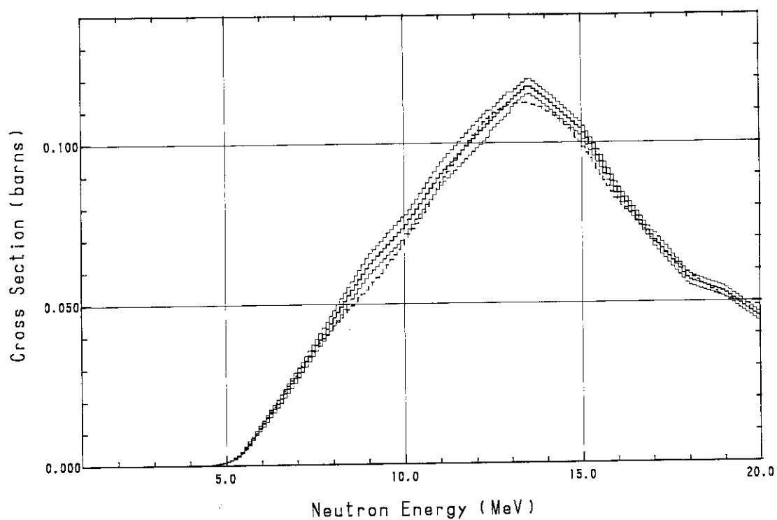
Fig. A.27  $^{56}\text{Fe}(\text{n}, \text{p})^{56}\text{Mn}$  cross section
