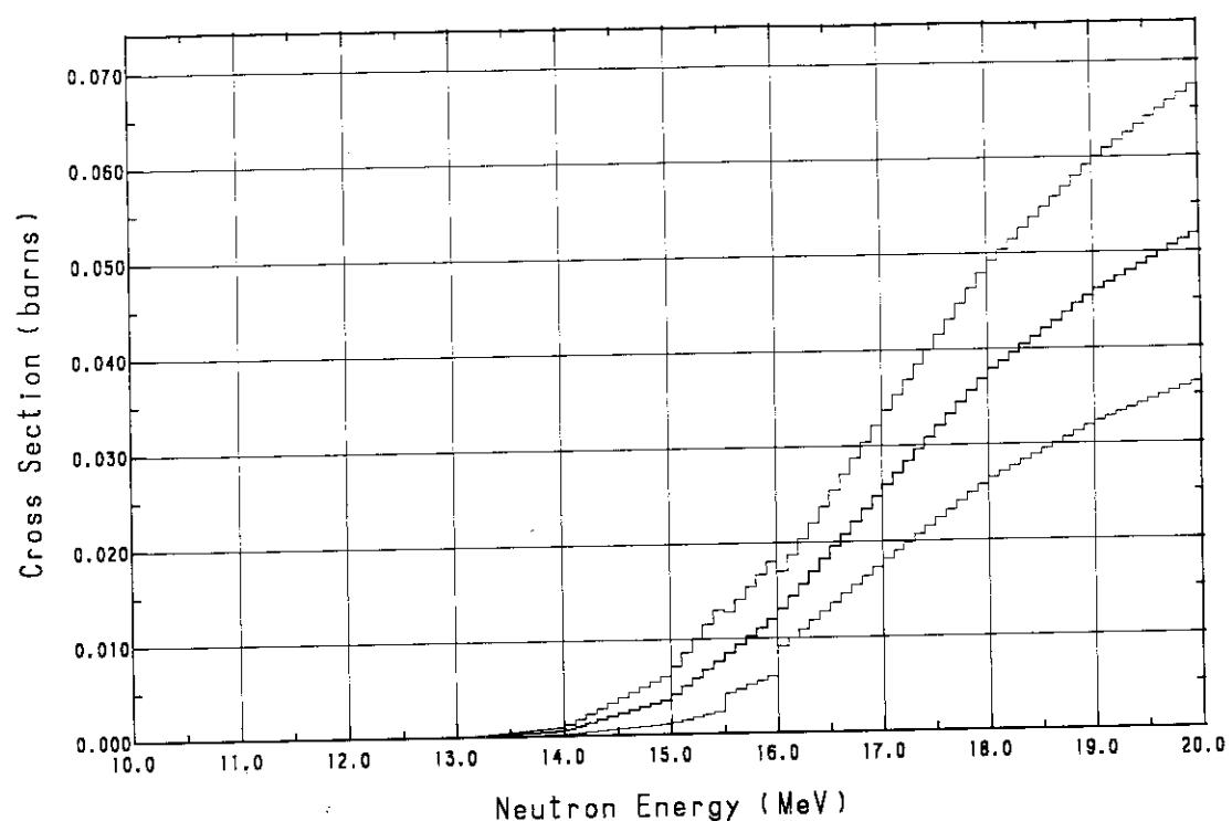
Fig. A.23  $^{49}\text{Ti}(\text{n}, \text{np})^{48}\text{Sc}$  cross section
