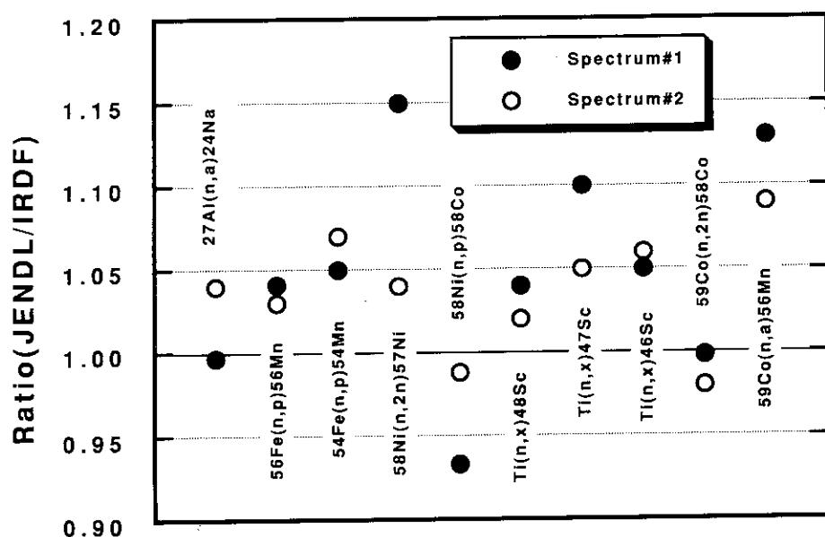
Fig. 4.1.4 Ratios of reaction rates derived from JENDL to those from IRDF.
