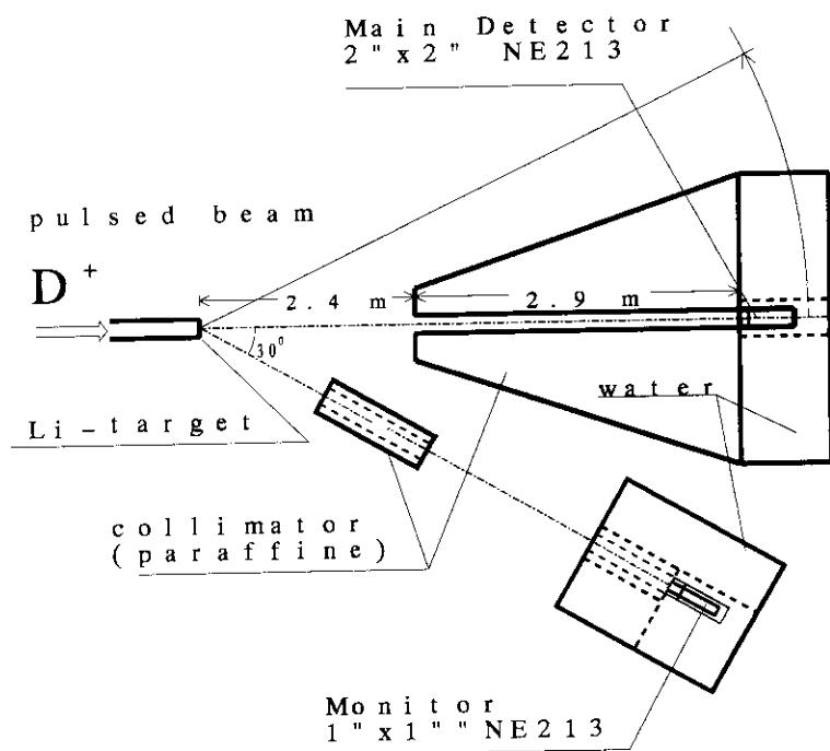
**Fig. 4.2.2** Layout of the experiment for the neutron source characterization.
