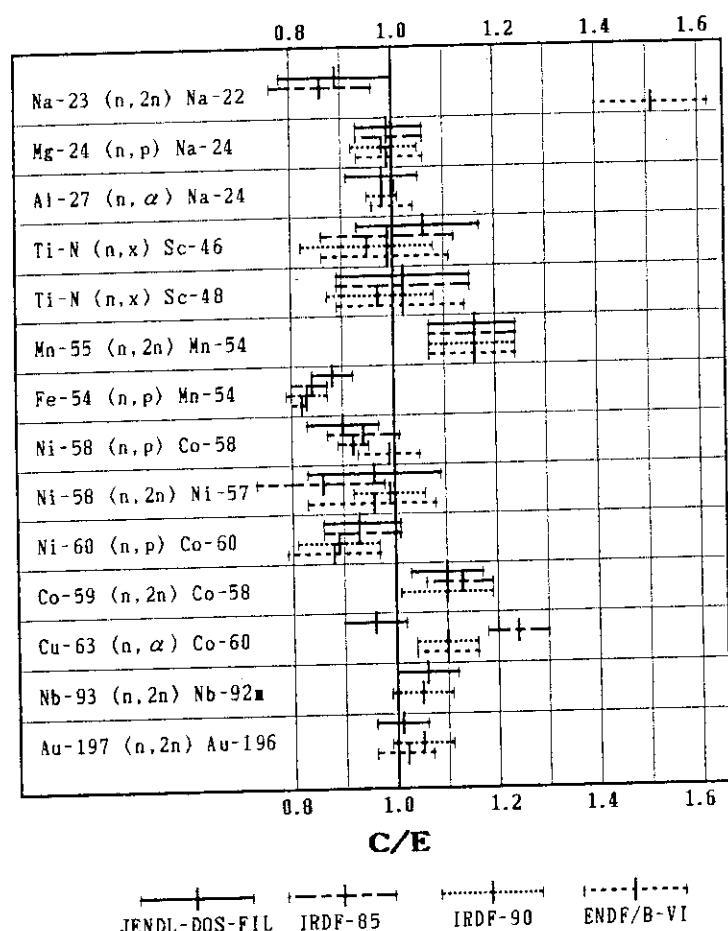
**Fig. 4.2.6** Ratios of the average cross sections (C/E) in the thick Li(d, n) neutron spectrum with the ranges of their uncertainties of the tested dosimetry reactions for the files, the JENDL Dosimetry File, IRDF-85, IRDF-90 and ENDF/B-VI.
