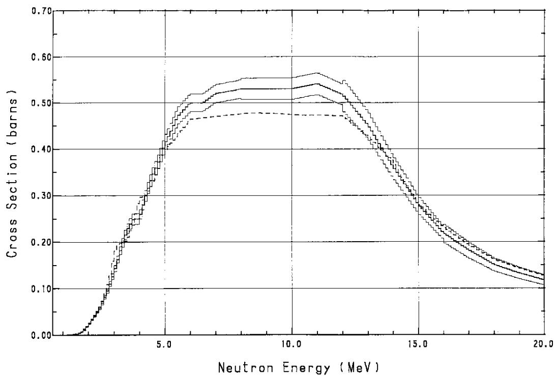
**Fig. A.26**  $^{54}\text{Fe} (\text{n}, \text{p}) ^{54}\text{Mn}$  cross section
