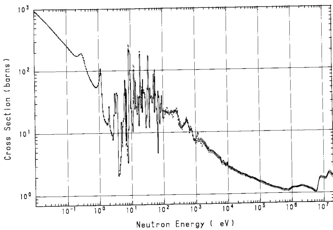
Fig. A.56  $^{235}\text{U}$  fission cross section
