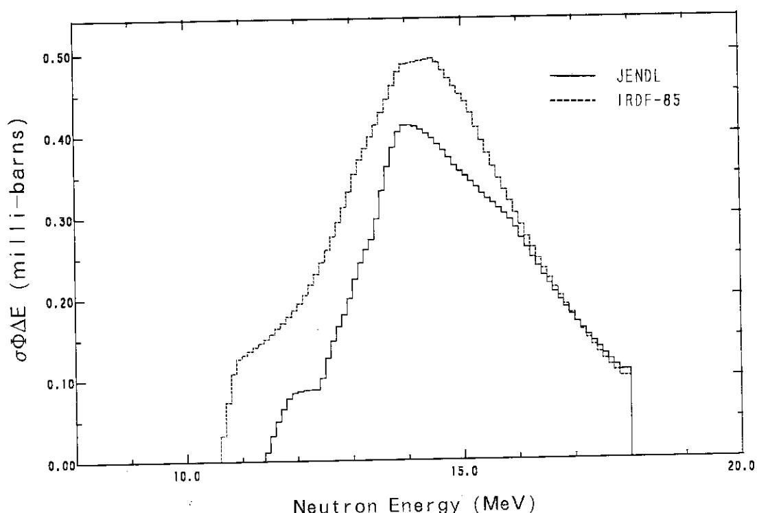
**Fig. 3.1.4** Contributions to the  $^{252}\text{Cf}$  spontaneous fission spectrum average values of  $^{47}\text{Ti}(\text{n}, \text{np})^{46}\text{Sc}$  reaction cross section.
