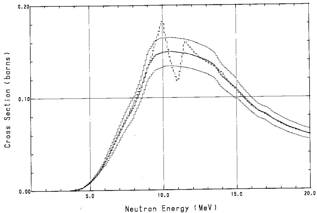
Fig. A.35  $^{60}\text{Ni}(\text{n}, \text{p})^{60}\text{Co}$  cross section
