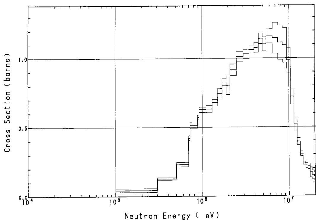
Fig. A.44  $^{103}\text{Rh}(\text{n}, \text{n}')^{103\text{m}}\text{Rh}$  cross section
