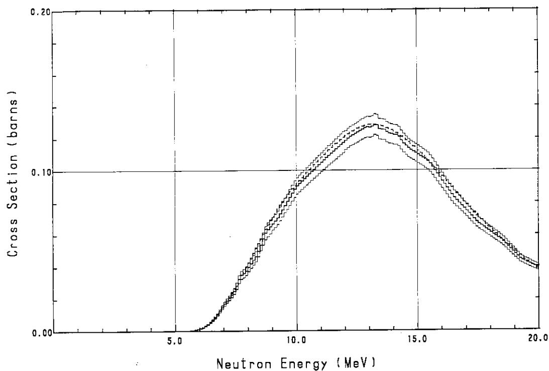
Fig. A.11  $^{27}\text{Al}(\text{n}, \alpha)^{24}\text{Na}$  cross section
