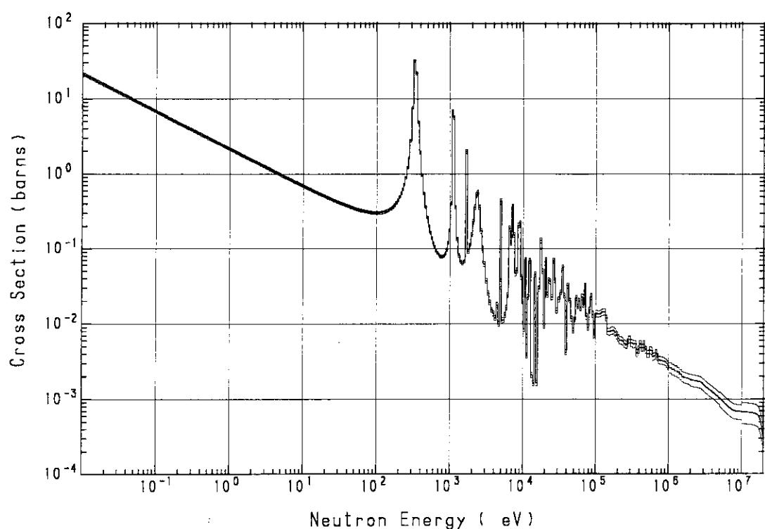
**Fig. A.25**  $^{55}\text{Mn} (\text{n}, \gamma) ^{56}\text{Mn}$  cross section
