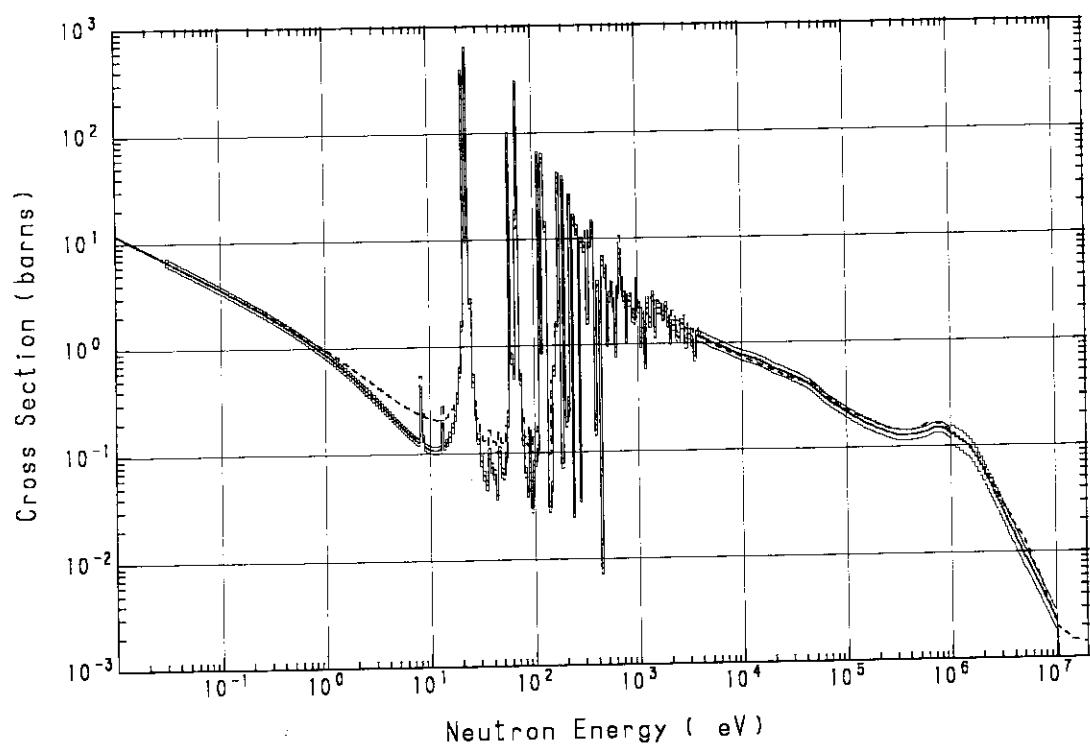
Fig. A.55  $^{232}\text{Th}(n, \gamma)^{233}\text{Th}$  cross section
