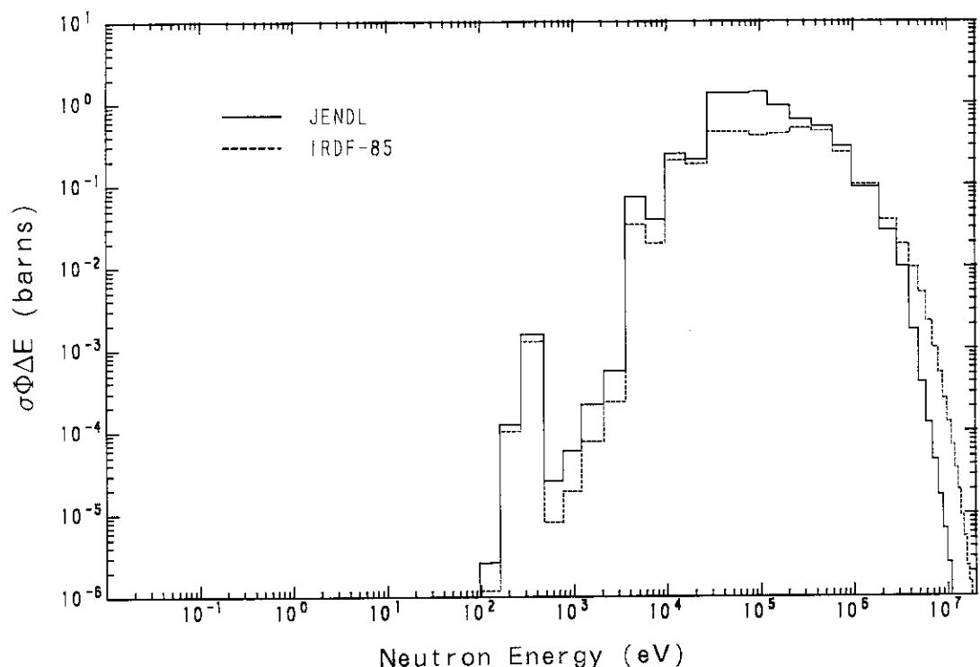
**Fig. 3.1.11** Contributions to the BIG-TEN spectrum average values of  $^{58}\text{Fe}$  ( $n, \gamma$ )  $^{59}\text{Fe}$  reaction cross section.
