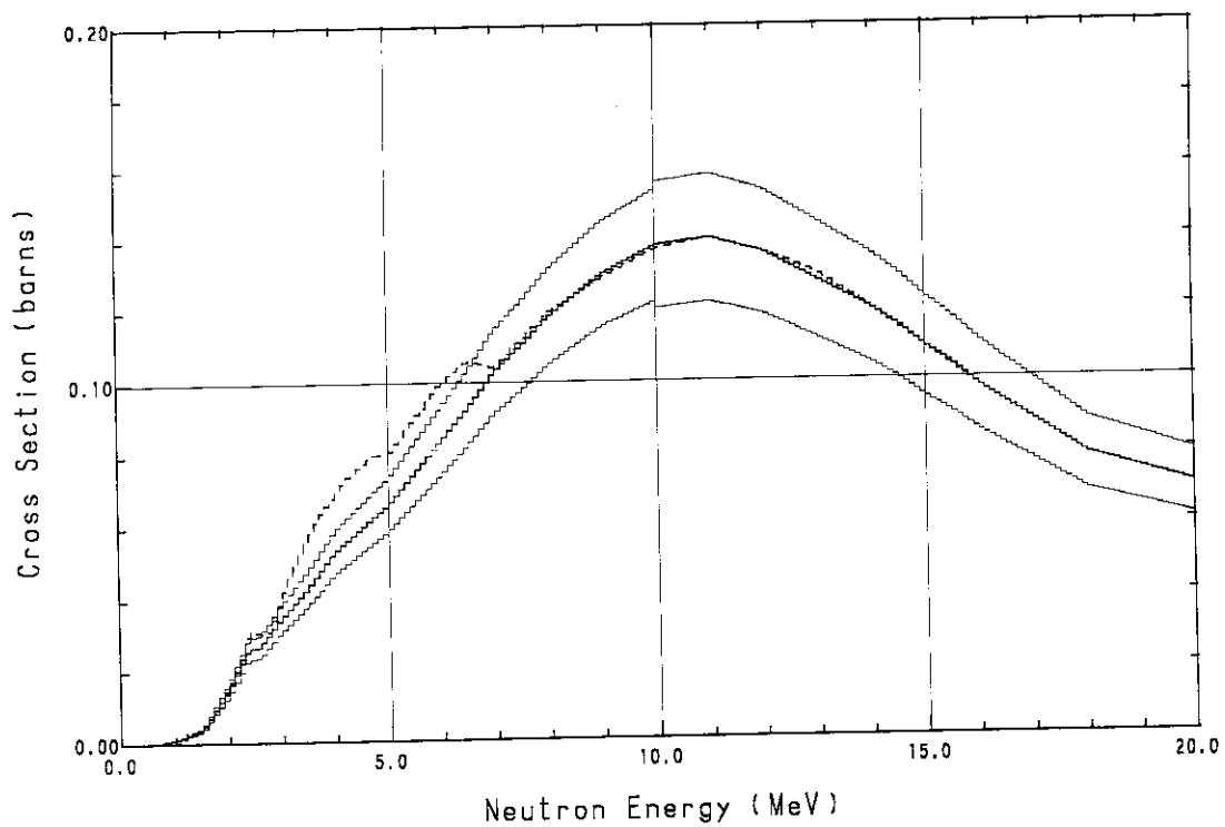
Fig. A.20  $^{47}\text{Ti} (\text{n}, \text{p}) ^{47}\text{Sc}$  cross section
