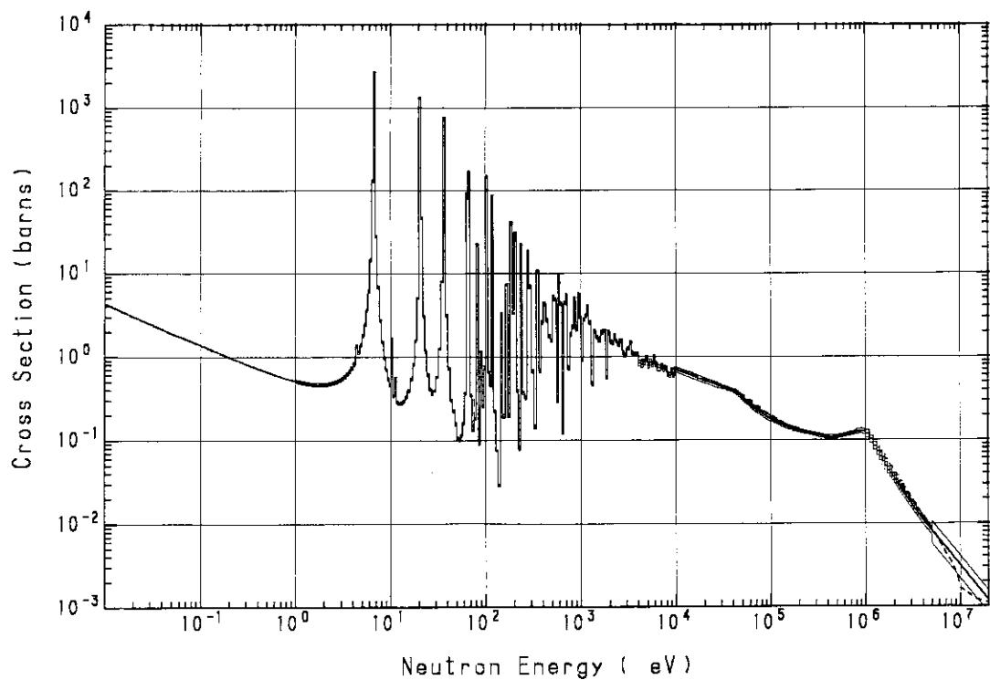
Fig. A.58  $^{238}\text{U}(n, \gamma)^{239}\text{U}$  cross section
