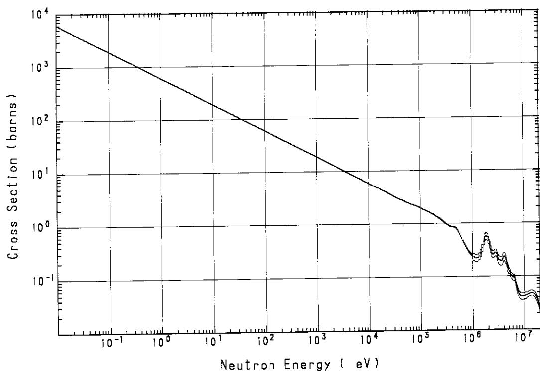
**Fig. A.4**  ${}^{10}\text{B}(n, \alpha){}^7\text{Li}$  cross section
