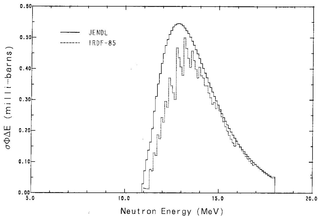
**Fig. 3.1.2** Contributions to the  $^{252}\text{Cf}$  spontaneous fission spectrum average values of  $^{19}\text{F}(\text{n}, 2\text{n})^{18}\text{F}$  reaction cross section.
