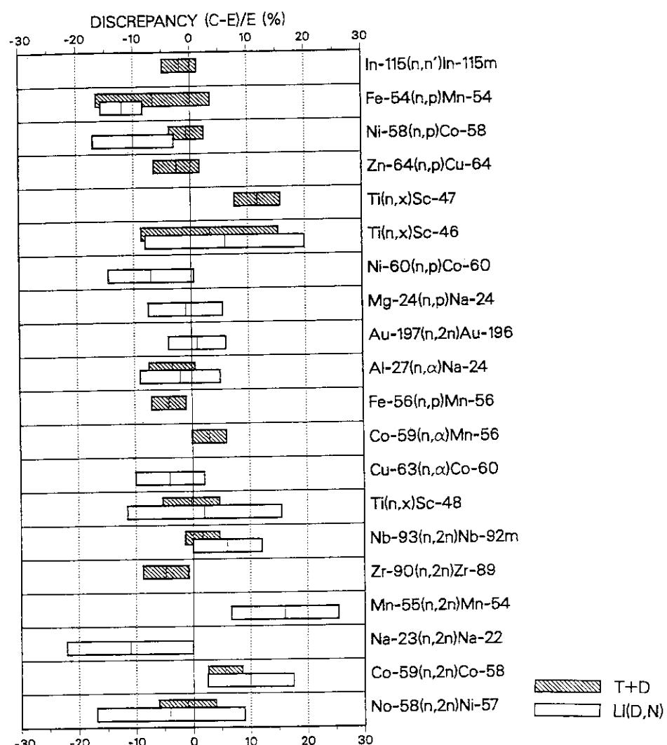
**Fig. 5.2.1** (C-E)/E values of the average cross sections of tested 14 reactions for the JENDL Dosimetry File in the T+d fusion simulated field and the thick Li (d, n) neutron field.
