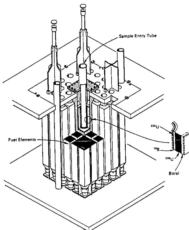
**Fig. 3.3.2** Cutaway pictorial diagram showing the general assembly of the CFRMF.
