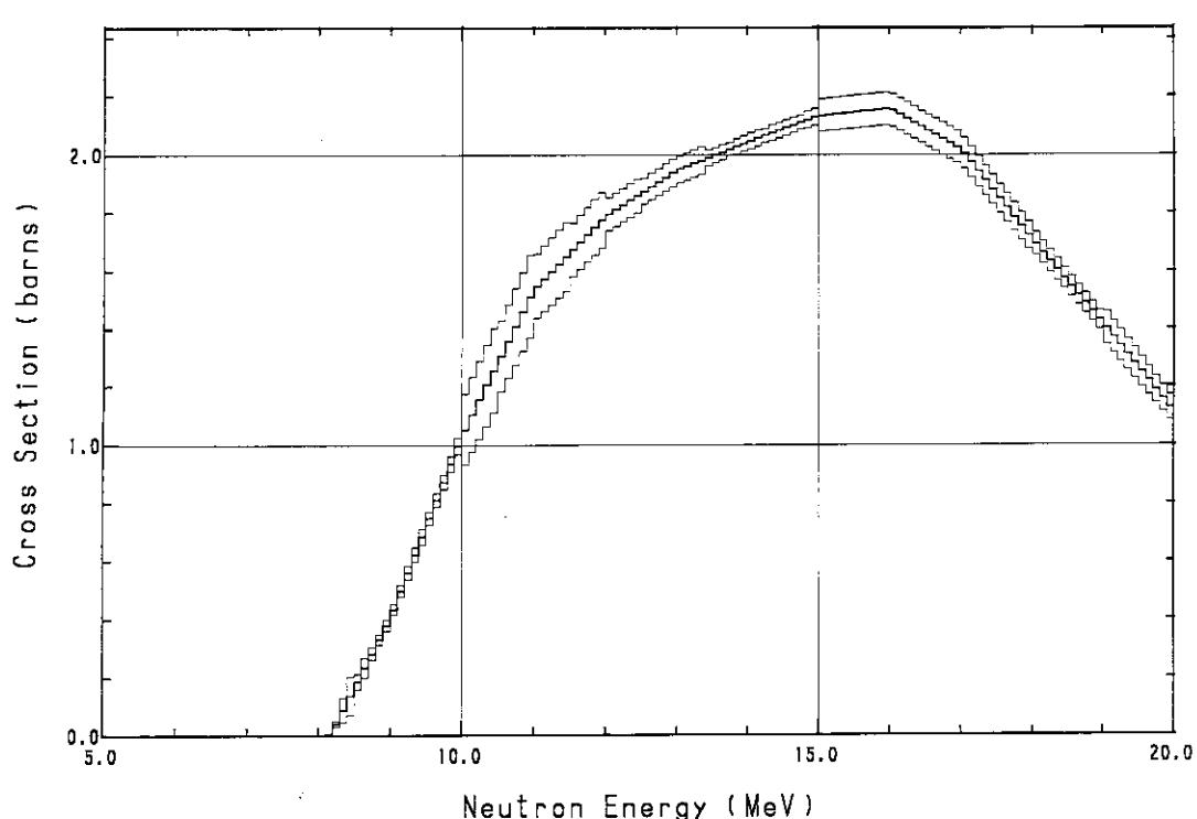
Fig. A.51  $^{197}\text{Au}(\text{n}, 2\text{n})^{196}\text{Au}$  cross section
