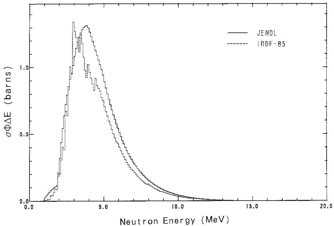
**Fig. 3.1.7** Contributions to the  $^{252}\text{Cf}$  spontaneous fission spectrum average values of  $^{64}\text{Zn}(\text{n}, \text{p})^{64}\text{Cu}$  reaction cross section.
