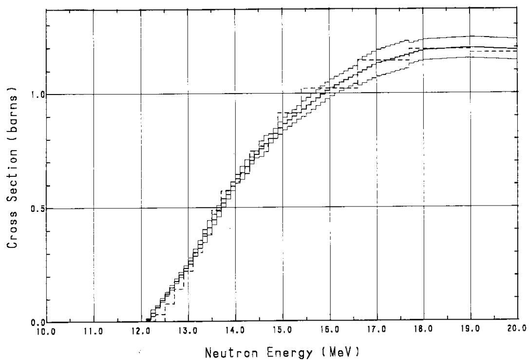
Fig. A.41  $^{90}\text{Zr}(n, 2n)^{89}\text{Zr}$  cross section
