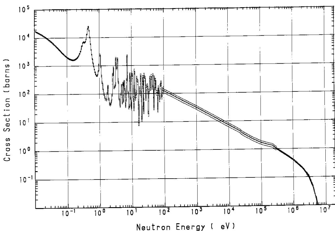
Fig. A.48  $^{151}\text{Eu}(\text{n}, \gamma)^{152}\text{Eu}$  cross section
