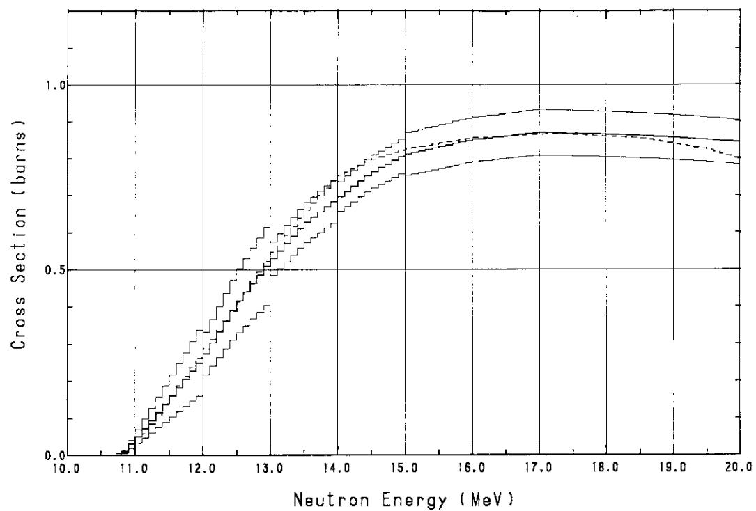
**Fig. A.30**  $^{59}\text{Co}(n, 2n)^{58}\text{Co}$  cross section
