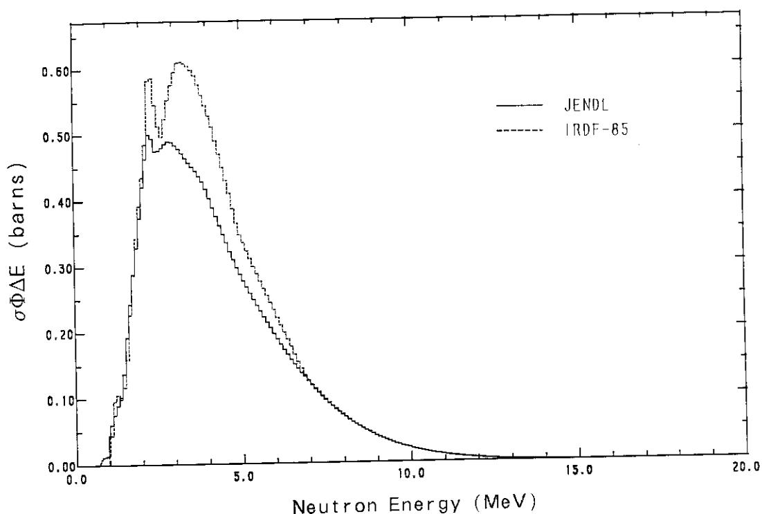
**Fig. 3.1.5** Contributions to the  $^{252}\text{Cf}$  spontaneous fission spectrum average values of  $^{47}\text{Ti}(\text{n}, \text{p})^{47}\text{Sc}$  reaction cross section.
