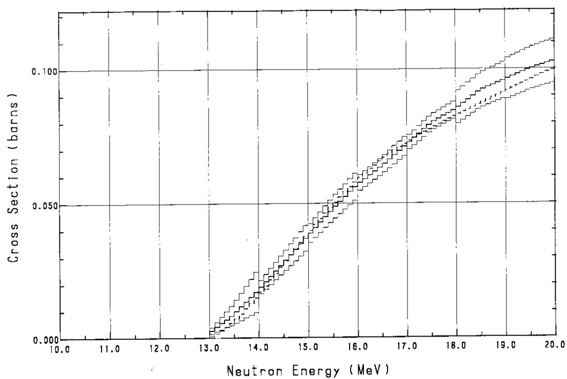
Fig. A.7  $^{23}\text{Na}(n, 2n)^{23}\text{Na}$  cross section
