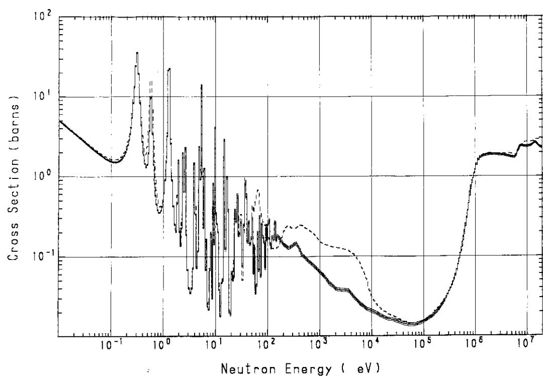
Fig. A.61  $^{241}\text{Am}$  fission cross section
