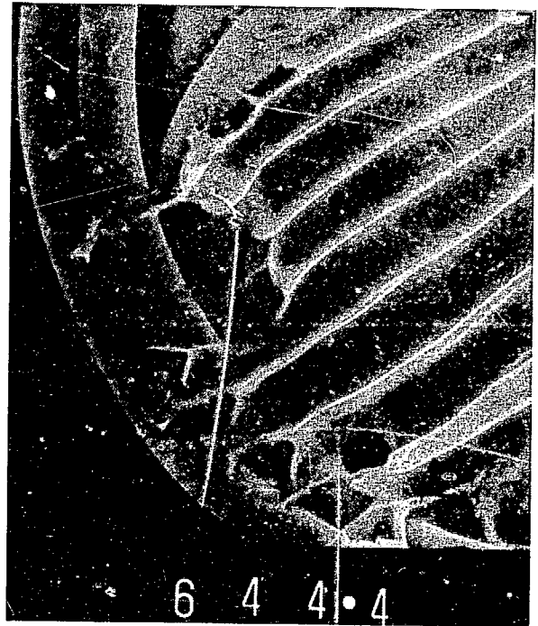
(b) Apparent graft 27.0%, prepared by the irradiation at 23°C.
