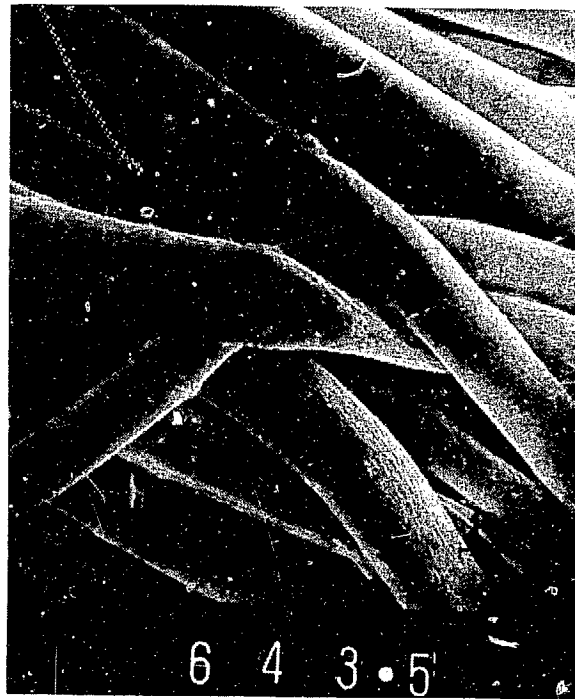
(e) Apparent graft 27.0%, prepared by the irradiation at 100°C.
