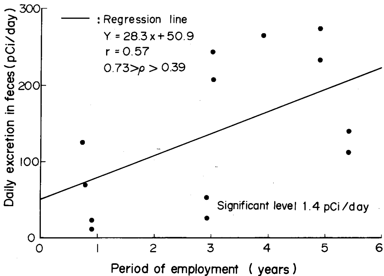
Fig. 2-3 Plots of the excreted ^{147}\text{Pm} activity versus the periods of employment of subjects.
