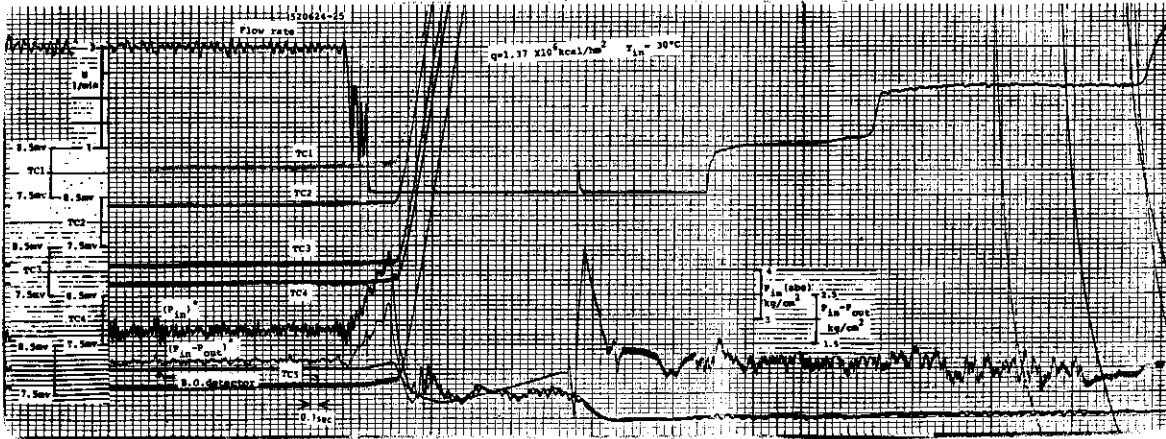
(b) \Delta t = 0.11 \text{ sec} , \left| \frac{\Delta v}{\Delta t} \right| = 660 \text{ cm/sec/sec} Lead wire of burnout detector detached from the test section
