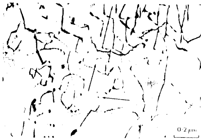
Fig. 2.23(a) Micro-structure of Japanese weld 1JW10 after irradiation at 250°C. Evidence of dislocation climb blocked by small invisible obstacles
