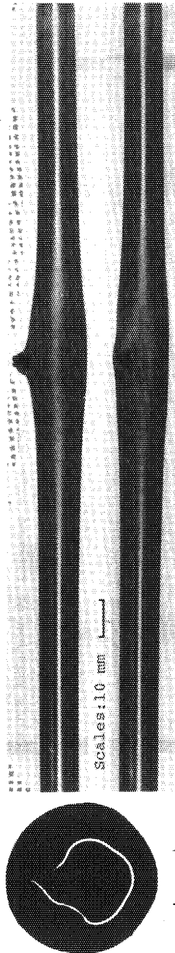
Photo. 5 Specimen cladding of Case A-2 (Fig.10). Seen from two directions (Right); cross section at rupture site (Left). Tested in eight external heater pipes.
