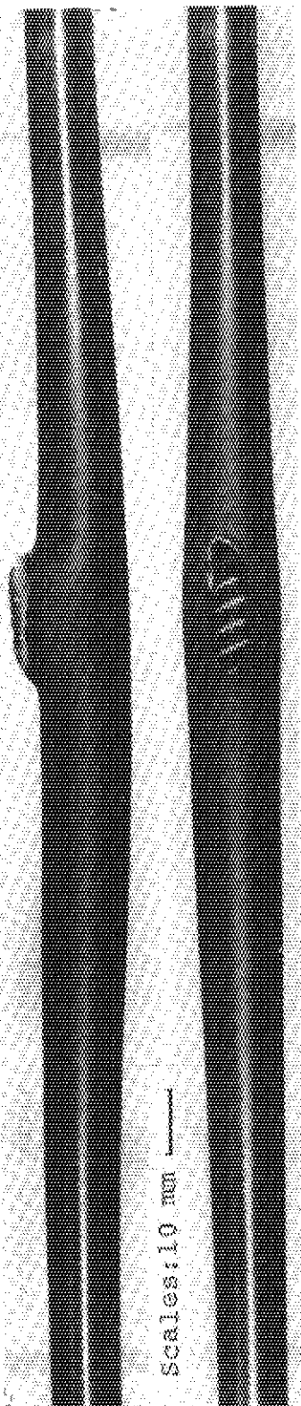
Photo.2 Ruptured specimen cladding tested alone in air with no external heater pipes ( Case P-1, Fig.5). Seen from two directions (Right); cross section at rupture site (Left).
