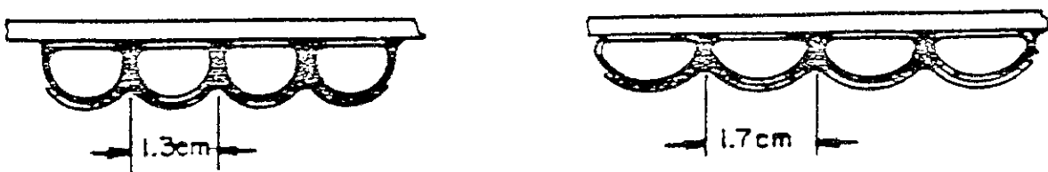
Fig.5.1.10 Semi-circular Tube Wall with Flattening in Poloidal Direction (TFTR)
