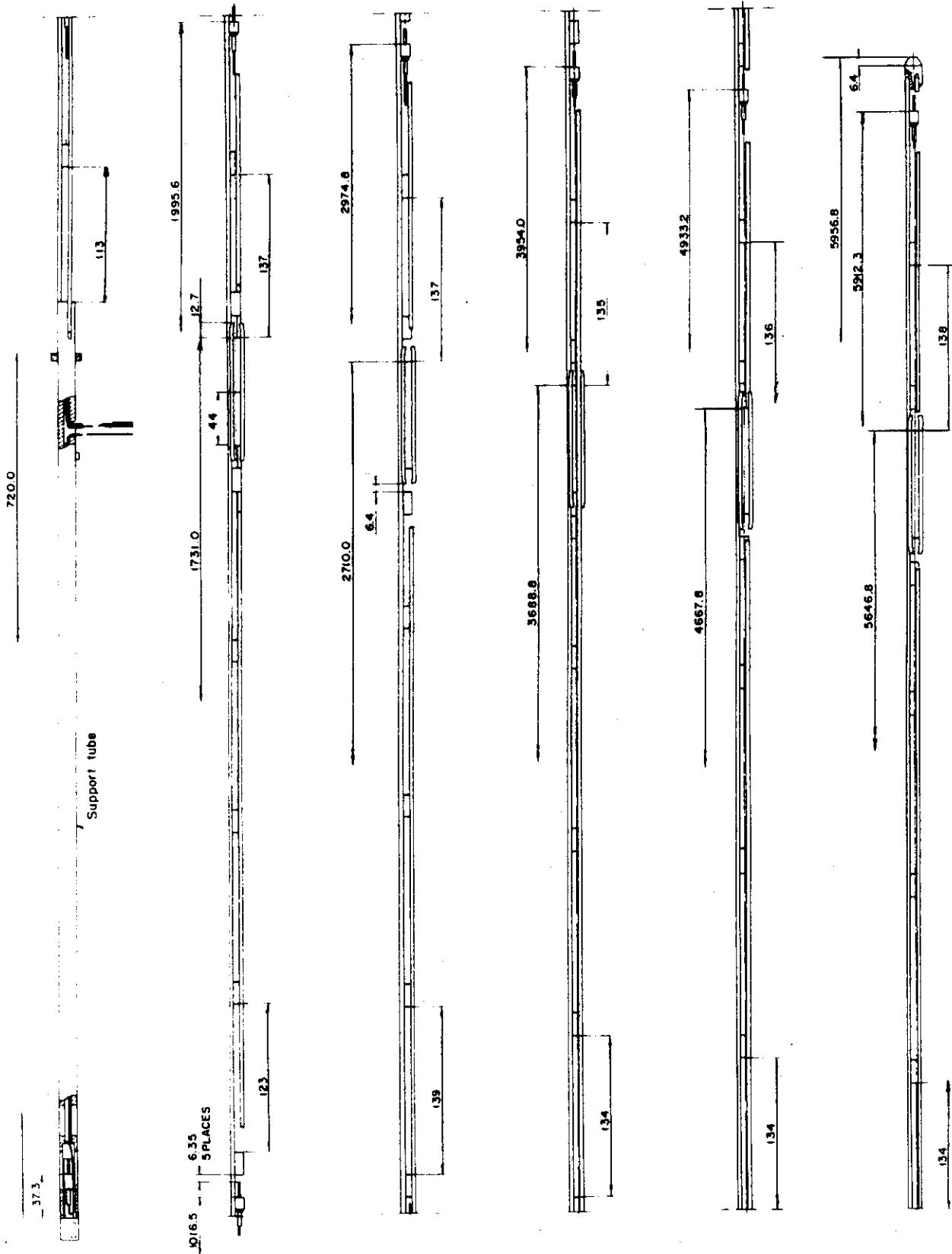
Fig. 2-20 Downcomer FDG assembly
