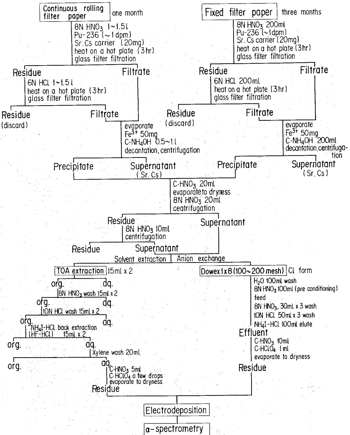
Fig. II-1-3 Analytical procedure for  $^{239}\text{Pu}$  in air dust
