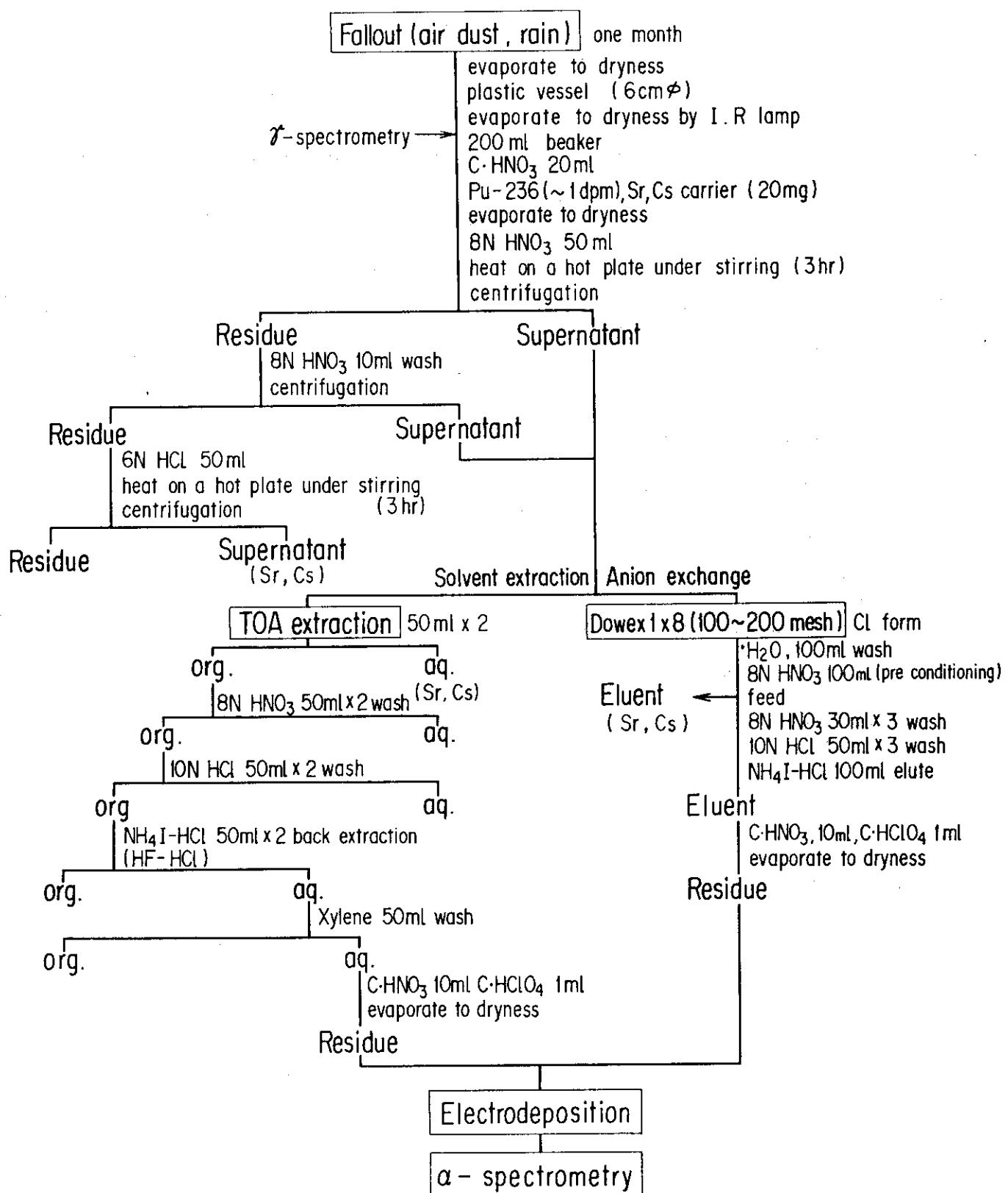
Fig. II-2-1 Analytical procedure for  $^{239}Pu$  in fallout
