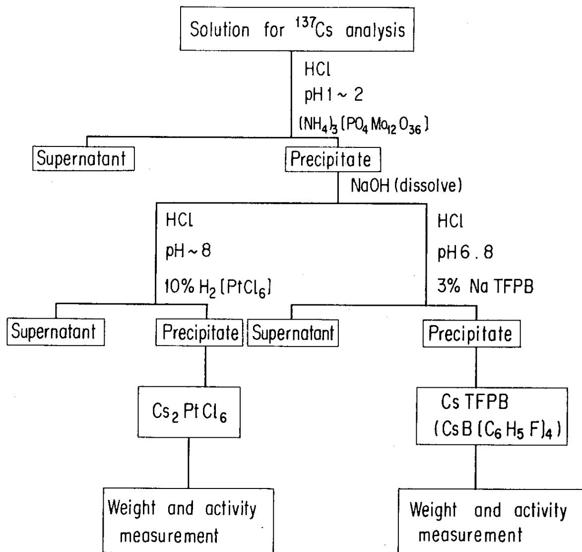
Fig.II-1-6 Analytical procedure for  $^{137}\text{Cs}$
