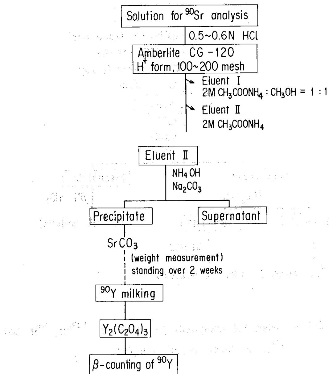
Fig.II-1-5 Analytical procedure for  $^{90}\text{Sr}$
