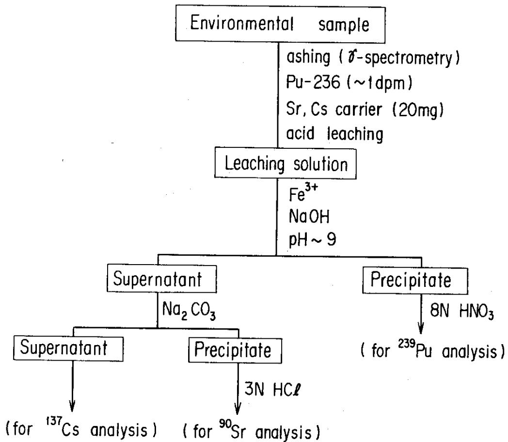
Fig. II-1-4 Sequential analytical procedure for  $^{239}\text{Pu}$ ,  $^{90}\text{Sr}$  and  $^{137}\text{Cs}$  in environmental samples
