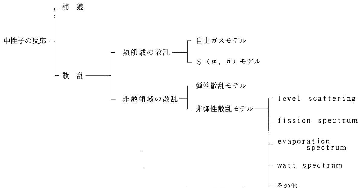
Fig. 4 Nuclear reaction types treated in MCNP code.
