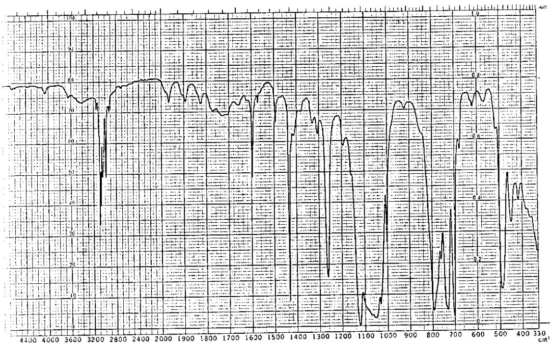
Infrared spectrum (30 MGy in bubbling oxygen)
