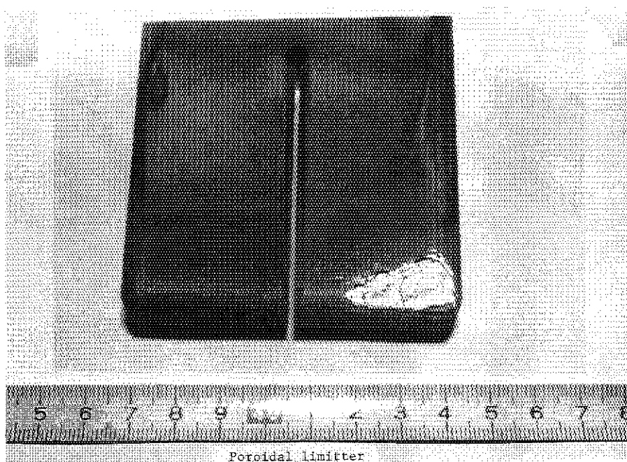
Fig. 3.25 Eroded poloidal limiter used for the experiment.
