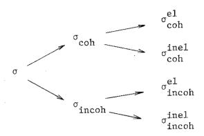
In this diagram, suffixes coh and incoh correspond to the coherent and incoherent scattering of neutrons, and el and inel to the elastic and inelastic scattering. Analysis of so-called thermalization problems or design of thermal neutron reactors have been generally performed within the approximation of incoherent scattering. The coherent inelastic scattering kernel has been obtained only for few crystal materials.
