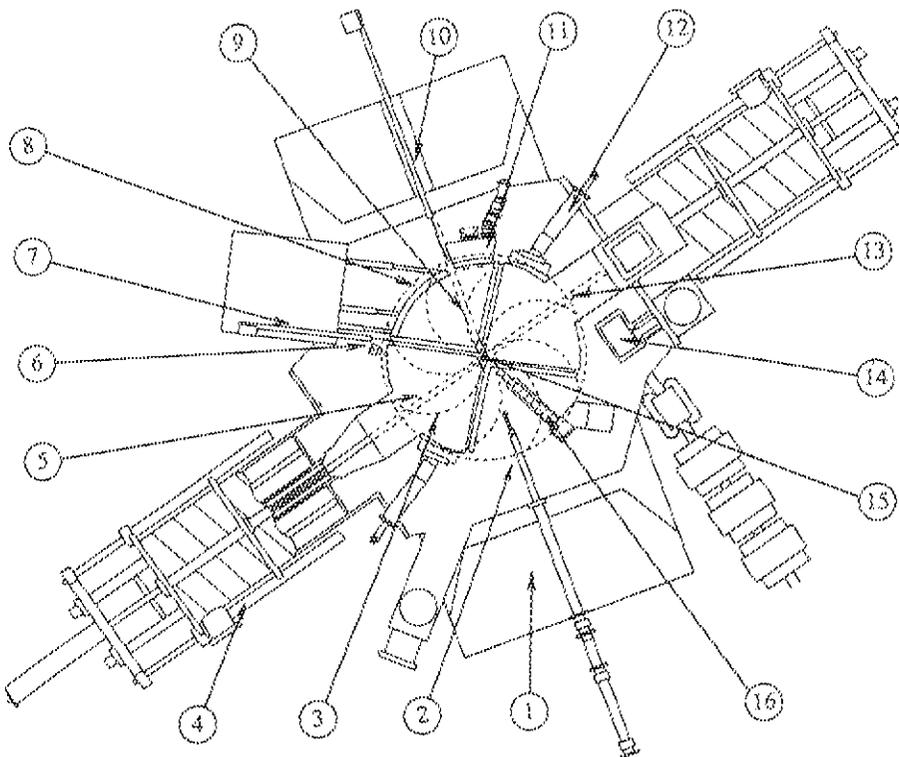
Fig.2 Schematic drawing of the cyclotron. (1)Yoke, (2)Main radial probe, (3)Spiral sector, (4)Resonator, (5)Puller, (6)Dee voltage pickup, (7)Deflector probe, (8)Deflector, (9)Phase slit II, (10)Magnetic channel probe, (11)Magnetic channel, (12)Capacitive fine frequency tuner, (13)Phase slit I, (14)Gradient corrector, (15)Inflector, (16)Phase probe.
