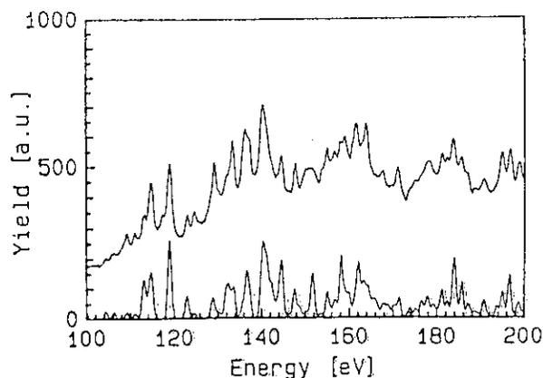
Fig.5 Comparisons of the observed (upper) and simulated (lower) spectra of aluminum. The width of the broadening function is 0.8eV.
