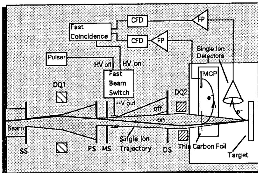
Fig.4 Schematic diagram of single ion hit. SE1: transmission type secondary electron detector, SE2: electron multiplier, FP: fast pre-amp, CFD: constant fraction discriminator, FCM: fast coincidence module.
