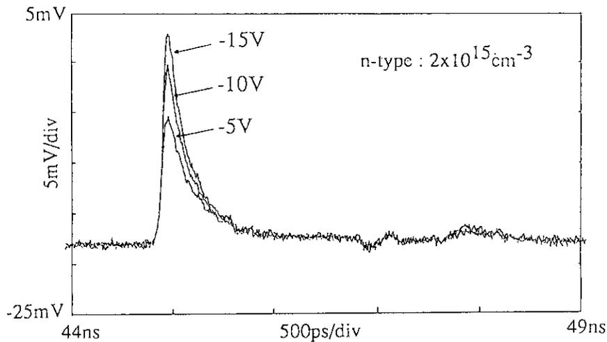
Figure 2. Effect of bias on SEU transient current induced with 15MeV  $C^{+4}$  ions.
