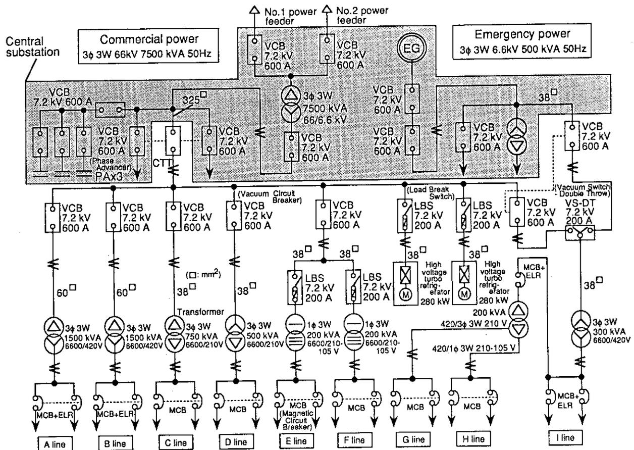
Fig. 5 Trunk connection diagram of the electric-supply lines for ion beam research facility.
