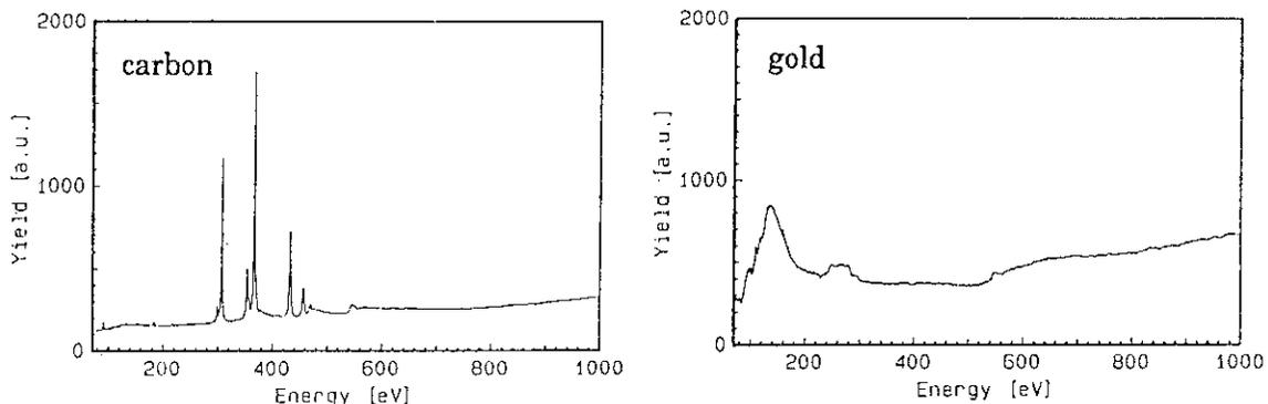
Fig.4 The source X-ray spectra from carbon and gold in the lower energy region.
