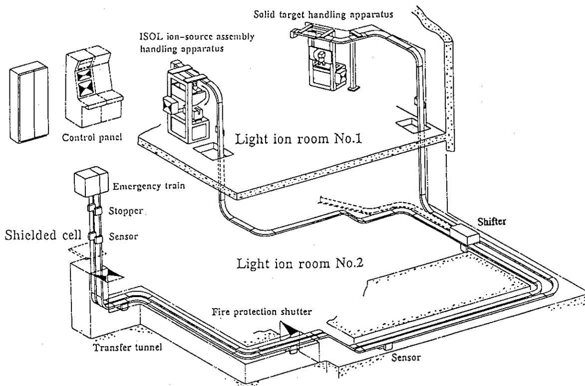
Fig. 3 Solid-target transfer system between the shielded cell and two ports: the irradiation apparatus and the isotope separator on-line.
