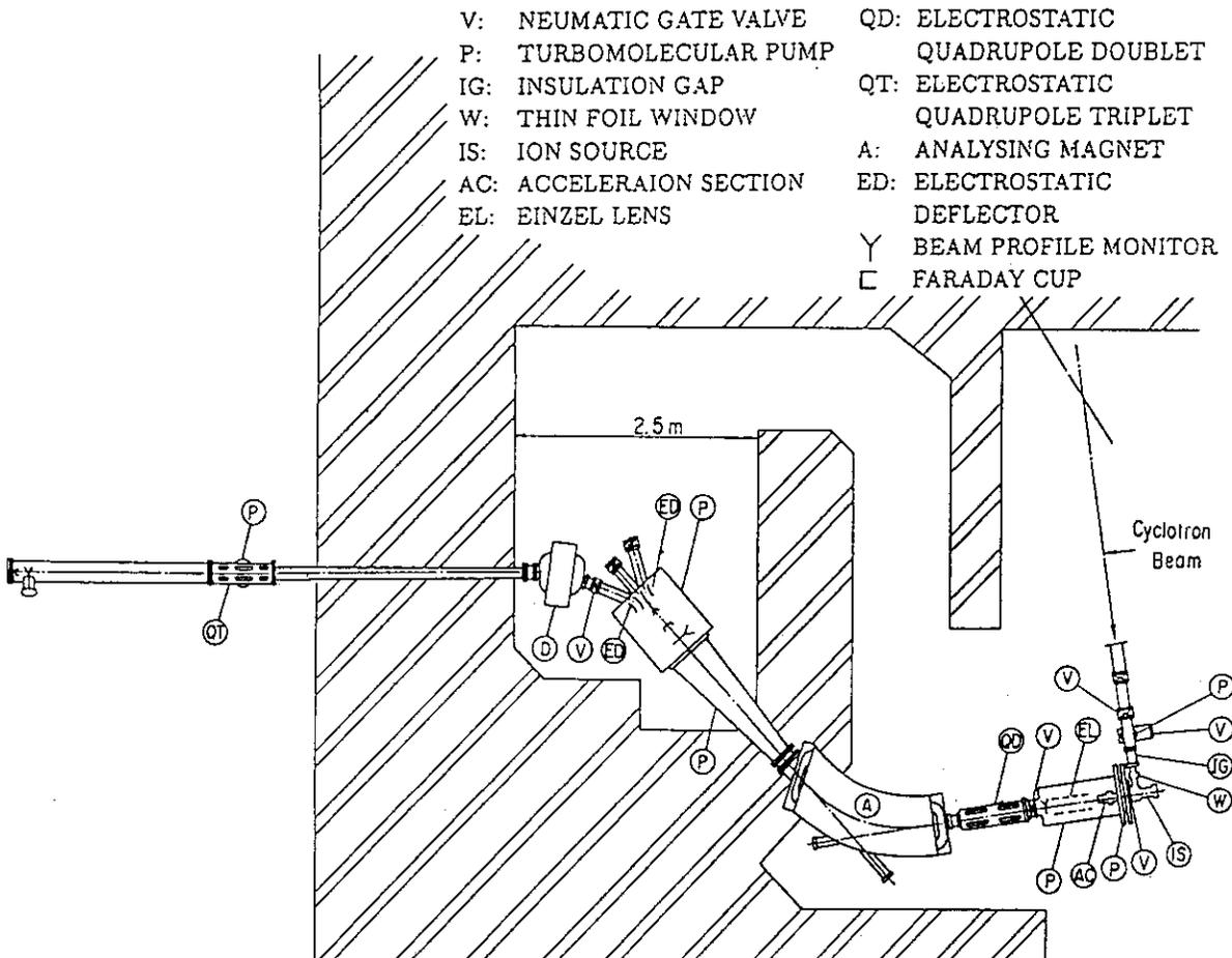
Fig. 1 The ISOL installed in TIARA.
