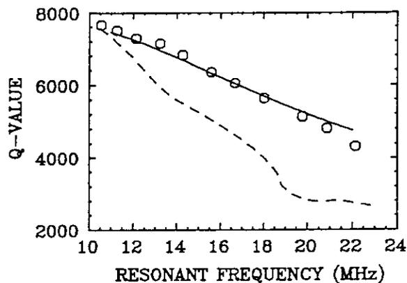
Fig.6 Frequency dependence of Q-value. The solid line shows 75 % of the calculated value based on one-dimensional transmission-line approximation. The dashed line shows the measured value of the movable-panel type cavity.
