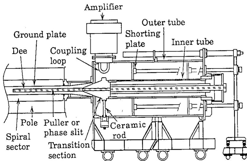
Fig.5 Schematic view of the coaxial resonator with a movable shorting plate.
