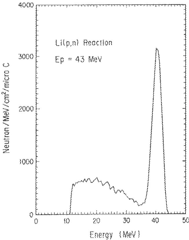
Fig.3 Measured neutron spectrum produced by  ${}^7\text{Li}(p,n)$  reaction of 43 MeV proton beam.
