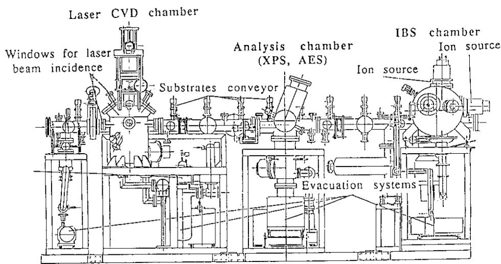
Fig. 1 The apparatus for preparing hybrid thin films
