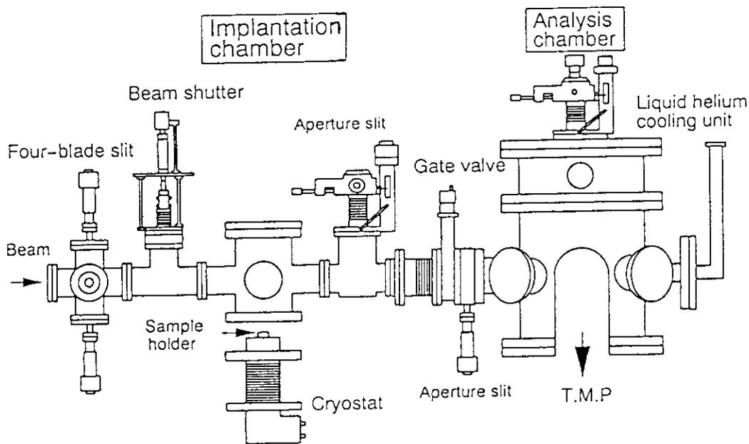
Fig. 1 Schematic Illustration of Ion Beam Analysis System(Baby BAS)
