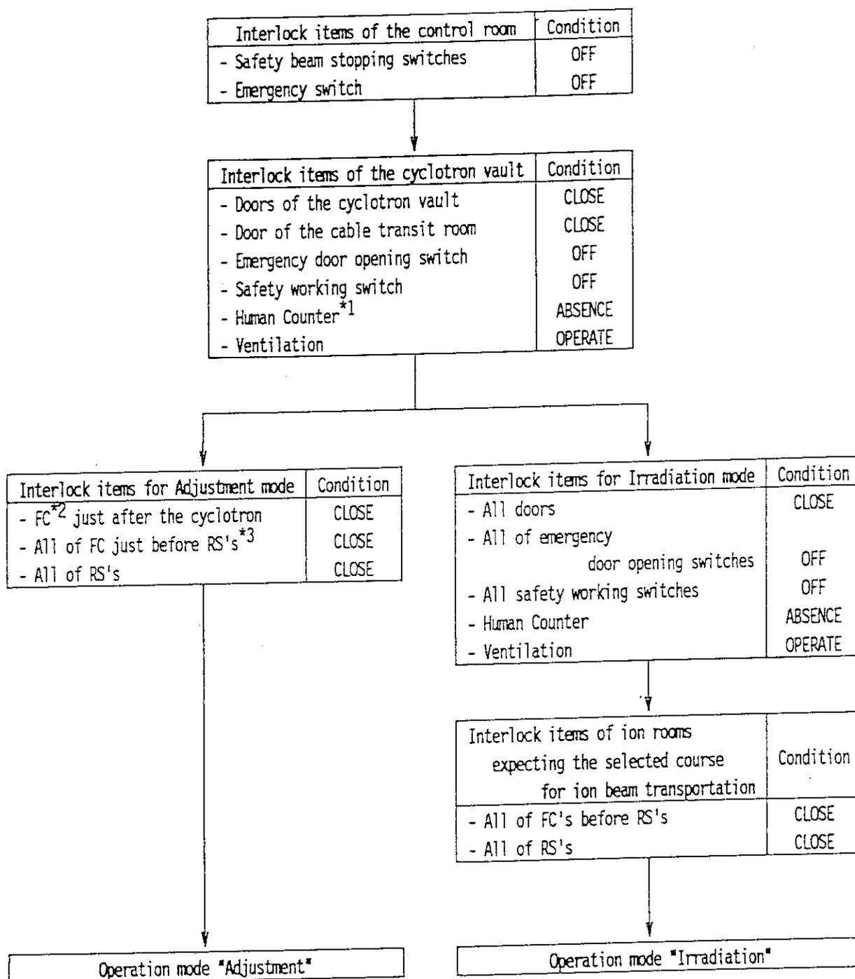
Fig.1 Interlock Condition of Cyclotron Operation.
