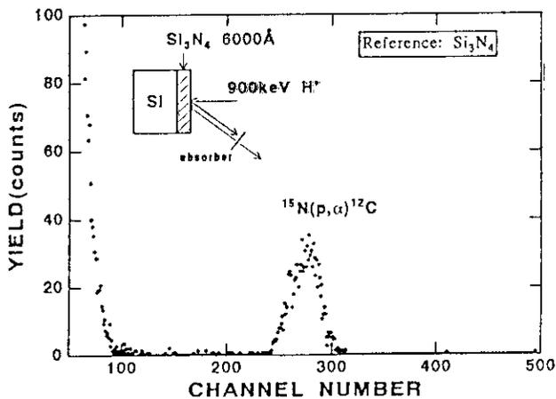
Fig.4 Energy spectrum for 900keV H<sup>+</sup> incident on  $\text{Si}_3\text{N}_4$  film
