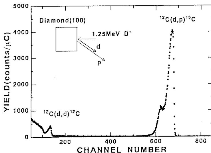
Fig.3 Energy spectrum for 1.25MeV  $\text{D}^+$  incident on a diamond(100) surface under a random condition
