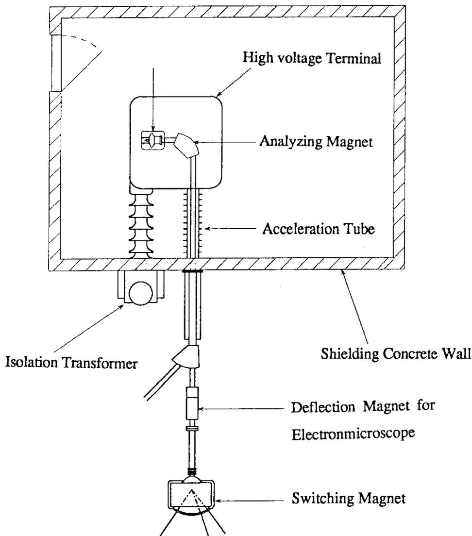
Fig.2. General layout of the 400 kV D.C. Accelerator
