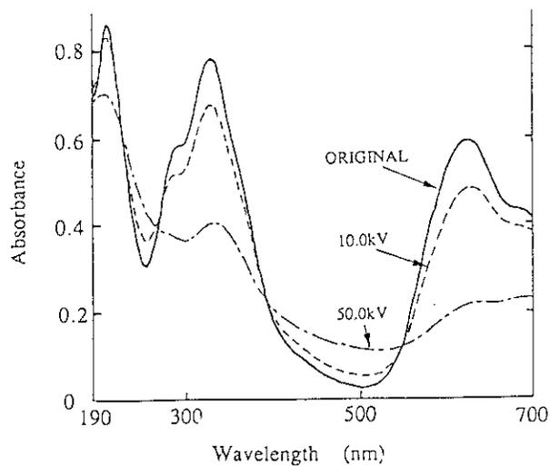
Fig. 2 UV absorption spectra of  $H_2Pc$  PVD thin films irradiated with  $Cu^+$  ion beams.  $Cu^+$  fluence =  $1 \times 10^{13}$  ion/cm<sup>2</sup>.
