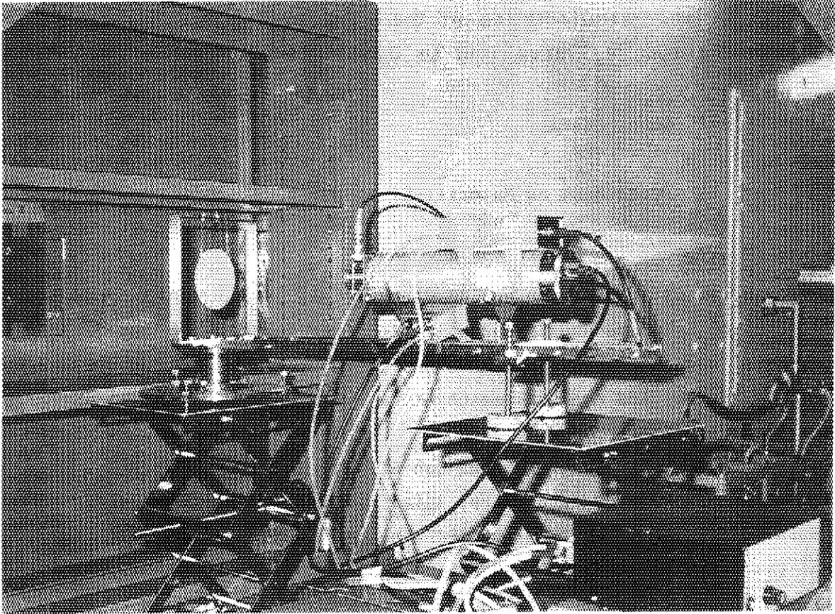
Photo.1 Picture of telescope detector for neutron spectrum measurement.
