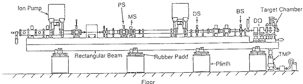
Fig.1 Side view of the heavy ion microbeam system. DQ: precision doublet quadrupole lens PS: preslits, MS: microslits, DS: divergence-defining-slits and BS: baffle slits.
