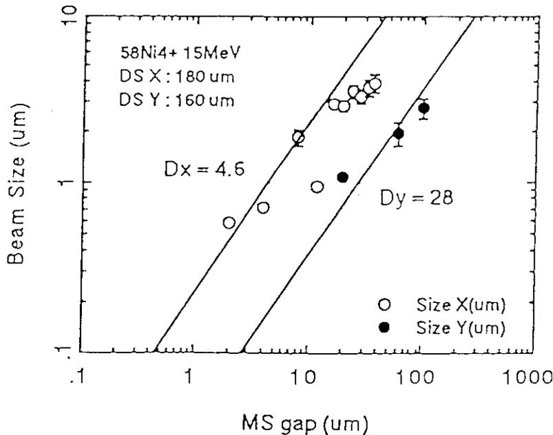
Fig. 3 Beam spot sizes in X and Y directions as functions of MS gaps. Solid lines indicate demagnification factors for each direction.
