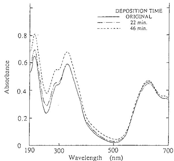
Fig. 3 UV absorption spectra of  $H_2Pc$  PVD thin films deposited with Cu by IBS method.  $Ar^+$  ion energy = 0.5 kV.
