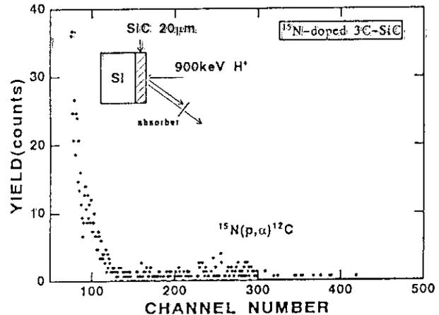
Fig.5 Energy spectrum for 900keV H<sup>+</sup> incident on  $^{15}\text{N}$ -doped SiC
