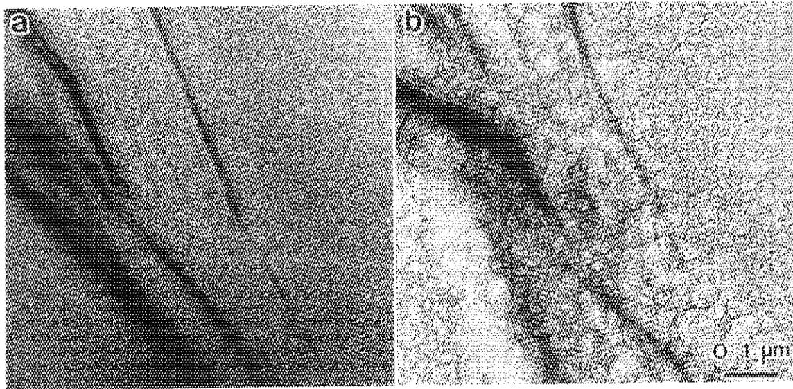
Fig.2 Structural changes of SiC during 15keV  $\text{H}_2^+$  and 12keV  $\text{He}^+$  simultaneous dual ion irradiation. The atomic fluxes of both hydrogen and helium were about  $1 \times 10^{14}$  (H,He)/ $\text{cm}^2$ . fluence:(a)  $1.8 \times 10^{17}$  (He)/ $\text{cm}^2 + 1.8 \times 10^{17}$  (H)/ $\text{cm}^2$ , (b)  $2.7 \times 10^{17}$  (He)/ $\text{cm}^2 + 2.7 \times 10^{17}$  (H)/ $\text{cm}^2$ .
