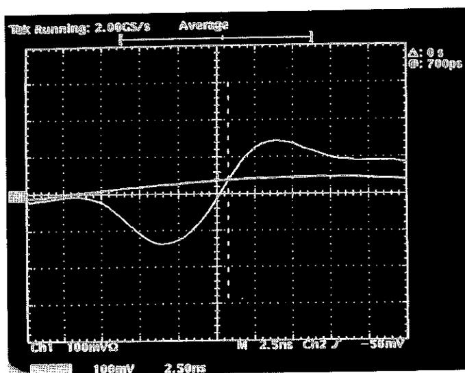
Fig.10 Pickup signal of the phase probe induced by ion beams.
