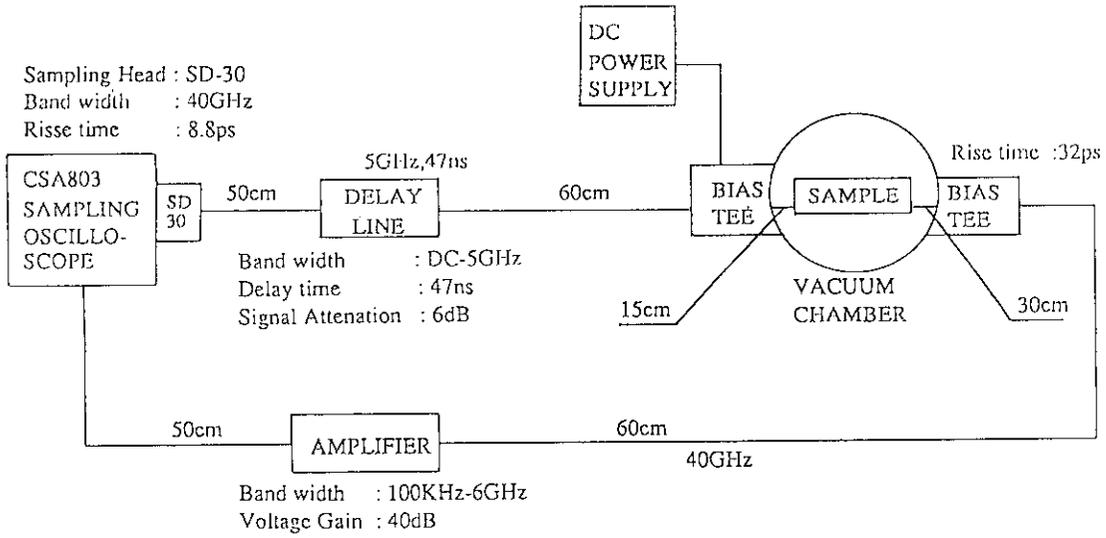
Figure 1. Block diagram of the electronic system for transient current measurements.
