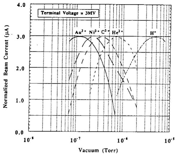
Fig.5 Beam Currents Measured for Several Ion Species at 3MV as a Function of Stripper Gas Pressure.
