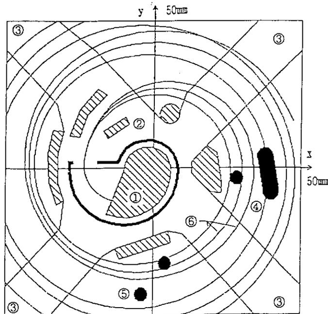
Fig.9 Schematic drawing of the central region of the cyclotron. (1)Inflector, (2)Puller, (3)Dee gap, (4)Phase slit II, (5)Phase slit I, (6)Beam trajectories(dee voltage of 40, 50 and 60 kV).
