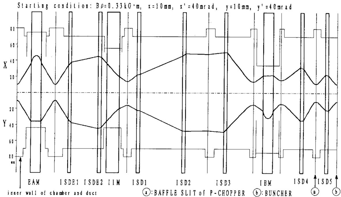
Fig.4 Beam envelope for the JAERI ECR ion source.
