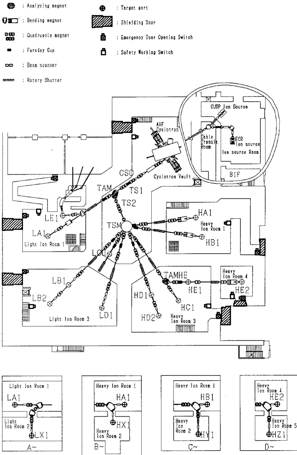
Fig. 1 Beam transport system.
