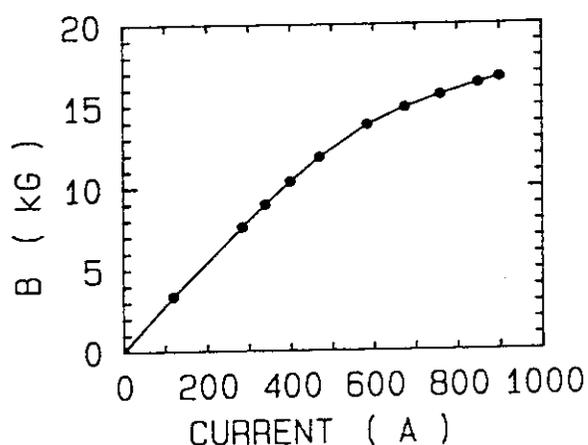
Fig.3 Excitation curve of the cyclotron magnet at an extraction radius of 923 mm.
