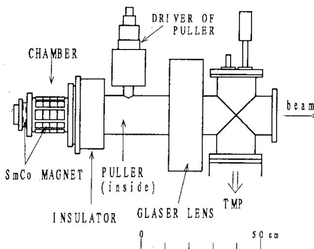
Fig.2 Side view of the multi-cusp ion source.
