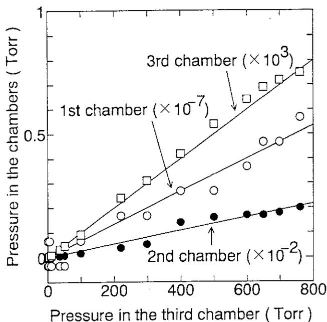
Fig.2 The relationship between the amount of pressure increase in three chambers and the controlled pressure of the third chamber.
