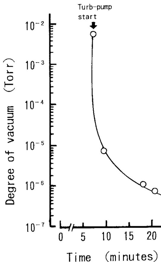
Fig. 4 Efficiency of evacuation for the irradiation apparatus
