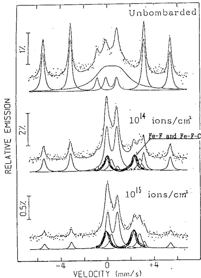
Fig.1 Mössbauer spectra of  $^{57}\text{Fe}$  atoms on Teflon before and after irradiation
