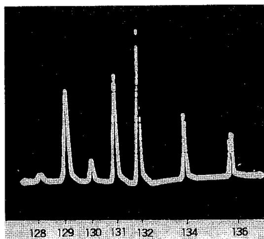
Fig. 2 Mass spectrum of Xe obtained with the ISOL.
