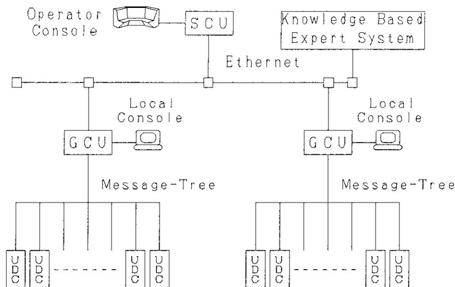
Fig.1 Architecture of the cyclotron control system.
