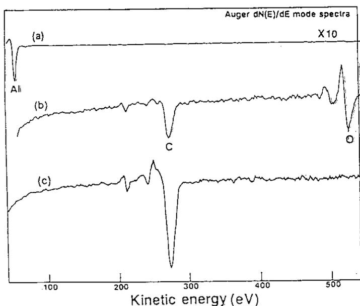
Fig.3 AES spectra of the carbon film deposited on poly-aluminium
