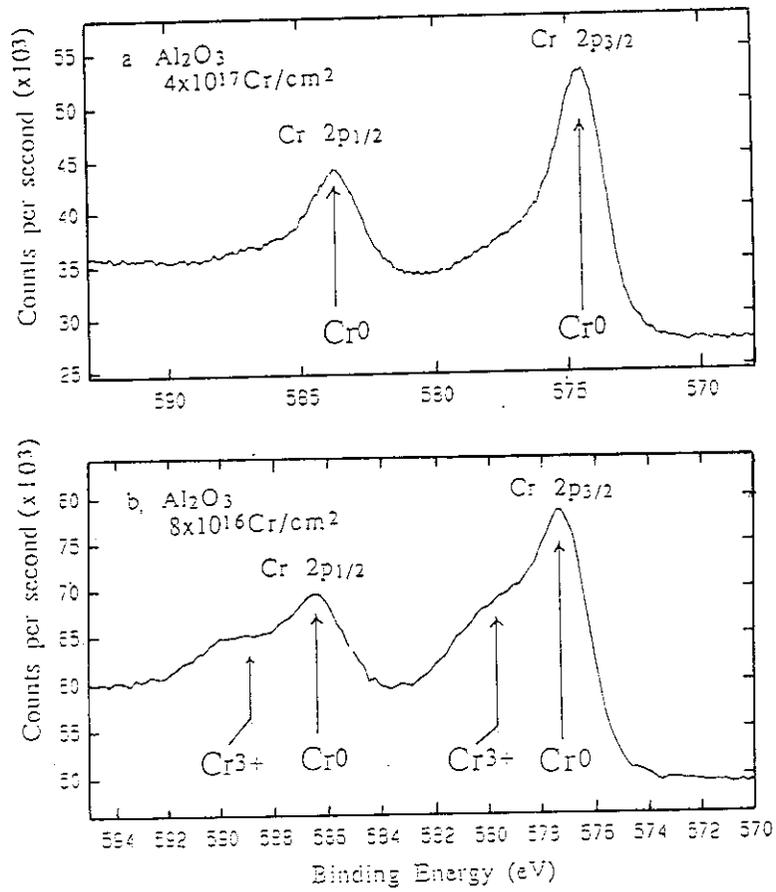
Fig. 1 Cr  $2p_{3/2}$  and Cr  $2p_{1/2}$  spectra from the implanted  $\alpha$ - $\text{Al}_2\text{O}_3$  crystals. The peaks in b shift to higher energy due to charging up of the sample surface during XPS measurement.
