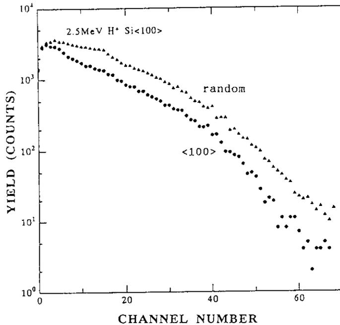
Fig.1 Energy spectra of secondary electrons induced by 2.5-MeV protons under <100> and random incidence conditions, measured at 180° with respect to the beam direction. The width of 1 channel corresponds to 0.096 keV.
