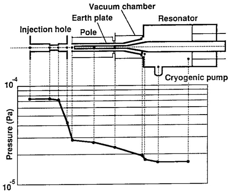
Fig.5 Pressure distribution in the JAERI AVF cyclotron.
