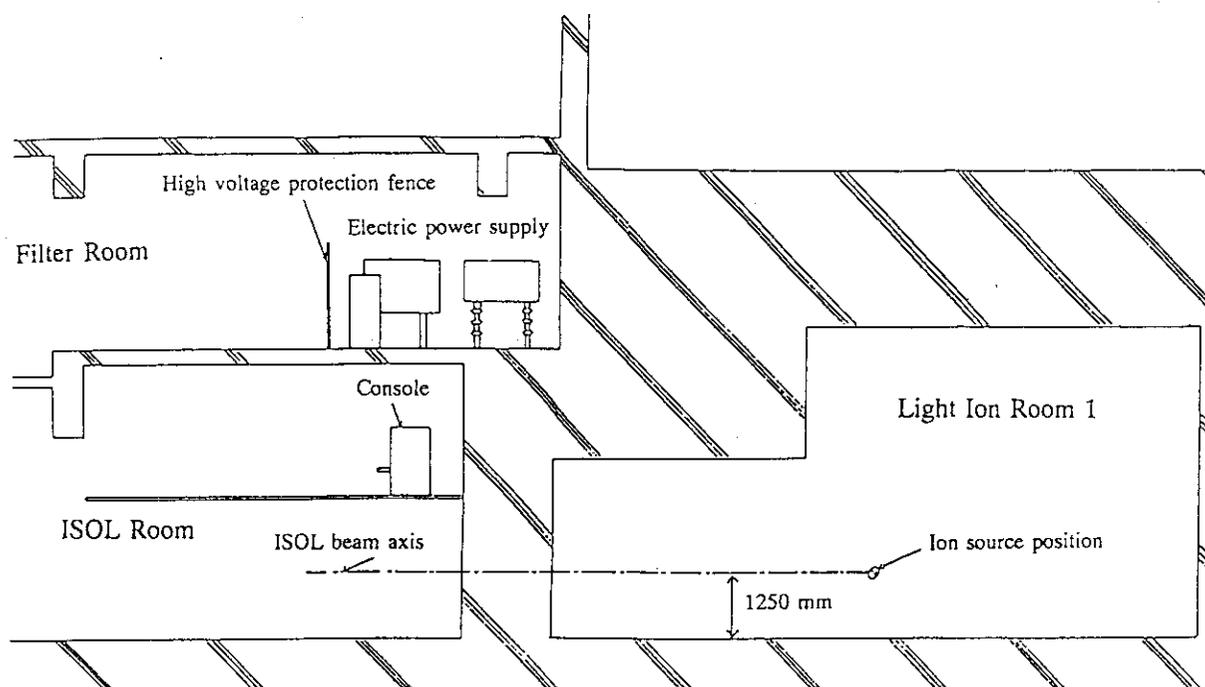
Fig. 3 Arrangement of the ISOL system.
