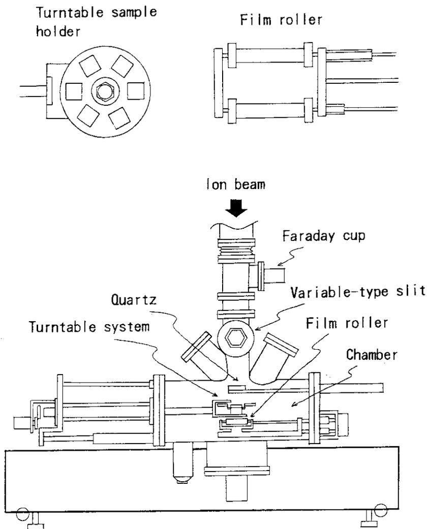
Fig. 3 Illustration of the irradiation apparatus
