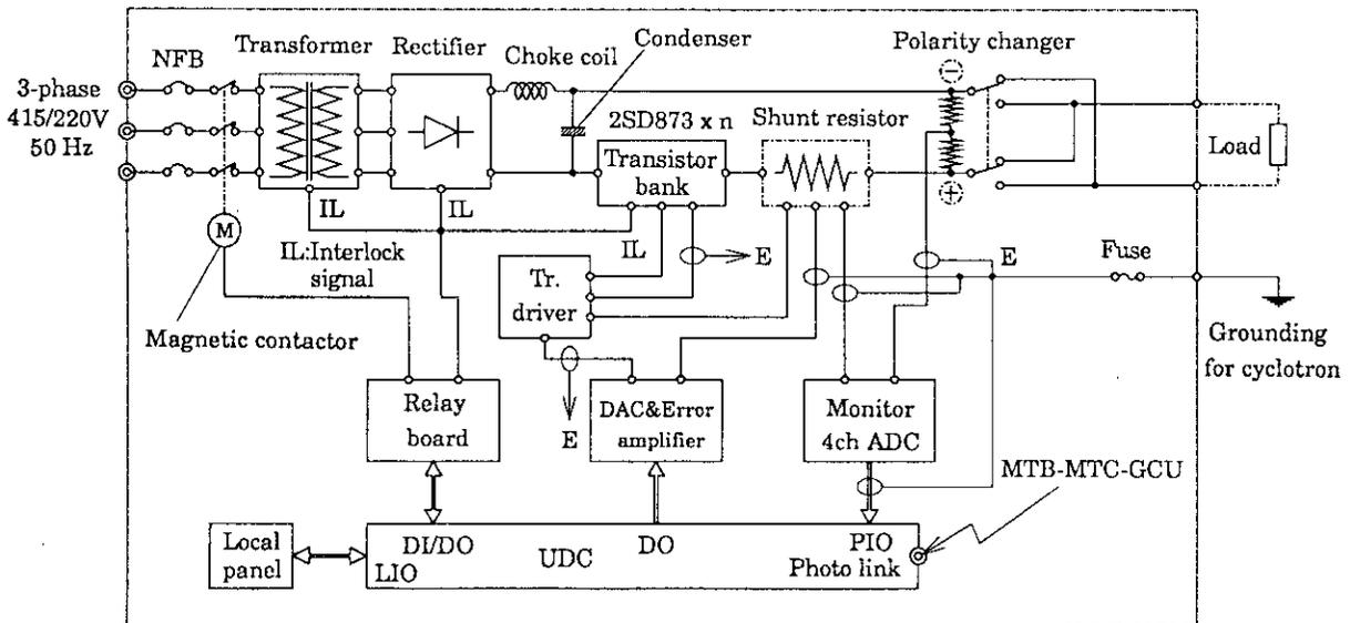
Fig. 3 Block diagram of a power supply for each magnet.
