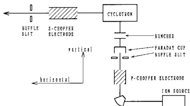
Fig.1 Schematic layout of beam chopping system.
