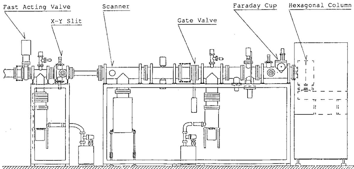
Figure 1. Irradiation Apparatus for Cell
