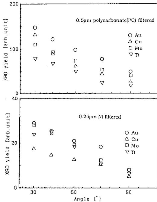
Fig.3 Angular distributions of the emitted X-ray intensity.
