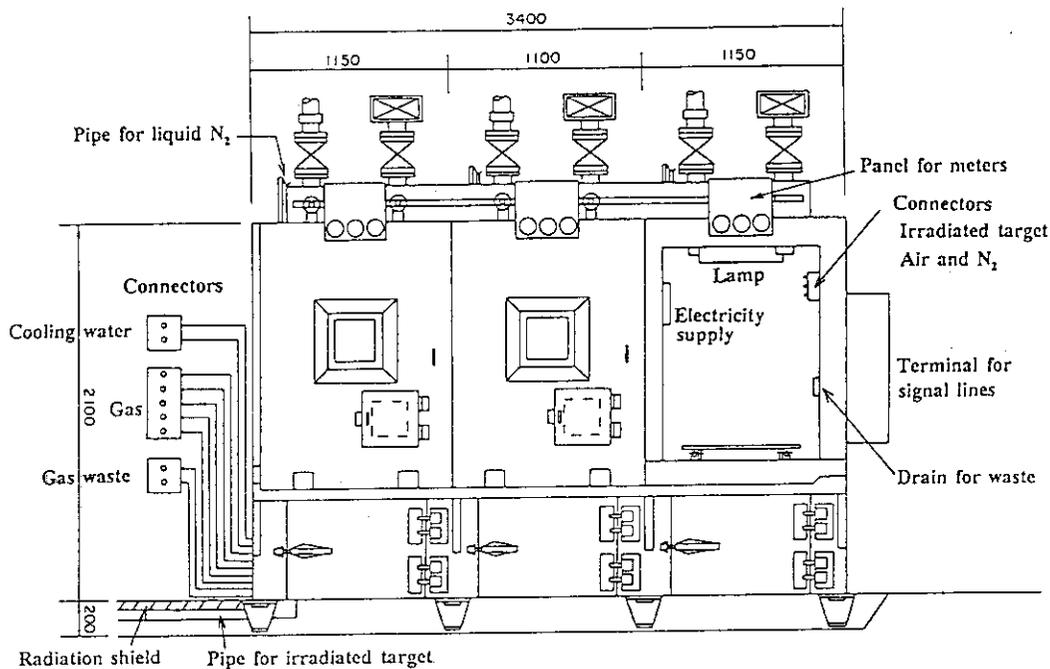
Fig. 5 The CBB cells in which CBBs for labeled compound synthesis are placed.
