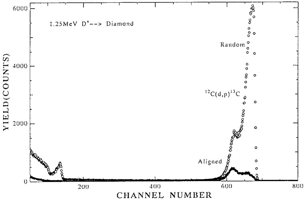
Fig. 2. NRA spectrum from (100) diamond crystal for  $\text{D}^+$  beam incident along a random direction and along the  $\langle 100 \rangle$  axis.
