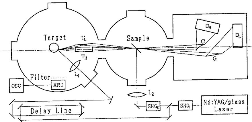
Fig.1 A schematic diagram of the time-resolved soft X-ray absorption spectroscopy apparatus using laser produced plasma X-rays.
