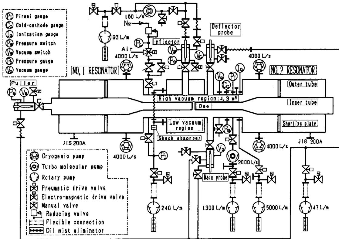
Fig.2 Vacuum system of the JAERI AVF cyclotron.
