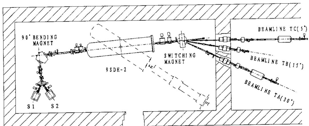
Fig.1 Layout of the 3MV Tandem Accelerator System, S1 and S2 are Negative Ion Sources.
