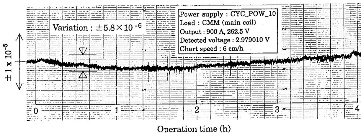
Fig. 4 Measured stability of the power supply when 900 A current was supplied to the cyclotron main coil.
