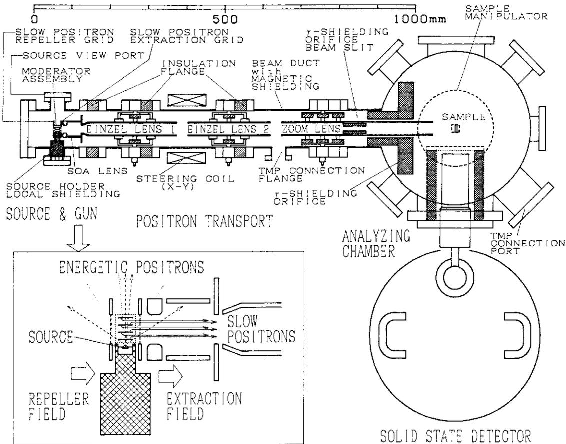
Fig.2. A concept of PALADIS (Positron Annihilation Lattice Defect Investigation System)
