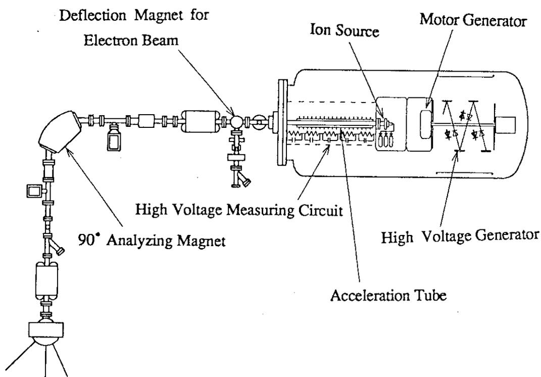
Fig. 1. General layout of the 3 MV D.C. Accelerator
