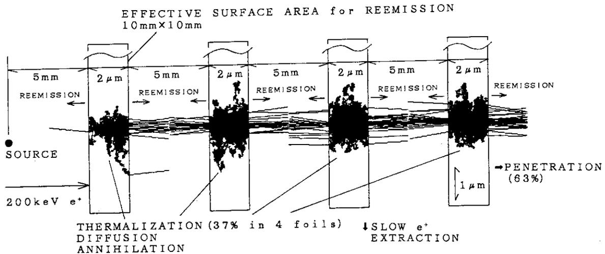
Fig.3. The Monte Carlo simulation on positron behavior in the new moderator configuration in PALADIS.
