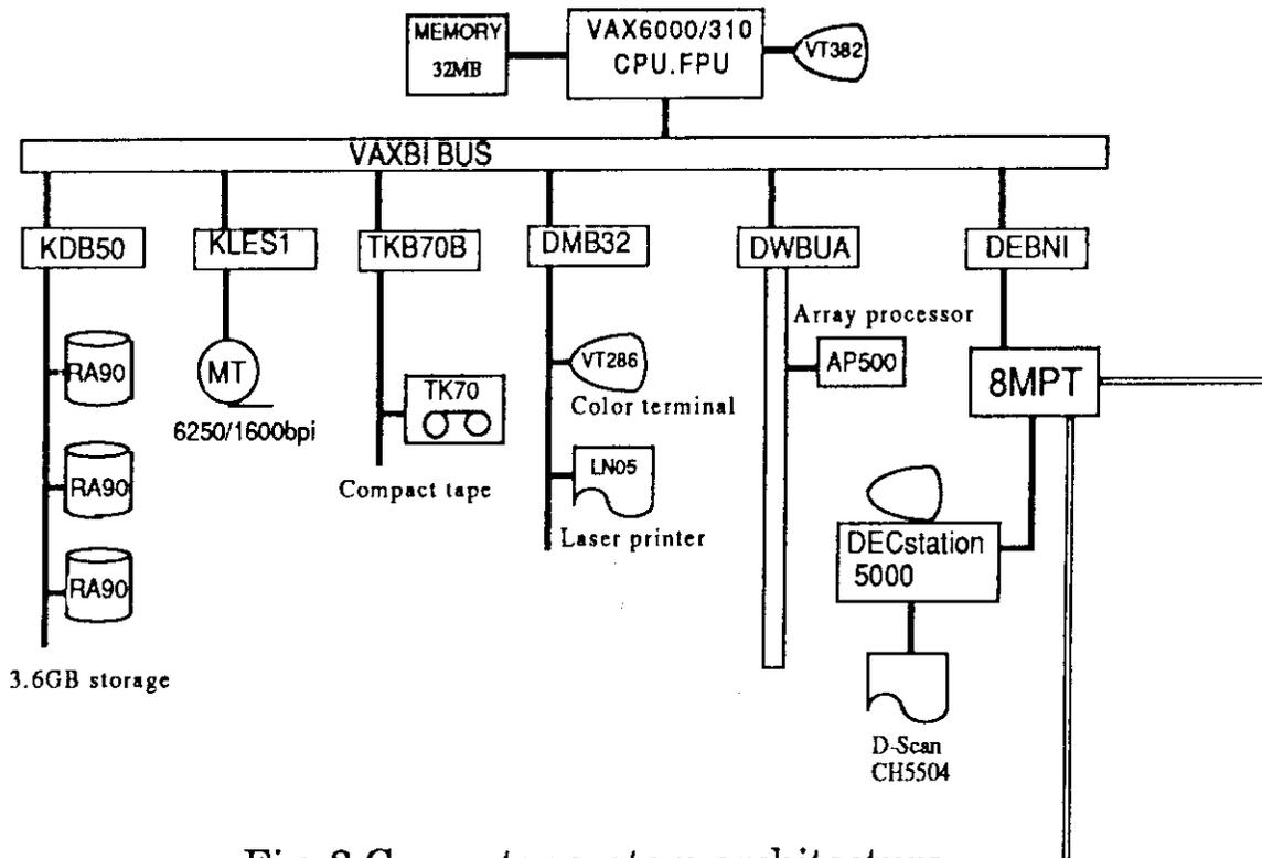
Fig. 2 Computer system architecture
