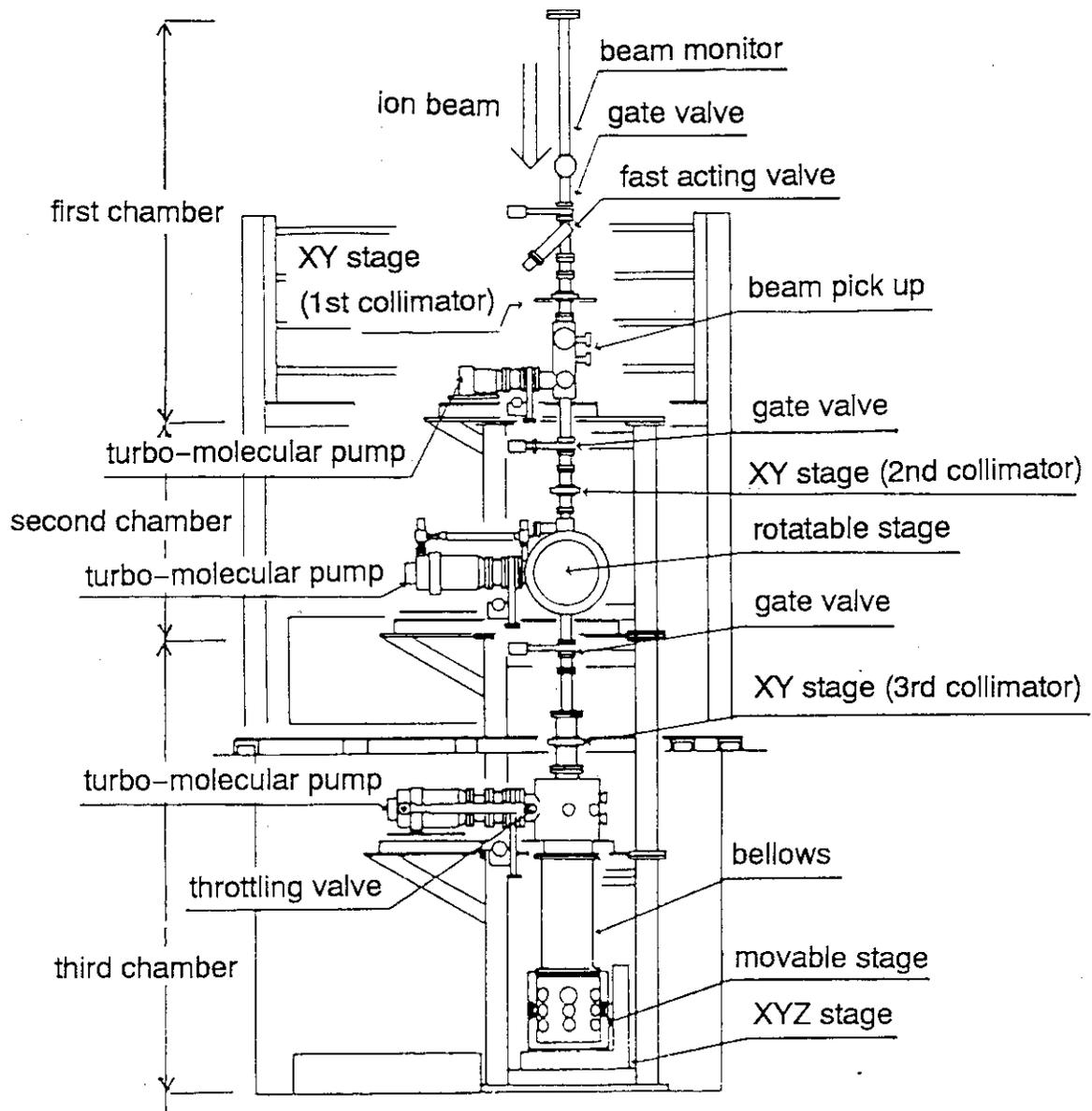
Fig.1 Schematic diagram of EA-BRACHI
