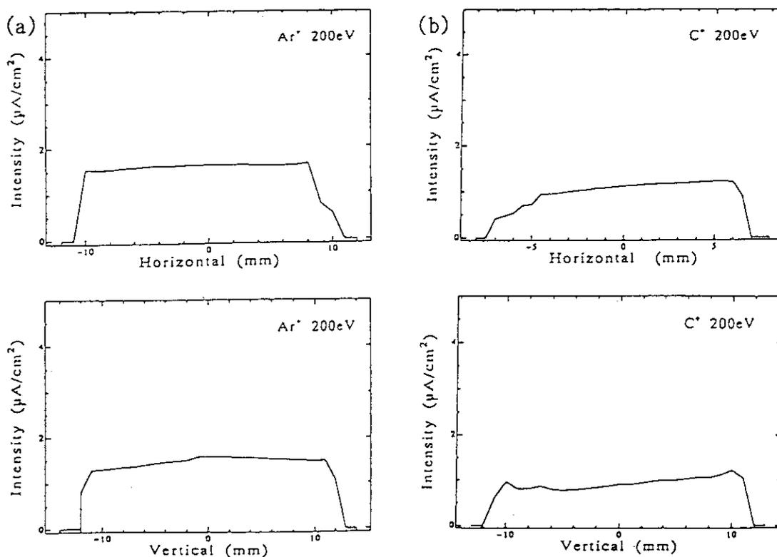
Fig.2 Beam profile for 200 eV (a)  $\text{Ar}^+$  and (b)  $\text{C}^+$
