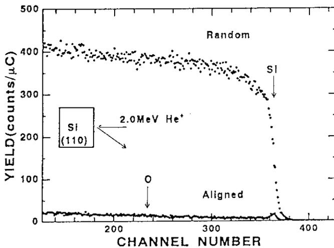
Fig.1 Energy spectra for 2.0 MeV He incident on Si(100) under random and aligned conditions
