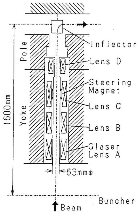
Fig.8 Layout of the axial injection system.
