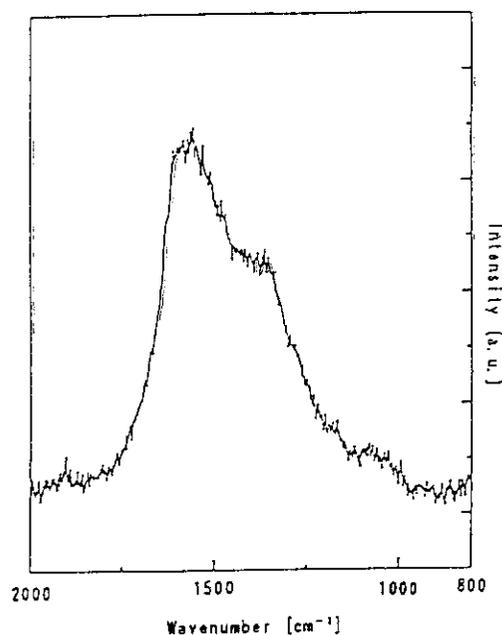
Fig.4 Raman spectrum of the carbon film deposited on poly-aluminium
