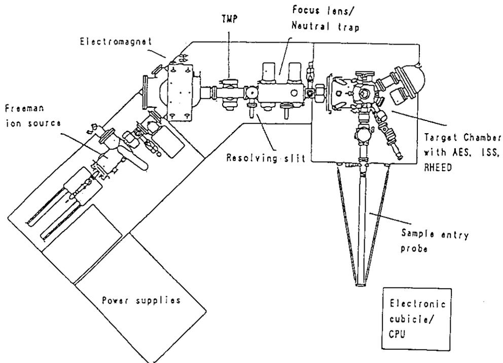
Fig.1 Plan view of the ultra-low energy ion beam deposition system
