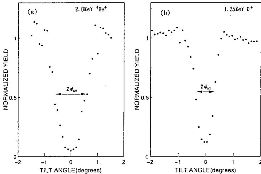
Fig. 3. Angular profiles for (100) diamond crystal, (a) from RBS of 2.0MeV  $^4\text{He}$  and (b) from NRA of 1.25MeV  $\text{D}^+$ .
