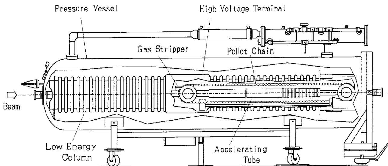
Fig.2 Structure of the 3MV Tandem Accelerator.
