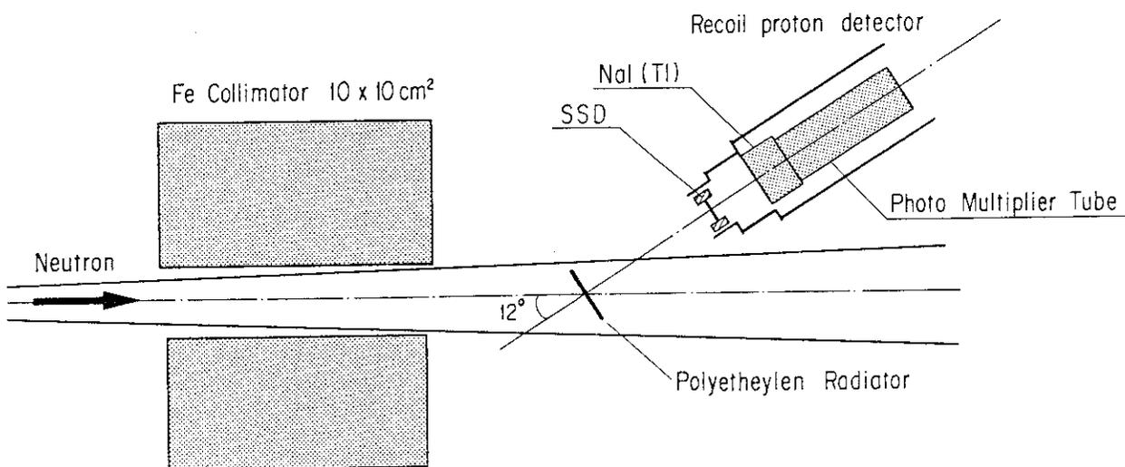
Fig.2 Arrangement of neutron spectrum measurement with the recoil proton telescope.
