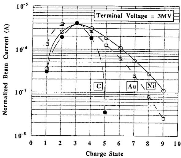
Fig.4 Charge State Distributions of C, Ni and Au Ions at 3MV after Passing Through the Stripper Gas.
