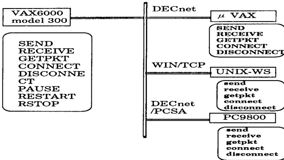
Fig. 3 Schematic diagram communication program
