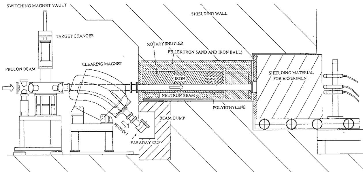
Fig.1 Schematic view of the monoenergetic neutron beam line.
