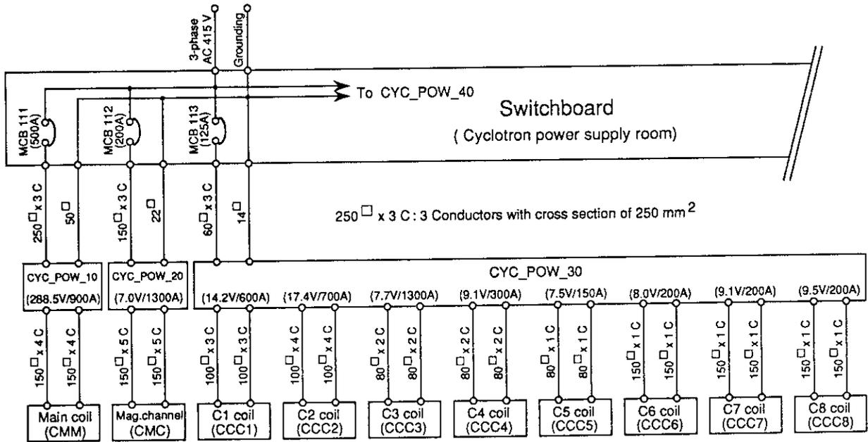
Fig. 2 Circuit diagram of three-phases 415 V lines for the power supplies of AVF cyclotron.
