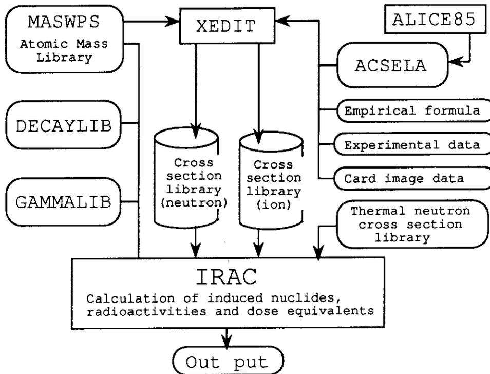
Fig. 1 Flow chart of induced radioactivity calculation in the IRAC code system
