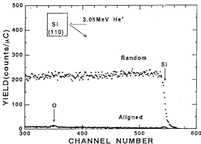
Fig.2 Energy spectra for 3.05 MeV He incident on Si(100) under random and aligned conditions
