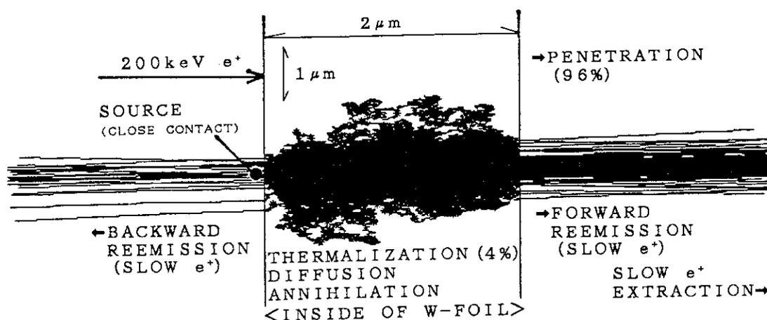
Fig.1. The Monte Carlo simulation on positron behavior in the conventional moderator configuration.
