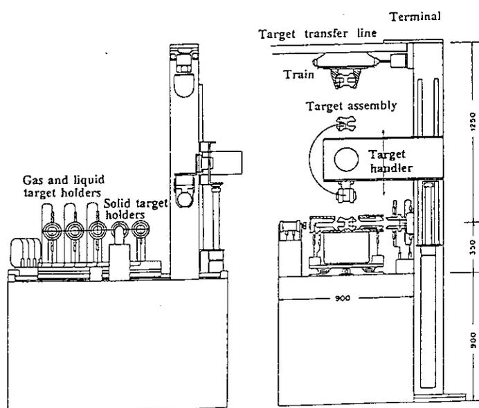
Fig.2 The irradiation apparatus of gas, liquid and solid targets and the terminal of solid-target transfer line equipped with a manipulator of solid target assembly.
