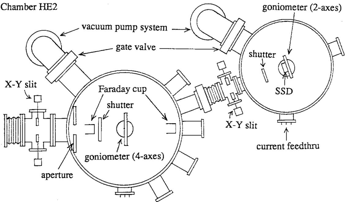
Fig.1 Heavy-ion irradiation system.
