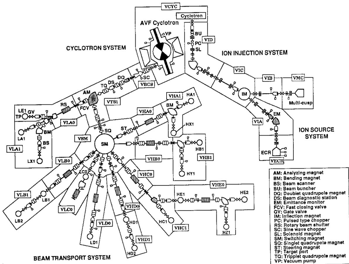
Fig.1 General construction and division of vacuum sections on the vacuum system for JAERI AVF cyclotron.
