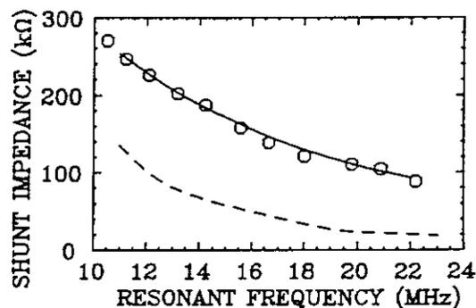
Fig.7 Frequency dependence of shunt impedance. The solid line shows 75 % of the calculated value based on one-dimensional transmission-line approximation. The dashed line shows the measured value of the movable-panel type cavity.
