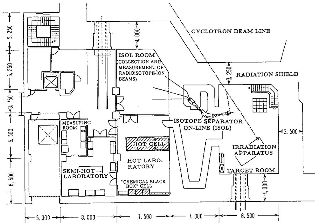
Fig.1 The radioisotope production facility in TIARA/JAERI utilizing ion beams from AVF cyclotron.
