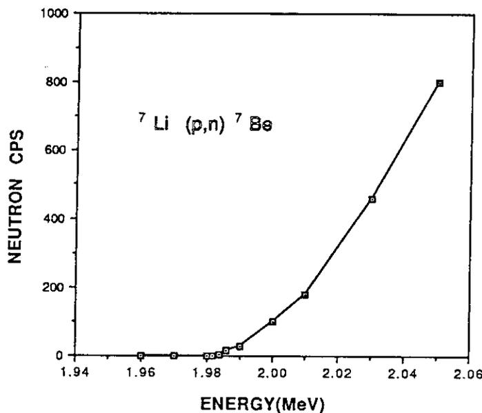
Fig.3 Measurement of the Threshold Proton Energy in the Nuclear Reaction  ${}^7\text{Li}(p, n)$  for Calibration of the Generating Voltmeter.
