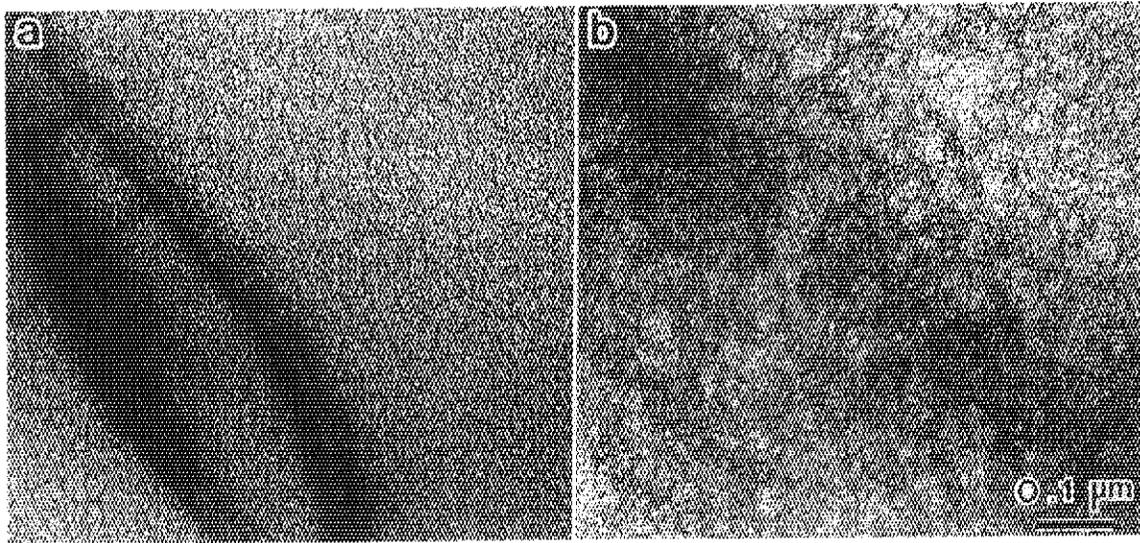
Fig.3 Structural changes of SiC during successive and alternative  $\text{He}^+$  and  $\text{H}_2^+$  ion irradiation. The atomic fluxes of both hydrogen and helium were about  $1 \times 10^{14}(\text{H,He})/\text{cm}^2/\text{sec}$ . fluence:(a)  $1.8 \times 10^{17}(\text{He})/\text{cm}^2$  (b)  $2.7 \times 10^{17}(\text{He})/\text{cm}^2 + 2.7 \times 10^{17}(\text{H})/\text{cm}^2$ .
