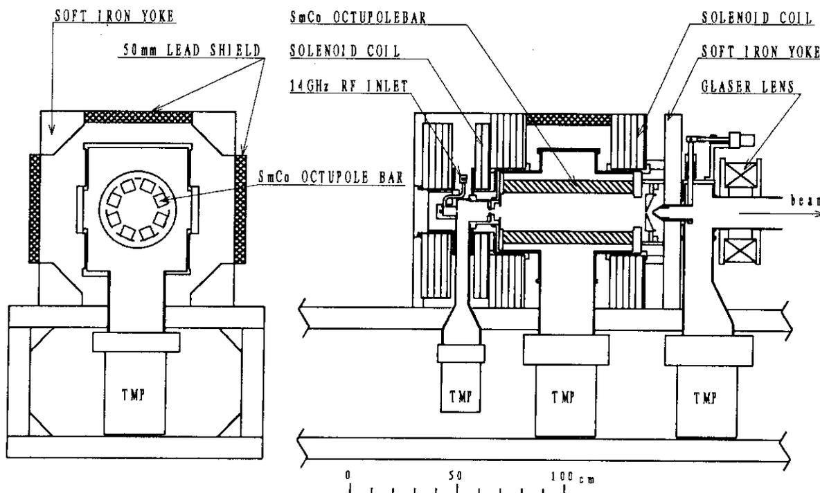
Fig.1 Cross section of the JAERI ECR ion source.
