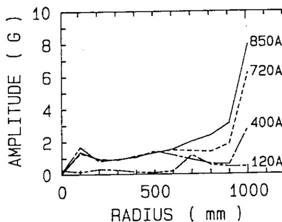
Fig.4 Radial Distributions of the first harmonic amplitude at four base field levels.
