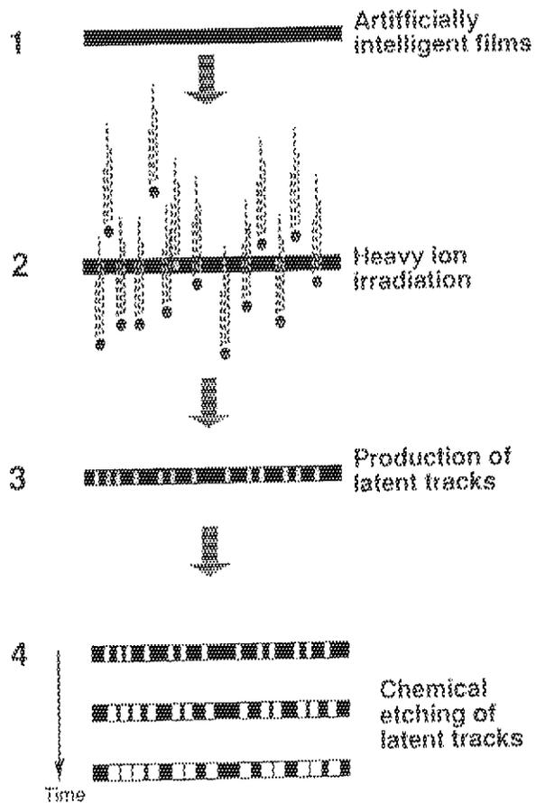
Fig. 1 Scheme for the fabrication of ion track pore in polymer films
