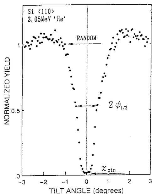
Fig. 1. Angular profiles for 3.05MeV  $^4\text{He}$  ions incident along  $\langle 110 \rangle$  axis of Si.
