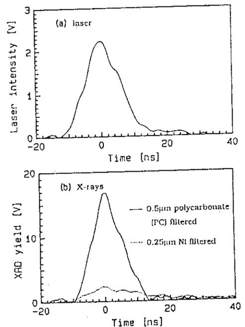
Fig.2 Pulse shapes of the laser and generated X-rays.
