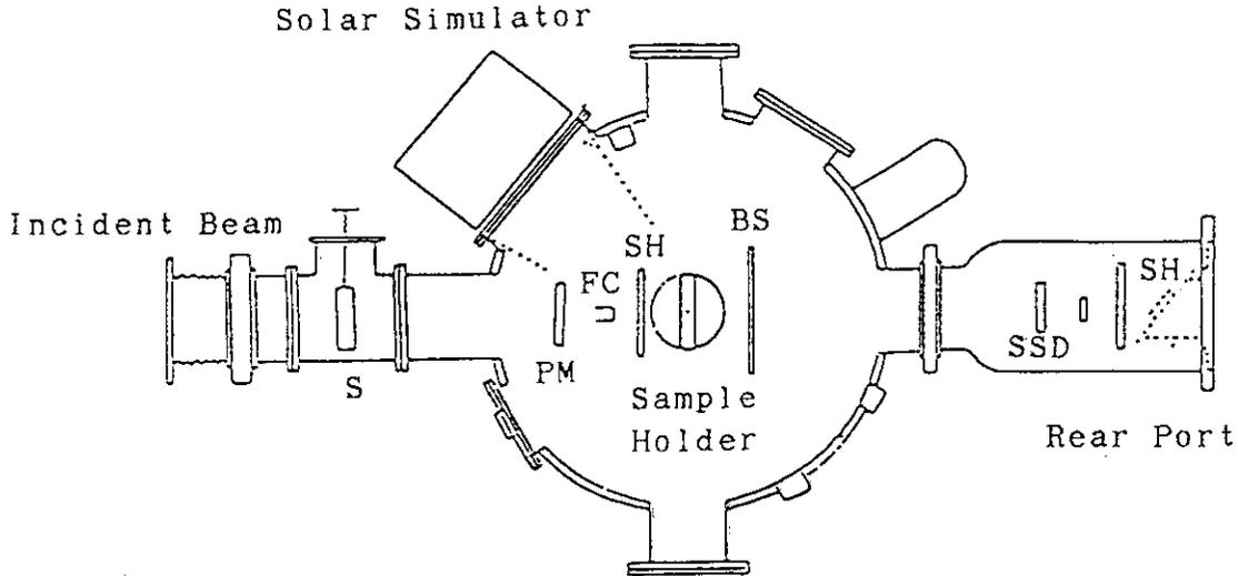
Fig. 1 Schematic Drawing of Chamber for Ion Irradiation of Solar Cells and Semiconductor Materials
