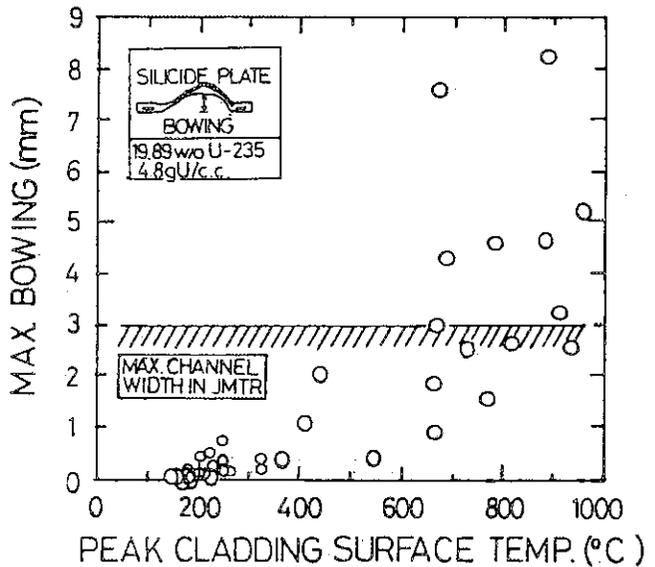
Fig. 12 Observed maximum bowing of silicide plate-type fuel from PIE, where five cuttings a plate fuel were made either of longitudinal (T/C #5) or of transversal sections (T/C #1-4) resulting in at least one T/C in a specimen
