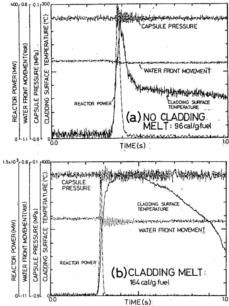
Fig. 10 In-core measurement of capsule pressure, water front movement, cladding surface temperature, and reactor power obtained from
