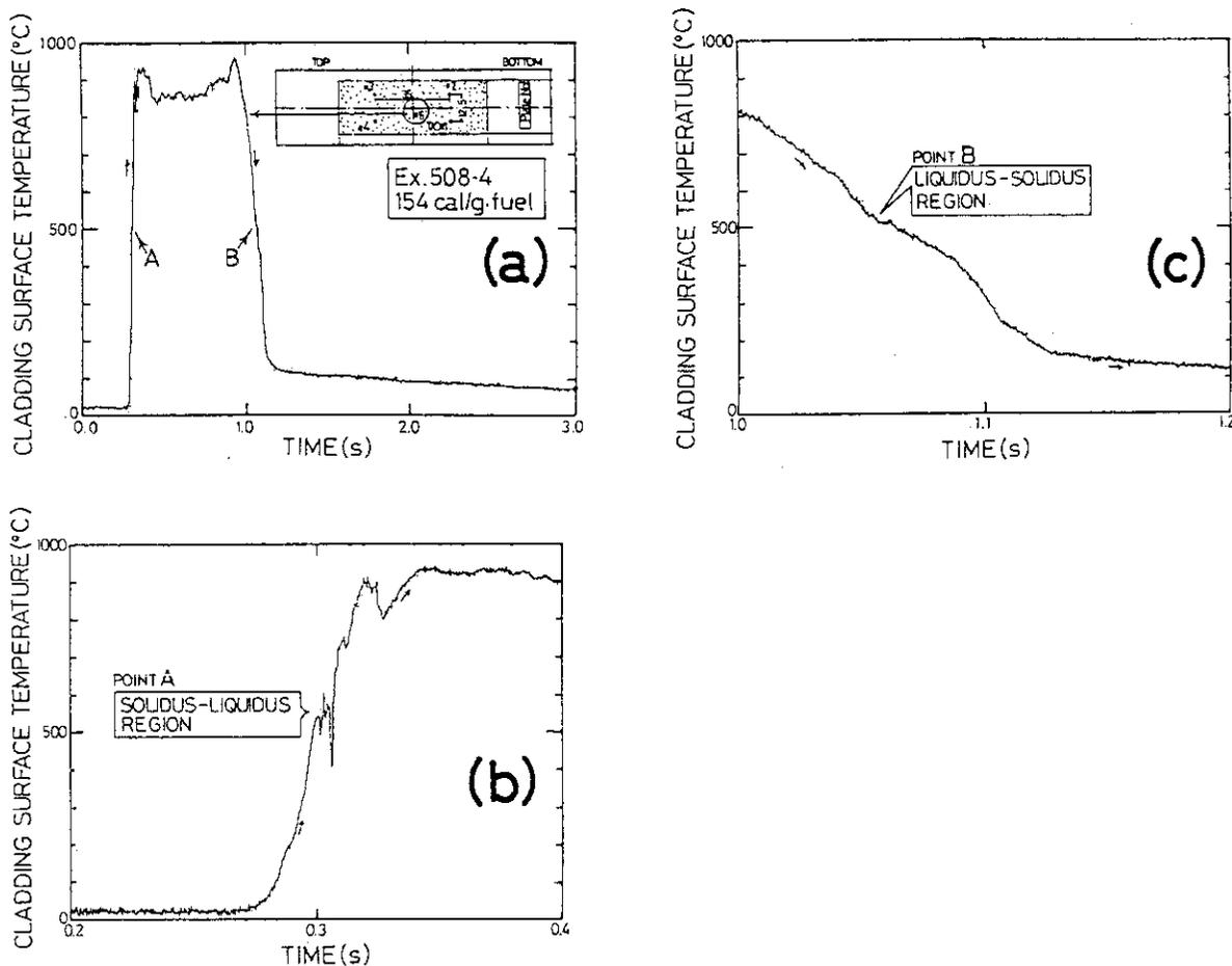
Fig. 7 Solidus-liquidus phase transformation of silicide plate fuel observed about 500°C in ex. 508-4 (154cal/g·fuel)
