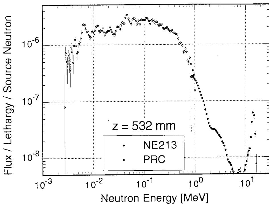
Fig. 3.1.1.8 Neutron spectra at 532 mm depth in the copper assembly measured by NE213 counter and proton-recoil gas proportional counters (PRC).
