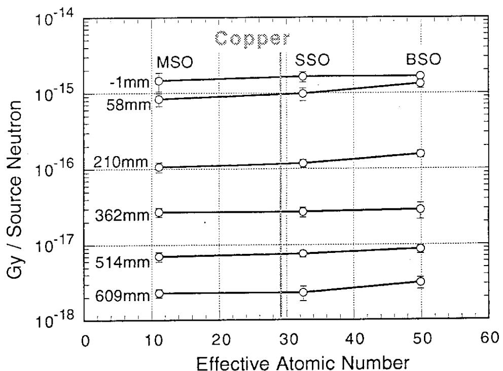
Fig. 3.4.2 Figure for explanation of derivation of gamma-ray heating rates of copper by interpolation.
