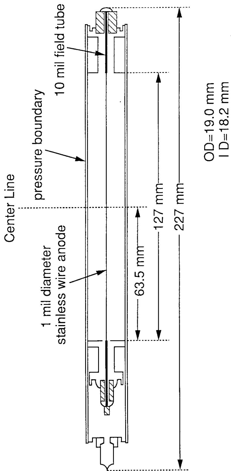
Fig. 3.1.2.1 Sectional view of the proton-recoil gas proportional counters (PRC).
