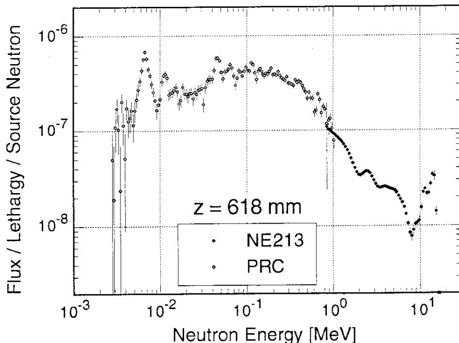
Fig. 3.1.1.9 Neutron spectra at the rear surface of the copper assembly measured by NE213 counter and proton-recoil gas proportional counters (PRC).
