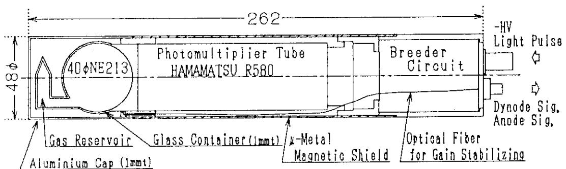
Fig. 3.3.1.1 Sectional view of the 40 mm diameter NE213 gamma-ray spectrometer
