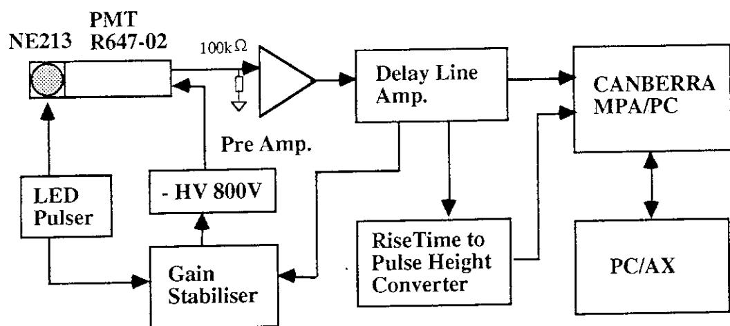
Fig. 3.1.1.3 Schematic diagram of electronic circuit.
