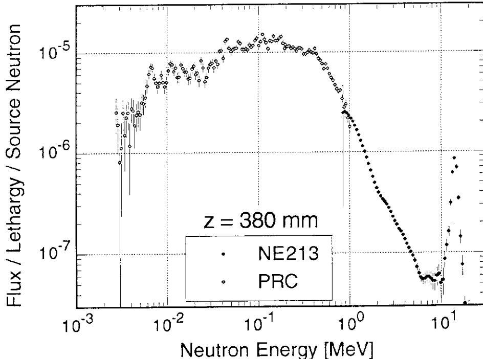
Fig. 3.1.1.7 Neutron spectra at 380 mm depth in the copper assembly measured by NE213 counter and proton-recoil gas proportional counters (PRC).
