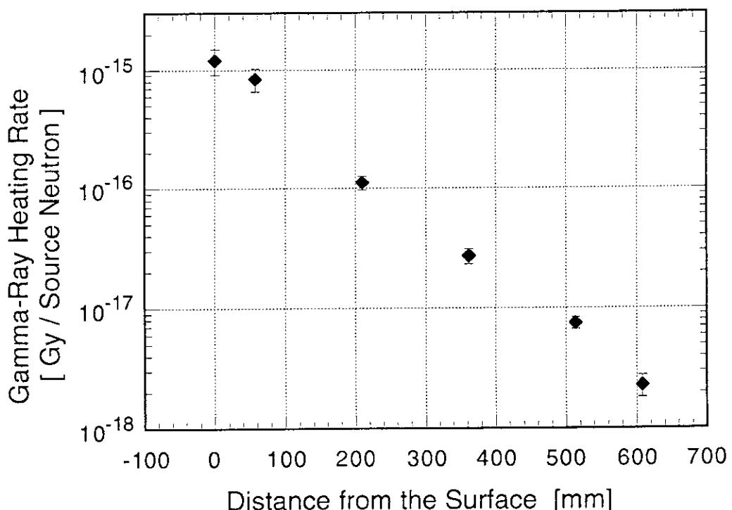
Fig. 3.4.3 Measured gamma-ray heating rates of copper in the copper assembly.
