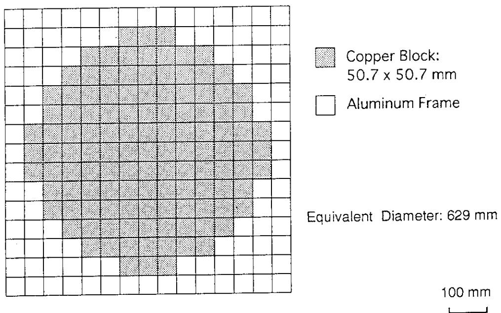
Fig. 2.1.2 Front view of the experimental assembly.
