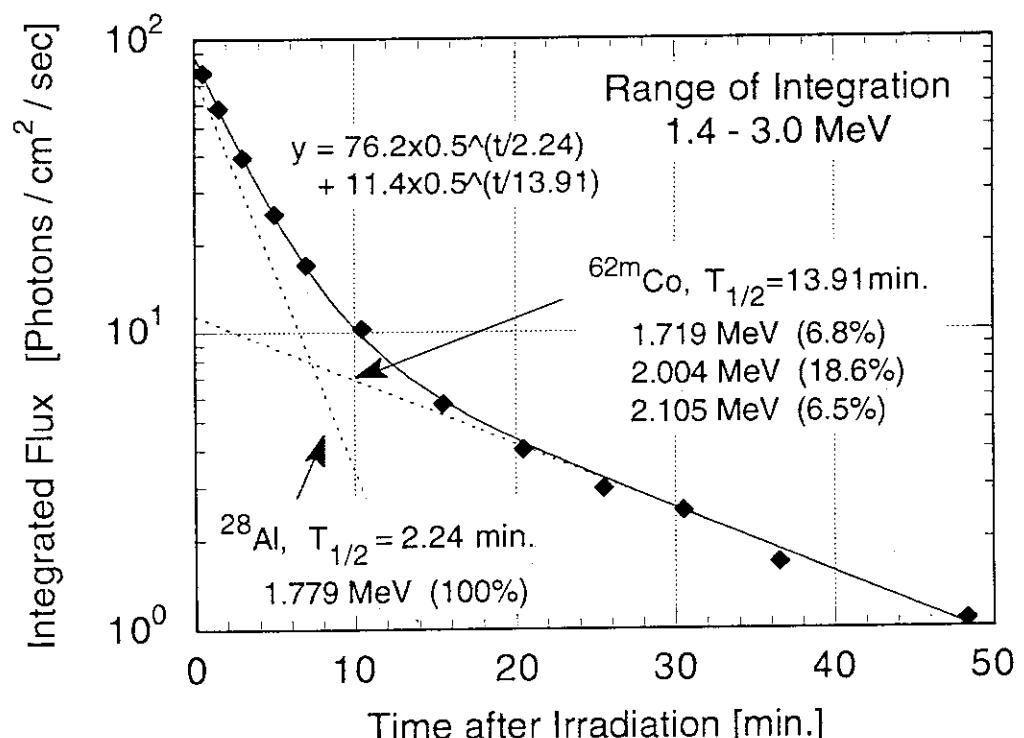
Fig. 3.3.2.5 Integrated decay gamma-ray spectra between 1.4 and 3.0 MeV as a function of cooling time.
