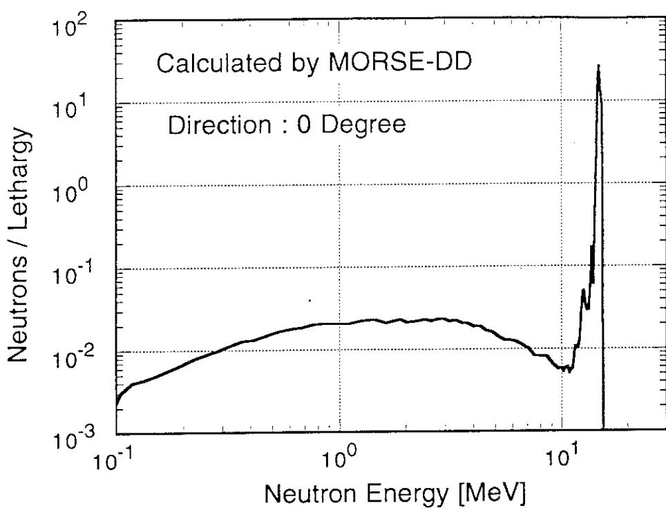
Fig. 2.2.2 Source neutron spectrum of the FNS fast water cooled target calculated with MORSE-DD.
