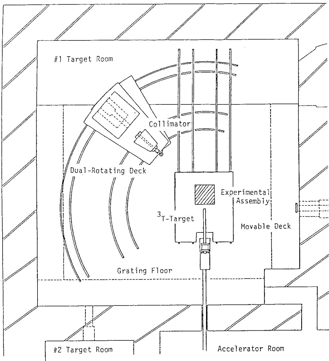
Fig. 2.1.1 Layout of the FNS first target room.
