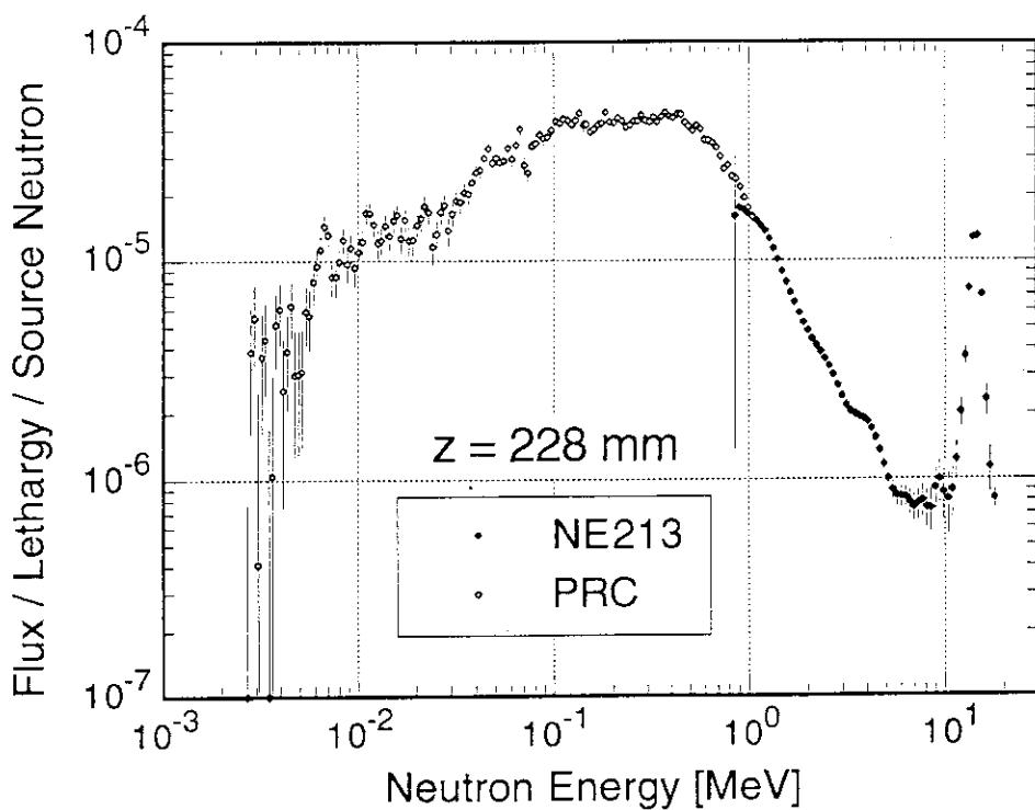
Fig. 3.1.1.6 Neutron spectra at 228 mm depth in the copper assembly measured by NE213 counter and proton-recoil gas proportional counters (PRC).
