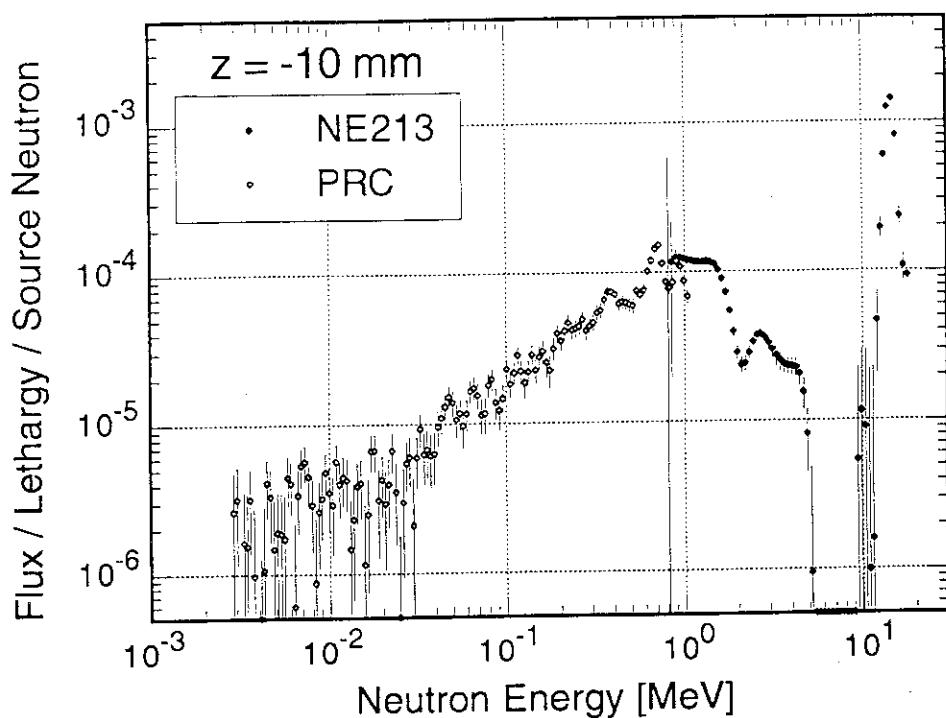
Fig. 3.1.1.4 Neutron spectra at the front surface of the copper assembly measured by NE213 counter and proton-recoil gas proportional counters (PRC).
