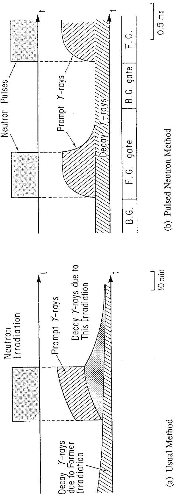
Fig. 3.3.1.3 Figure for explanation of rejection of decay gamma-rays. Amount of decay gamma-rays can not be determined accurately with (a) usual method but with (b) pulsed neutron method.
