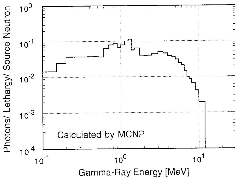
Fig. 2.2.3 Source gamma-ray spectrum of the FNS fast water cooled target calculated with MCNP.
