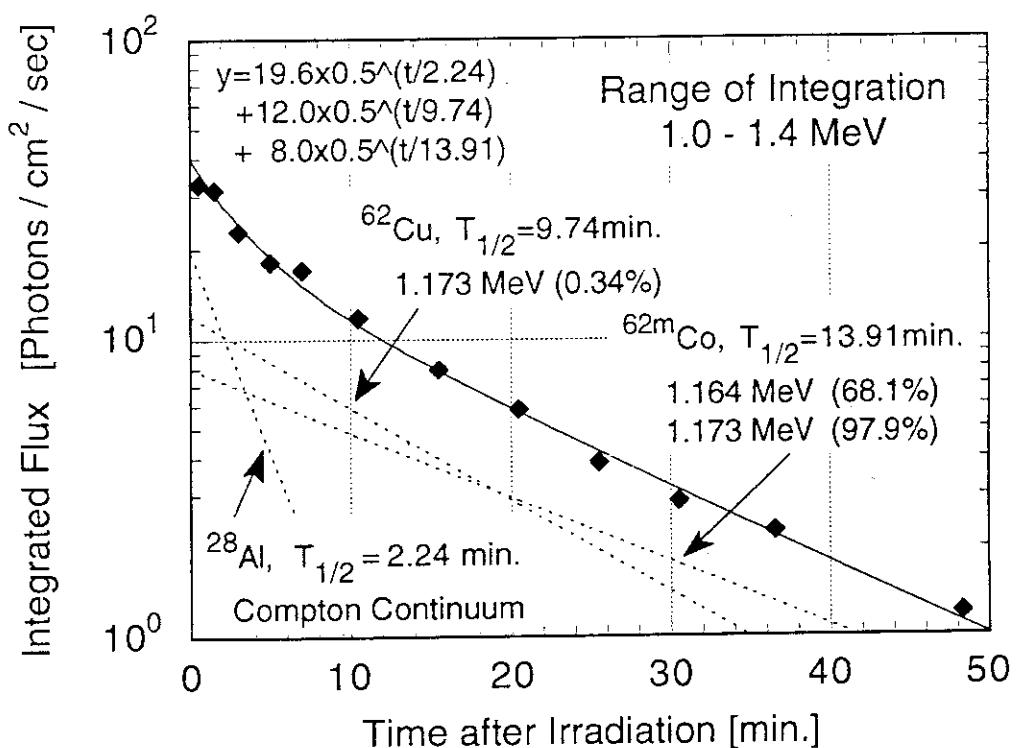
Fig. 3.3.2.4 Integrated decay gamma-ray spectra between 1.0 and 1.4 MeV as a function of cooling time.
