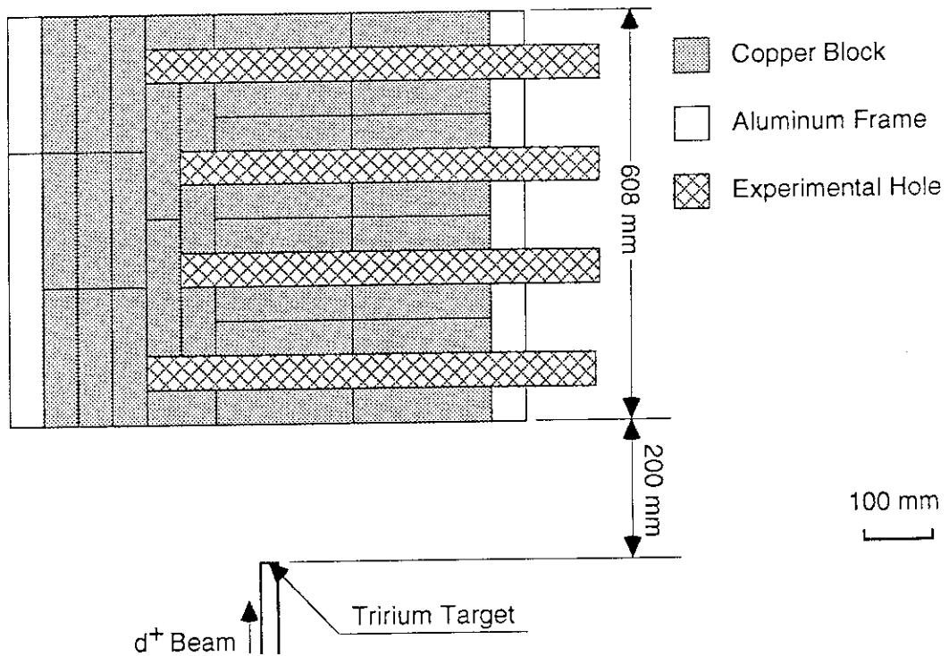
Fig. 2.1.3 Equatorial view of the experimental assembly.
