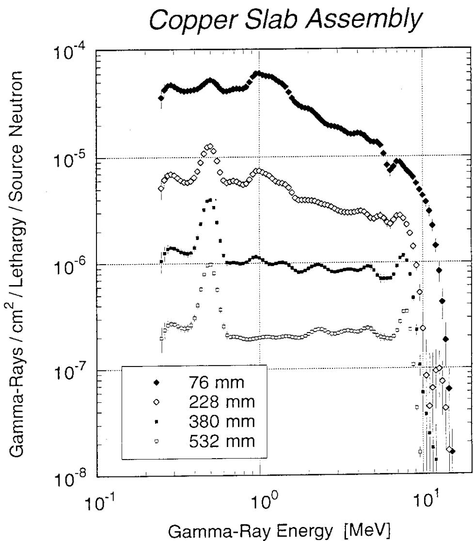
Fig. 3.3.1.4 Prompt gamma-ray spectra at 76, 228, 380 and 532 mm from the front surface of the copper assembly measured by the 40 mm diameter NE213 gamma-ray spectrometer.
