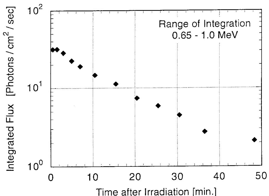
Fig. 3.3.2.3 Integrated decay gamma-ray spectra between 0.65 and 1.0 MeV as a function of cooling time.
