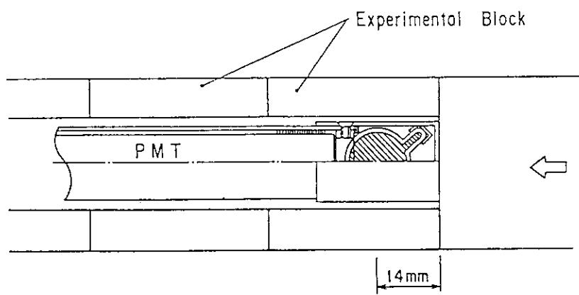
Fig. 3.1.1.2 Arrangement in measurement using the experimental drawer.
