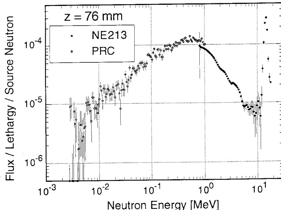
Fig. 3.1.1.5 Neutron spectra at 76 mm depth in the copper assembly measured by NE213 counter and proton-recoil gas proportional counters (PRC).
