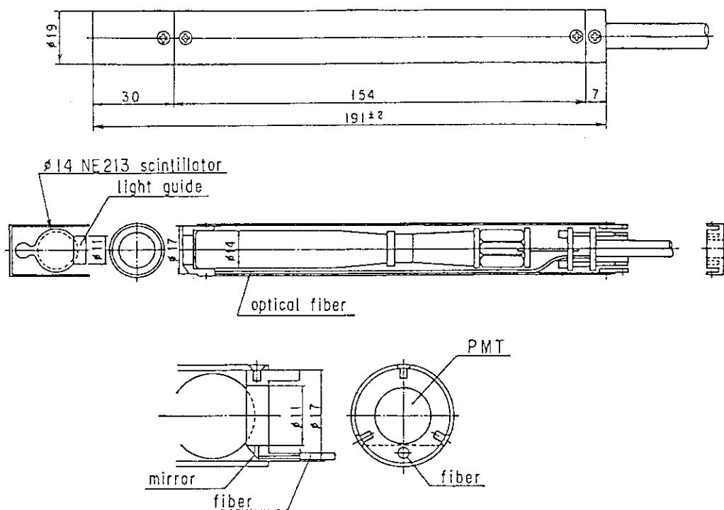
Fig. 3.1.1.1 Sectional view of small sphere NE213 scintillation detector assembly.
