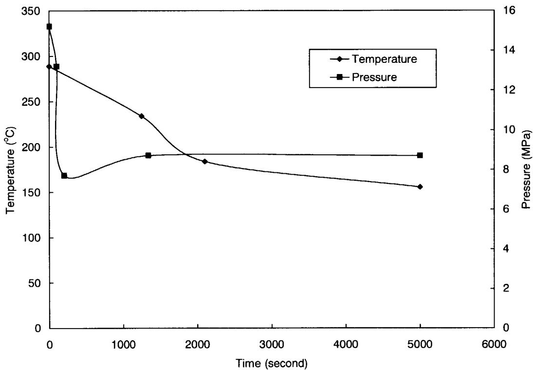
Fig.4 SB-LOCA (SB) transient
