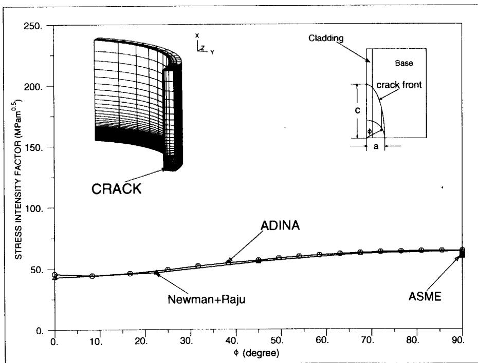
Fig.7 Comparison of stress intensity factor between different methods (no PTS)
