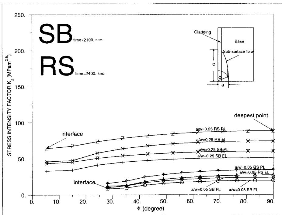
Fig.21 Comparison of  $K_J$  between elastic and plastic calculations for sub-surface flaw
