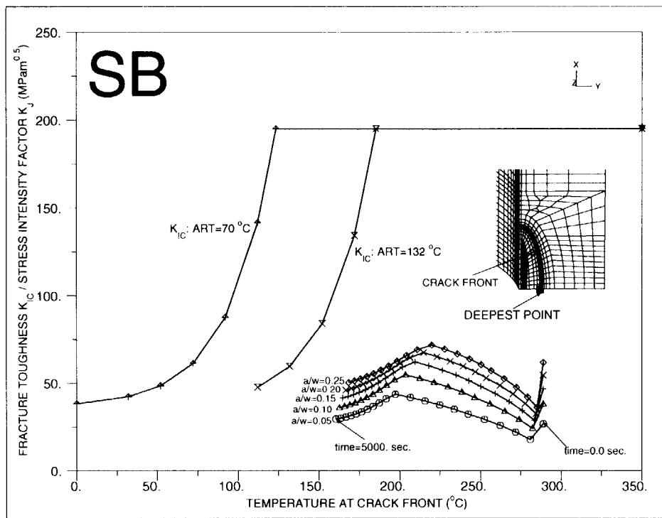
Fig.12 Fracture evaluation for shallow cracks under SB-LOCA
