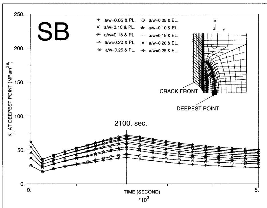
Fig.8 Comparison of  $K_J$  between elastic and plastic calculations under SB-LOCA
