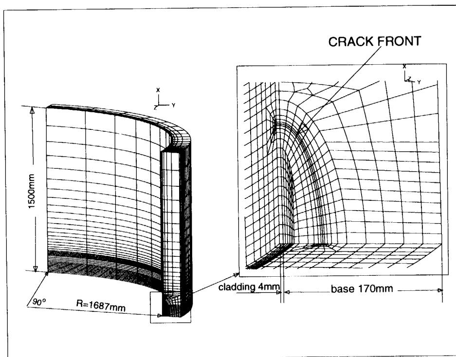
Fig.2 Structural model and mesh
