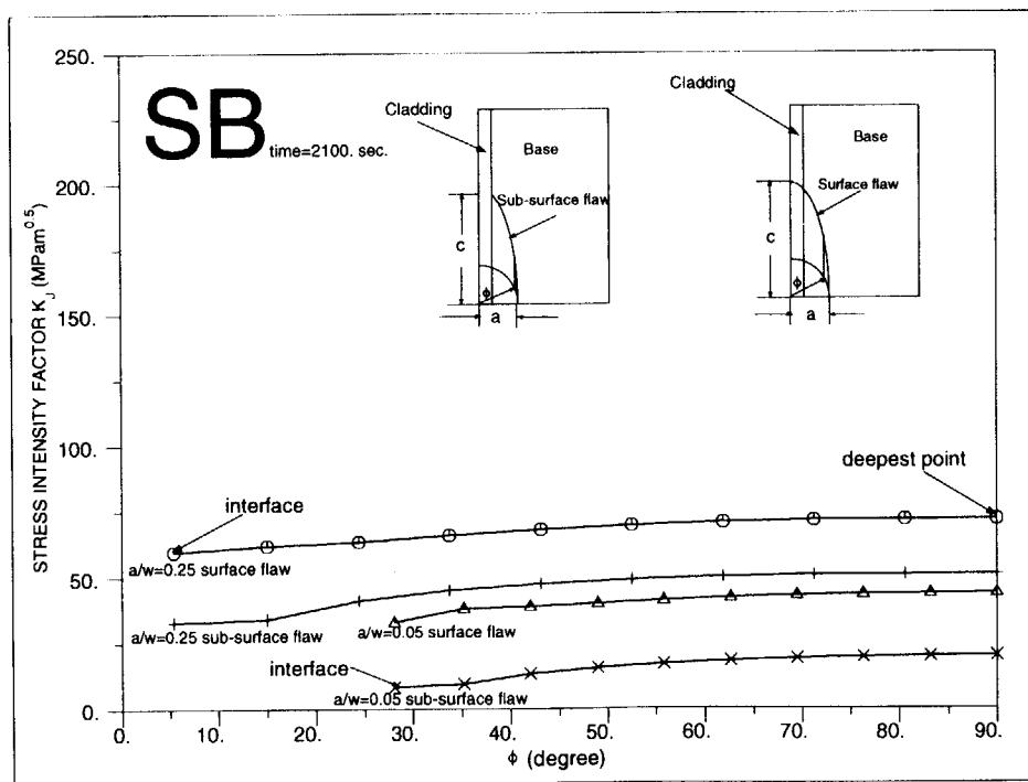
Fig.19 Comparison of  $K_J$  between surface and sub-surface flaw under SB-LOCA
