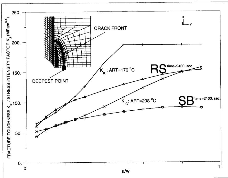
Fig.14  $K_J$  and  $K_{IC}$  for different flaws ( $a/w=0.05 \sim 0.9$ ) and PTS transients
