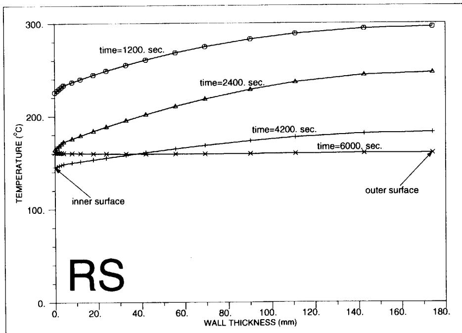
Fig. 11 Temperature distribution through the wall thickness under RS PTS
