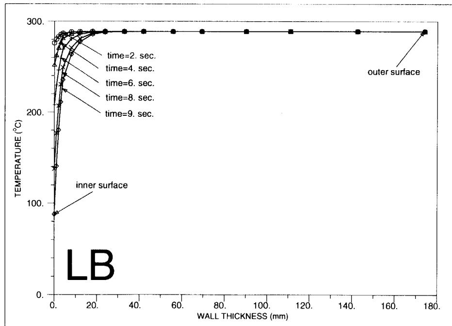
Fig. 17 Temperature distribution through the wall thickness under LB-LOCA
