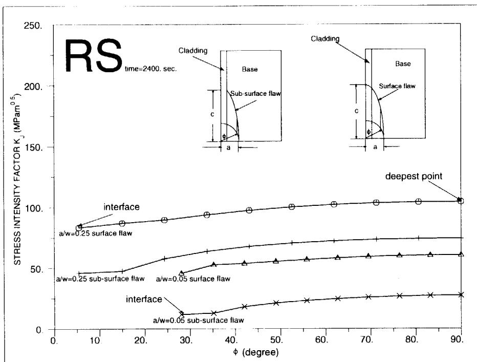
Fig.20 Comparison of  $K_J$  between surface and sub-surface flaw under RS PTS
