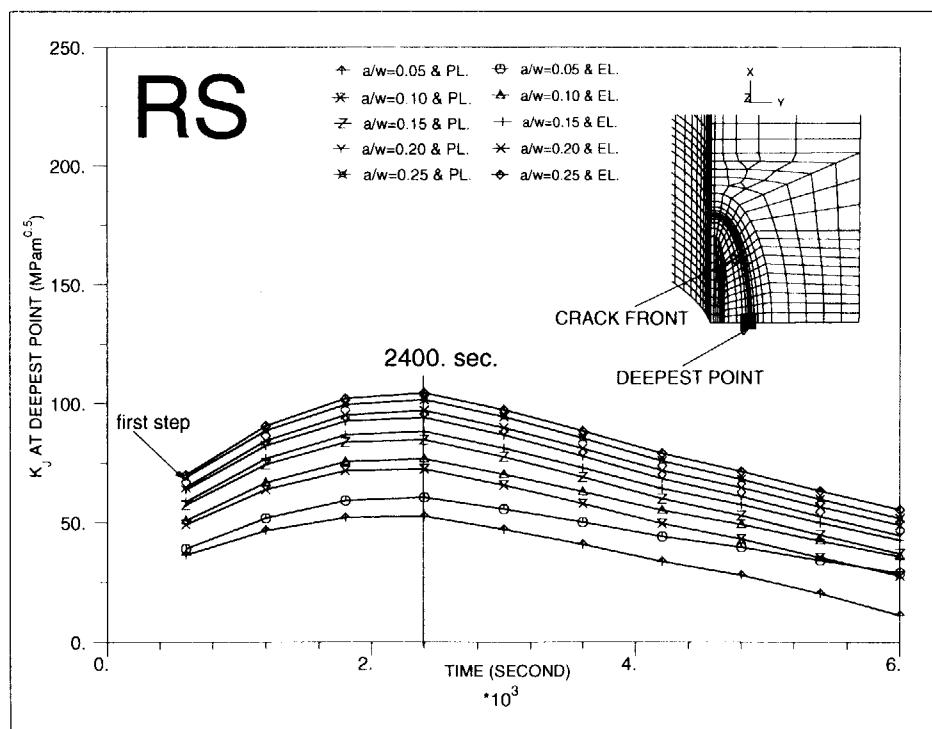
Fig.9 Comparison of  $K_J$  between elastic and plastic calculations under RS PTS
