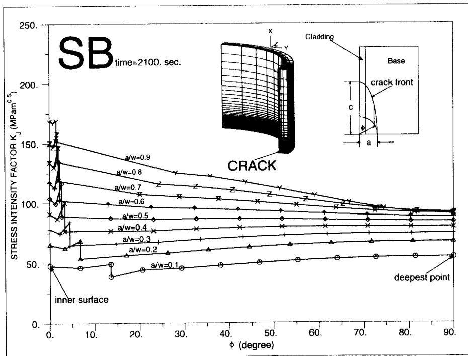
Fig.15 Distribution of  $K_J$  along crack front for  $a/w=0.1 \sim 0.9$  under SB-LOCA
