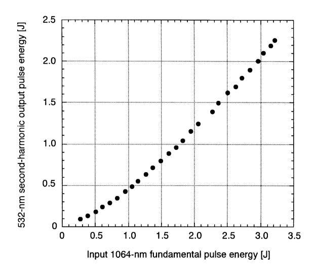
Fig.2 532-nm second harmonic output pulse energy as a function of the input 1064-nm fundamental pulse energy.
