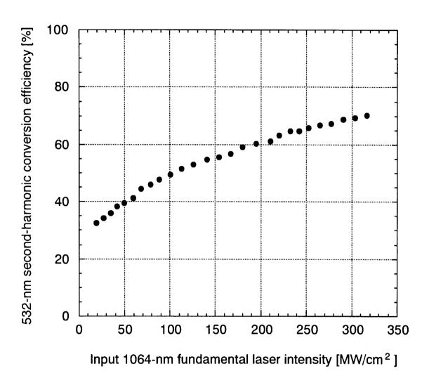
Fig.3 532-nm second-harmonic conversion efficiency as a function of the input 1064-nm fundamental laser intensity.
