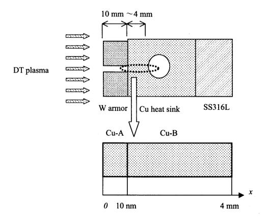
Fig. 2 Analytical geometry for the TMAP calculation of tritium permeation analysis.
