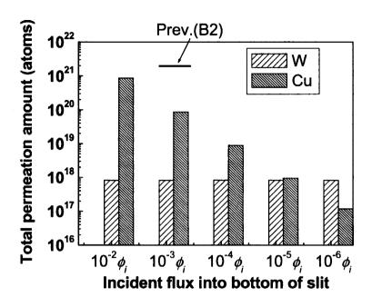
Fig. 7 Dependence of tritium permeation amount on the incident flux into the bottom of the slits (copper region) ranging from  $10^{-6}$  to 0.01 of the incident flux into the armor region ( $\phi_i$ ). Here, Prev. (B2) is the evaluation result with the previous data under the scenario B2.
