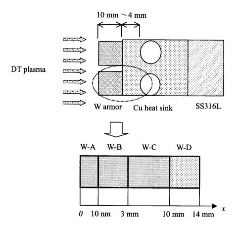
Fig. 2 Analytical geometry for the TMAP calculation of tritium permeation analysis.
