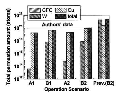
Fig. 6 Tritium permeation amount through the divertor under the various operation scenarios with the authors' data assuming incident flux to the copper region is 0.1% of the armor region.
