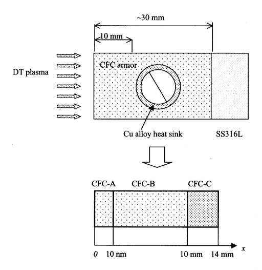
Fig. 2 Analytical geometry for the TMAP calculation of tritium permeation analysis.
