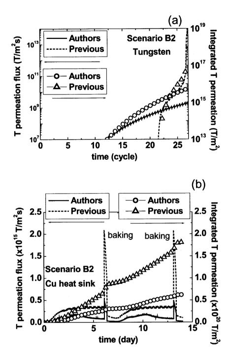
Fig. 5 Time evolution of tritium permeation rate and permeation amount per unit area through (a) tungsten armor region, (b) the copper heat sink region with the authors' data and previous data.
