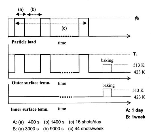
Fig. 4 Scenario of the heat load (temperature set value) and particle load into the divertor surface.
