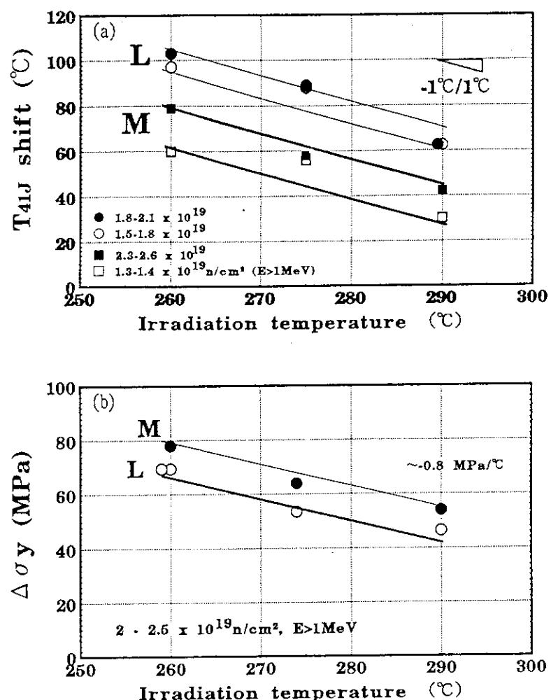
Fig. 5 Effects of irradiation temperature on (a) transition temperature shift and (b) yield stress increase, after irradiation to  $\sim 2 \times 10^{19} \text{n}/\text{cm}^2$  ( $\text{E}>1\text{MeV}$ ).
