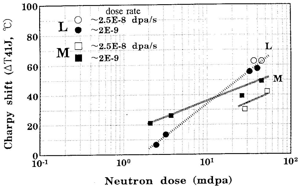
Fig. 3 Charpy shift ( $\Delta T_{41J}$ ) as a function of dose (dpa).
