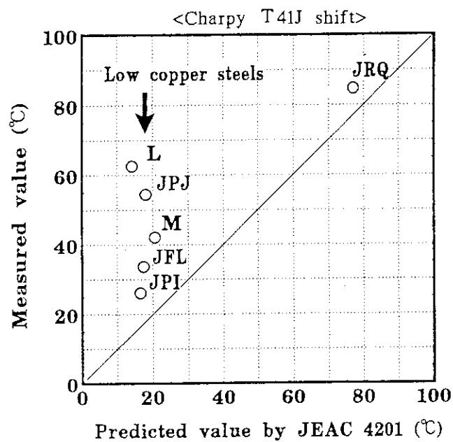
Fig. 7 Comparison of measured and predicted Charpy  $T_{41J}$  shift.
