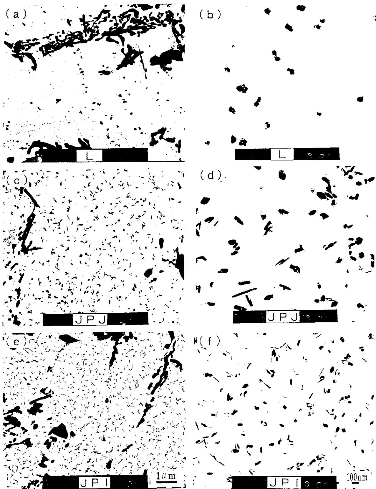
Fig.8 Carbide distribution for the alloy L (a,b), JPJ (c,d) and JPI (e,f) observed by TEM for carbon extraction replicas.
