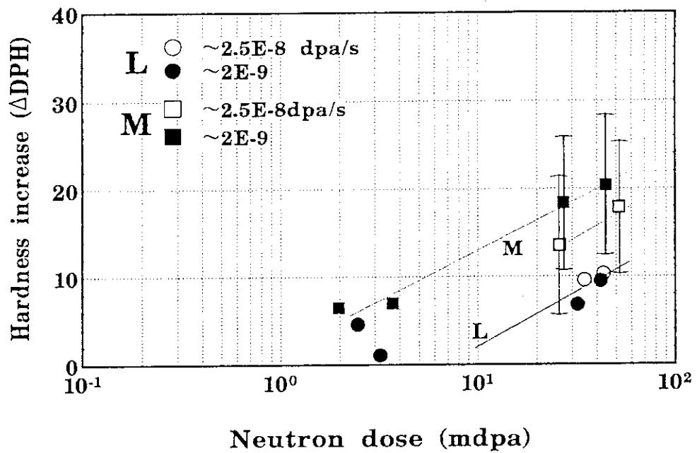
Fig. 4 Hardness increase ( $\Delta DPH$ ) as a function of dose (dpa).
