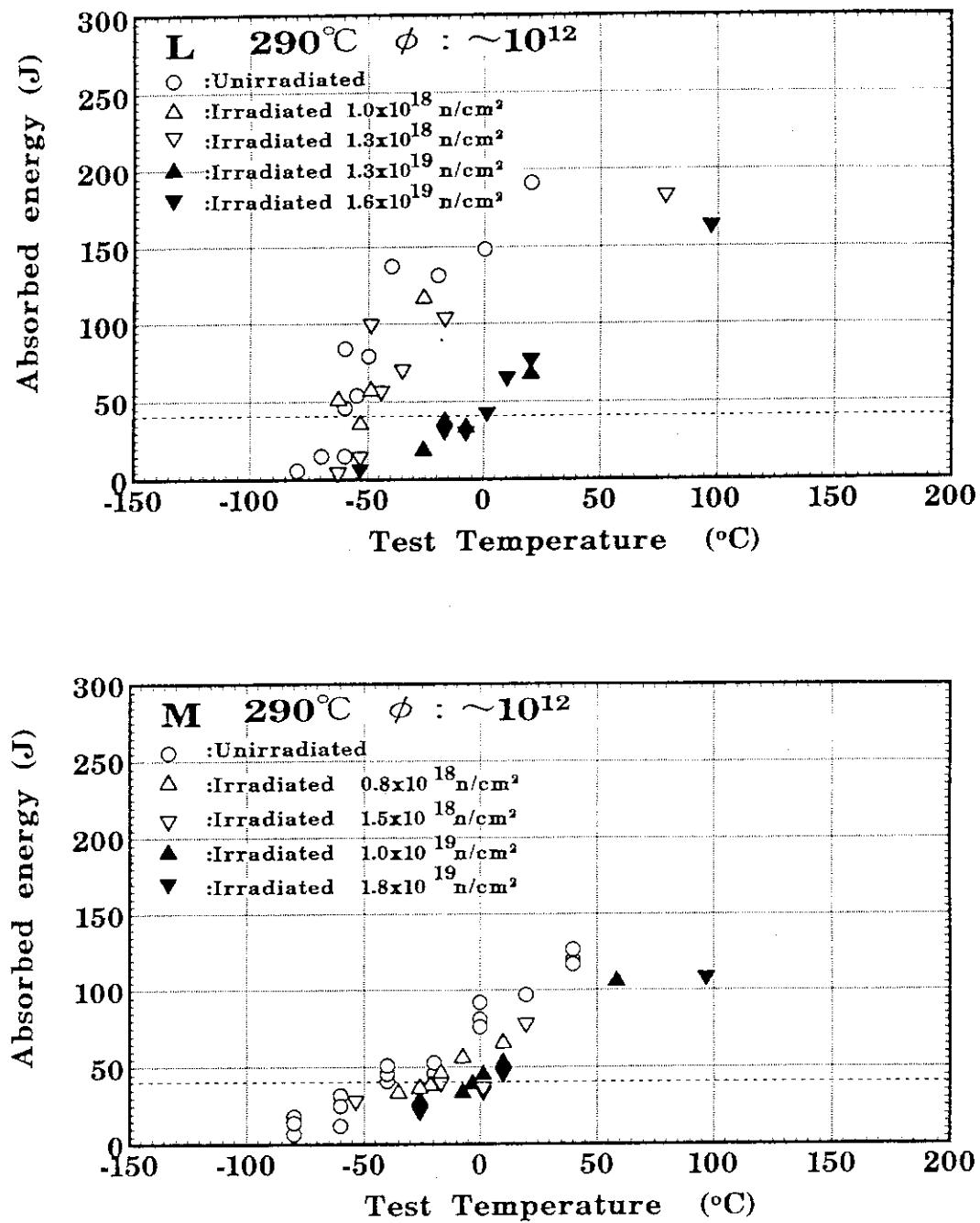
Fig. 2 Absorbed energy transition curves before and after irradiation to  $1 \times 10^{18}$  and  $2 \times 10^{19}$   $\text{n/cm}^2$  ( $E > 1\text{MeV}$ ) at  $290^{\circ}\text{C}$  for the alloys L and M.
