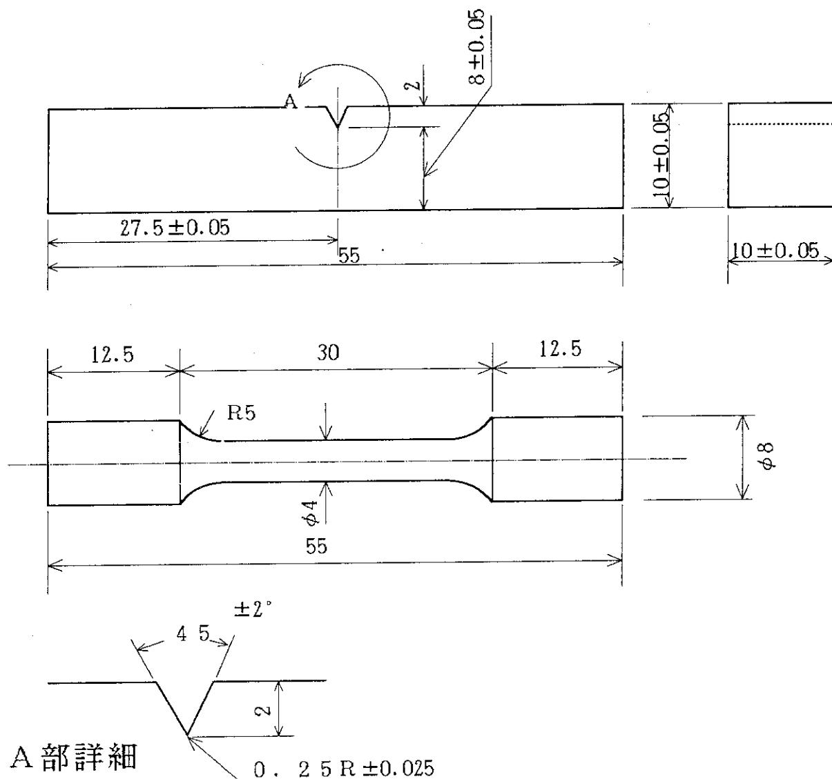
Fig. A-1 Configurations of Charpy and tensile test specimens
