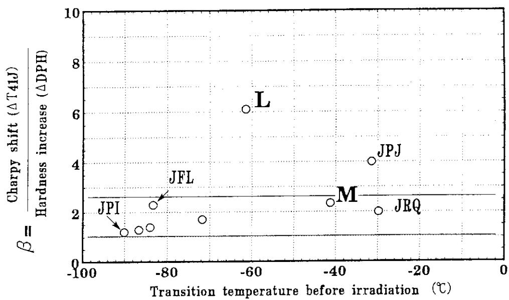
Fig. 6 Ratio of  $\Delta T_{41J}/\Delta DPH$  (=  $\beta$ ) for the alloys L, M and the IAEA heavy section steels.
