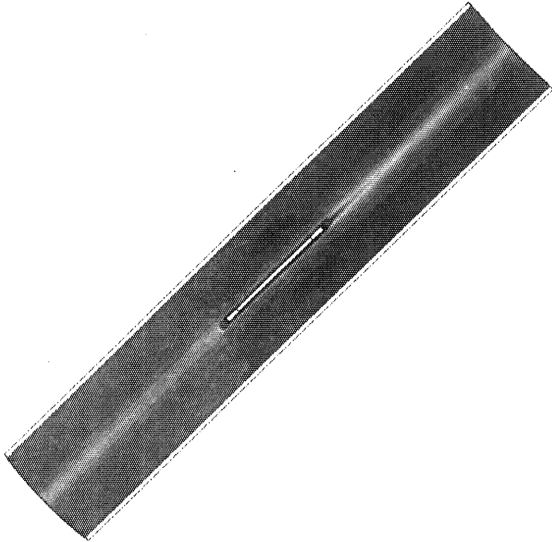
Fig. A1 Color filled axial velocity distribution at the center plane between the inner and outer walls
