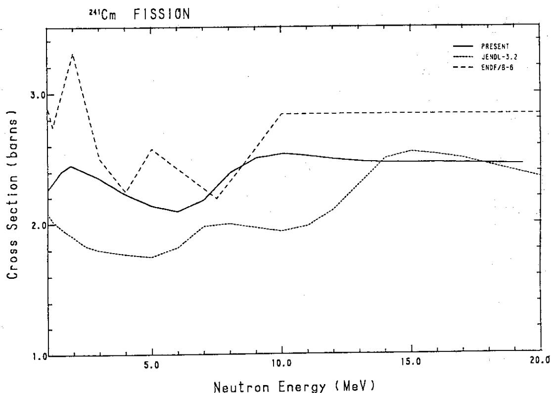
Fig. 254 Comparison of the fission cross-section for  $^{241}\text{Cm}$ .
