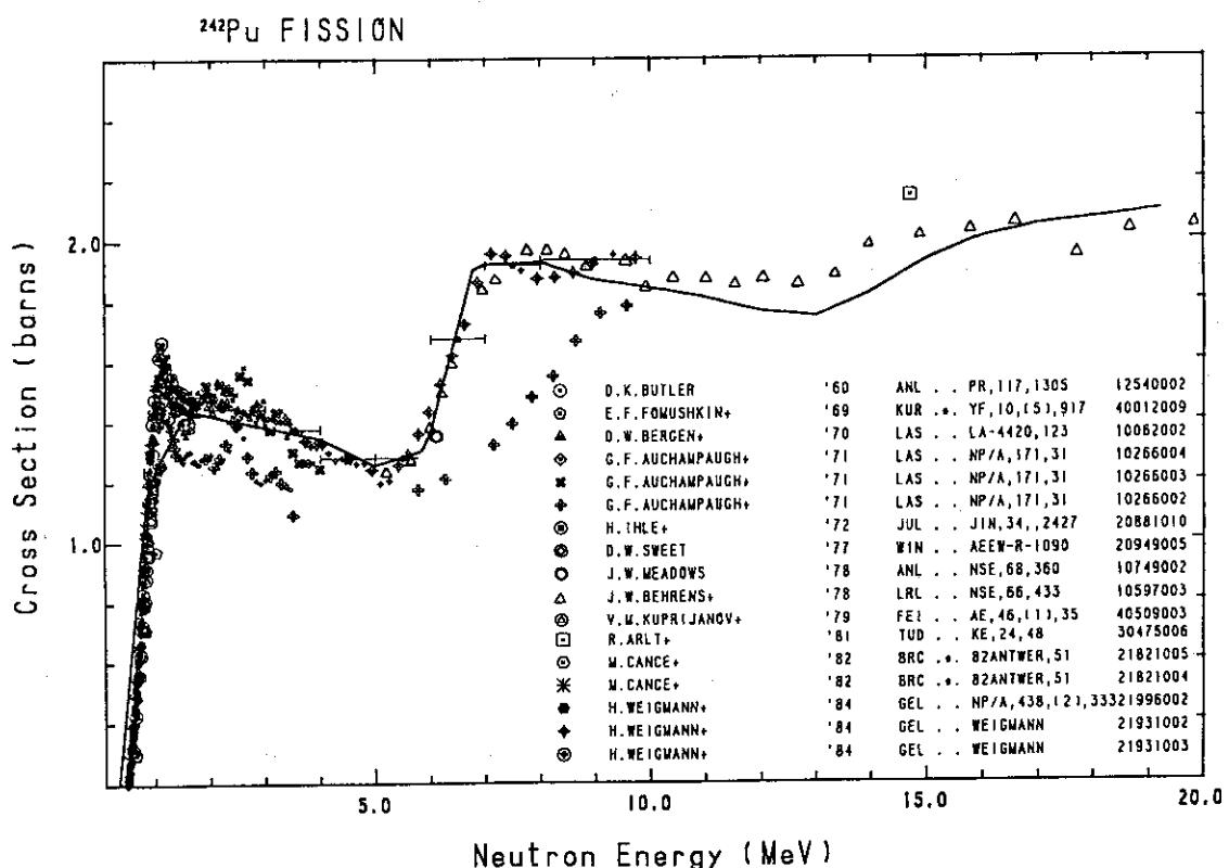
Fig. 106 The fission cross-section of  $^{242}\text{Pu}$ .
