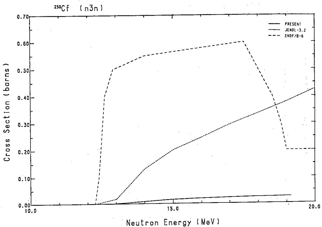
Fig. 274 Comparison of the ( $n,3n$ )-cross-section for  $^{250}\text{Cf}$ .
