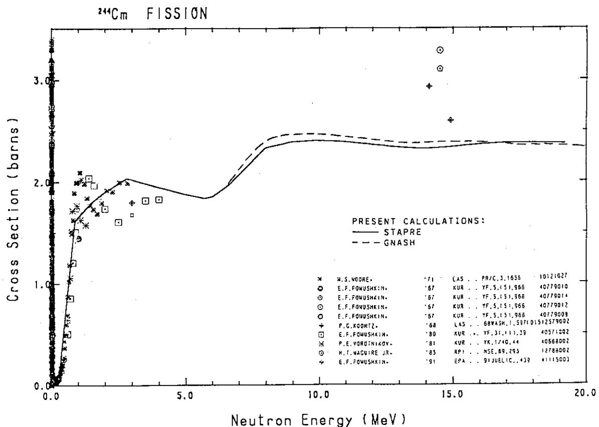
Fig. 163 The fission cross-section of  $^{244}\text{Cm}$ .
