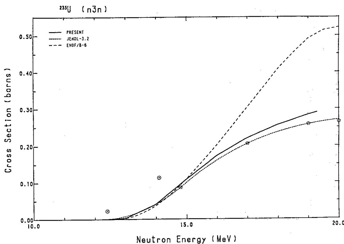
Fig. 223 Comparison of the ( $n,3n$ )-cross-section for  $^{235}\text{U}$ .
