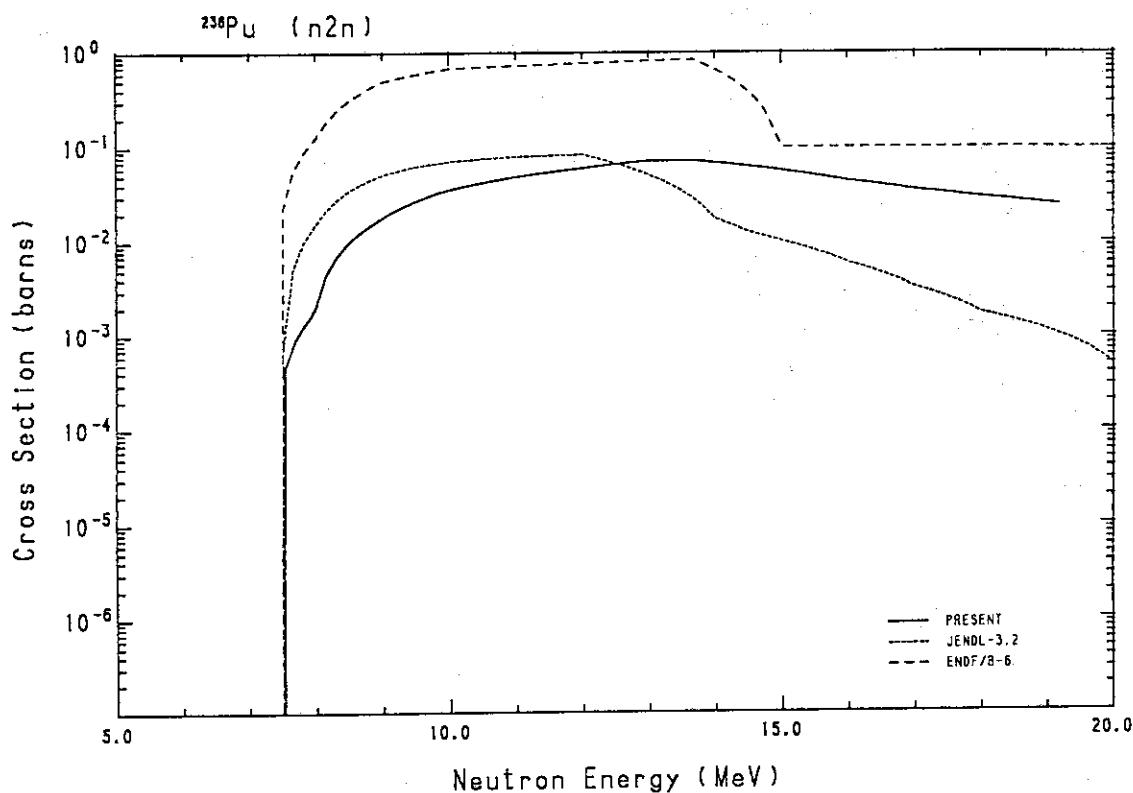
Fig. 238 Comparison of the ( $n,2n$ )-cross-section for  $^{236}\text{Pu}$ .
