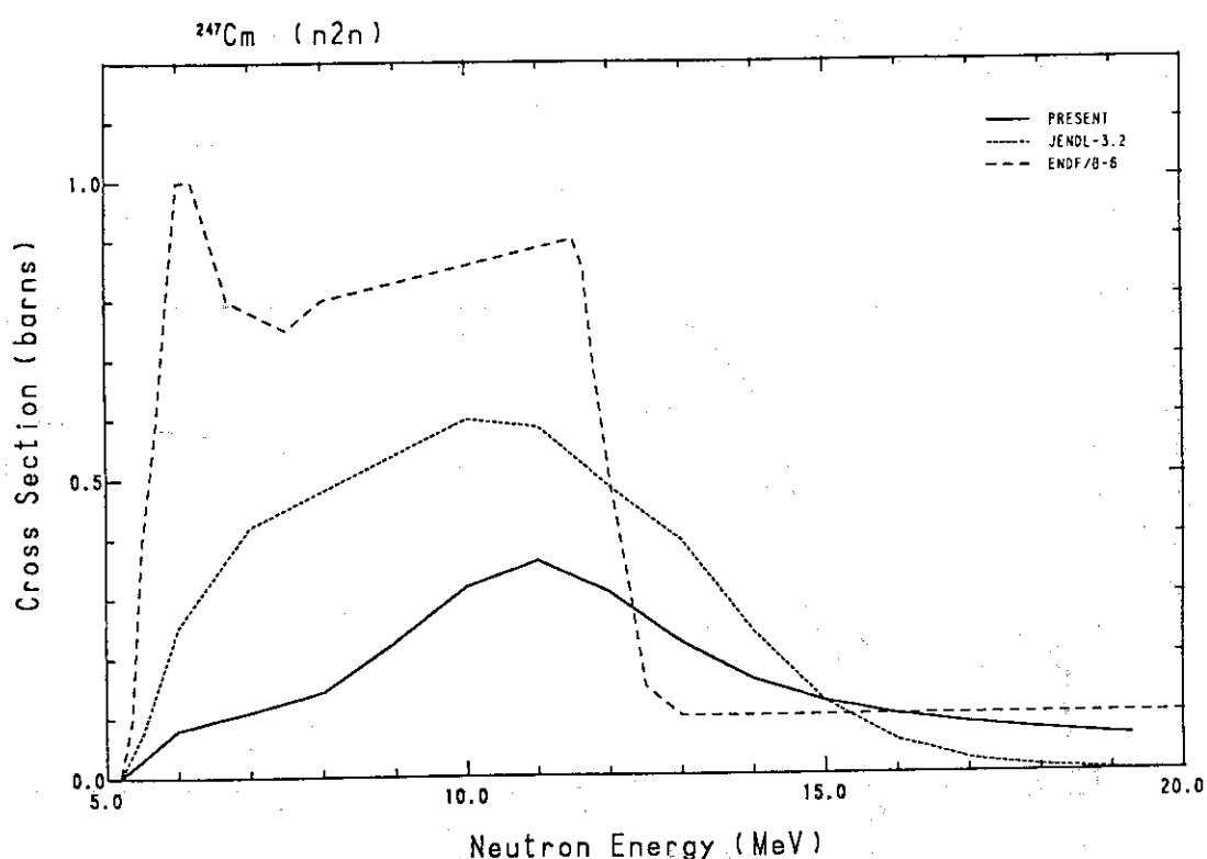
Fig. 267 Comparison of the  $(\text{n},2\text{n})$ -cross-section for  $^{247}\text{Cm}$ .
