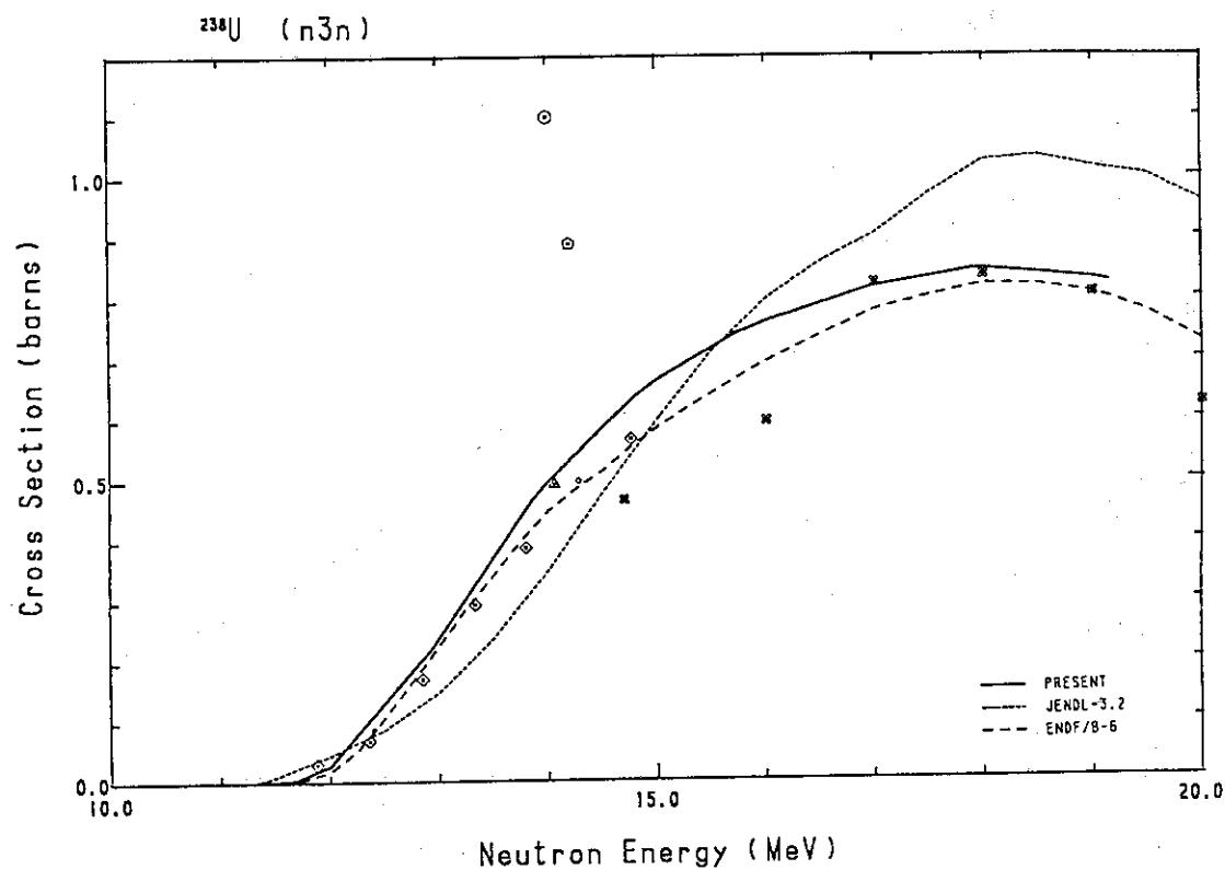
Fig. 226 Comparison of the ( $n,3n$ )-cross-section for  $^{238}\text{U}$ .
