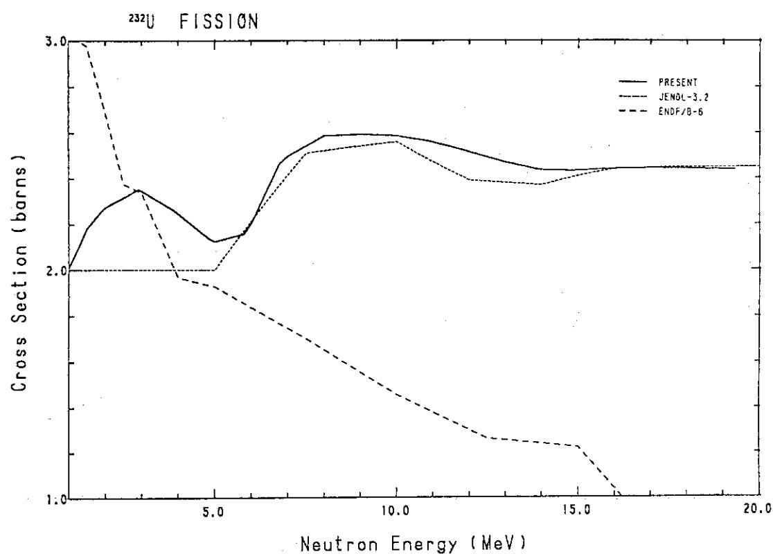
Fig. 216 Comparison of the fission cross-section for  $^{232}\text{U}$ .
