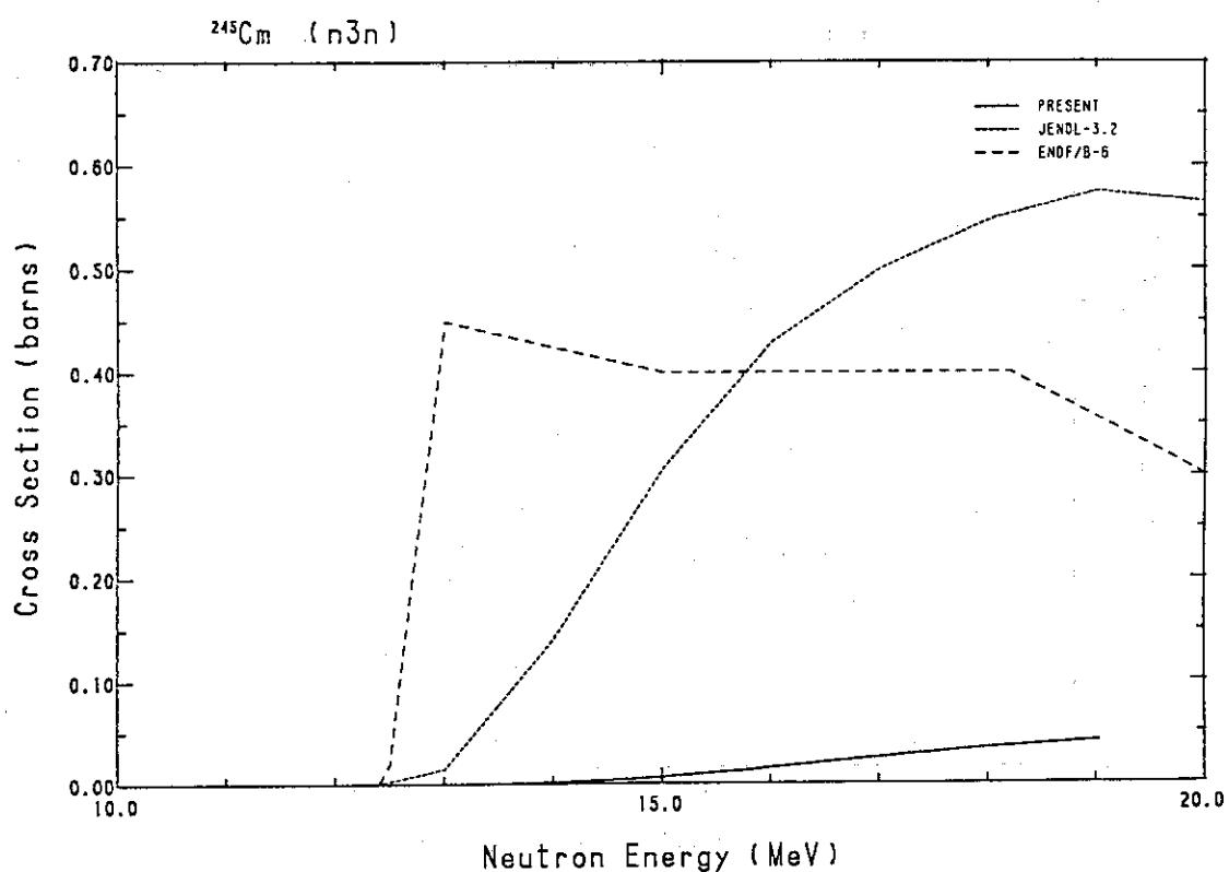
Fig. 262 Comparison of the ( $n,3n$ )-cross-section for  $^{245}\text{Cm}$ .
