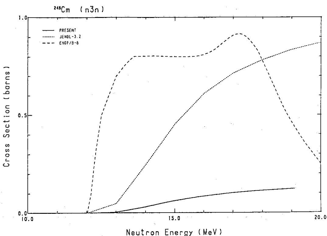
Fig. 265 Comparison of the ( $n,3n$ )-cross-section for  $^{246}\text{Cm}$ .
