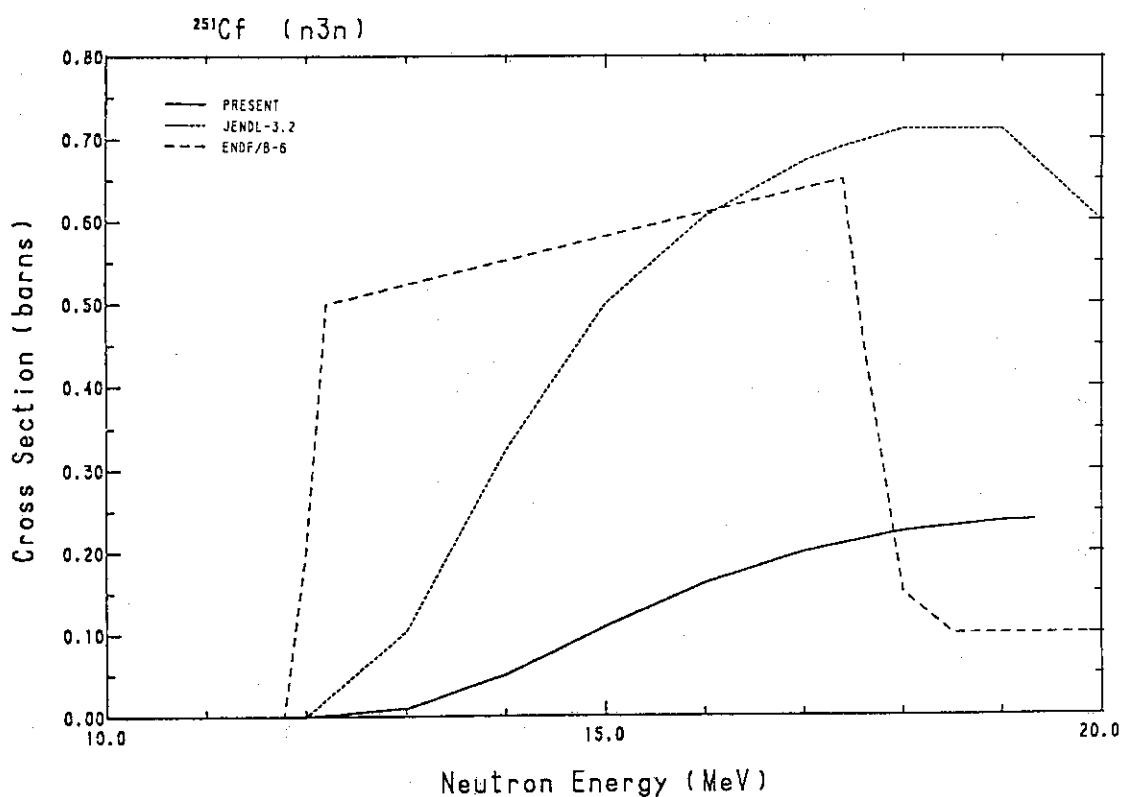
Fig. 277 Comparison of the  $(n,3n)$ -cross-section for  $^{251}\text{Cf}$ .
