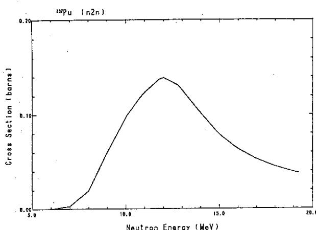
Fig. 92 The  $(n,2n)$ -reaction cross-section of  $^{237}\text{Pu}$ .
