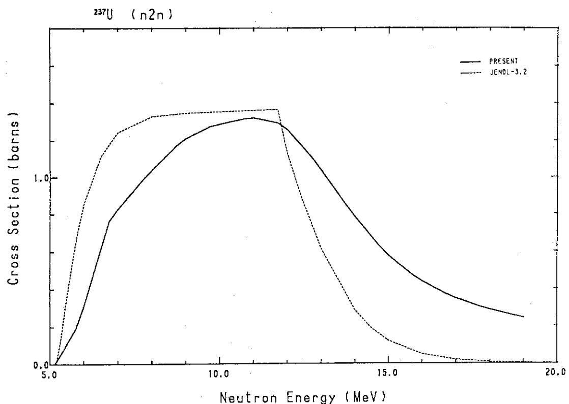
Fig. 224 Comparison of the ( $n,2n$ )-cross-section for  $^{237}\text{U}$ .
