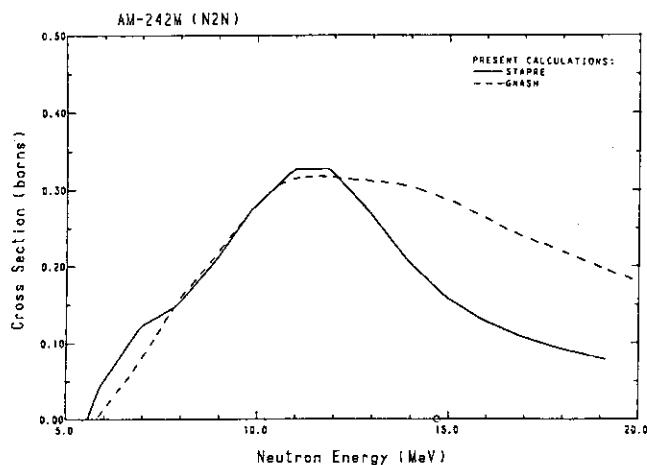
Fig. 134 The (n,2n)-reaction cross-section of  $^{242}\text{Am}$ .
