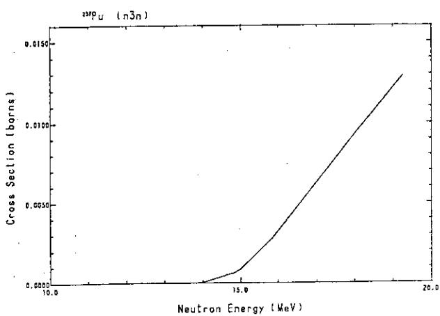
Fig. 93 The  $(n,3n)$ -reaction cross-section of  $^{237}\text{Pu}$ .
