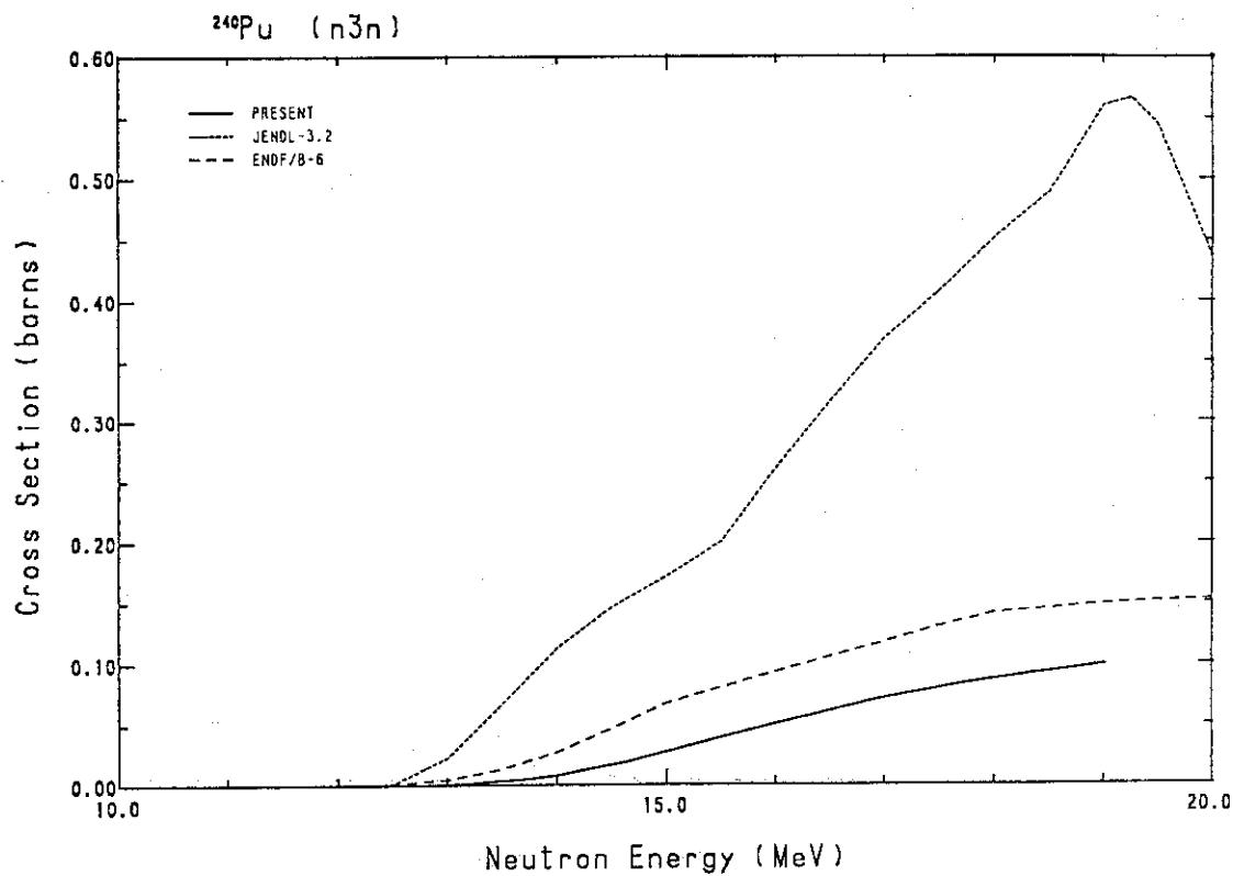
Fig. 244 Comparison of the (n,3n)-cross-section for  $^{240}\text{Pu}$ .
