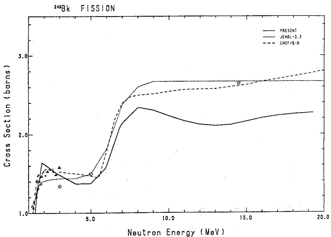
Fig. 269 Comparison of the fission cross-section for  $^{249}\text{Bk}$ .
