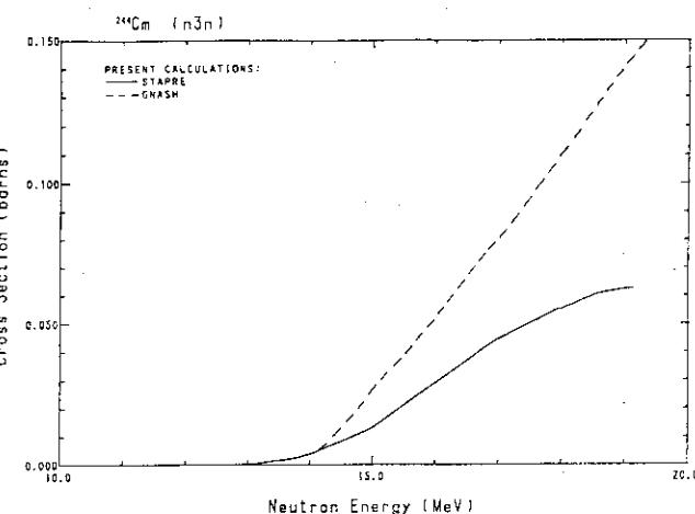
Fig. 165 The ( $n,3n$ )-reaction cross-section of  $^{244}\text{Cm}$ .
