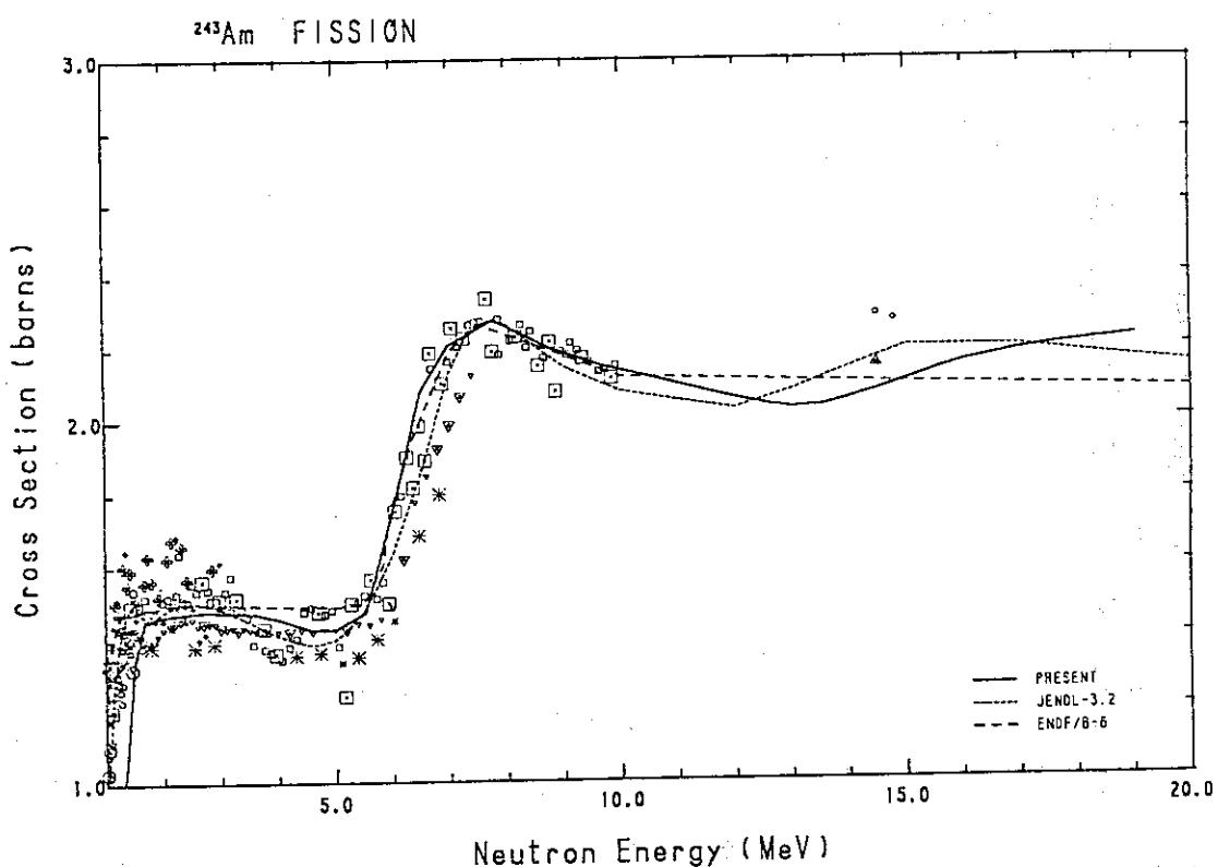
Fig. 251 Comparison of the fission cross-section for  $^{243}\text{Am}$ .
