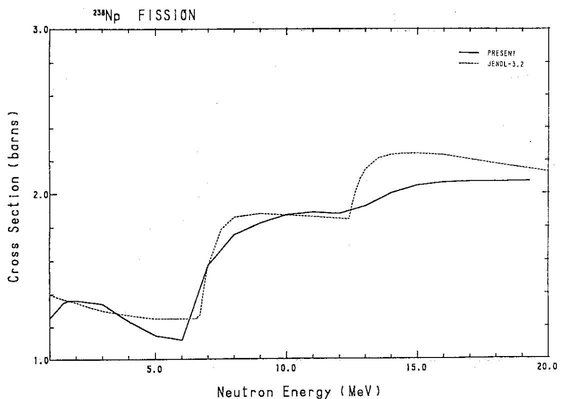
Fig. 233 Comparison of the fission cross-section for  $^{238}\text{Np}$ .
