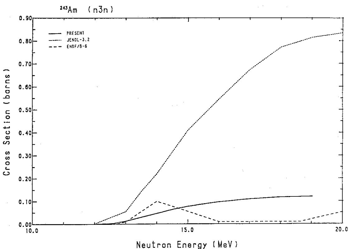
Fig. 253 Comparison of the ( $n,3n$ )-cross-section for  $^{243}\text{Am}$ .
