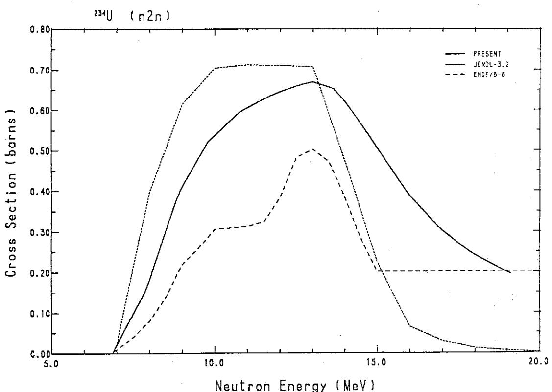
Fig. 221 Comparison of the ( $n,2n$ )-cross-section for  $^{234}\text{U}$ .
