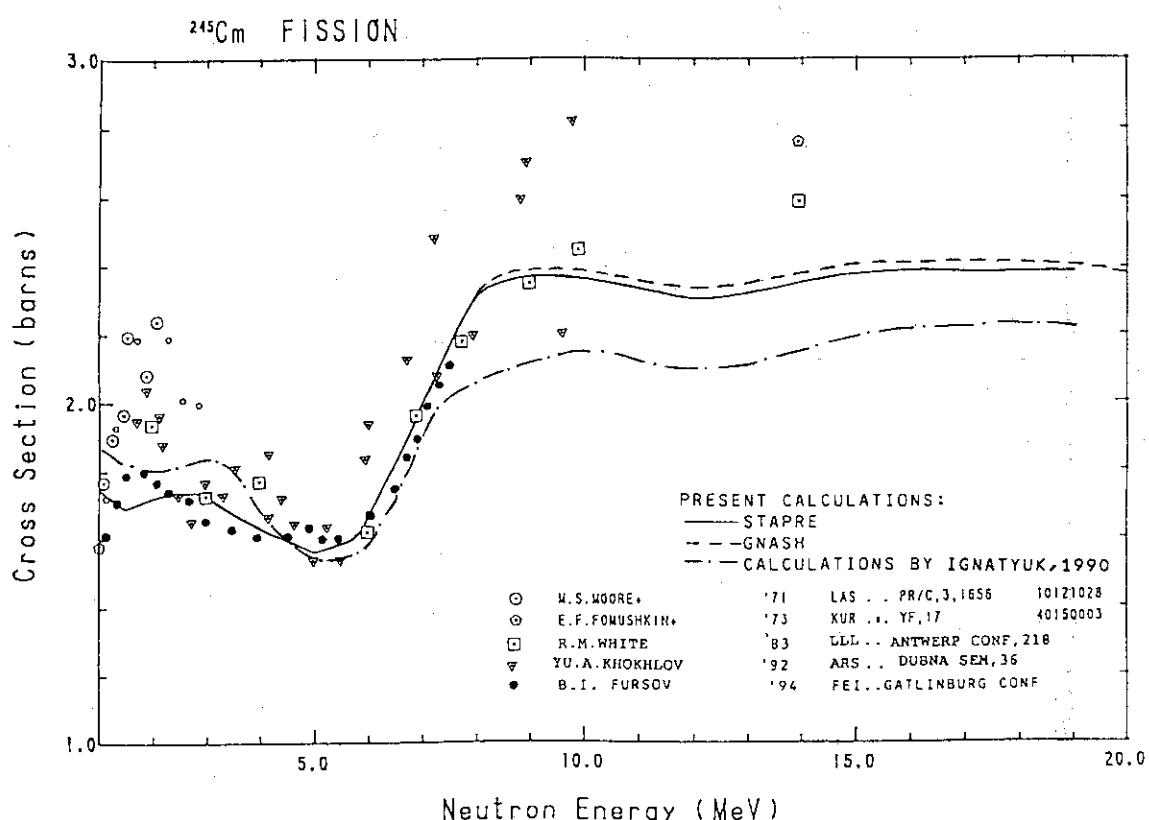
Fig. 166 The fission cross-section of  $^{245}\text{Cm}$ .
