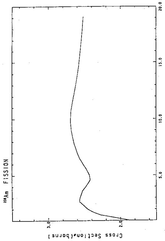
Fig. 124 The fission cross-section of  $^{239}\text{Am}$ .
