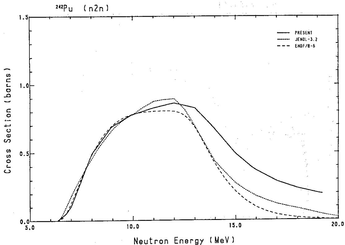
Fig. 246 Comparison of the ( $n,2n$ )-cross-section for  $^{242}\text{Pu}$ .
