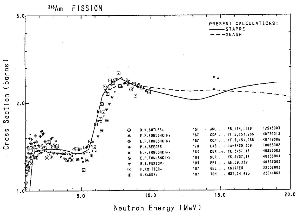
Fig. 136 The fission cross-section of  $^{243}\text{Am}$ .
