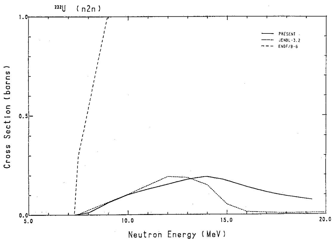
Fig. 217 Comparison of the ( $n,2n$ )-cross-section for  $^{232}\text{U}$ .
