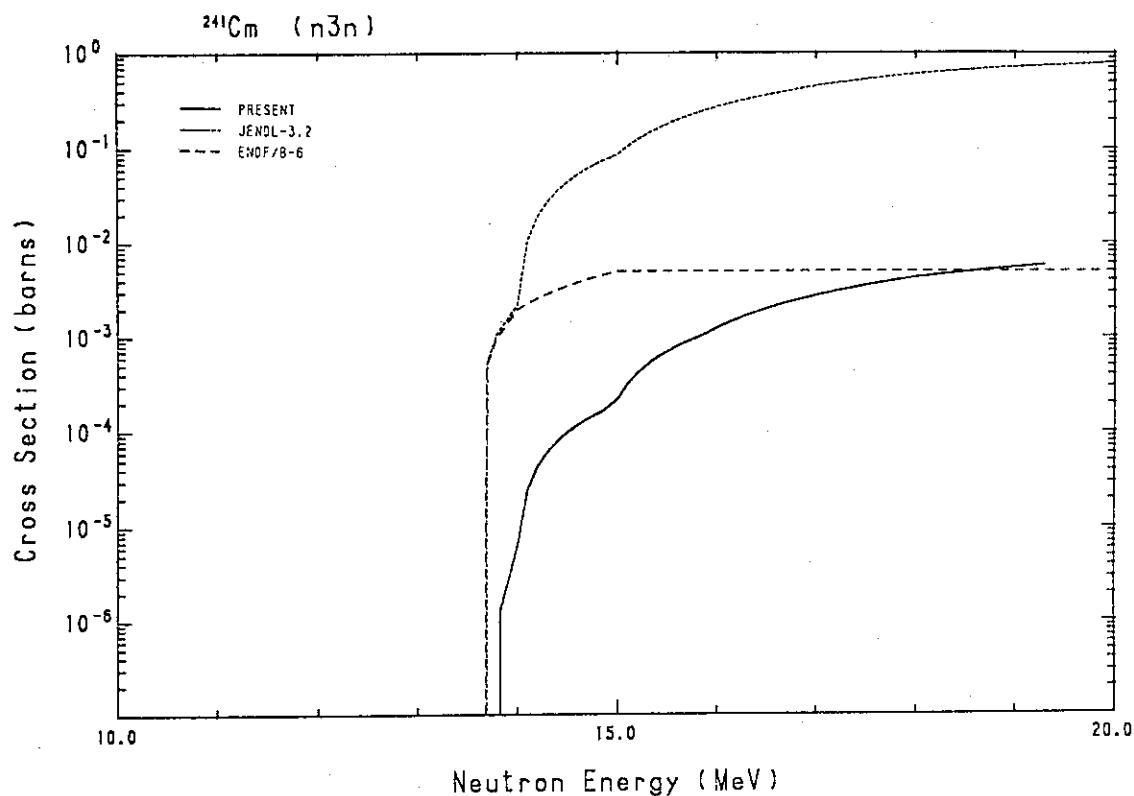
Fig. 256 Comparison of the ( $n,3n$ )-cross-section for  $^{241}\text{Cm}$ .
