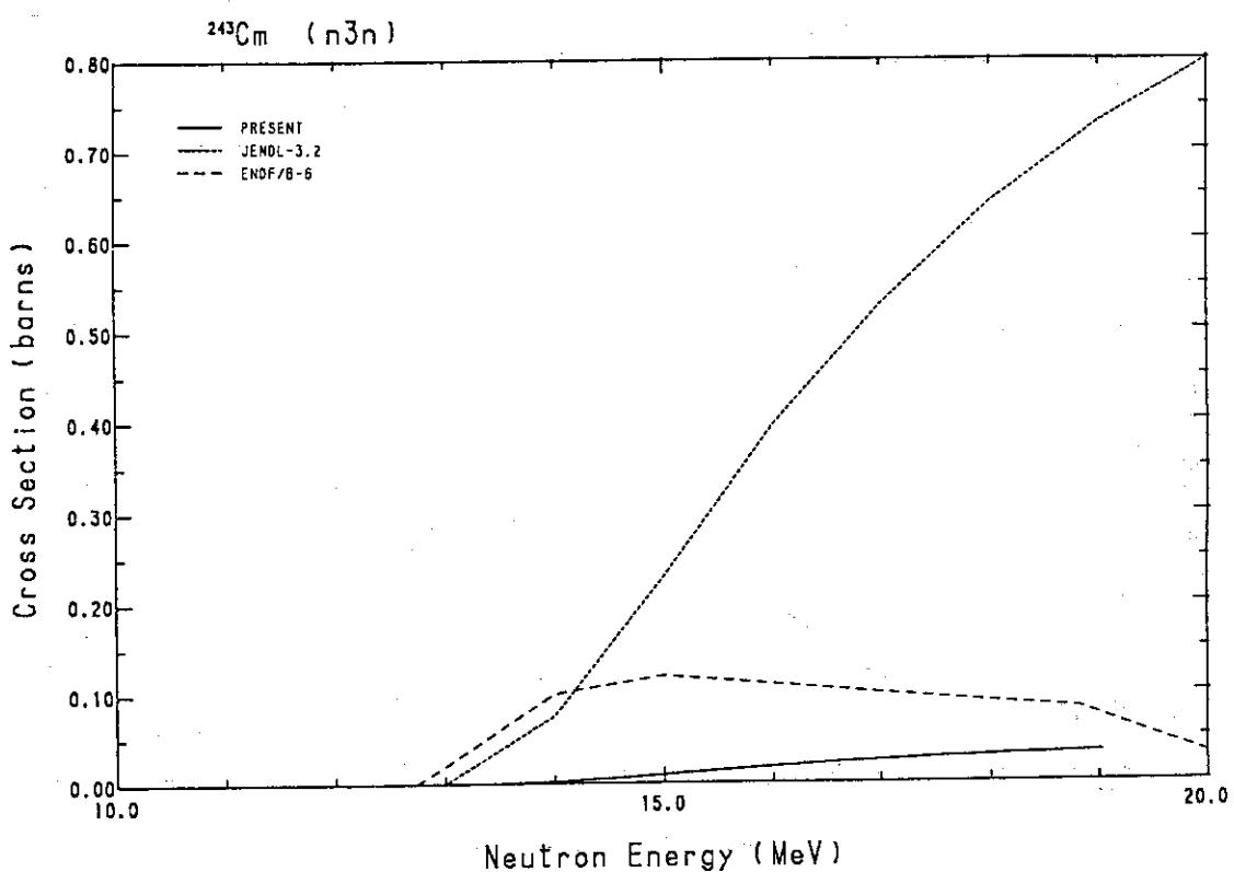
Fig. 259 Comparison of the ( $n,3n$ )-cross-section for  $^{243}\text{Cm}$ .
