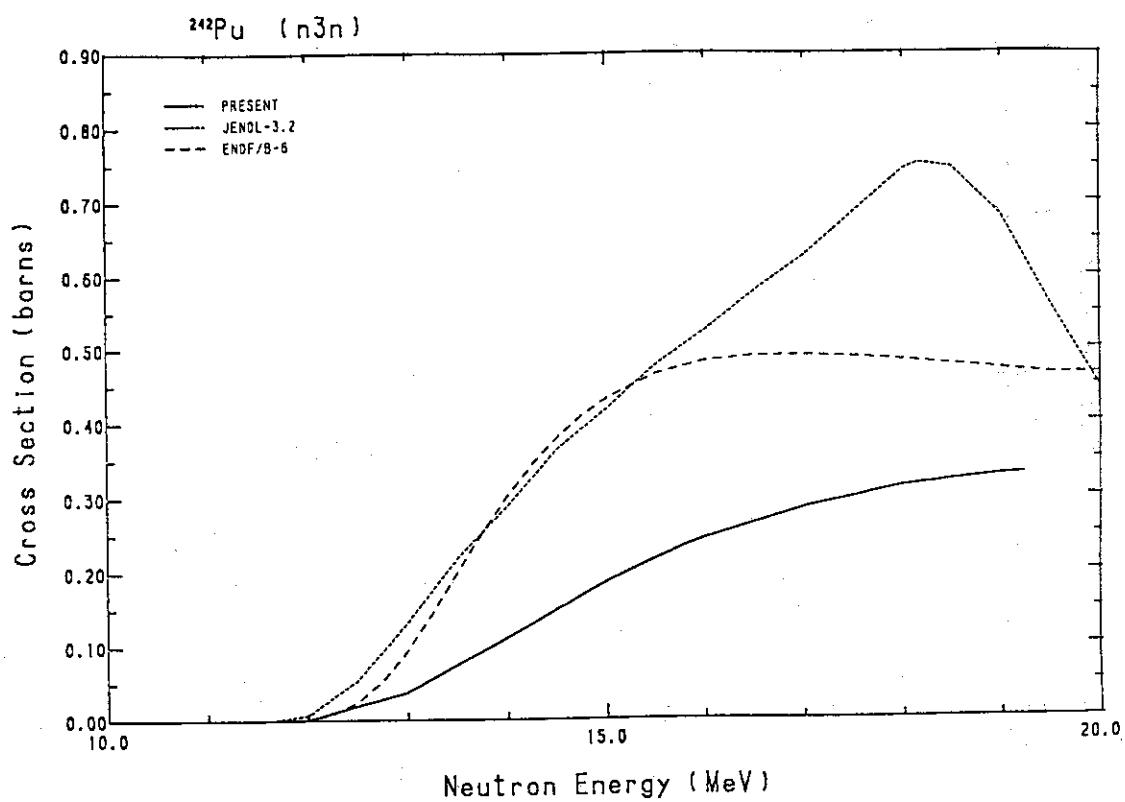
Fig. 247 Comparison of the ( $n,3n$ )-cross-section for  $^{242}\text{Pu}$ .
