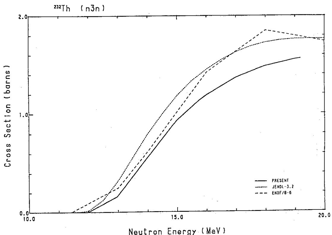
Fig. 215 Comparison of the ( $n,3n$ )-cross-section for  $^{232}\text{Th}$ .
