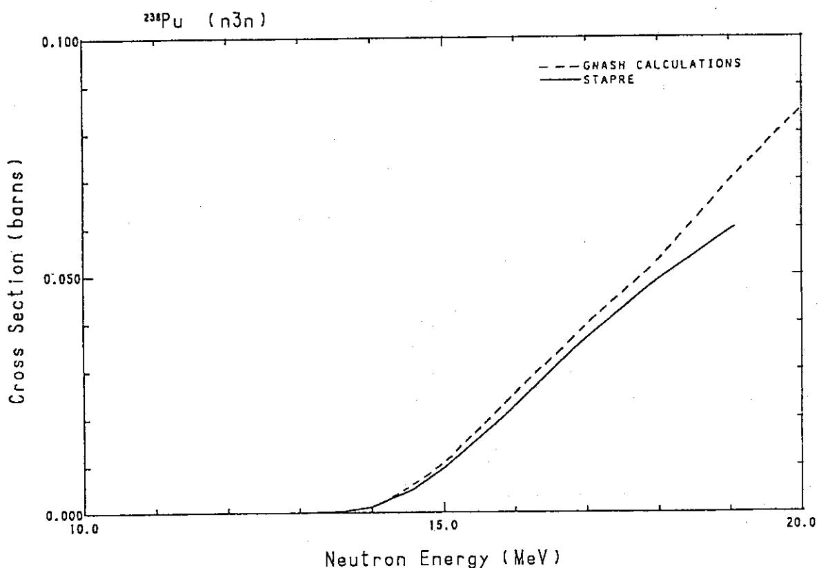
Fig. 96 The ( $n,3n$ )-reaction cross-section of  $^{238}\text{Pu}$ .
