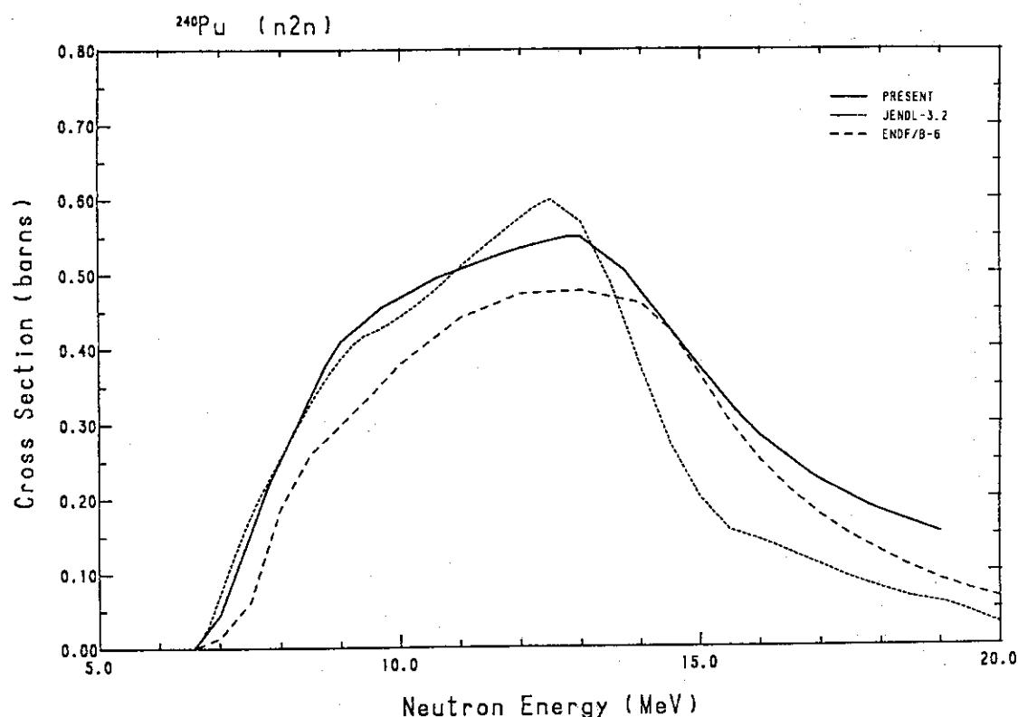
Fig. 243 Comparison of the ( $n,2n$ )-cross-section for  $^{240}\text{Pu}$ .
