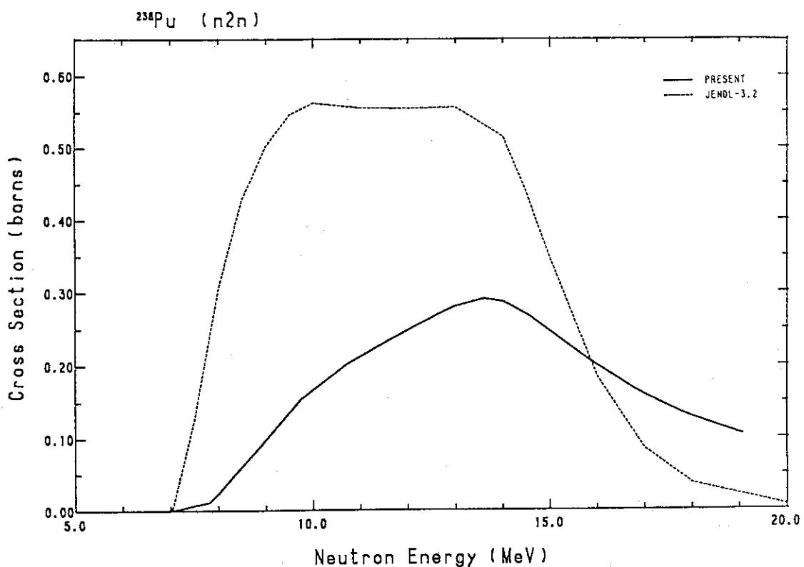
Fig. 241 Comparison of the ( $n,2n$ )-cross-section for  $^{238}\text{Pu}$ .
