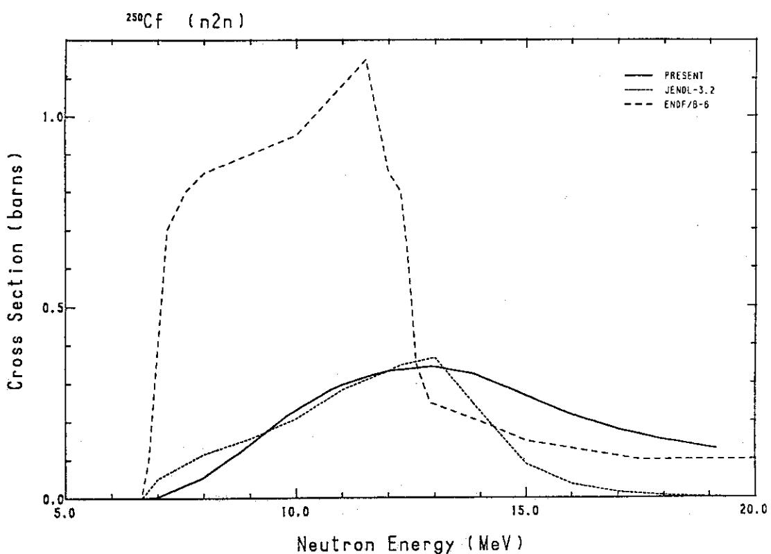
Fig. 273 Comparison of the ( $n,2n$ )-cross-section for  $^{250}\text{Cf}$ .
