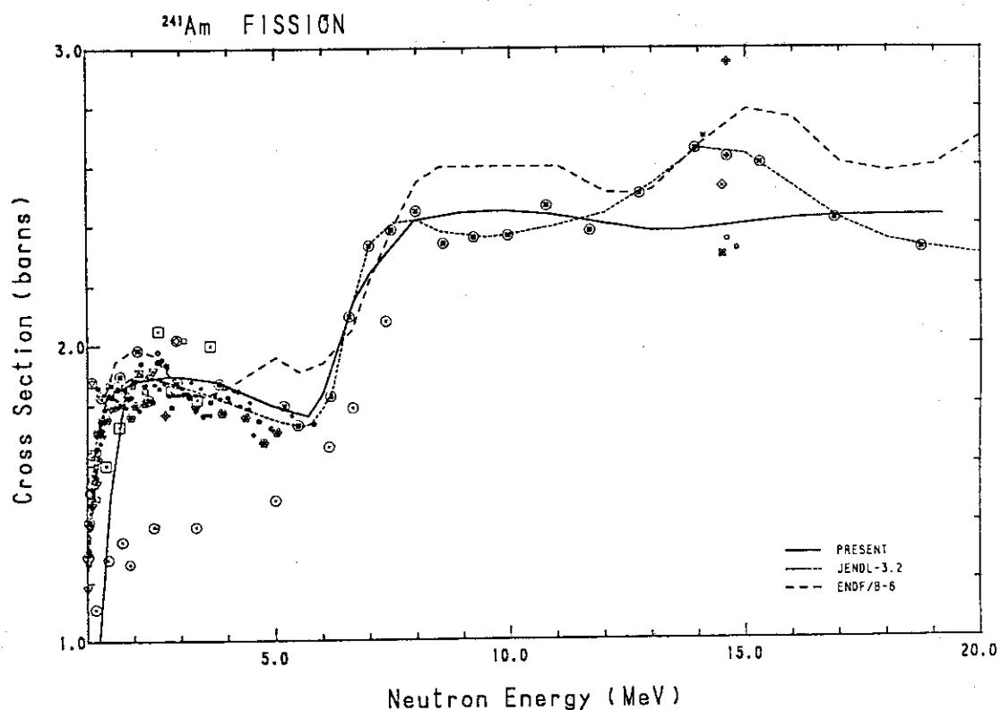
Fig. 248 Comparison of the fission cross-section for  $^{241}\text{Am}$ .
