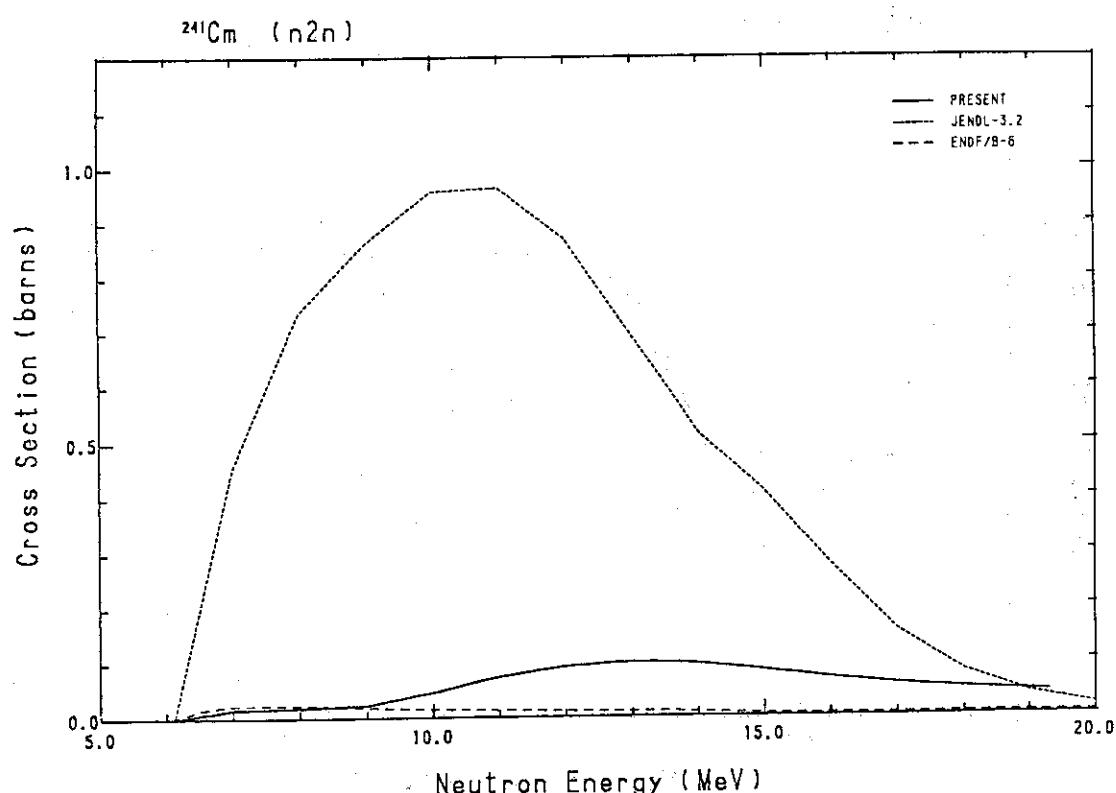
Fig. 255 Comparison of the ( $n,2n$ )-cross-section for  $^{241}\text{Cm}$ .
