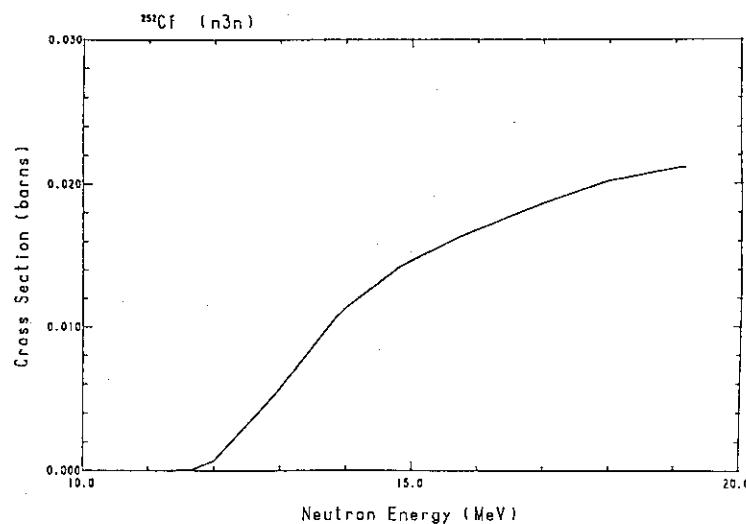
Fig. 213 The (n,3n)-reaction cross-section of <sup>252</sup>Cf.
