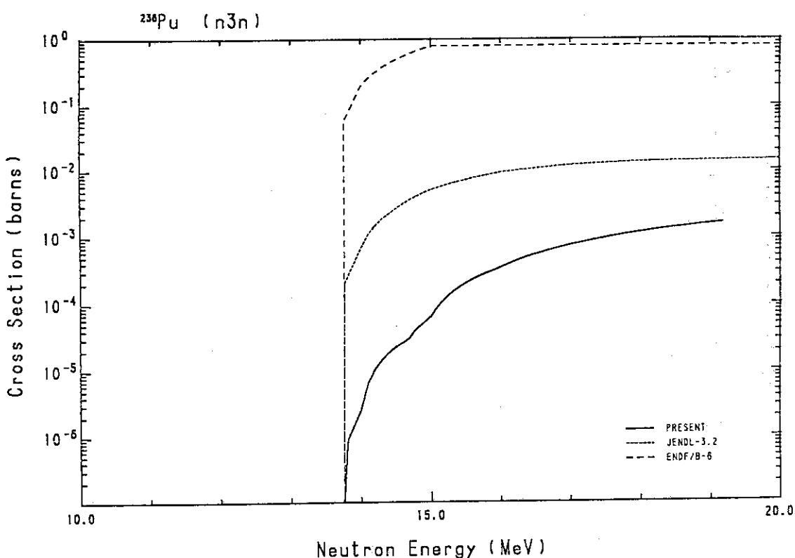
Fig. 239 Comparison of the ( $n,3n$ )-cross-section for  $^{236}\text{Pu}$ .
