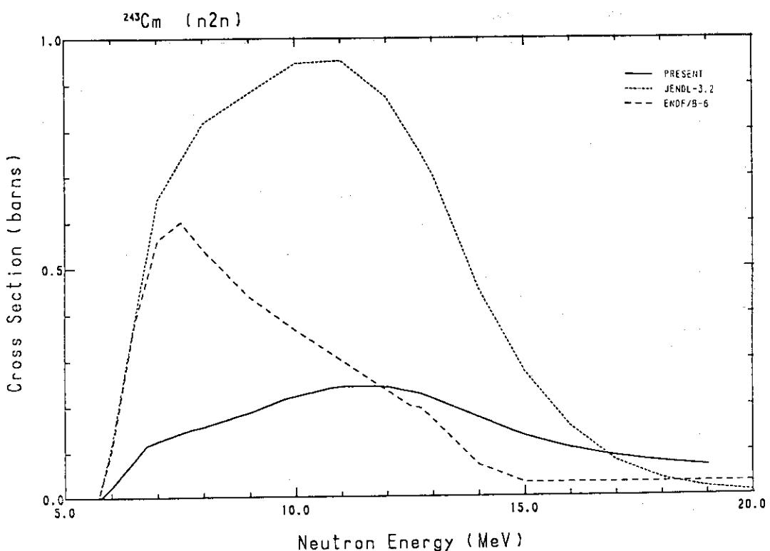
Fig. 258 Comparison of the ( $n,2n$ )-cross-section for  $^{243}\text{Cm}$ .
