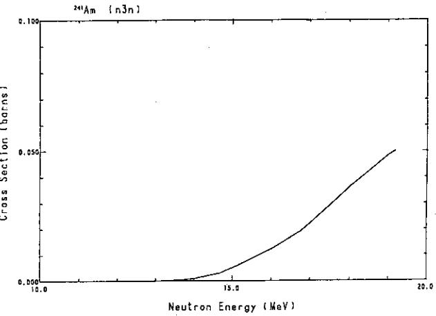
Fig. 132 The  $(n,3n)$ -reaction cross-section of  $^{241}\text{Am}$ .
