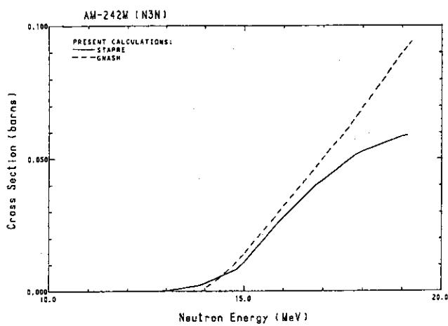
Fig. 135 The (n,3n)-reaction cross-section of  $^{242}\text{Am}$ .
