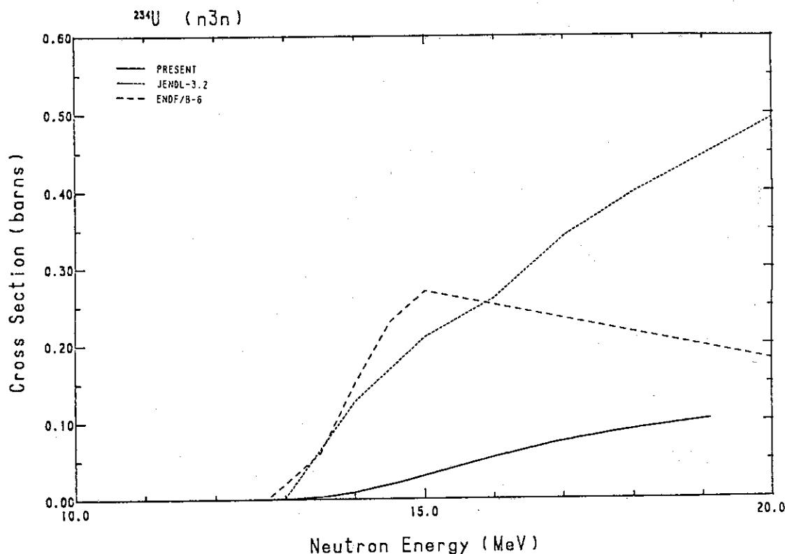
Fig. 222 Comparison of the ( $n,3n$ )-cross-section for  $^{234}\text{U}$ .
