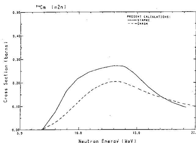
Fig. 164 The ( $n,2n$ )-reaction cross-section of  $^{244}\text{Cm}$ .
