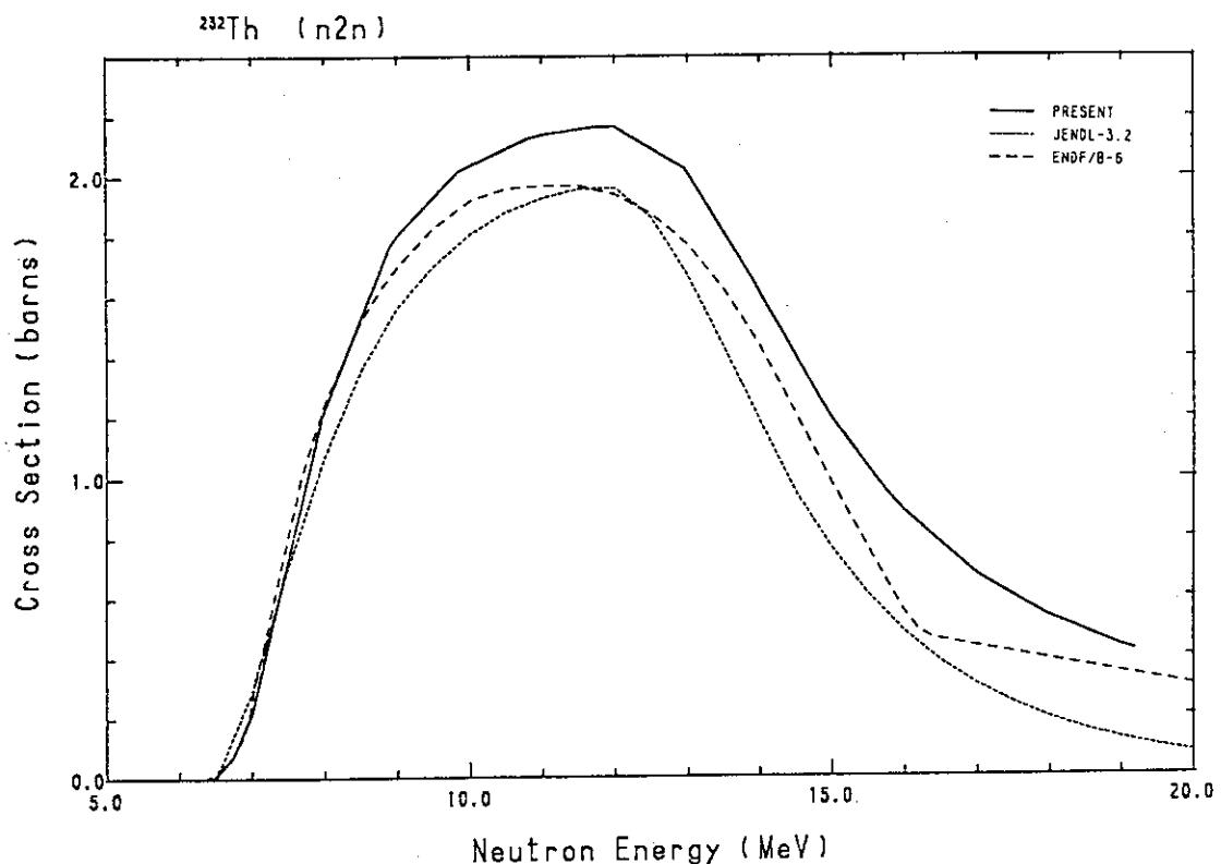
Fig. 214 Comparison of the ( $n,2n$ )-cross-section for  $^{232}\text{Th}$ .
