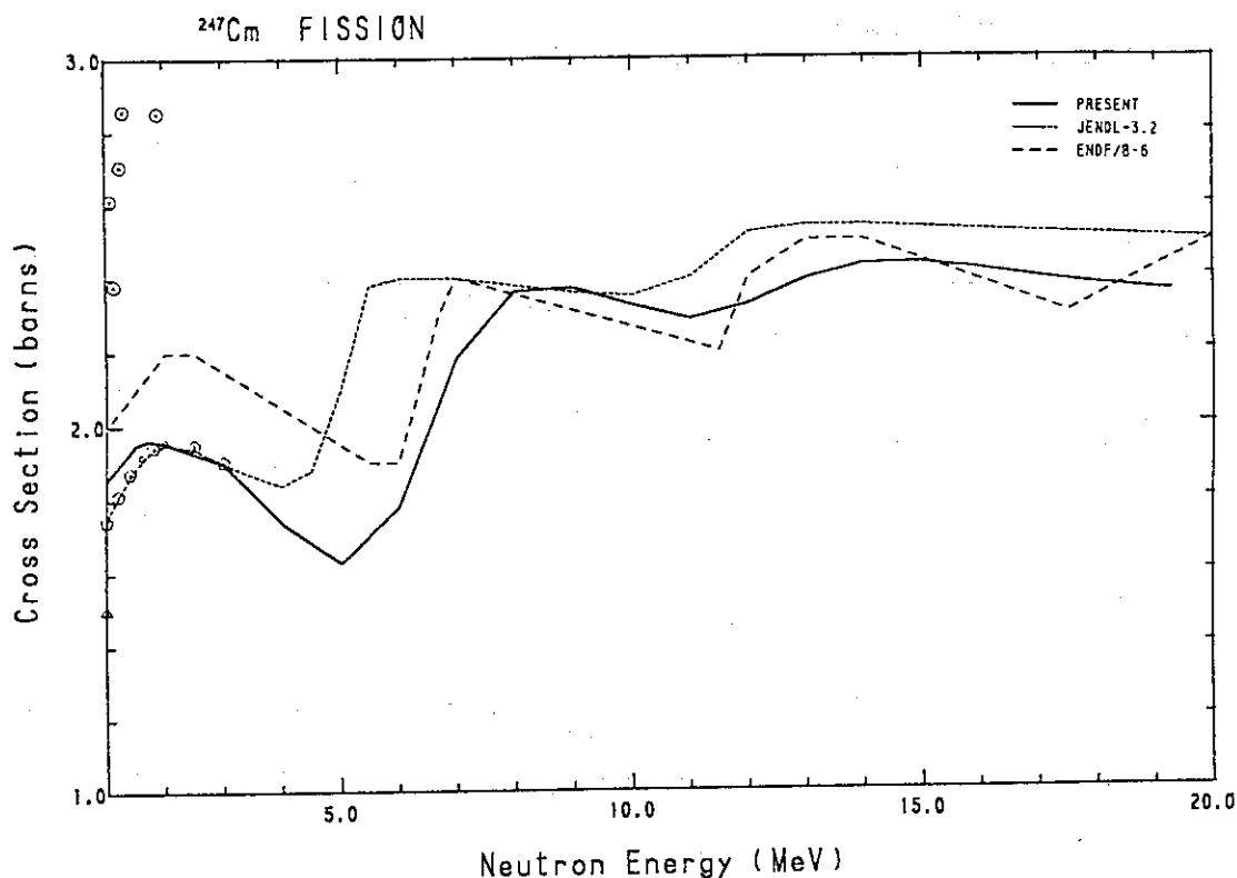
Fig. 266 Comparison of the fission cross-section for  $^{247}\text{Cm}$ .
