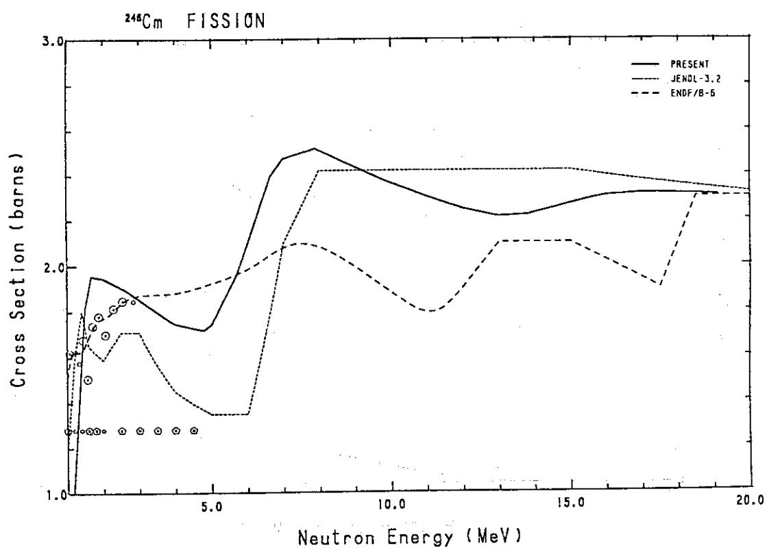
Fig. 263 Comparison of the fission cross-section for  $^{246}\text{Cm}$ .
