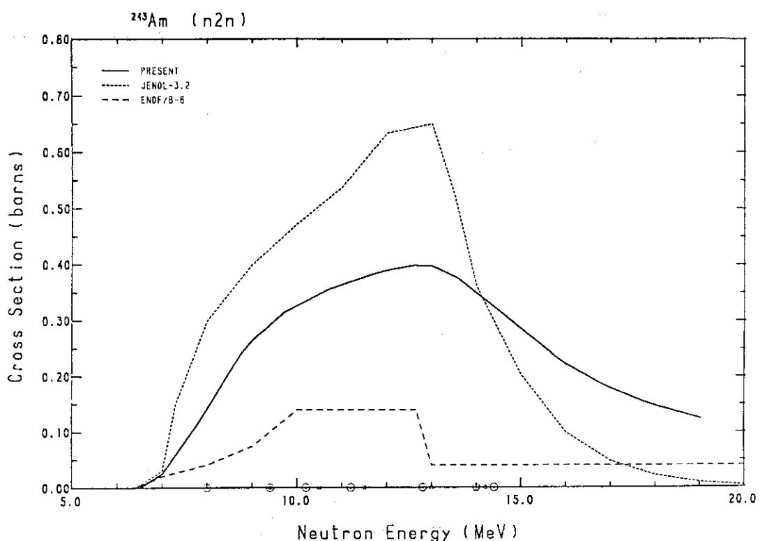
Fig. 252 Comparison of the ( $n,2n$ )-cross-section for  $^{243}\text{Am}$ .
