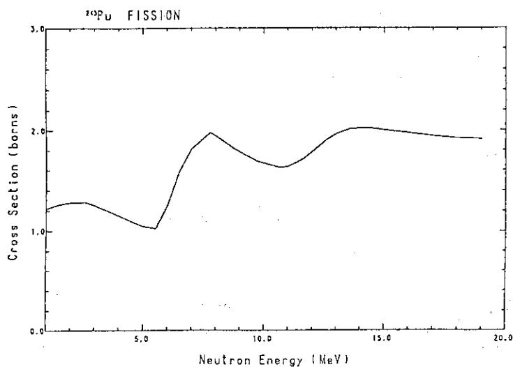
Fig. 109 The fission cross-section of  $^{248}\text{Pu}$ .
