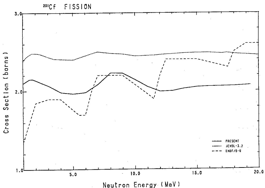
Fig. 275 Comparison of the fission cross-section for  $^{251}\text{Cf}$ .
