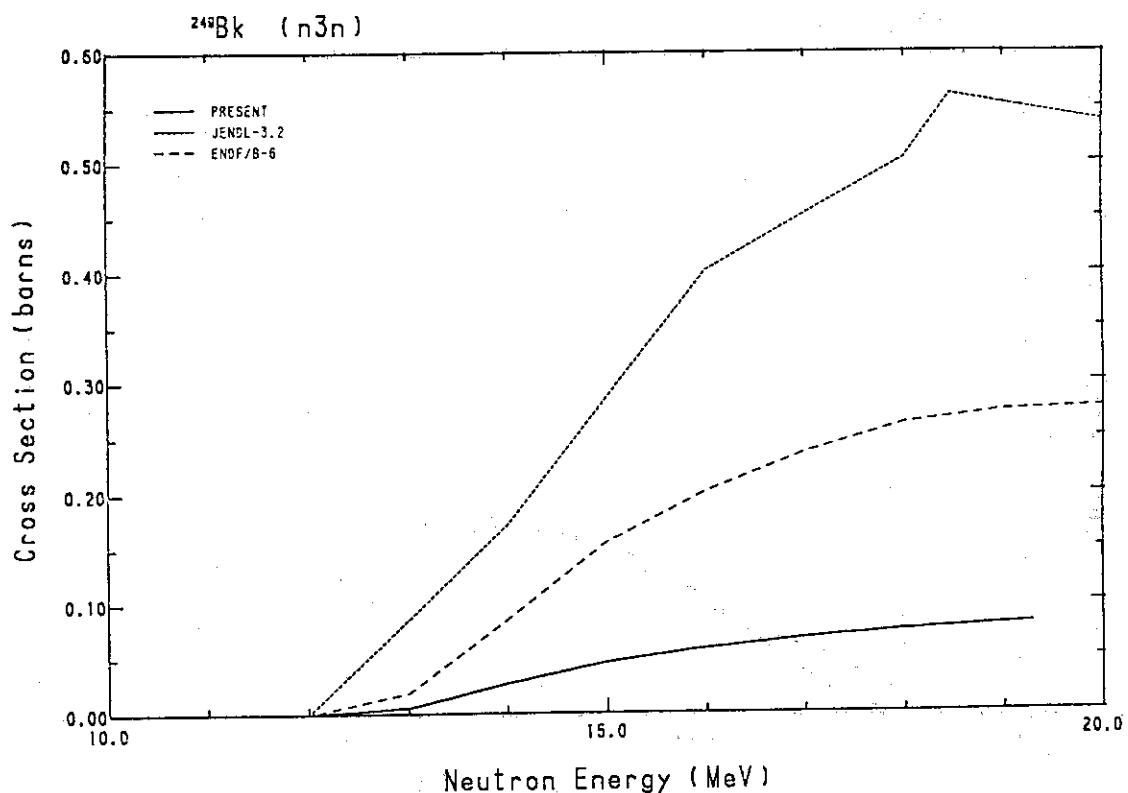
Fig. 271 Comparison of the  $(n,3n)$ -cross-section for  $^{249}\text{Bk}$ .
