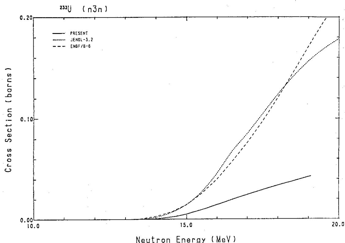
Fig. 220 Comparison of the ( $n,3n$ )-cross-section for  $^{233}\text{U}$ .
