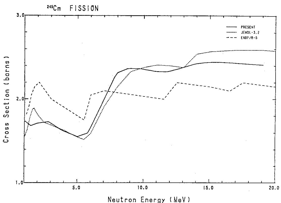
Fig. 260 Comparison of the fission cross-section for  $^{245}\text{Cm}$ .
