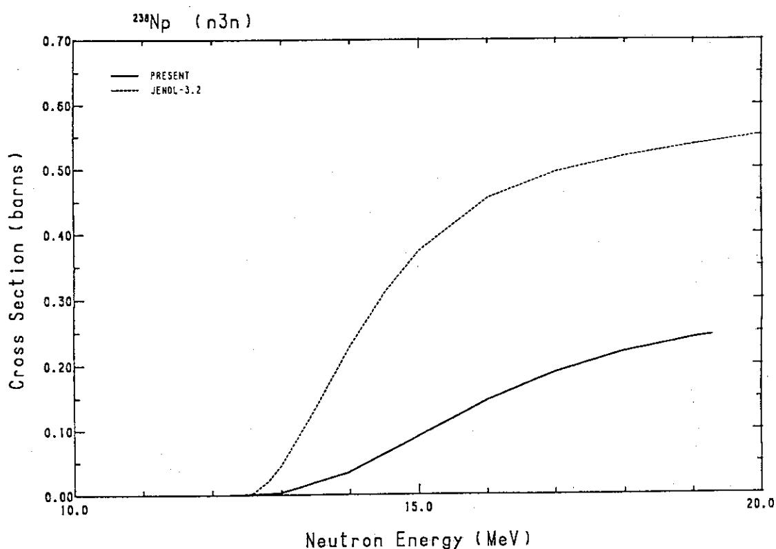
Fig. 235 Comparison of the ( $n,3n$ )-cross-section for  $^{238}\text{Np}$ .
