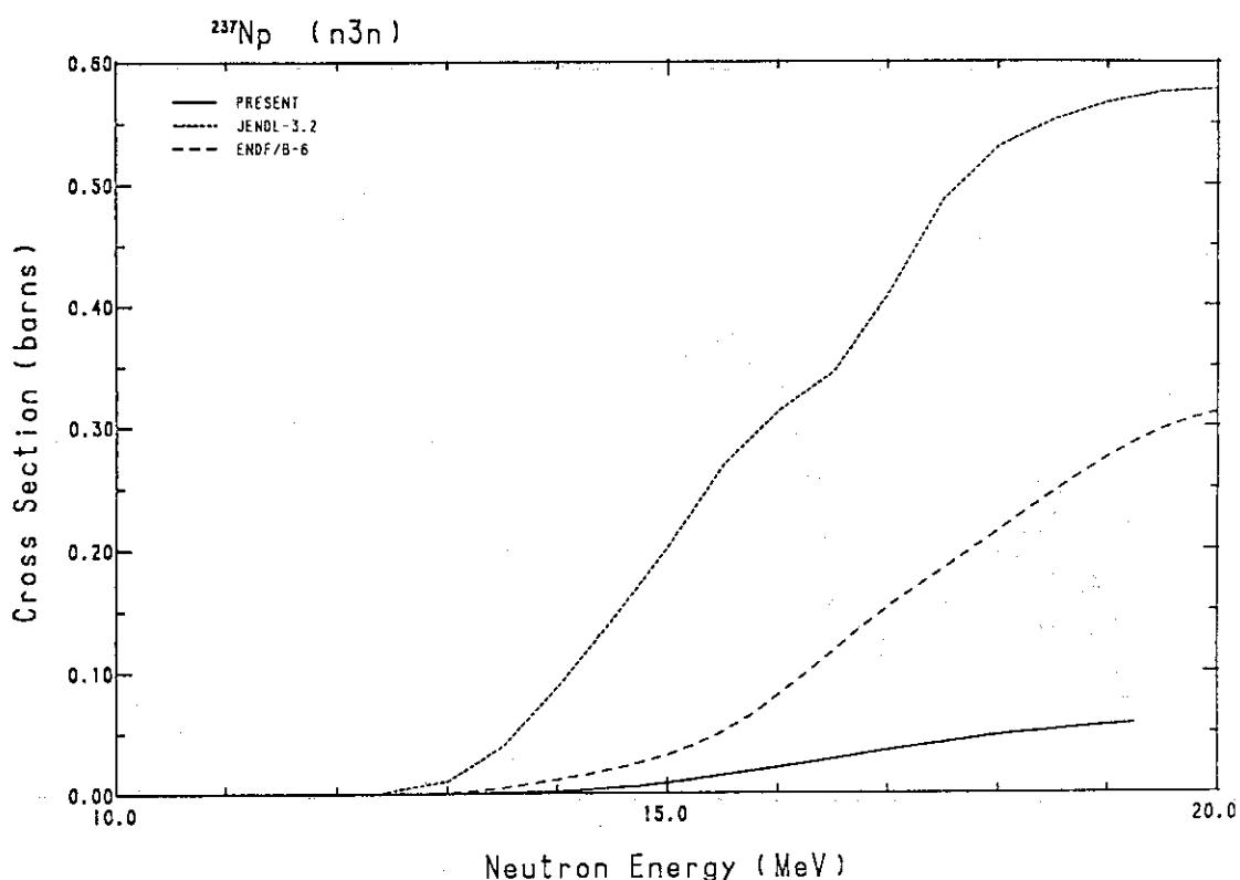
Fig. 232 Comparison of the ( $n,3n$ )-cross-section for  $^{237}\text{Np}$ .
