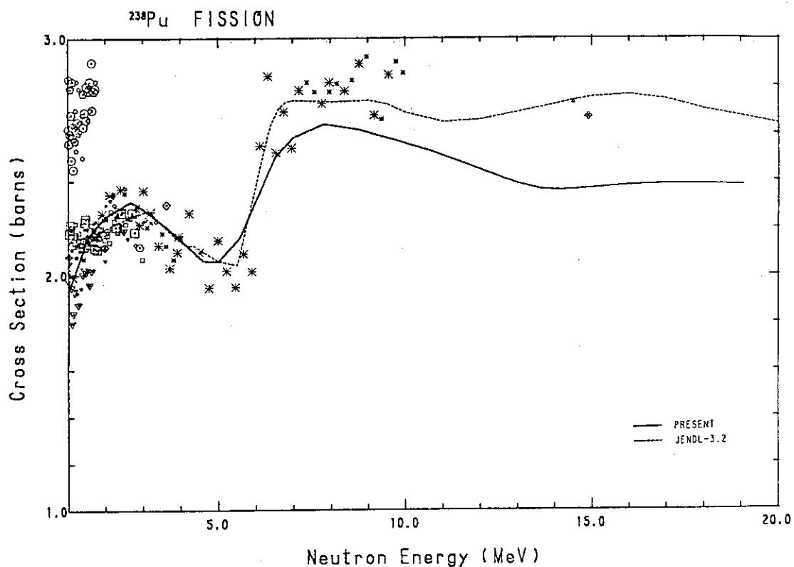
Fig. 240 Comparison of the fission cross-section for  $^{238}\text{Pu}$ .
