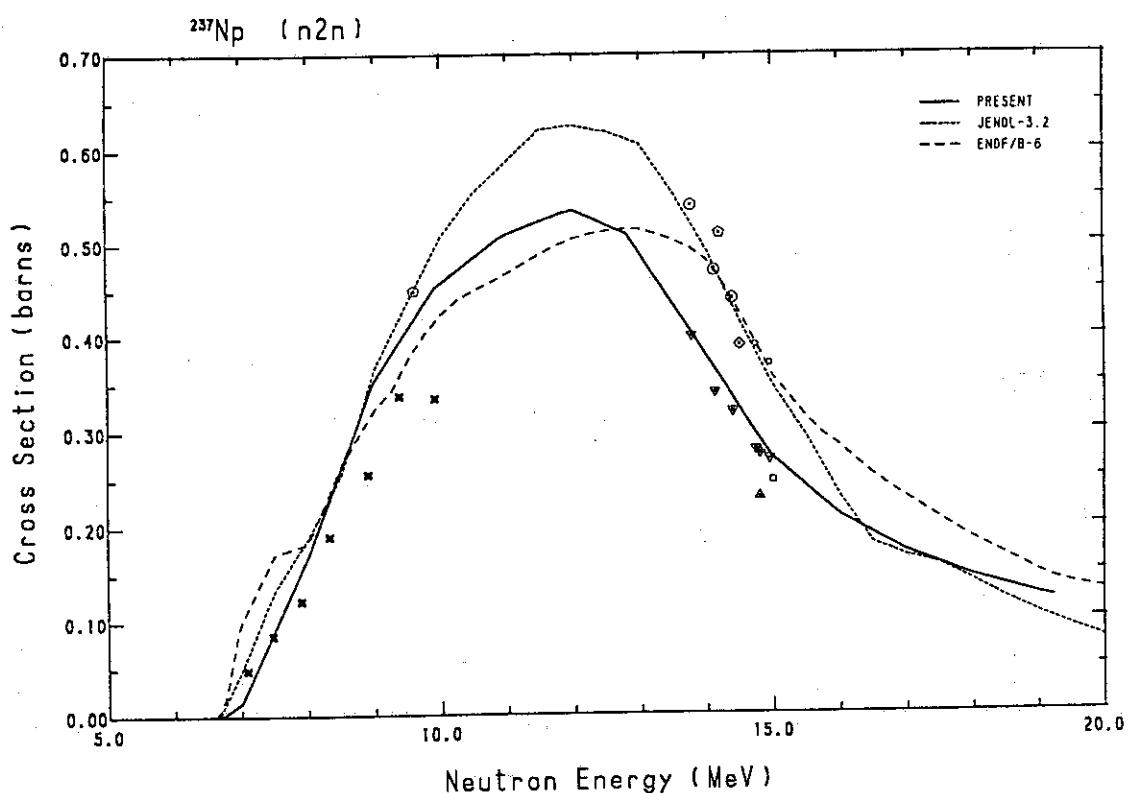
Fig. 231 Comparison of the ( $n,2n$ )-cross-section for  $^{237}\text{Np}$ .
