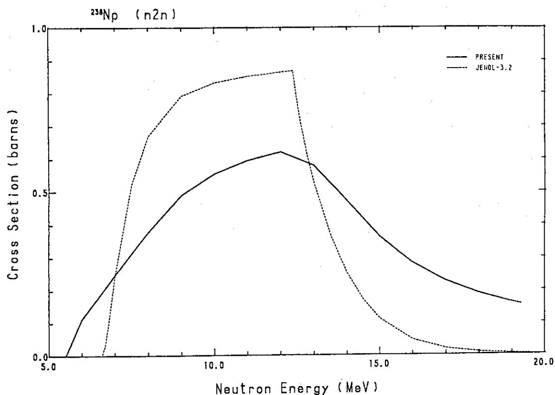
Fig. 234 Comparison of the ( $n,2n$ )-cross-section for  $^{238}\text{Np}$ .
