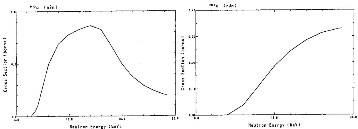
Fig. 107 The  $(n,2n)$ -reaction cross-section of  $^{242}\text{Pu}$ .Fig. 108 The  $(n,3n)$ -reaction cross-section of  $^{242}\text{Pu}$ .
