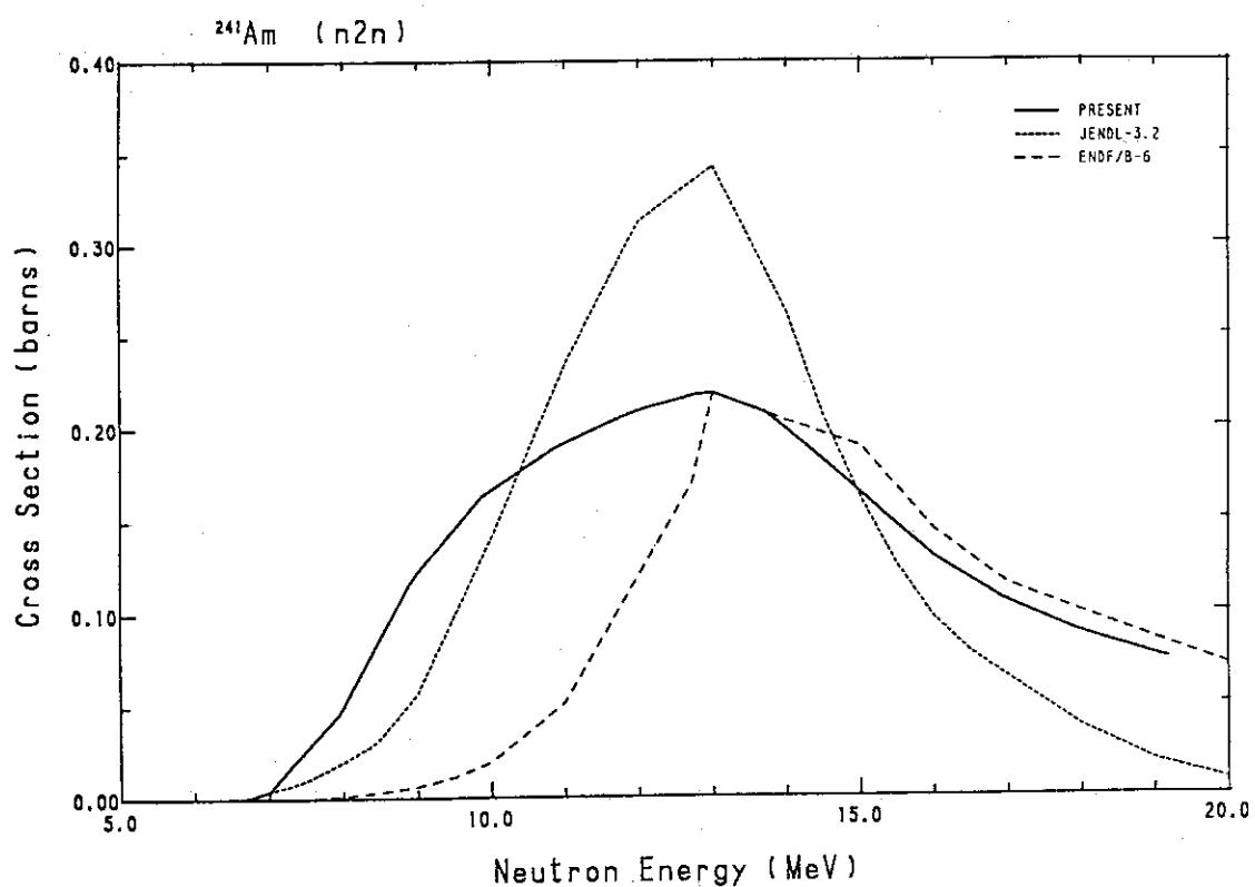
Fig. 249 Comparison of the ( $n,2n$ )-cross-section for  $^{241}\text{Am}$ .
