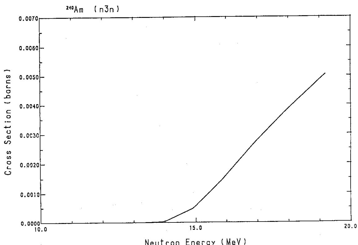
Fig. 129 The  $(n,3n)$ -reaction cross-section of  $^{240}\text{Am}$ .
