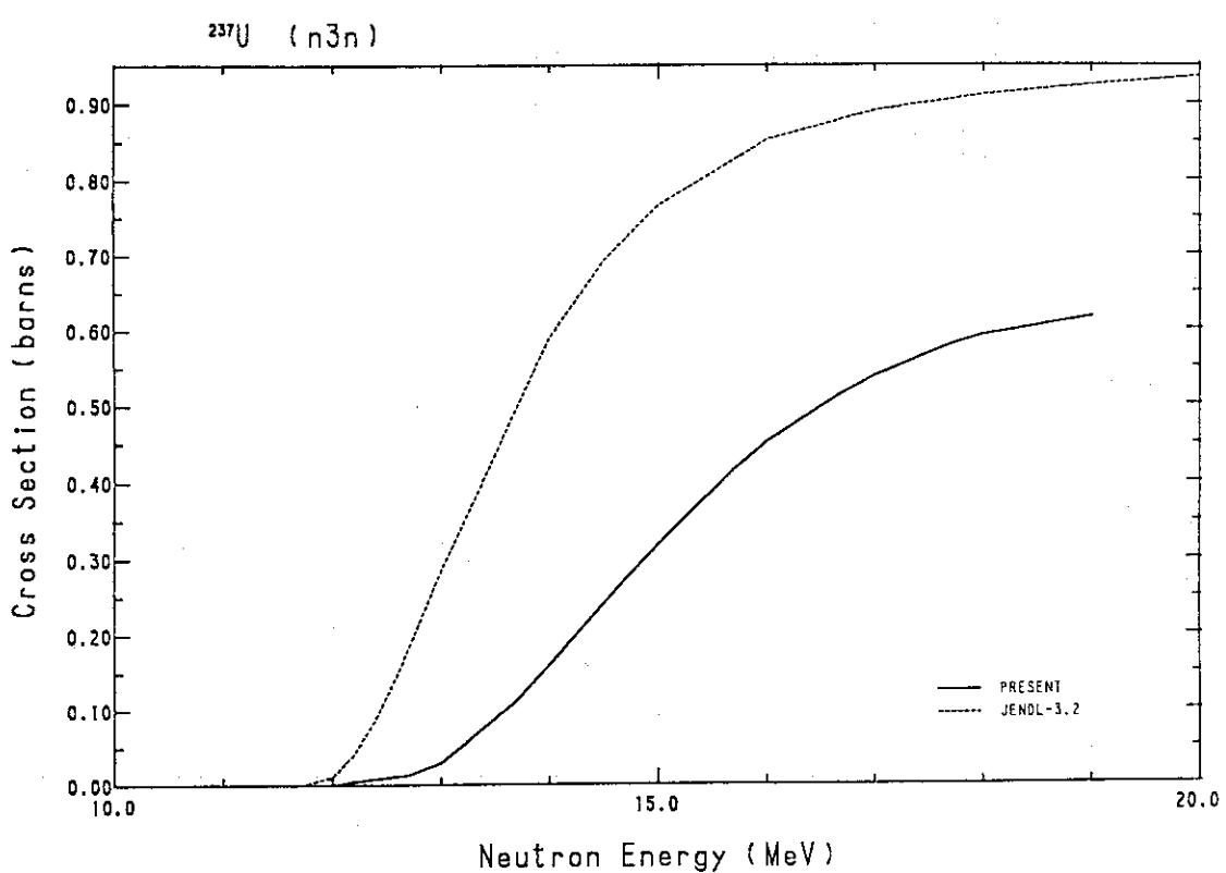
Fig. 225 Comparison of the ( $n,3n$ )-cross-section for  $^{237}\text{U}$ .
