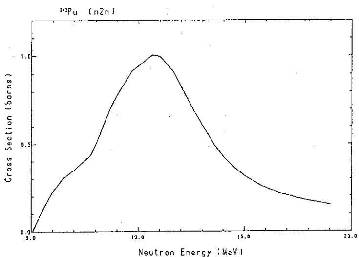
Fig. 110 The  $(n,2n)$ -reaction cross-section of  $^{248}\text{Pu}$ .
