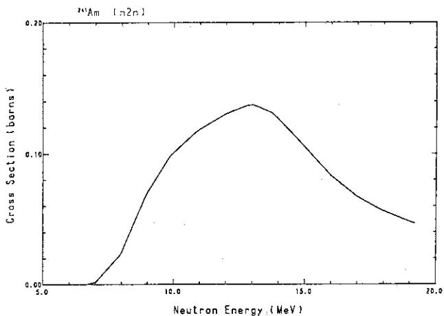
Fig. 131 The  $(n,2n)$ -reaction cross-section of  $^{241}\text{Am}$ .
