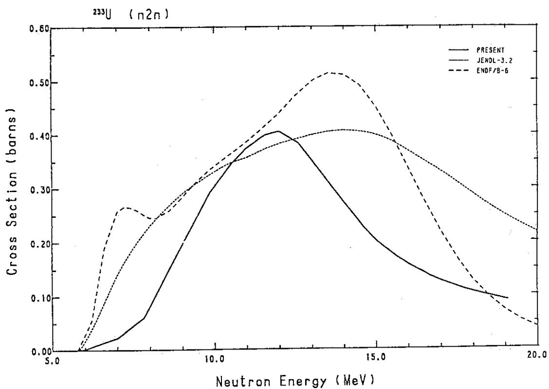
Fig. 219 Comparison of the ( $n,2n$ )-cross-section for  $^{233}\text{U}$ .
