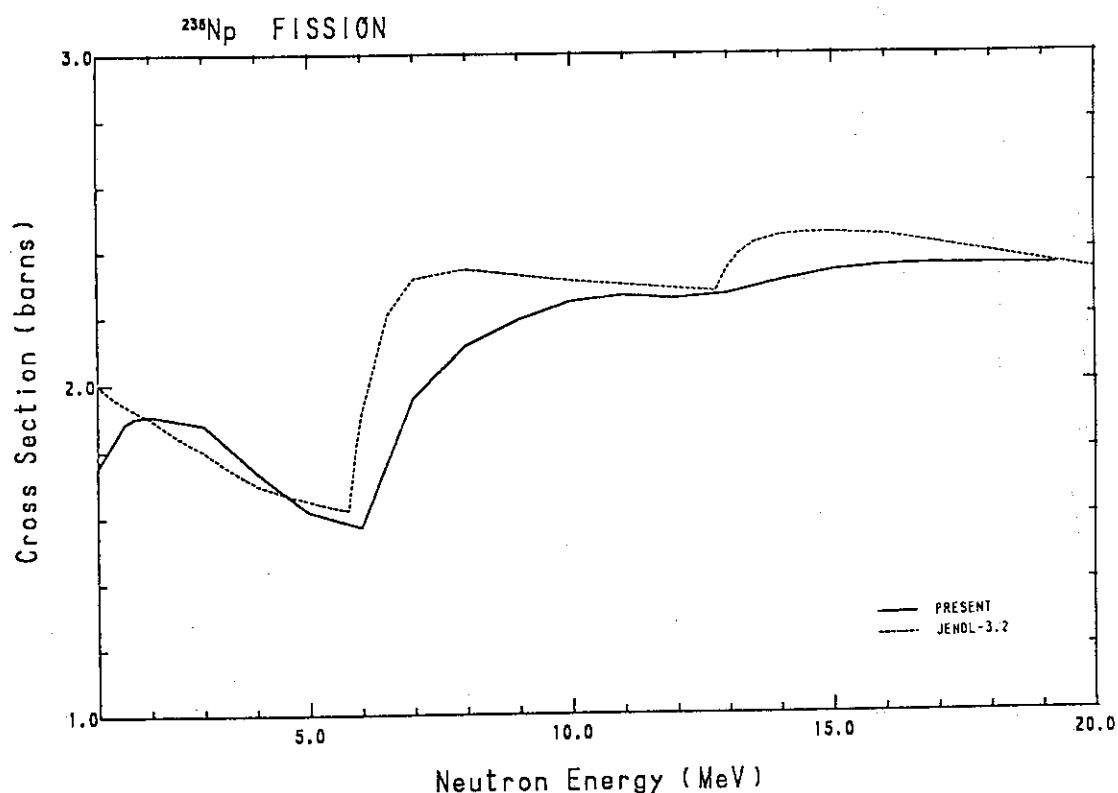
Fig. 227 Comparison of the fission cross-section for  $^{238}\text{Np}$ .
