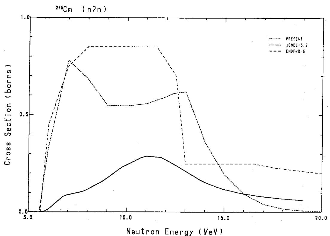
Fig. 261 Comparison of the ( $n,2n$ )-cross-section for  $^{245}\text{Cm}$ .
