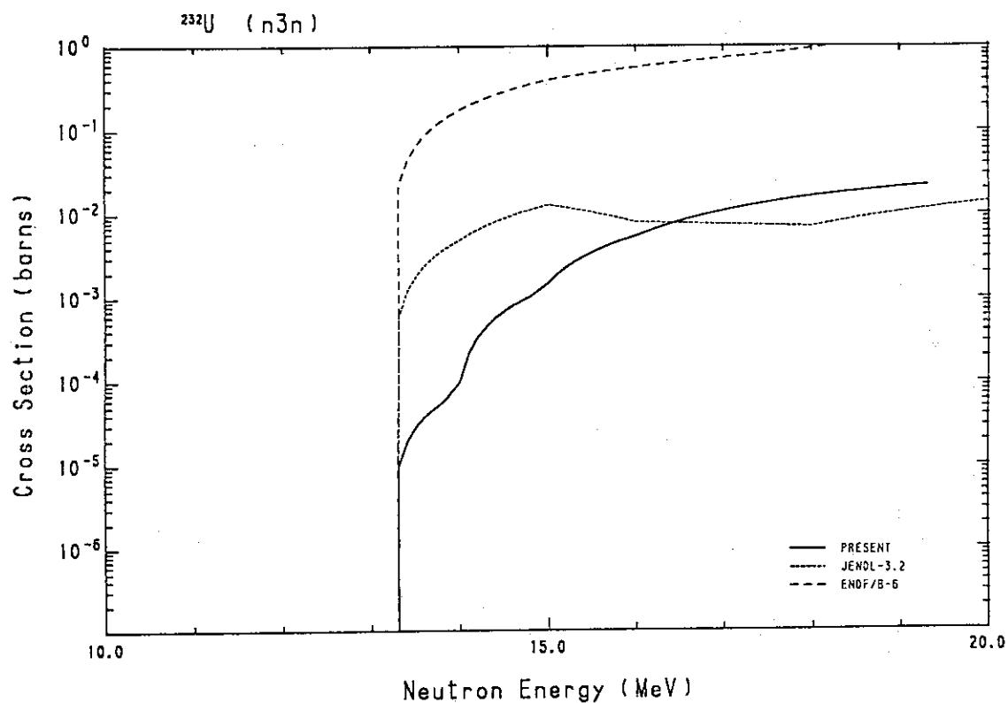
Fig. 218 Comparison of the ( $n,3n$ )-cross-section for  $^{232}\text{U}$ .
