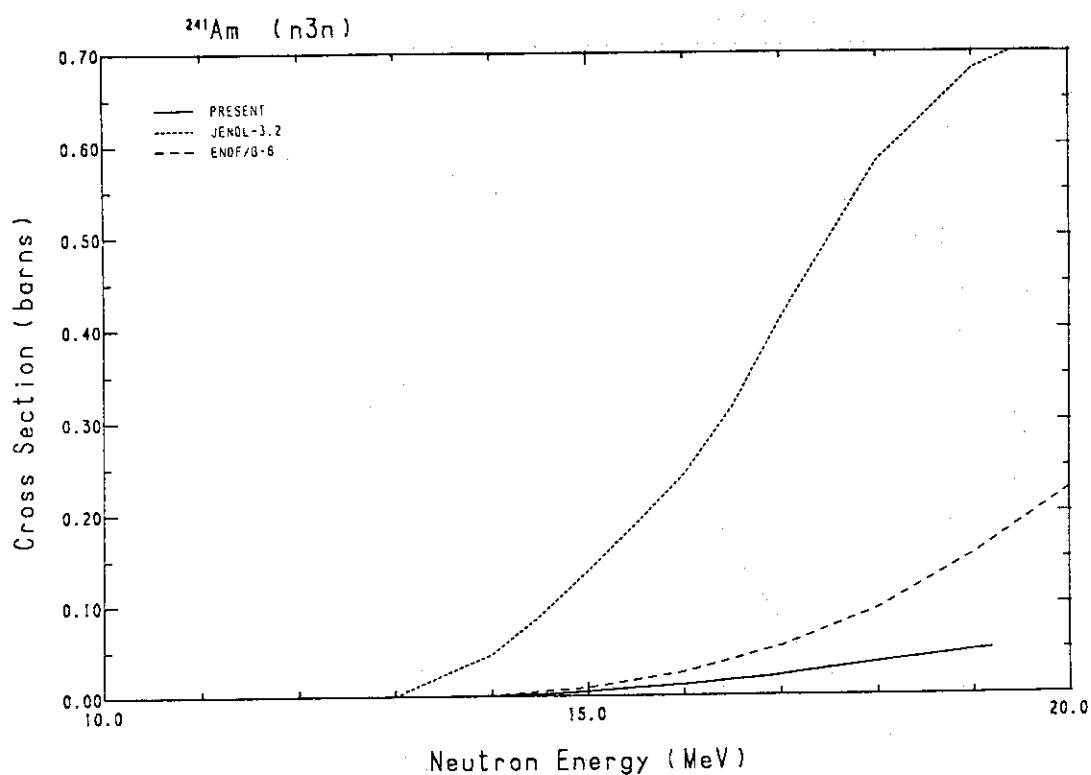
Fig. 250 Comparison of the ( $n,3n$ )-cross-section for  $^{241}\text{Am}$ .
