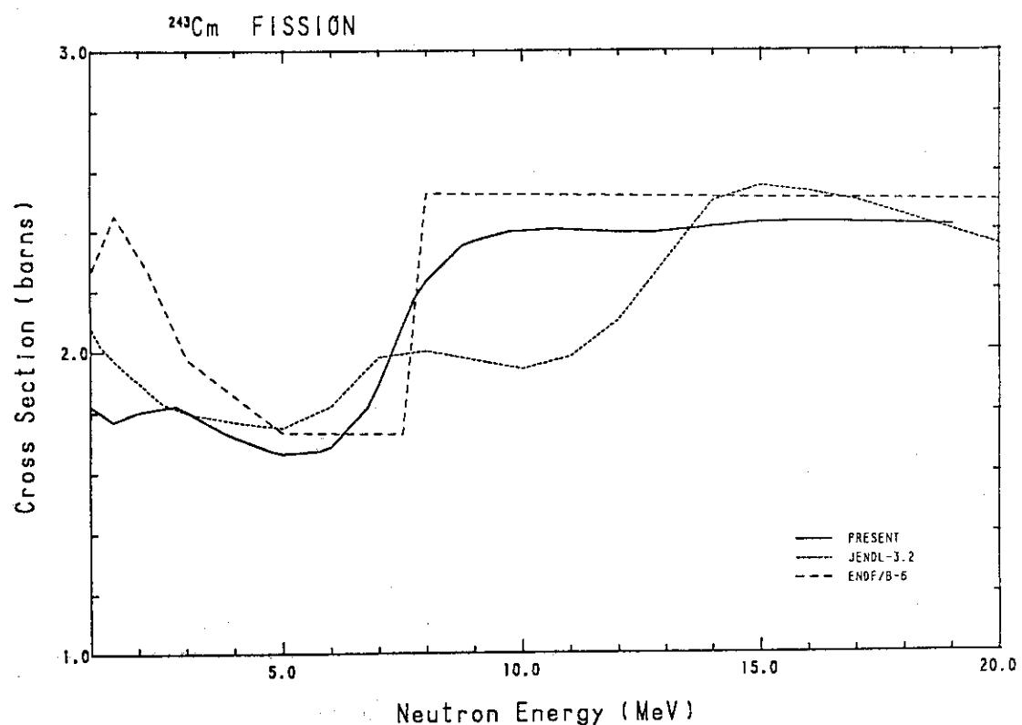
Fig. 257 Comparison of the fission cross-section for  $^{243}\text{Cm}$ .
