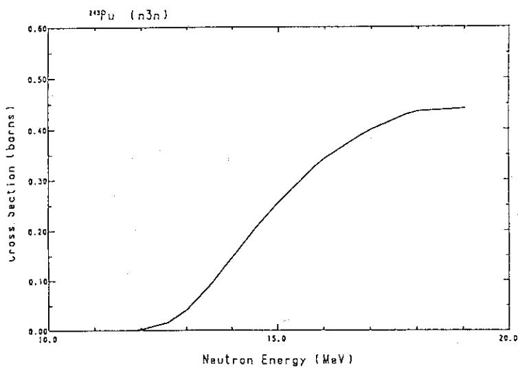
Fig. 111 The  $(n,3n)$ -reaction cross-section of  $^{248}\text{Pu}$ .
