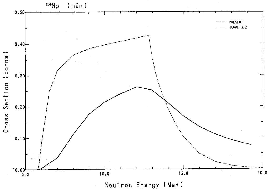
Fig. 228 Comparison of the  $(n,2n)$ -cross-section for  $^{236}\text{Np}$ .
