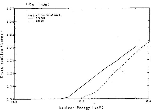
Fig. 161 The  $(n,3n)$ -reaction cross-section of  $^{243}\text{Cm}$ .
