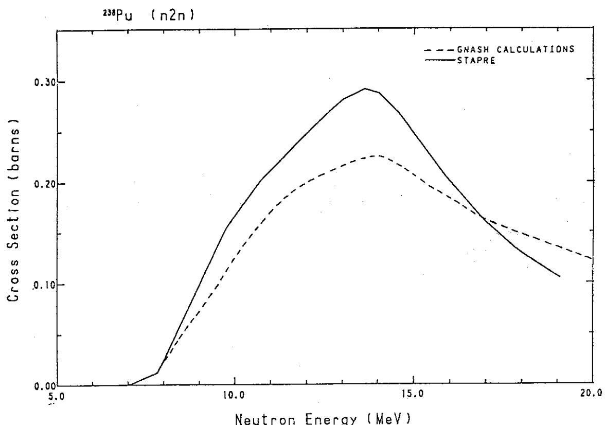
Fig. 95 The ( $n,2n$ )-reaction cross-section of  $^{238}\text{Pu}$ .
