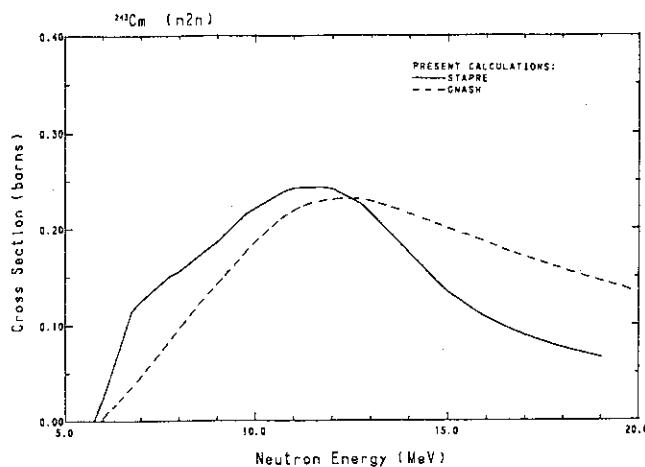
Fig. 162 The  $(n,2n)$ -reaction cross-section of  $^{243}\text{Cm}$ .
