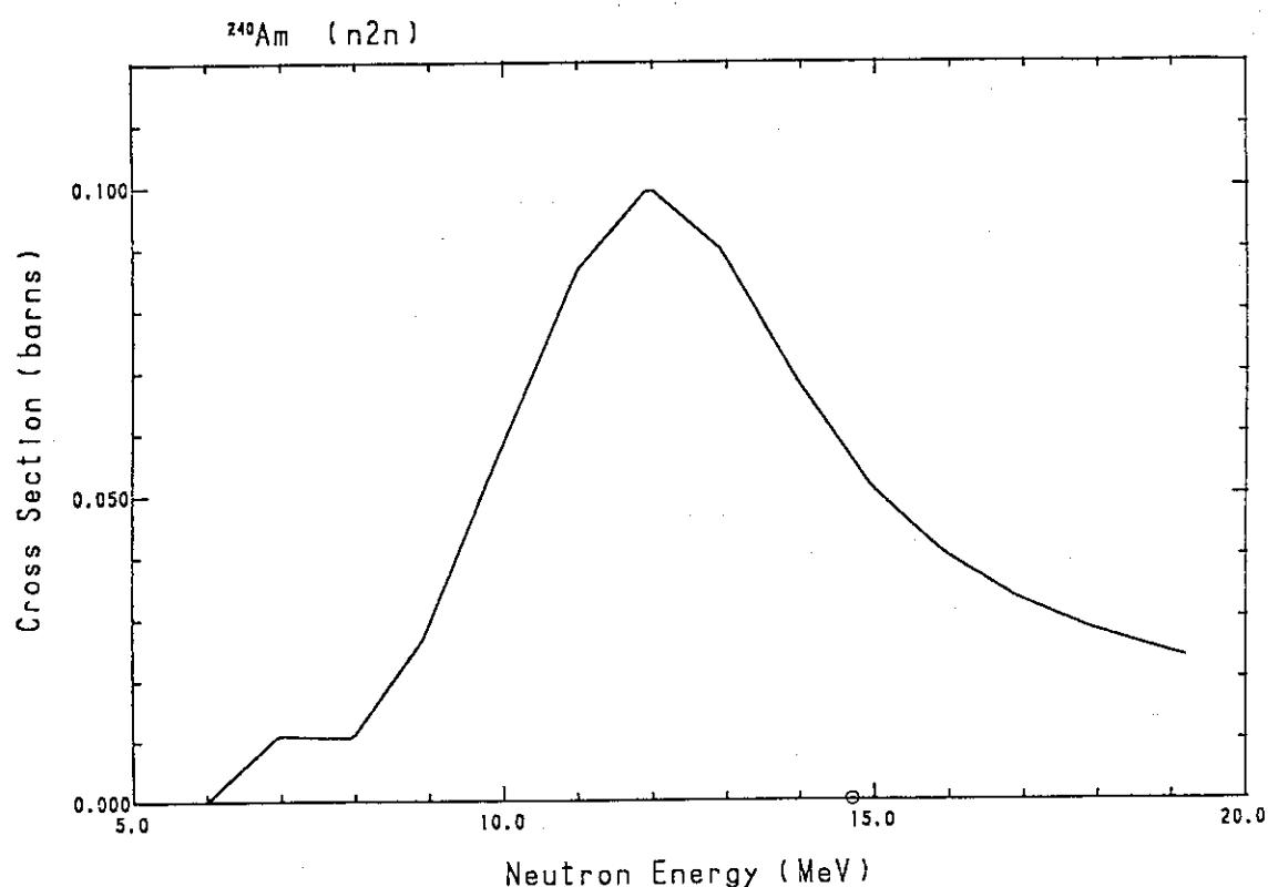
Fig. 128 The  $(n,2n)$ -reaction cross-section of  $^{240}\text{Am}$ .
