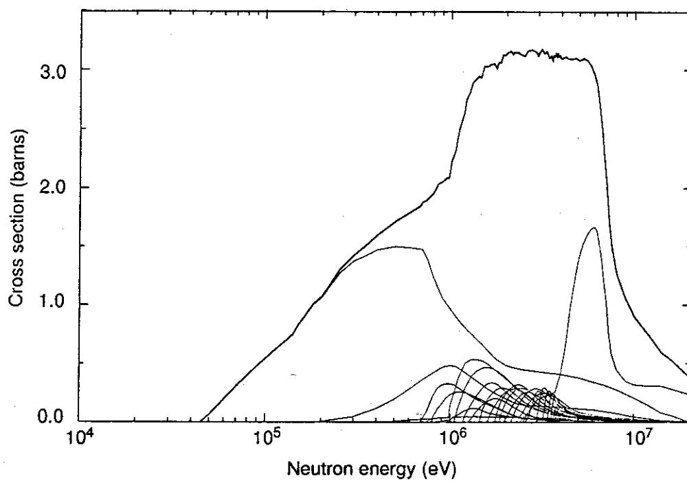
Fig. 17 Total inelastic scattering cross section of  $^{238}\text{U}$  and its partial cross sections of continuum and discrete levels in ENDF/B-VI library
