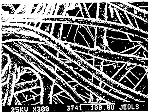
Photo 1. Clean surface of EC-2 felt.
