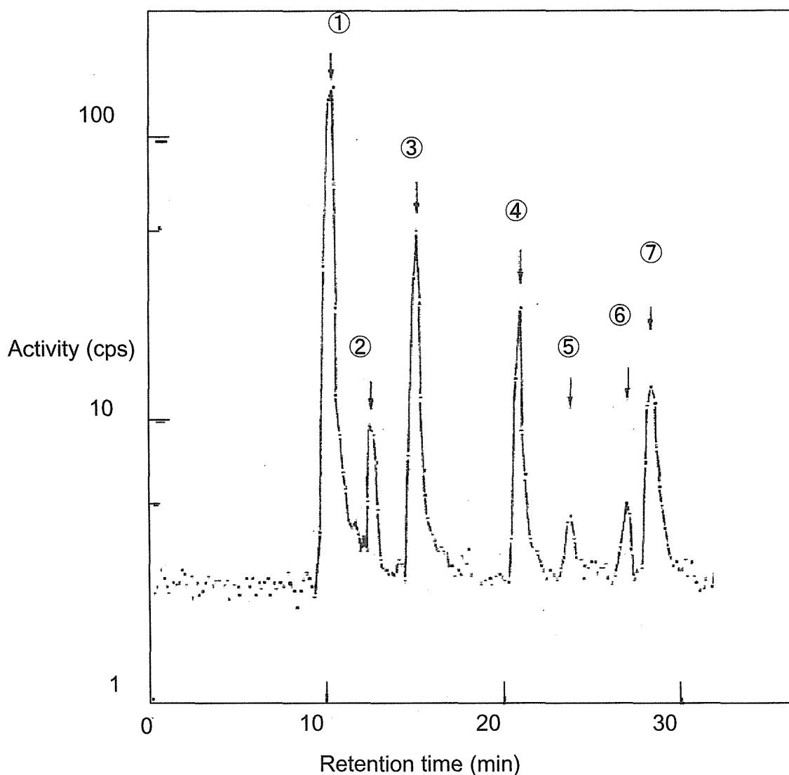
Fig. 4 Typical radio-gas chromatogram of organic iodides
