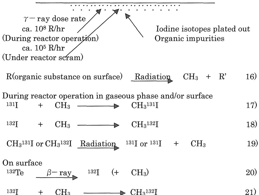
Fig. 10. Formation mechanisms of organic iodides from  $^{132}\text{Te}$
