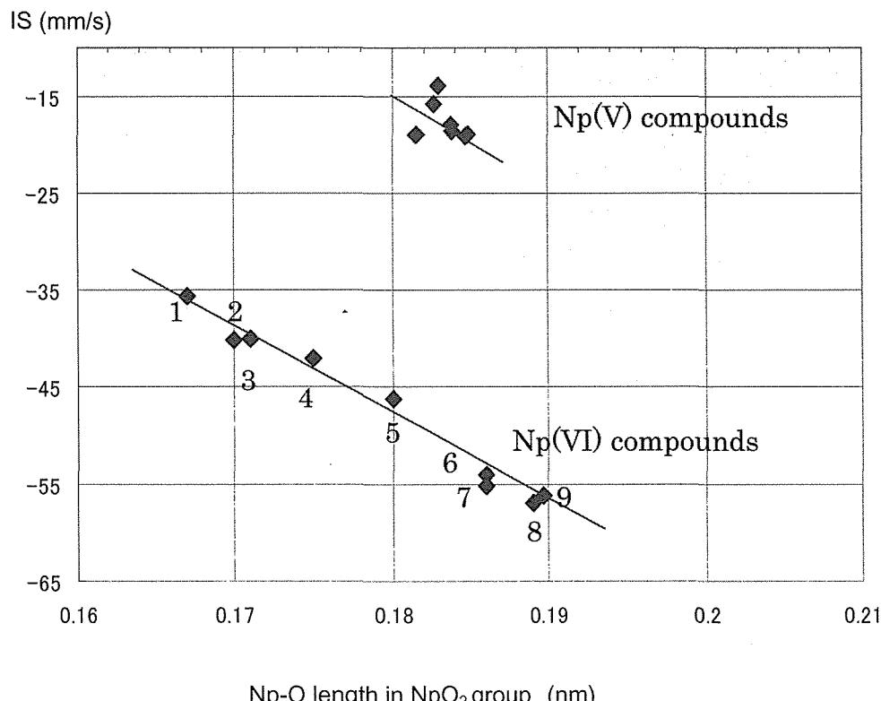
Fig. 15 Relationship between isomer shifts and bond length of Np-O in  $\text{NpO}_2^{+}$  or  $^{2+}$  group of compounds
