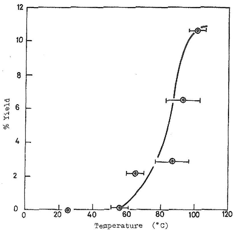
Fig. 5 Temperature dependence on yield of organic iodides
