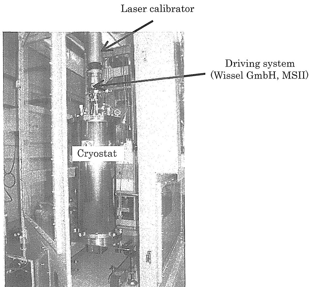
Fig. 12 Mössbauer driving system for  $^{237}\text{Np}$  with cryostat
