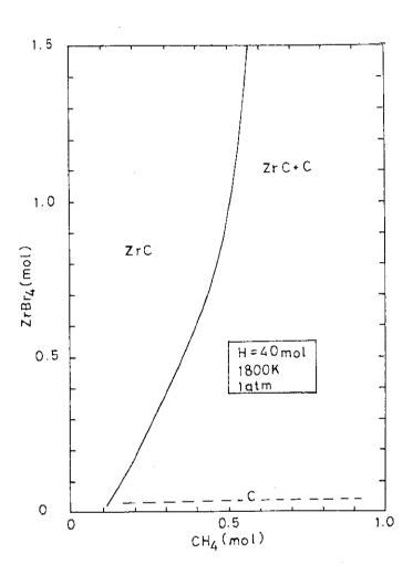
Fig. 2 A map of deposition products predicted by the thermochemical analysis. (reproduced from ref. [27])
