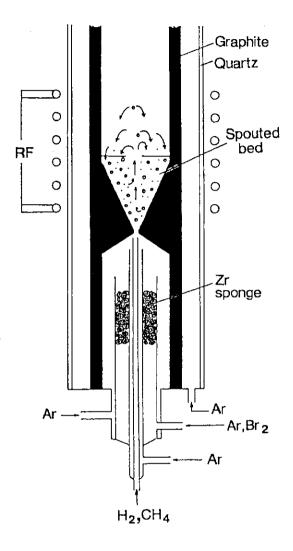
Fig. 1 Experimental apparatus for depositing ZrC by the bromide process. (reproduced from ref. [28])
