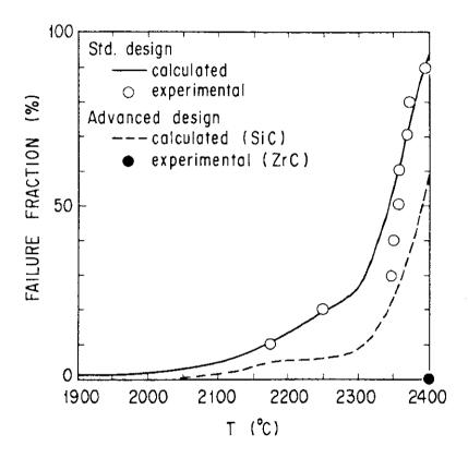
Fig. 4 Comparison of failure fraction of the ZrC-Triso coated fuel particles with the reference SiC-Triso coated particles. Dashed line gives model prediction for the SiC-Triso coated particles, which have the same dimensions as the ZrC-Triso coated particles in this study.
