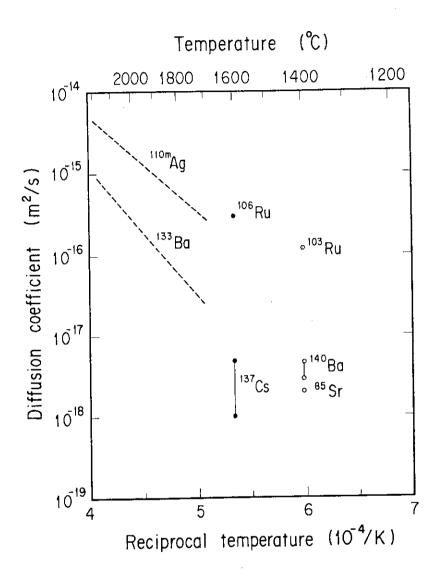
Fig. 6 Diffusion coefficients for fission product species in ZrC. Data of solid circles are from ref. [50], open circles from ref. [48], and broken lines from ref. [49]. (reproduced from ref. [50])
