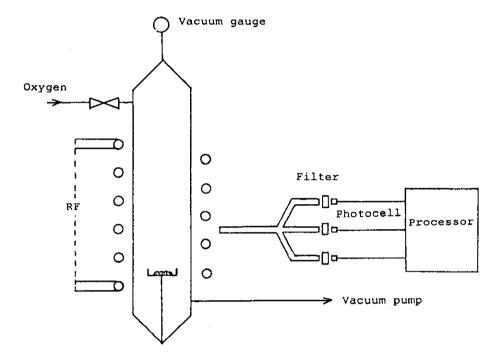
Fig. 3 Plasma oxidation apparatus for removing PyC layers from ZrC. (reproduced from ref. [28])
