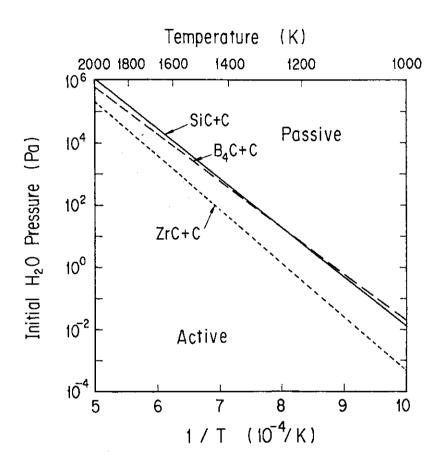
Fig. 5 Active-to-passive oxidation transitions for ZrC+C, B<sub>4</sub>C+C and SiC+C calculated in the (ZrC, B<sub>4</sub>C or SiC)-C-H<sub>2</sub>O-He system as a function of temperature and initial H<sub>2</sub>O pressure.
