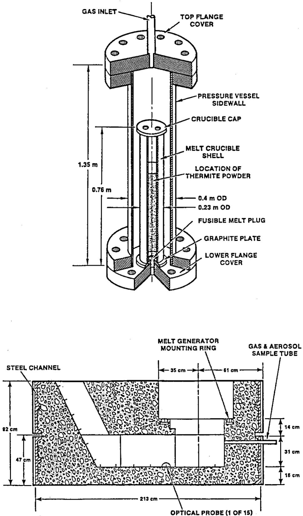
Figure 14: Schematic Diagram of the Melt Generator and Cavity for the HIPS Series of Tests in Sandia National Laboratories, USA
