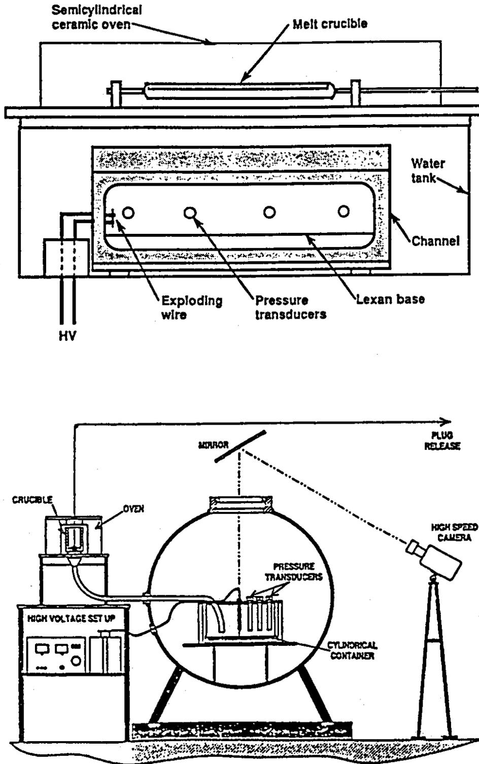
Figure 8: Schematic Diagrams of Experimental Apparatus (Top: Narrow Channel Experiment and Bottom: Cylindrical Tank Experiment) at McGill University, Canada
