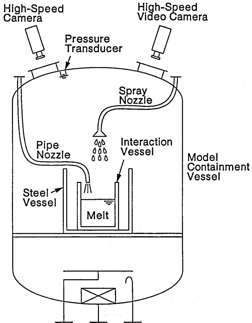
Figure 6: Schematic of Experimental Apparatus for ACM Series of Tests in JAERI, Japan
