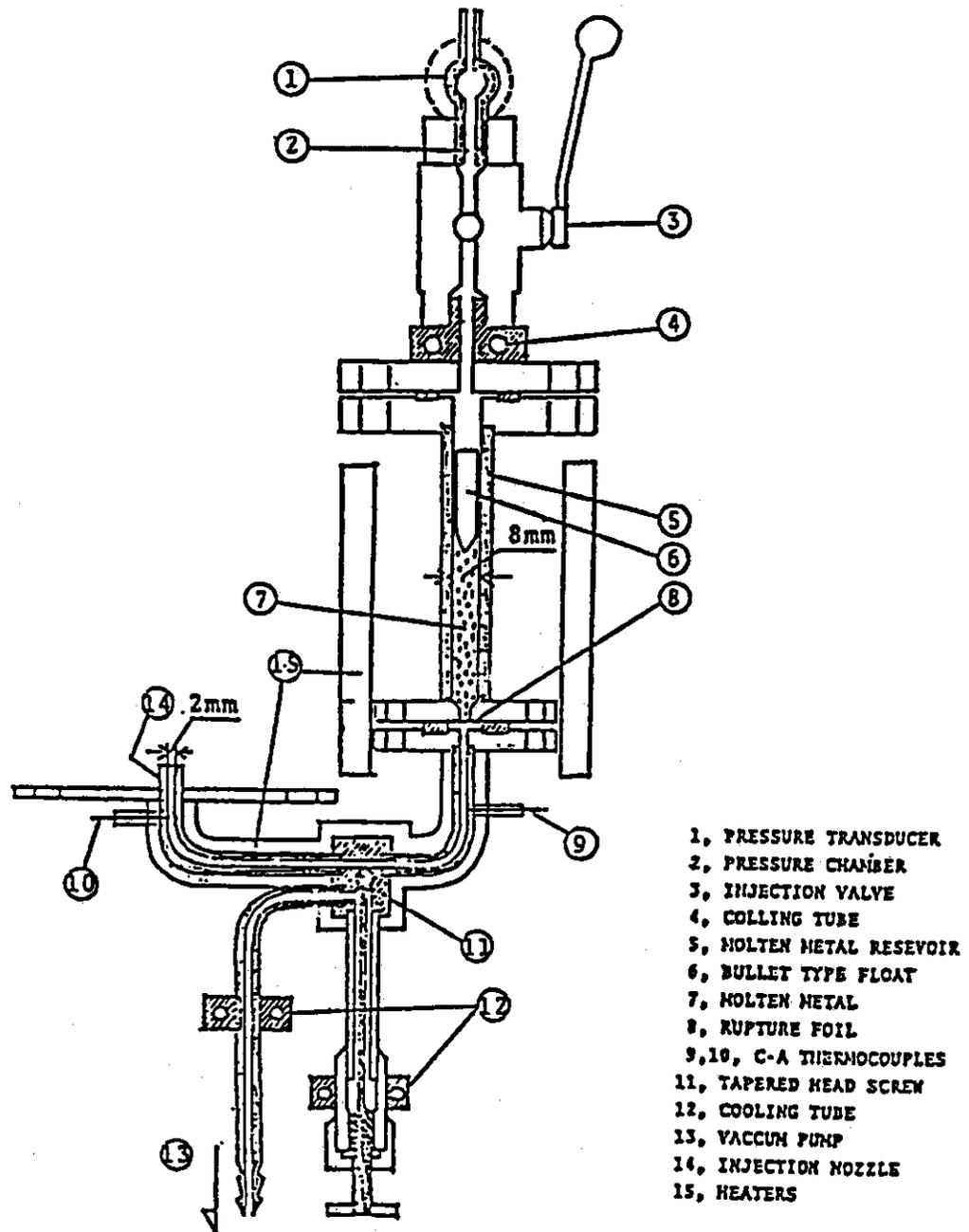
Figure 12: Schematic of Kondo's Experimental Apparatus at University of Tokyo, Japan
