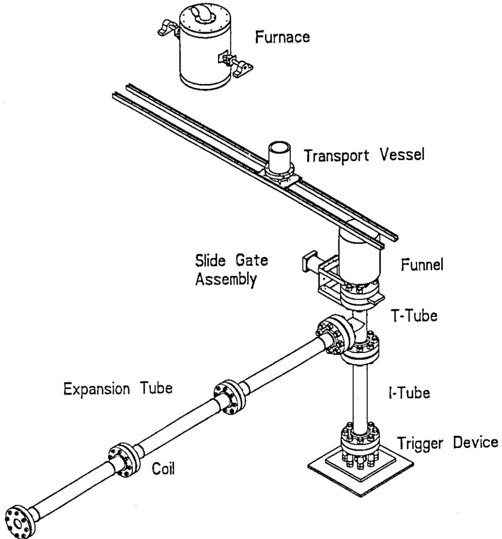
Figure 3: Overall Three Dimensional View of the WFCI Facility in University of Wisconsin-Madison, USA
