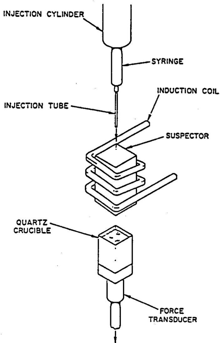
Figure 9: Schematic of Experimental Apparatus for Coolant Injection Mode of Contact in Argonne National Laboratories, USA
