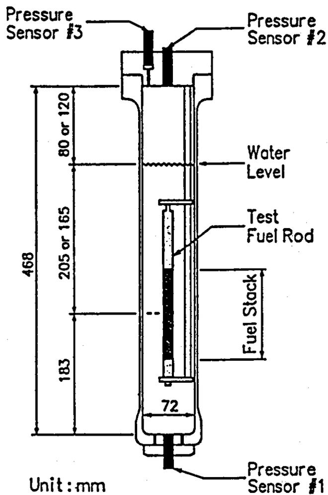
Figure 15: Schematic Diagram of the Test Capsule of Fuketa's Experiments at JAERI, Japan
