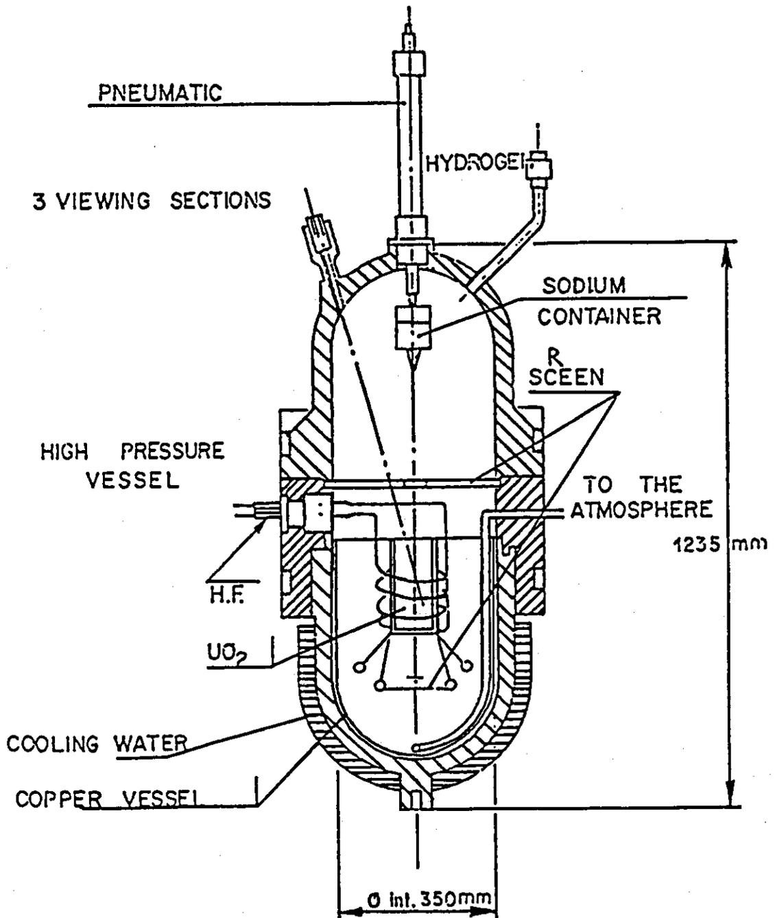
Figure 10: Schematic of CORECT-I Experimental Apparatus at Grenoble, France
