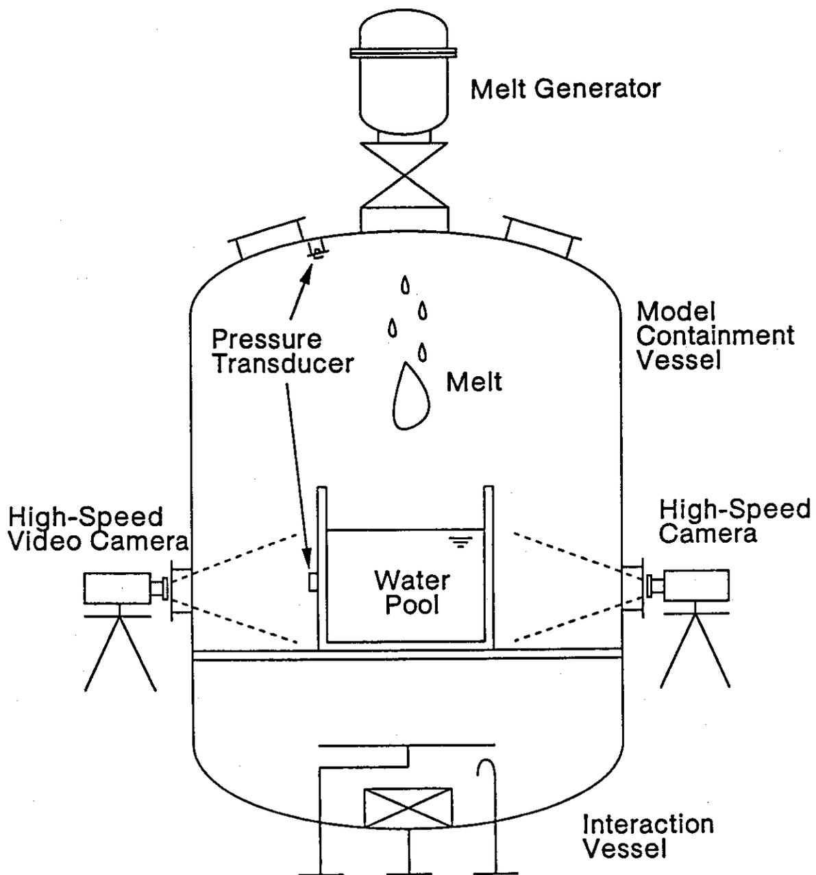
Figure 4: Schematic Illustration of the ALPHA Facility in JAERI, Japan
