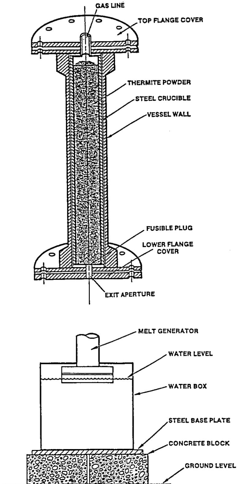
Figure 13: Schematic Diagram of the Melt Generator and Cavity for the STIP Series of Tests in Sandia National Laboratories, USA
