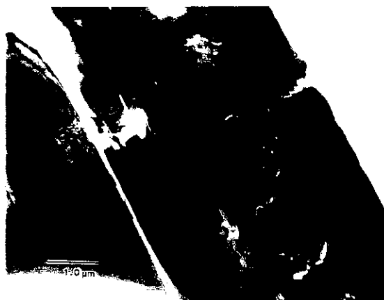
Fig. 2 Low magnified cross-sectional TEM image. Within the whole specimen, some areas with white contrast with a stair shape were observed.
