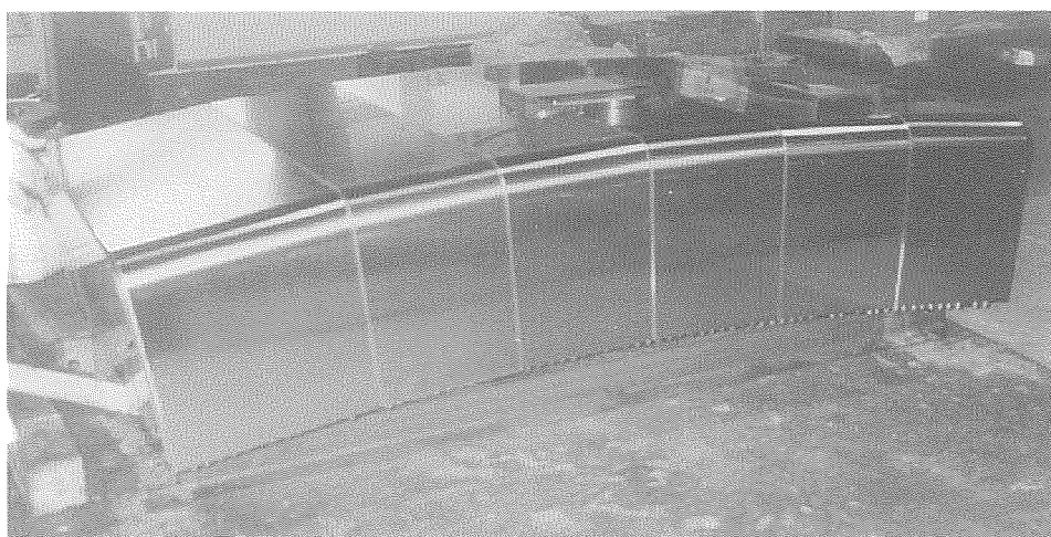
Fig. 4.12 Assembly of the SS canning for HIP process
