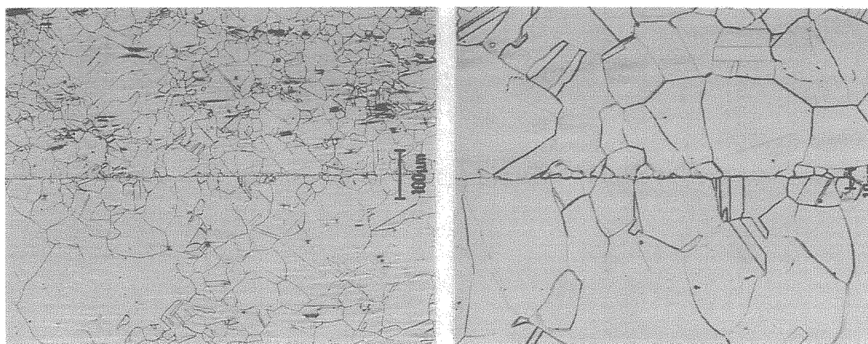
Fig. A-6.32 Micro-scopic images at the SS/SS HIP bonded interface in the location ③-2 of the cross-section G shown in Figs. A-1 and A-4
