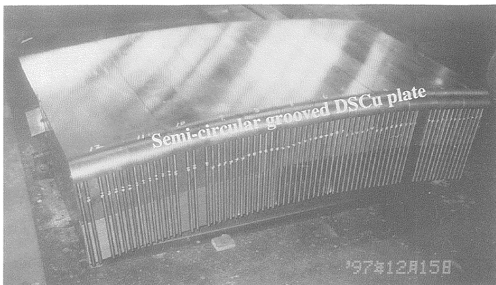
Fig. 4.11 Assembly of the first wall elements with the shield block into one assembly. Assembly of the semi-circular grooved DSCu plate (plasma-side)
