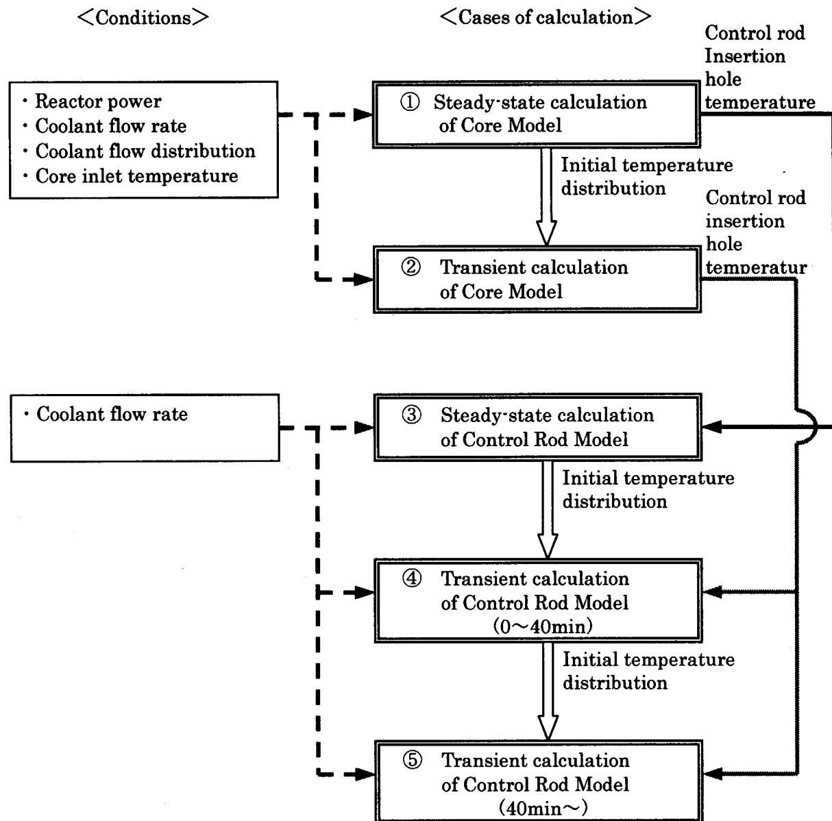
Fig.3.2.1 Flow diagram of Control rod temperature analysis
