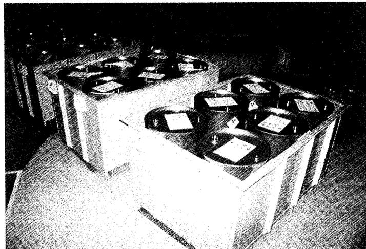
Fig.4.27 Seal Box for Transportation Drums
