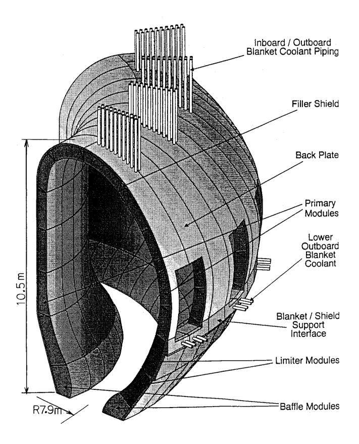
Fig. 1 Mechanical configuration of modular blanket structure
