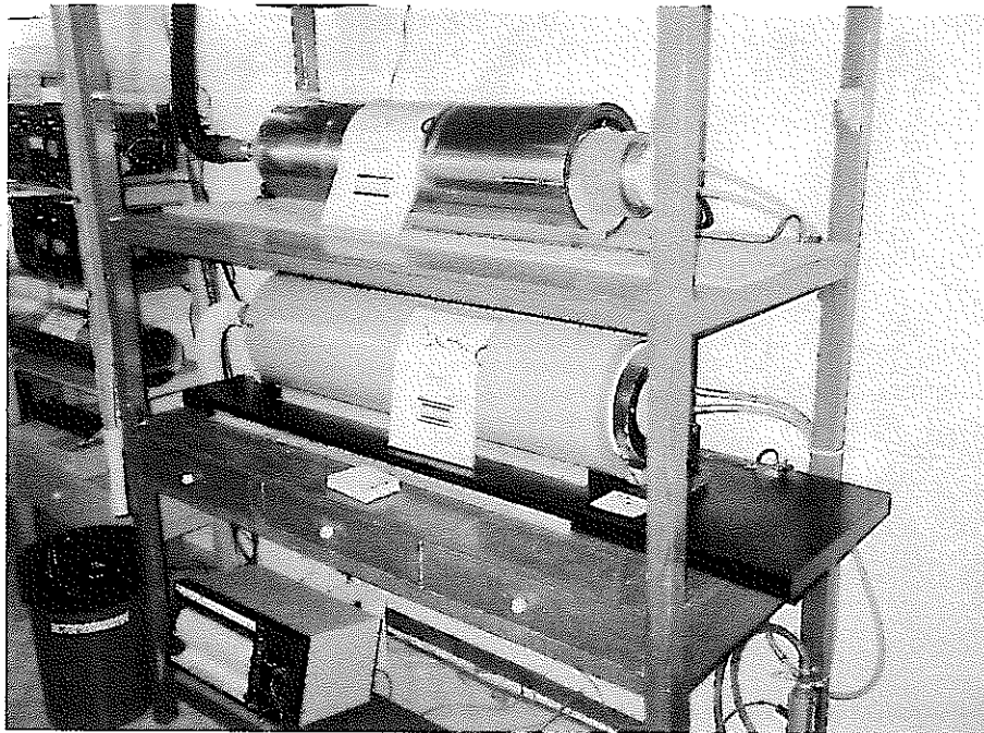
熱消磁用電気炉
