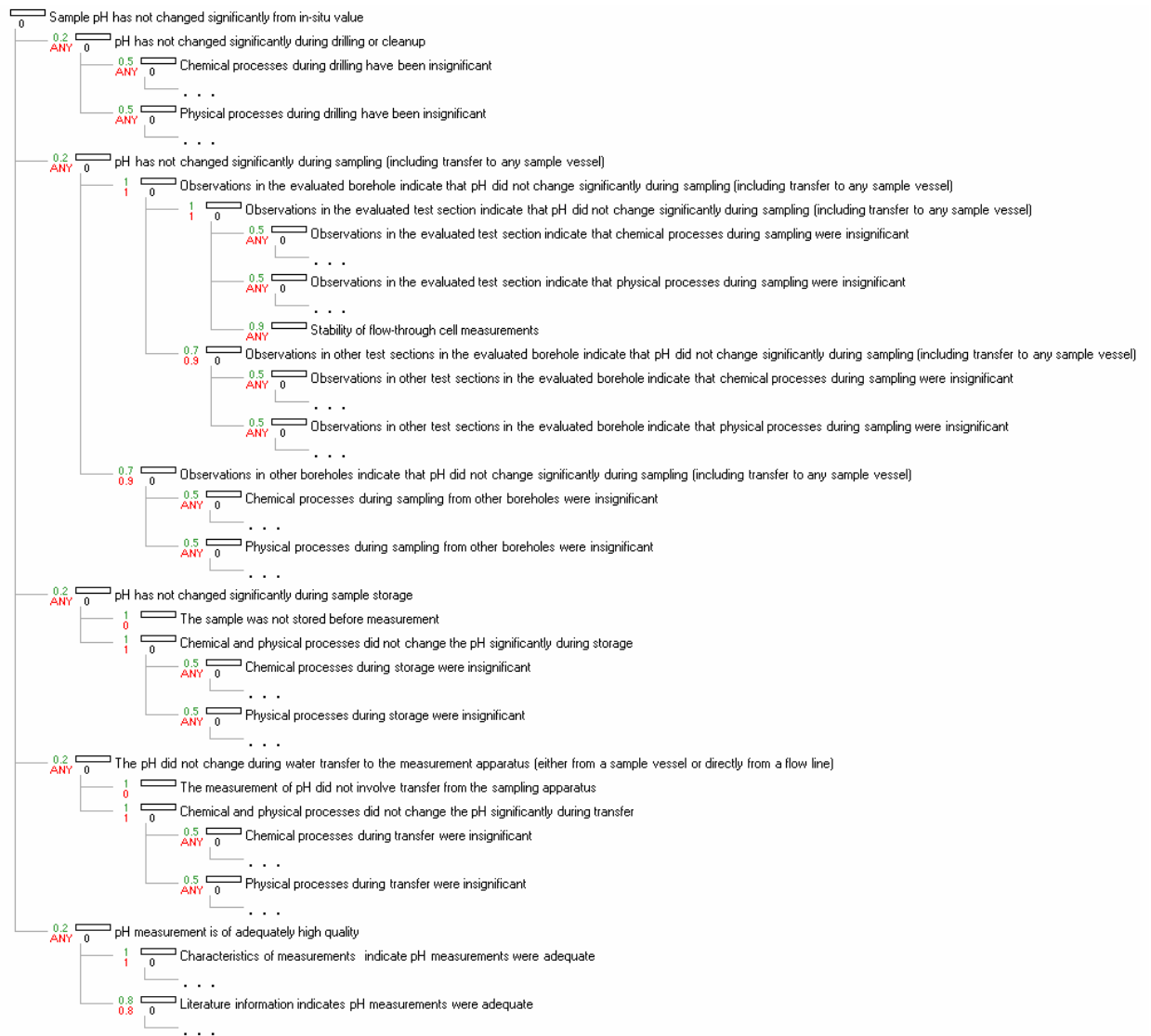
Figure 3-9 Iternative outline process model showing the overall evaluation of data quality. Processes that have associated sub-process models are indicated by '...'.
