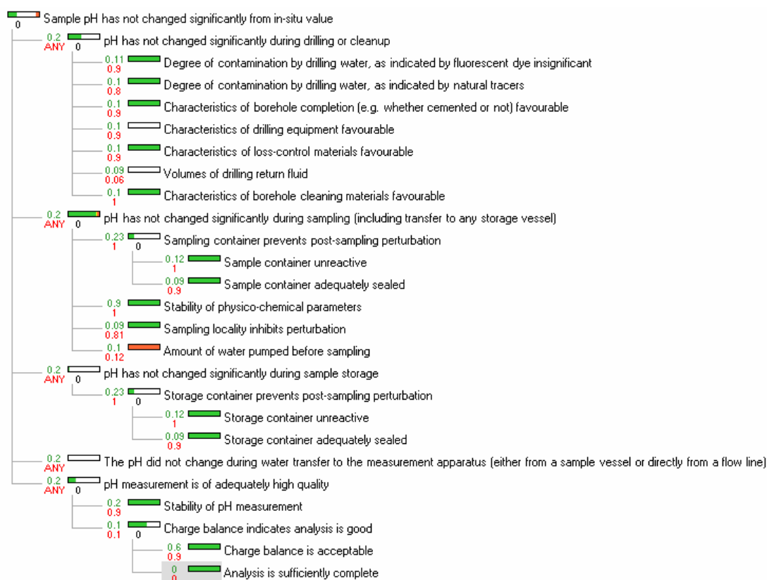
Figure 3-10 Example process model that includes only processes that correspond to possible quality indicators for which information actually exists.
