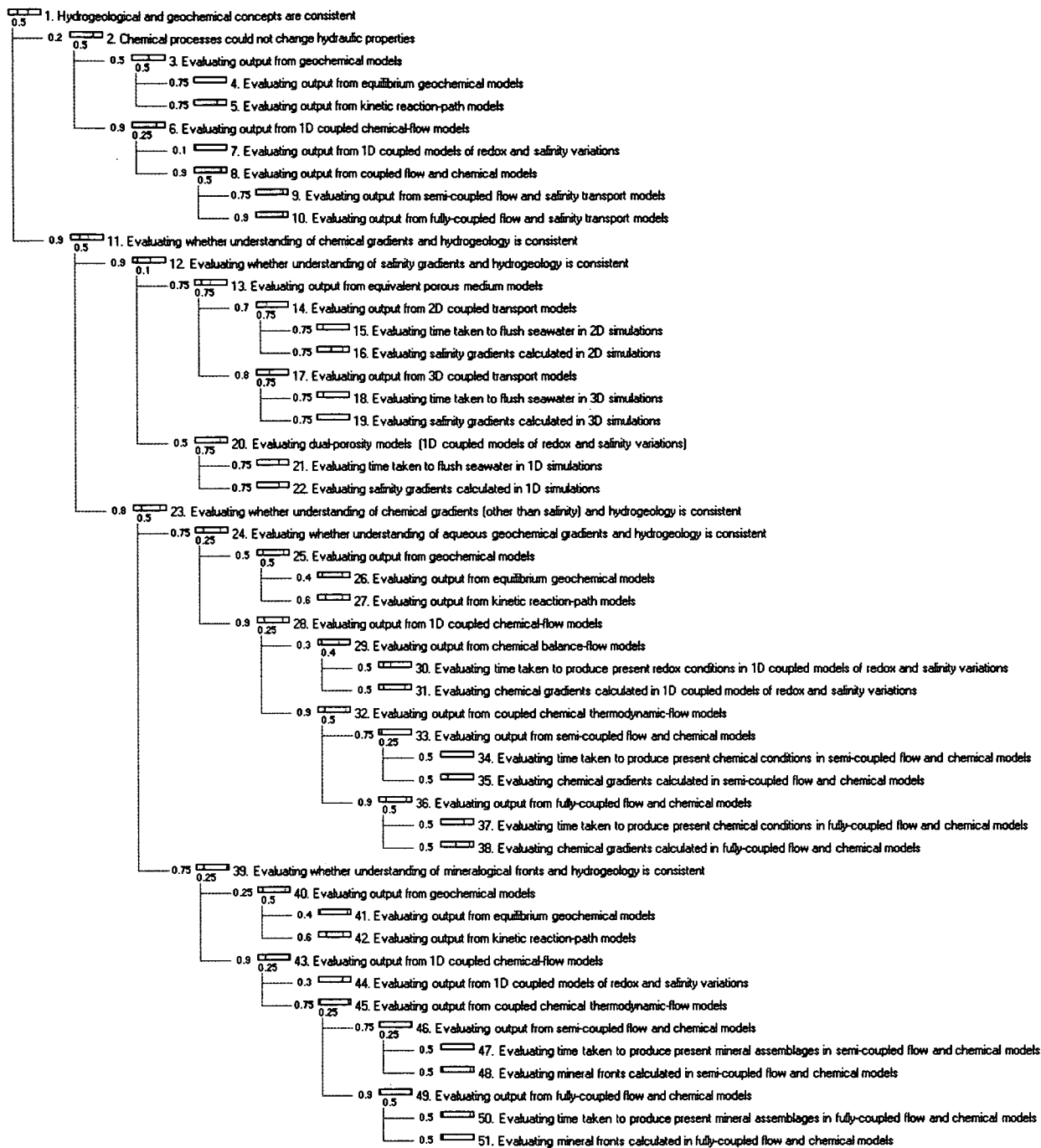
Figure 64. An ESL process model to evaluate the degree to which the hypothesis that the hydrogeological and geochemical concepts are consistent (process 1, top left) is valid.
