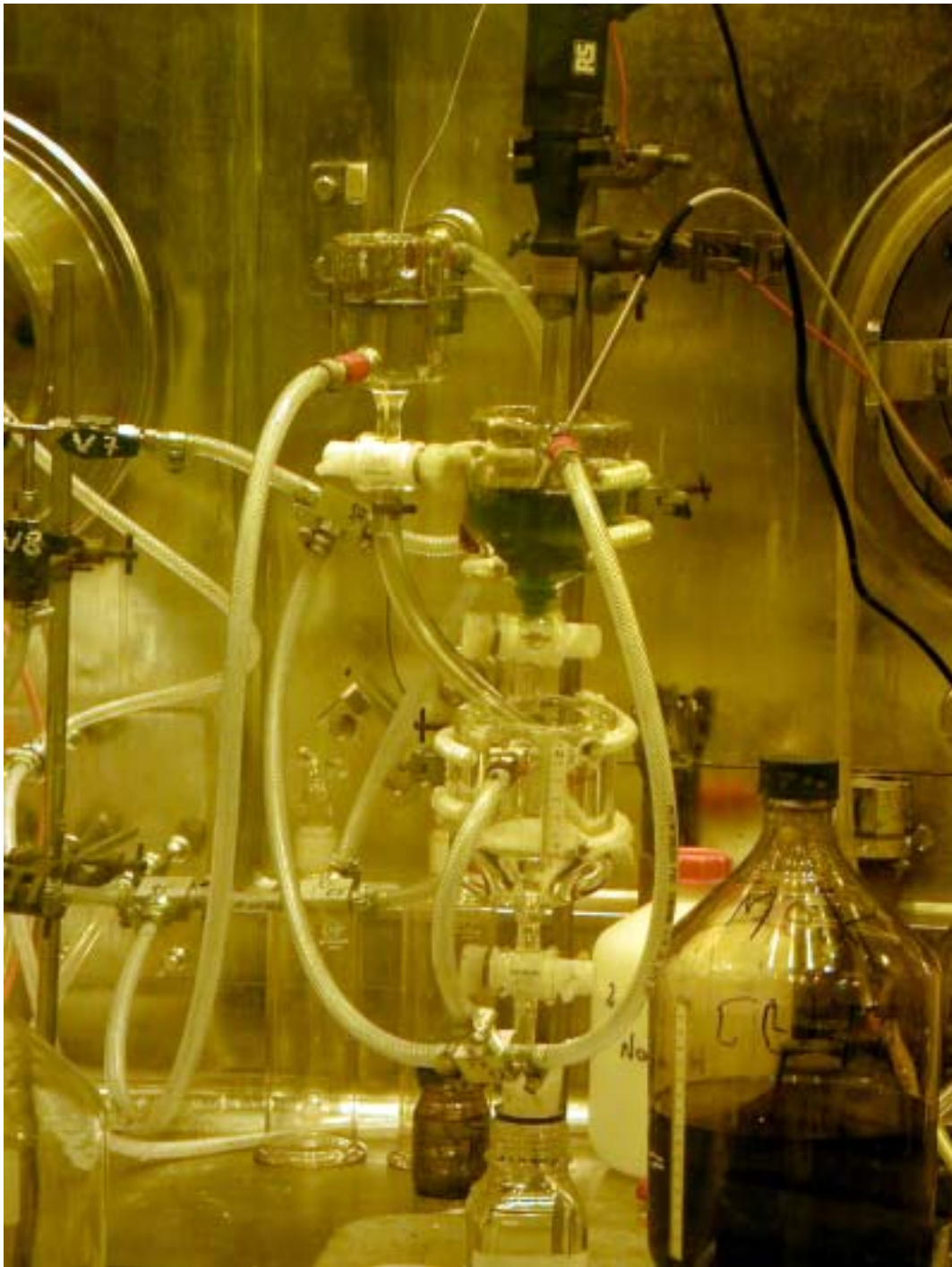
Photograph 1. MOX crystallisation equipment in hot cell
