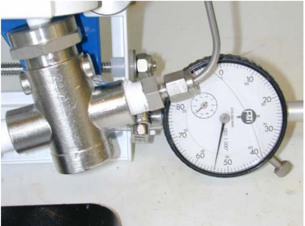
**Photograph 8. View of pump head for MOX feed with vernier setting gauge**
