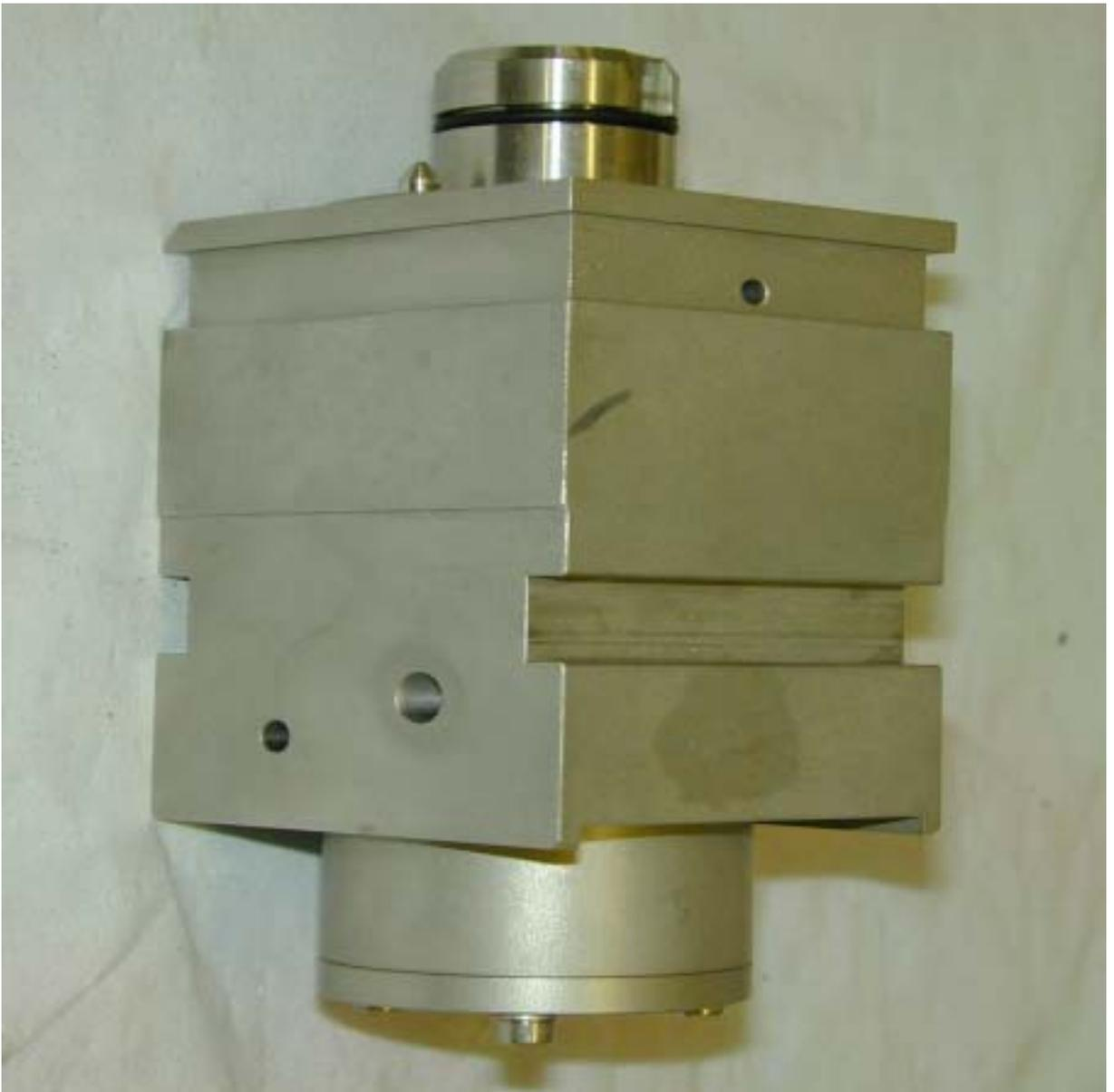
**Photograph 3. Complete Rousselet/Robatel BXP012 rotor and bowl assembly, looking from the side**
