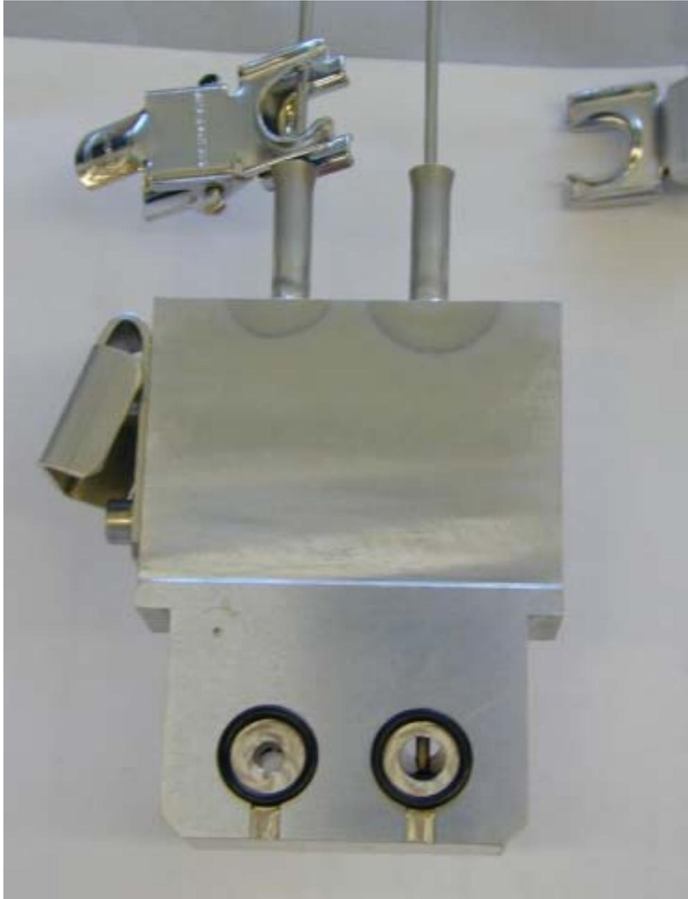
**Photograph 4. Close-up of Rousselet/Robatel BXP012 binding piece (also showing detail of syringe sampling system, with clip released and needle lowered into sampling position on right-hand side)**
