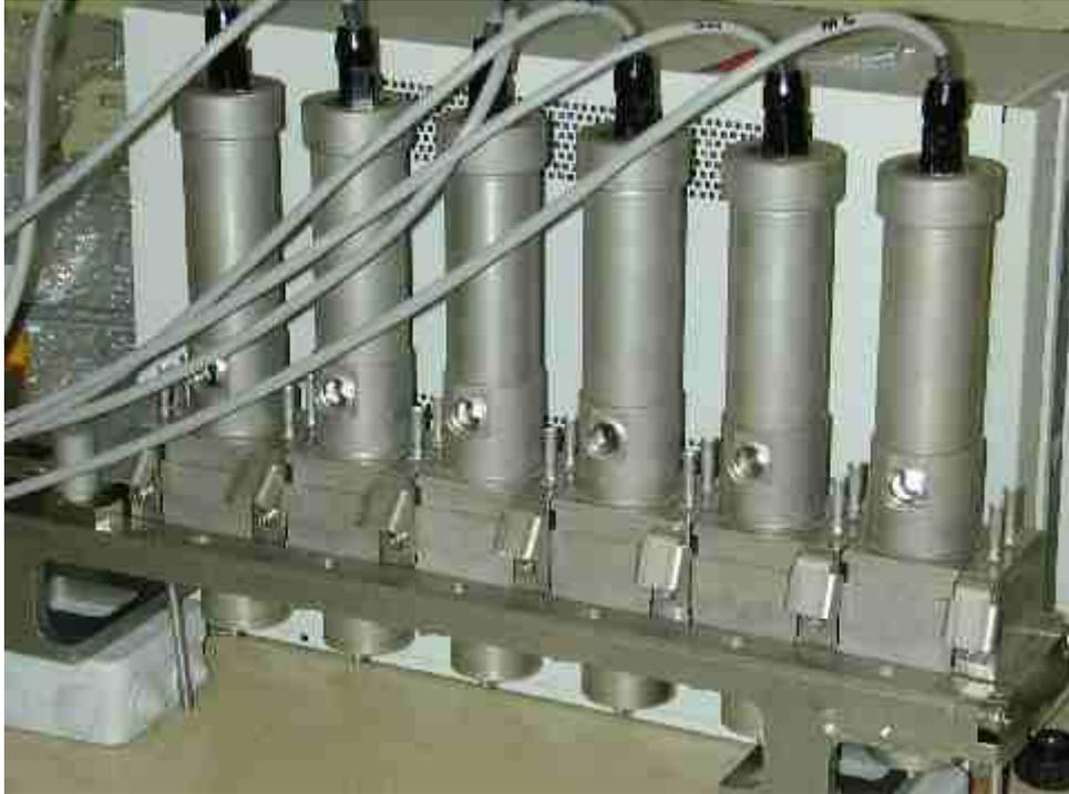
**Photograph 5. Complete assembly of Rousselet/Robatel BXP012 contactors, clamped with binding pieces to support rail**
