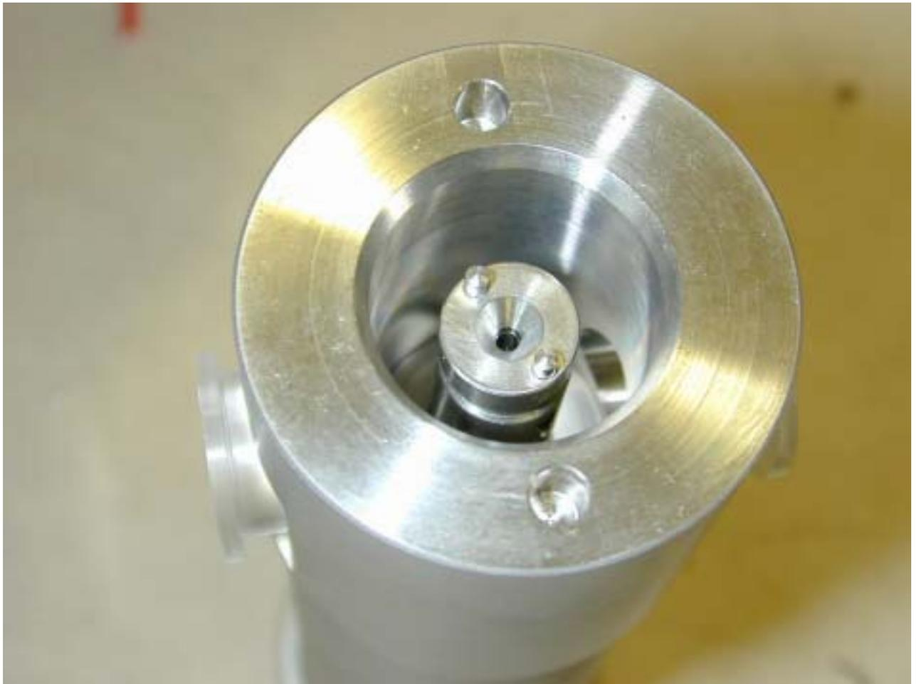
**Photograph 6. Motor housing for Rousselet/Robatel BXP012 contactor, from below, showing recesses for central and peripheral pins on rotor assembly and coupling**
