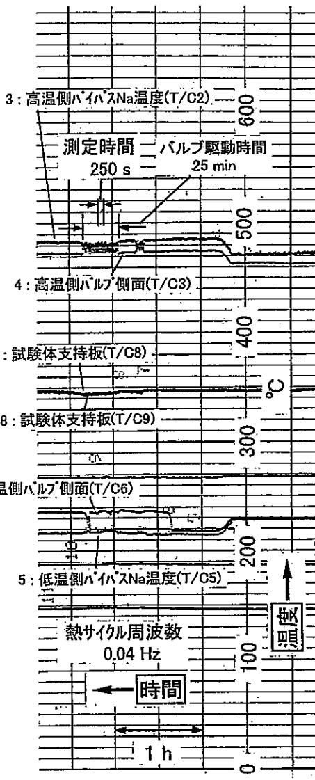
Appendix B-3 Sodium temperature under the experimental stage(3)
