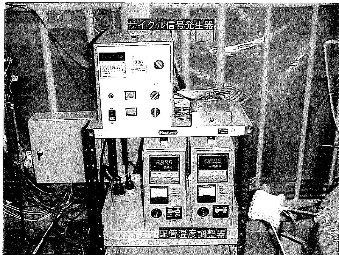
Fig.2-7 Frequency controller and temperature regulators
