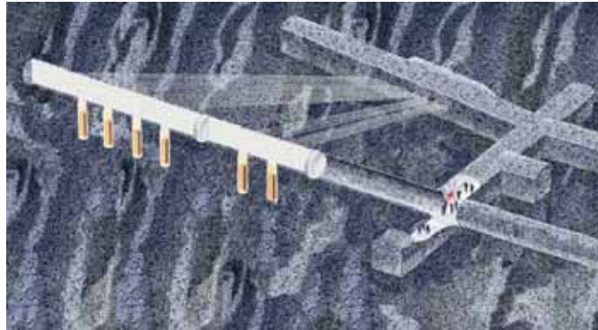
Figure 1. Schematic view of the Prototype Repository with one inner and one outer section.
