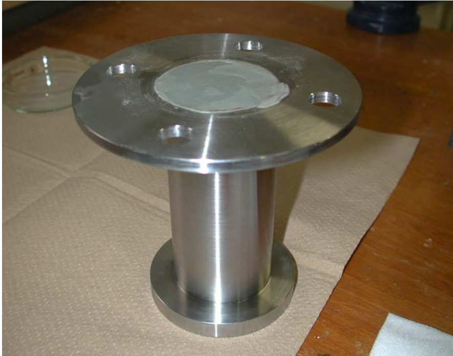
Fig. 4.1-1 Overview of the experimental column and bentonite disk distilled water, without PAA (W-B) upper part : inlet side (contacted PTFE filter)
