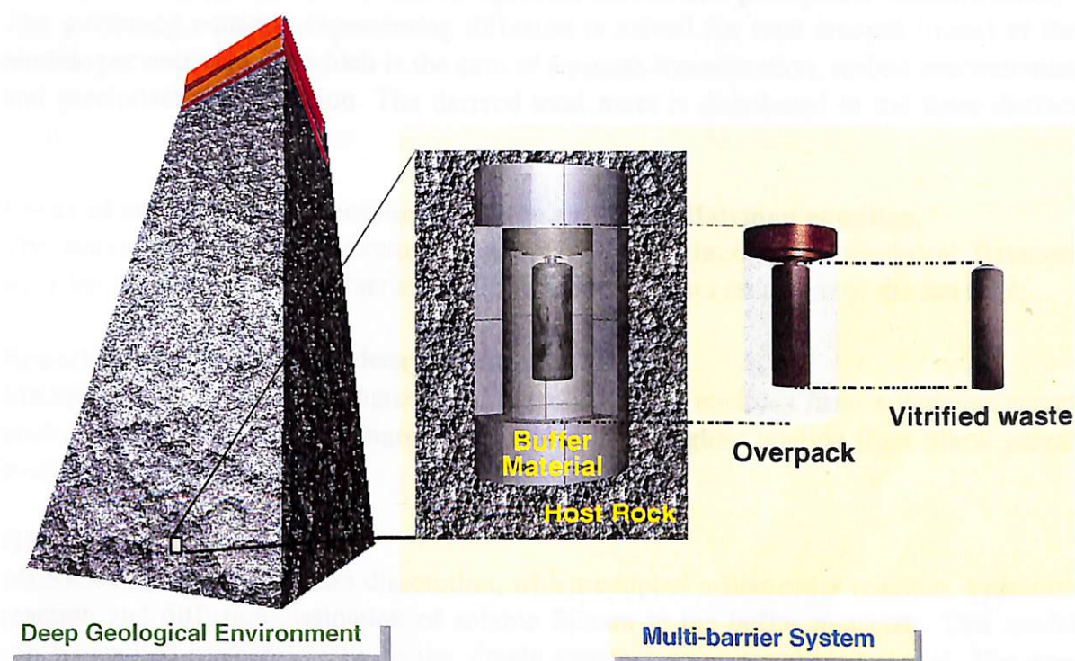
Figure 1-1 The basic concept of geological disposal in Japan
