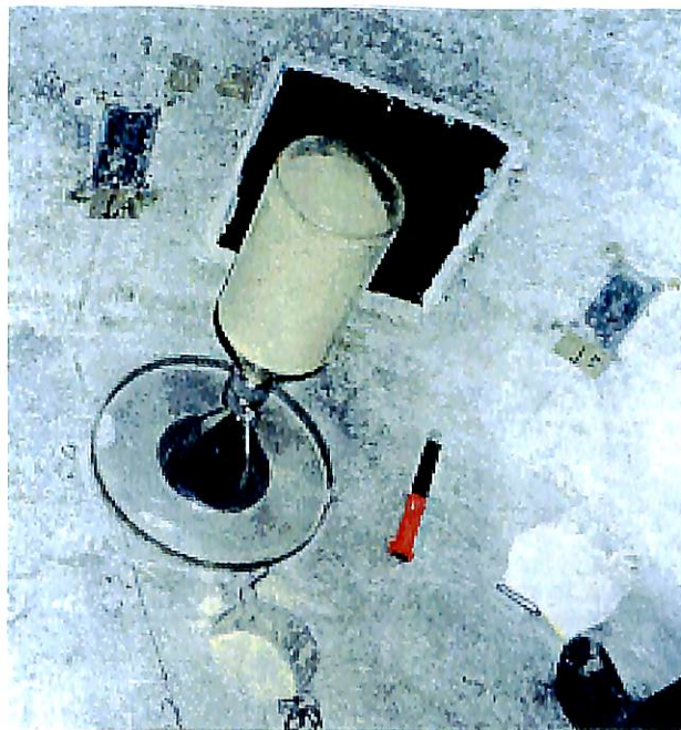
Figure 3-11 Schematic view of sand replacement method
