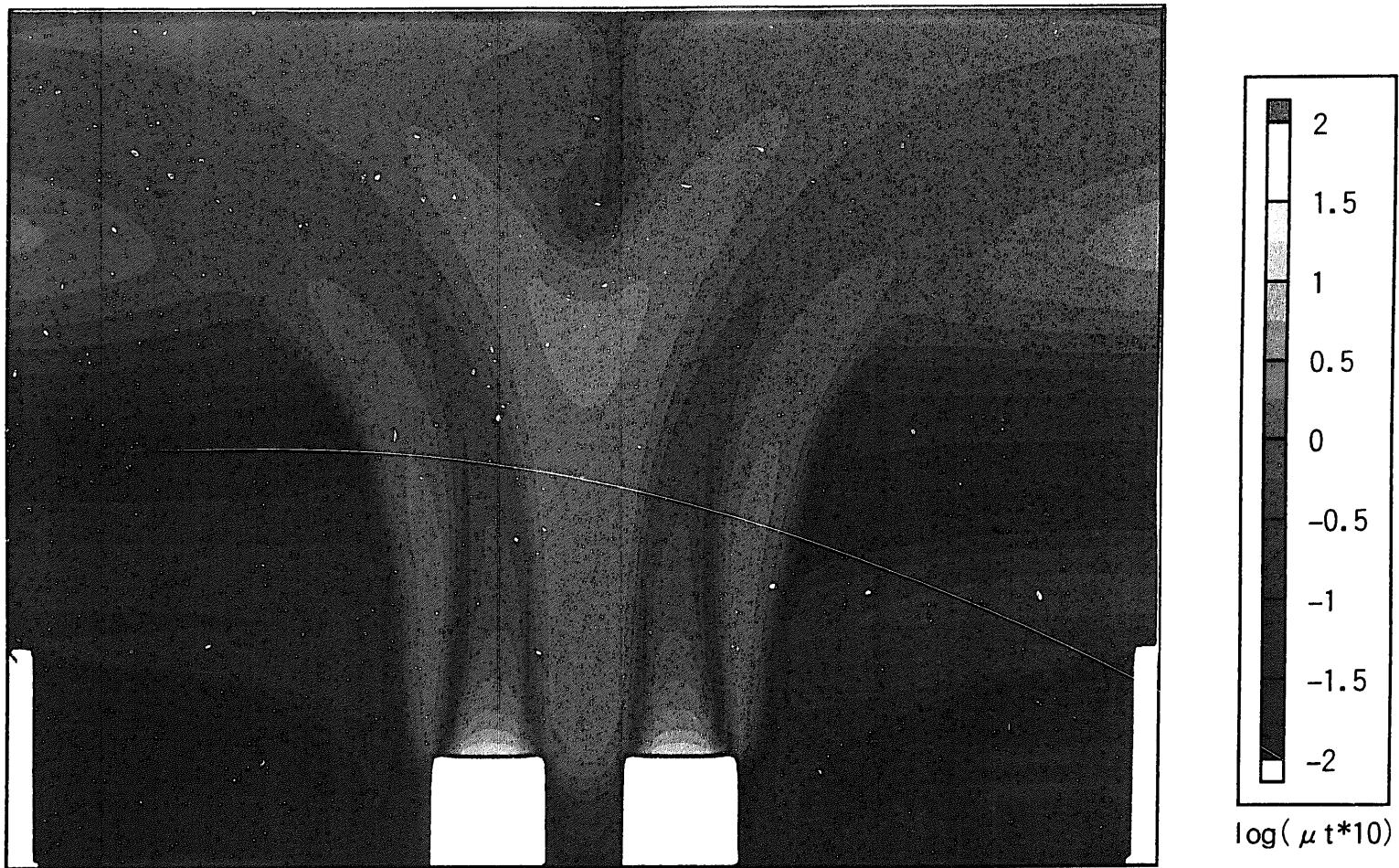
Fig.4-19 Pb: turbulent viscosity ( $\mu_t$ )
