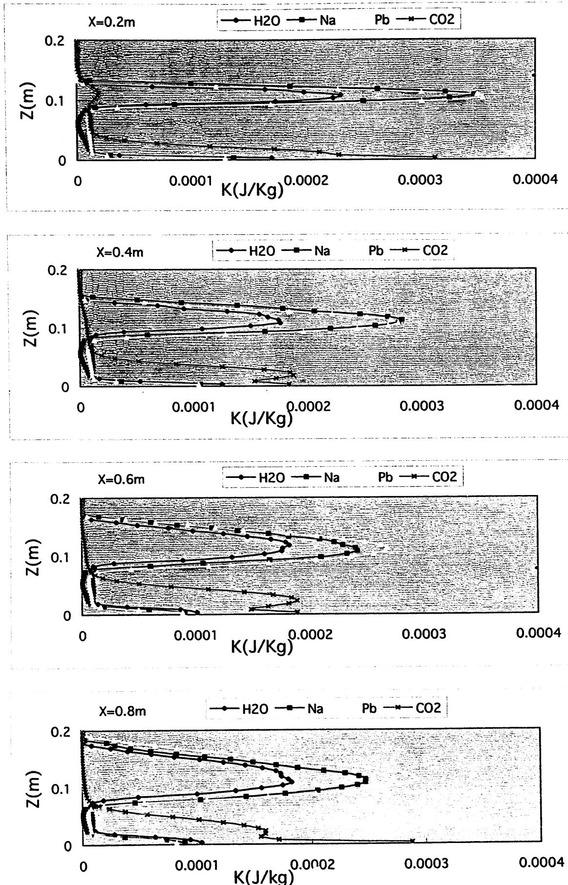
Fig.3-33 CASE1( $Ri=2, DV=0.084\text{m/s}$ ): turbulent kinetic energy( $K$ )
