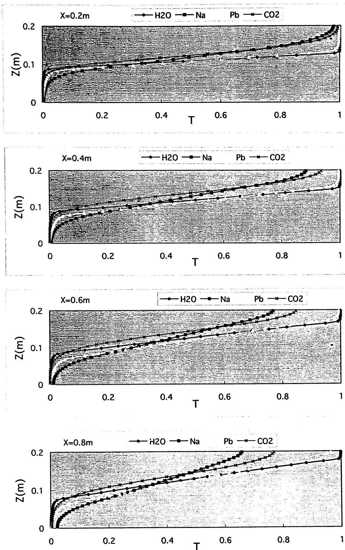
Fig.3-27 CASE1( $\text{Ri}=2, \text{DV}=0.084\text{m/s}$ ):normalized mean temperature
