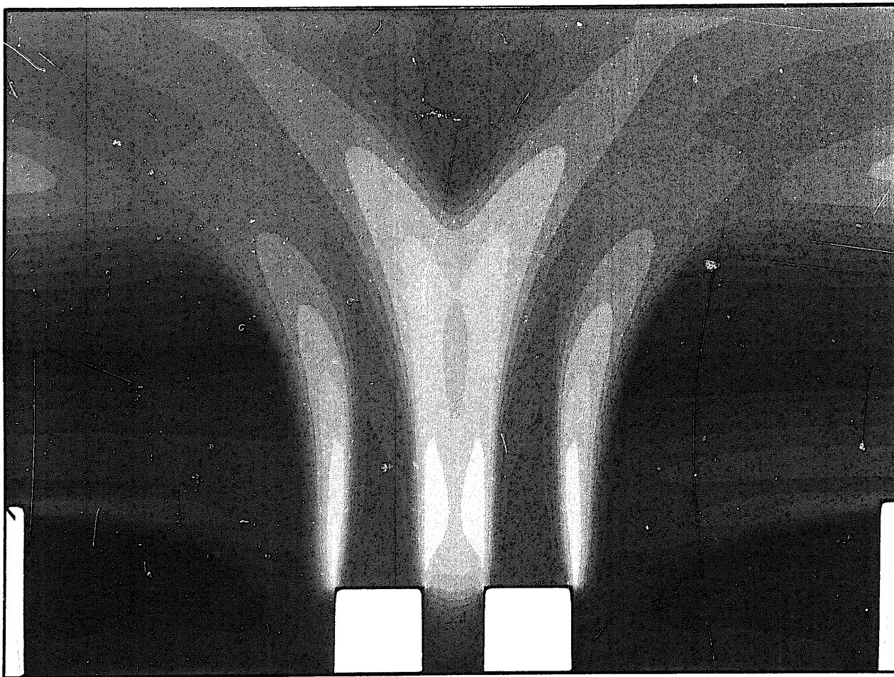
Fig.4-09 H20: turbulent kinetic energy(K)
