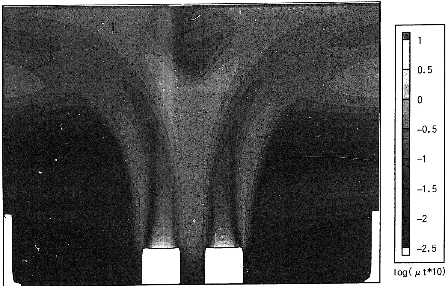
Fig.4-18 Na: turbulent viscosity ( $\mu_t$ )
