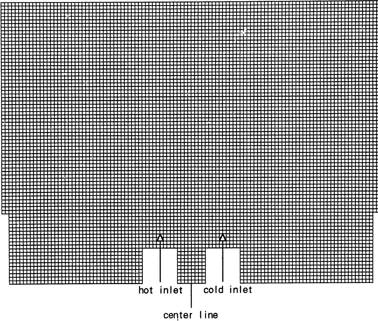
Fig.4-0 mesh arrangement for thermal striping
