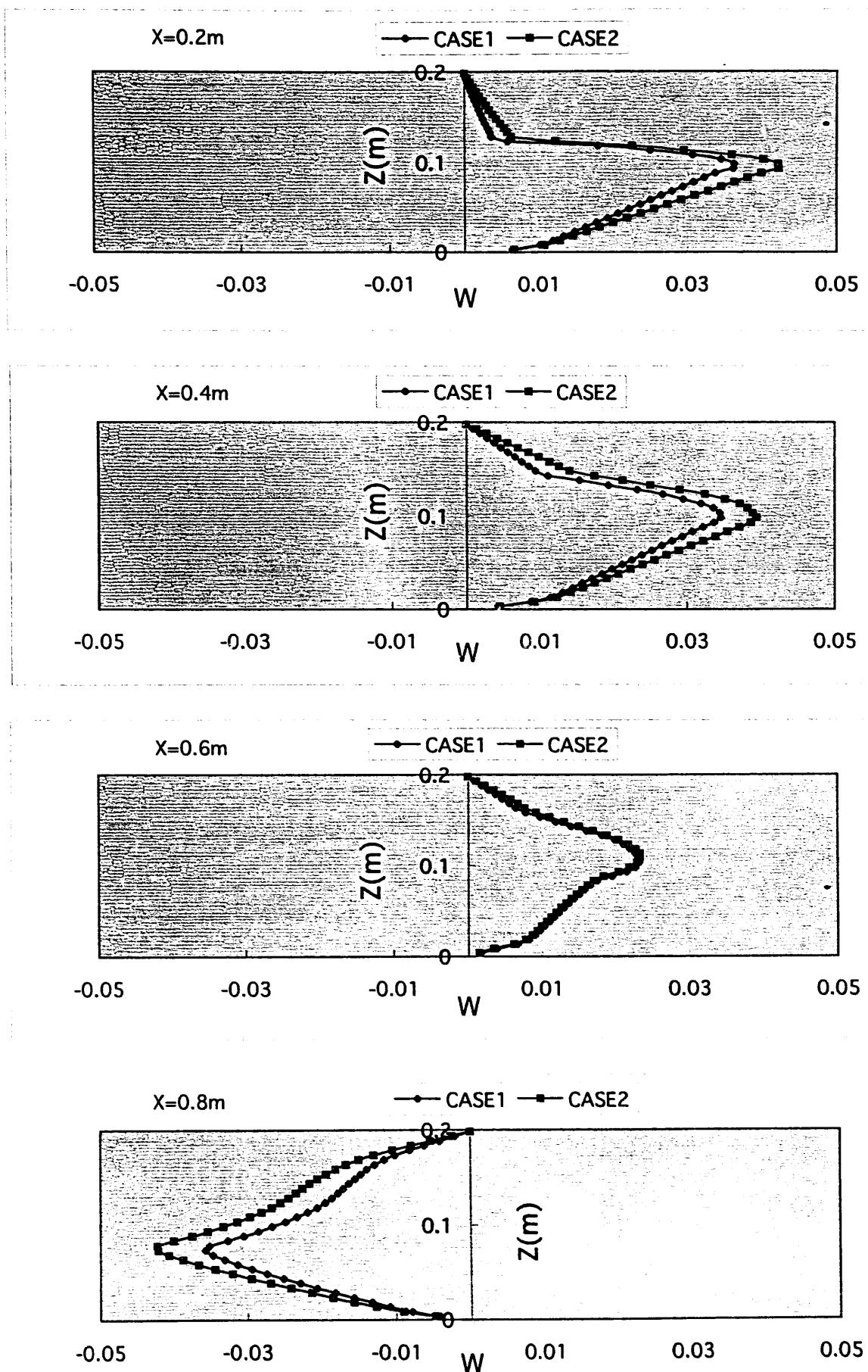
Fig.3-23 H<sub>2</sub>O: Z-direction normalized velocity
