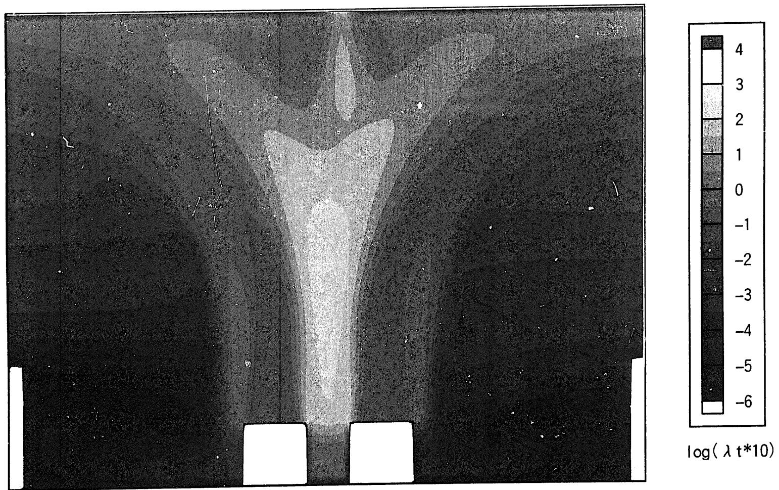
Fig. 4-23 Pb: turbulent conductivity ( $\lambda t$ )
