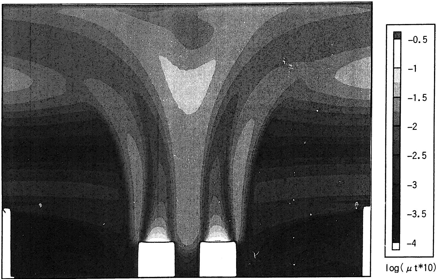
Fig.4-20 CO<sub>2</sub>: turbulent viscosity ( $\mu_t$ )
