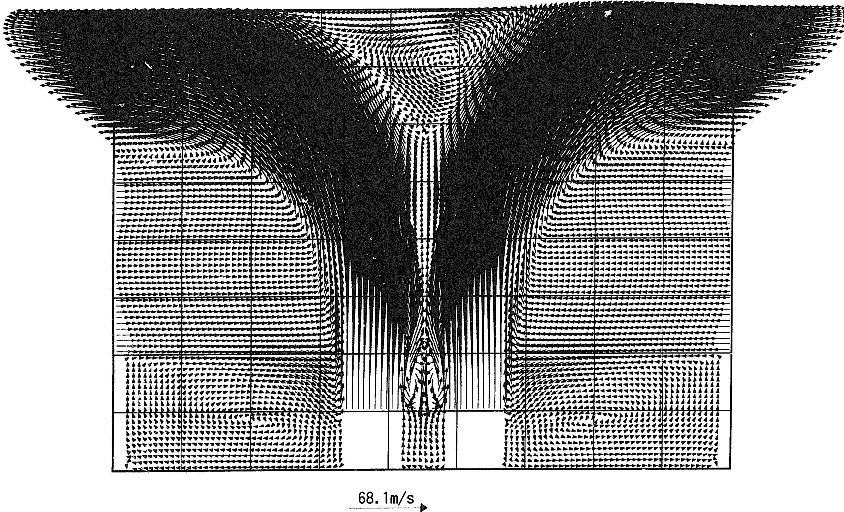
Fig.4-04 CO<sub>2</sub>: velocity field
