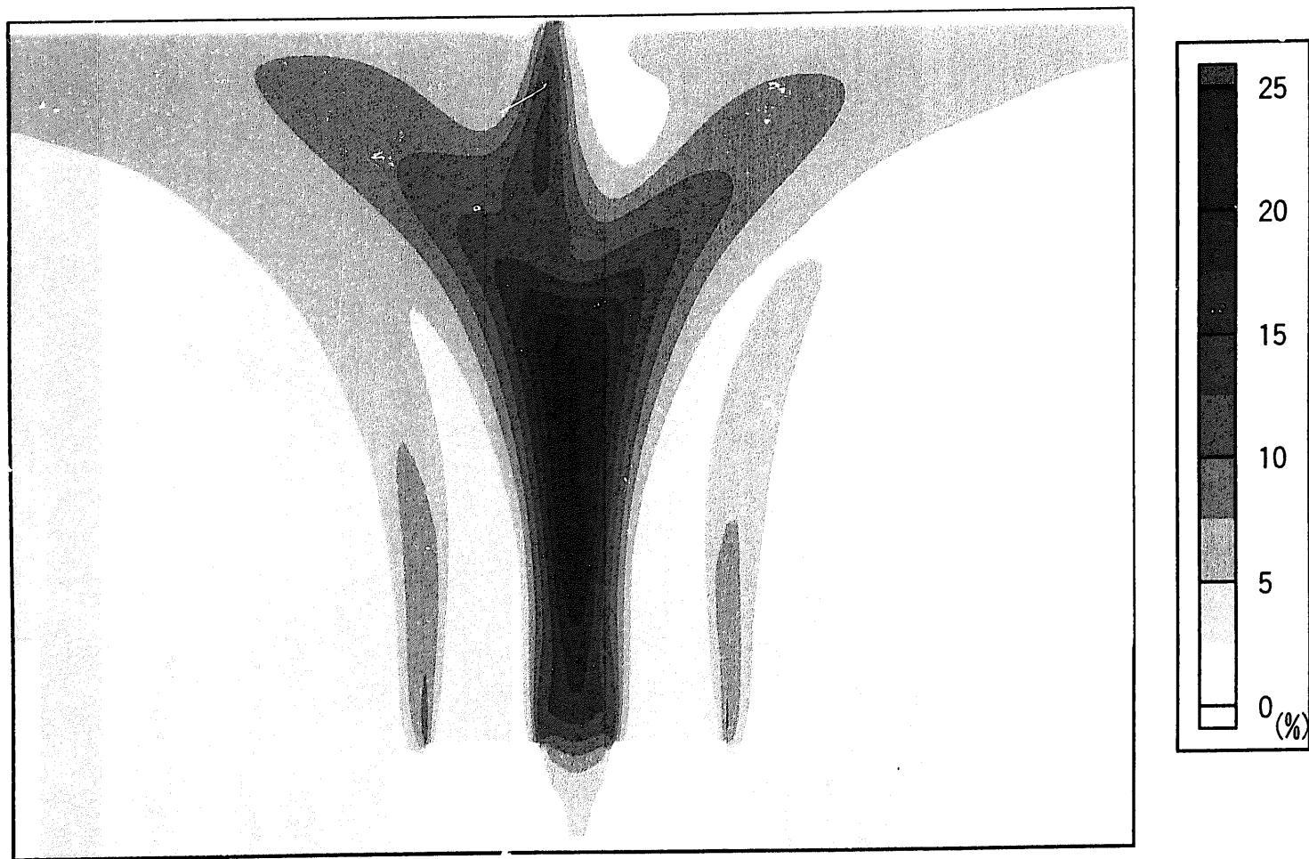
Fig.4-25 H<sub>2</sub>O: normalized temperature fluctuation
