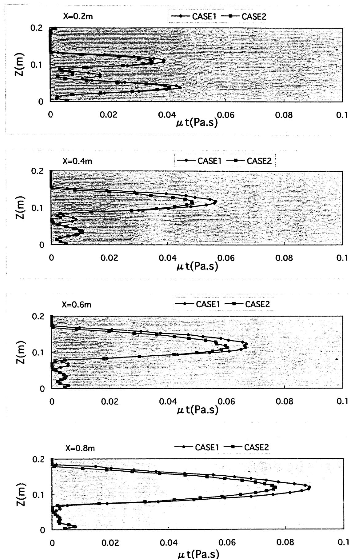
Fig.3-48 Na: turbulent viscosity ( $\mu t$ )
