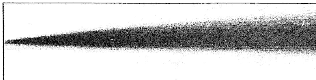
CASE24: CO<sub>2</sub> (V<sub>hi</sub>=0.033m/s, V<sub>ci</sub>=0.205m/s; T<sub>hi</sub>=400°C, T<sub>ci</sub>=380°C)
