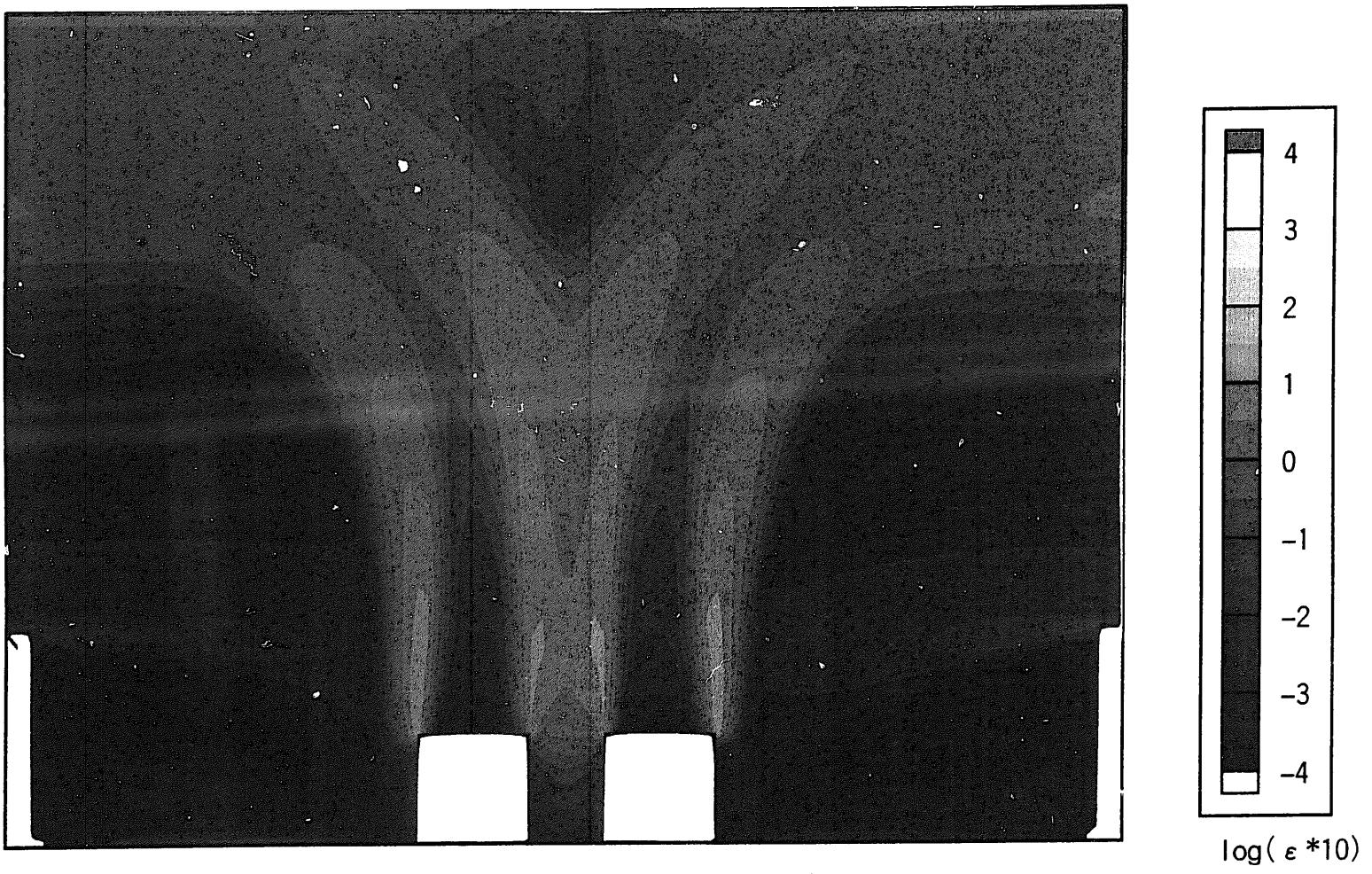
Fig.4-15 Pb: dissipation rate of K ( $\epsilon$ )
