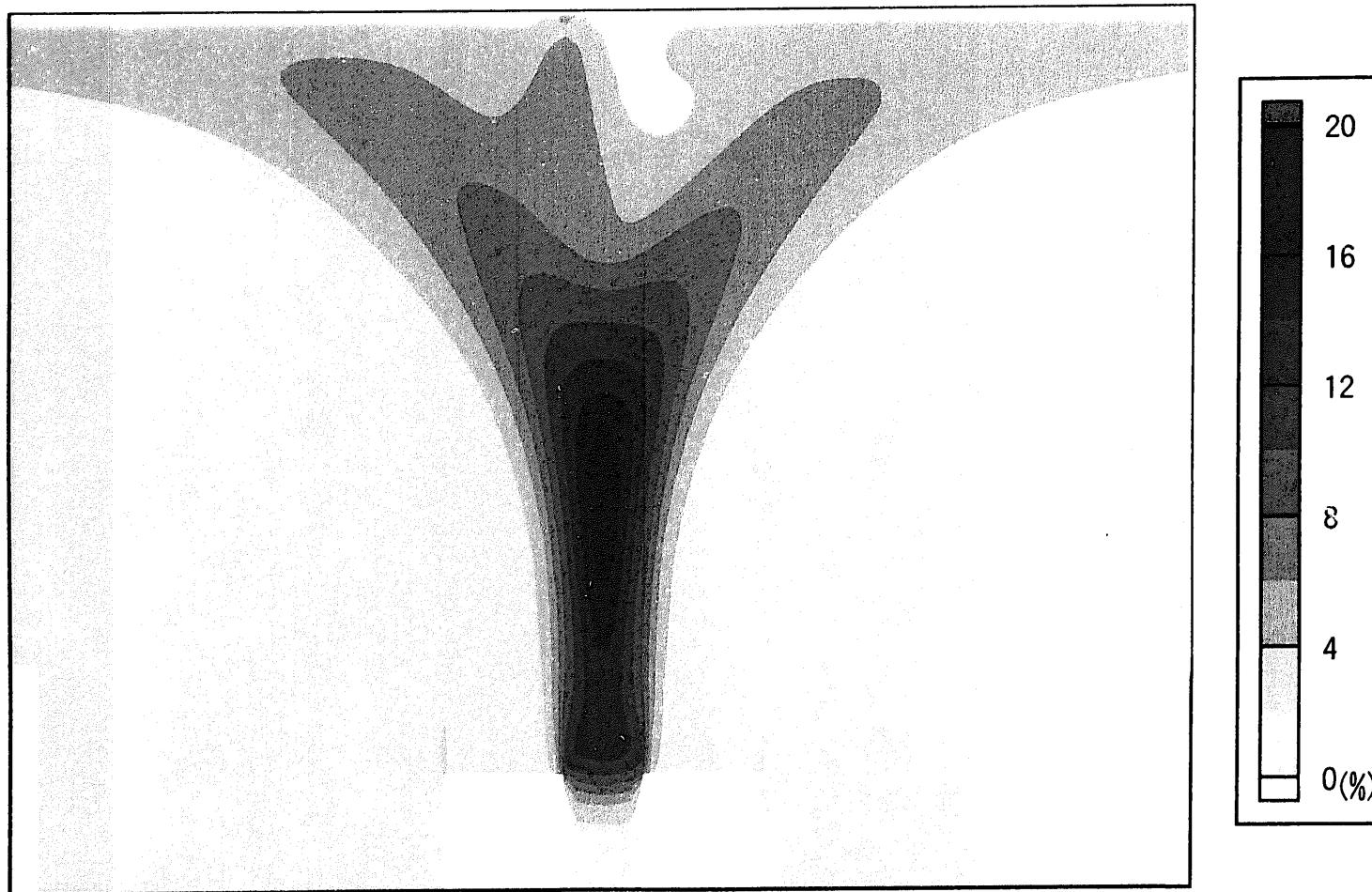
Fig.4-26 Na: normalized temperature fluctuation
