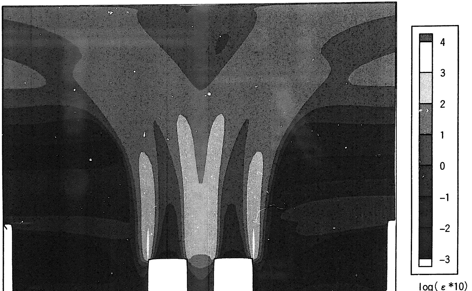
Fig.4-14 Na: dissipation rate of  $K(\epsilon)$
