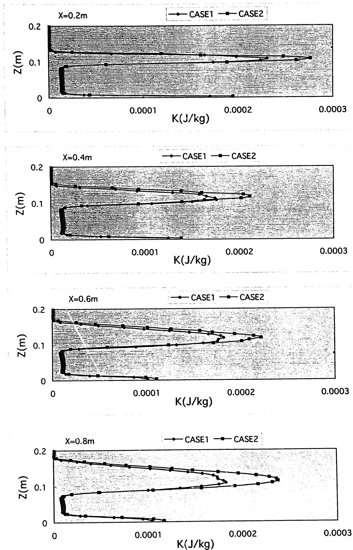
Fig.3-35 H<sub>2</sub>O: turbulent kinetic energy( $K$ )
