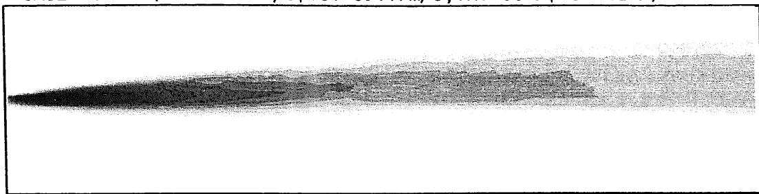
CASE12: Na (V<sub>hi</sub>=0.033m/s, V<sub>ci</sub>=0.117m/s; T<sub>hi</sub>=472.63°C, T<sub>ci</sub>=447.37°C)
