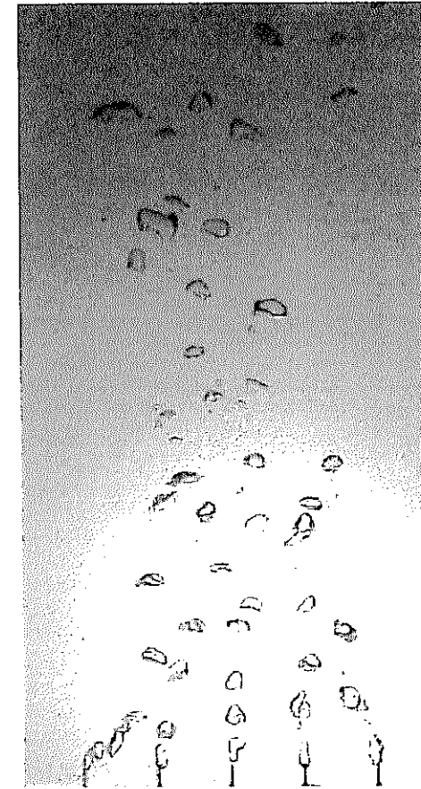
(c) steam and nitrogen gas ( T_f = 99^\circ\text{C} , Q_s = 539 \text{ L/hr} , Q_n = 15 \text{ L/hr} ) Volume fraction of nitrogen: 2.7%
