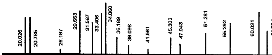
Fig. 6: X-ray diffraction pattern of \beta\text{-NaFeO}_2 reported by Watanabe and Fukase
