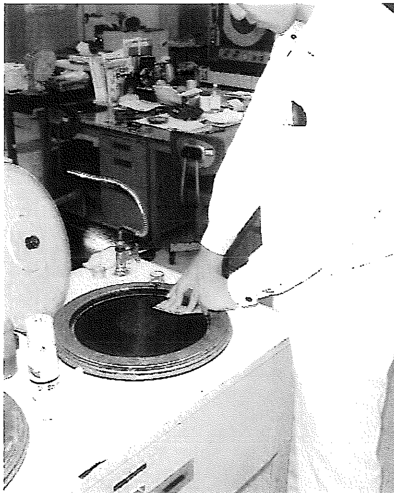
Photo 3-3 View of polishing process for tensile test specimen 引張試験片の研磨工程状況
